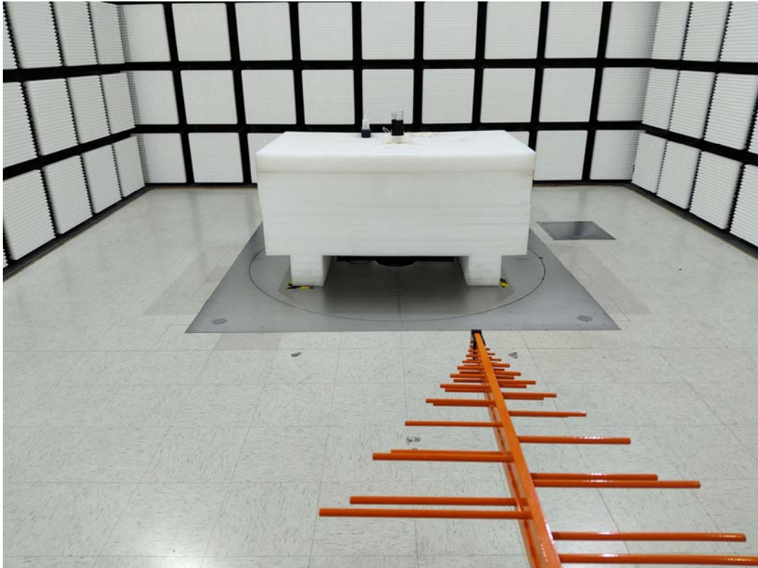
Radiated Emission 30 MHz-1 GHz View
