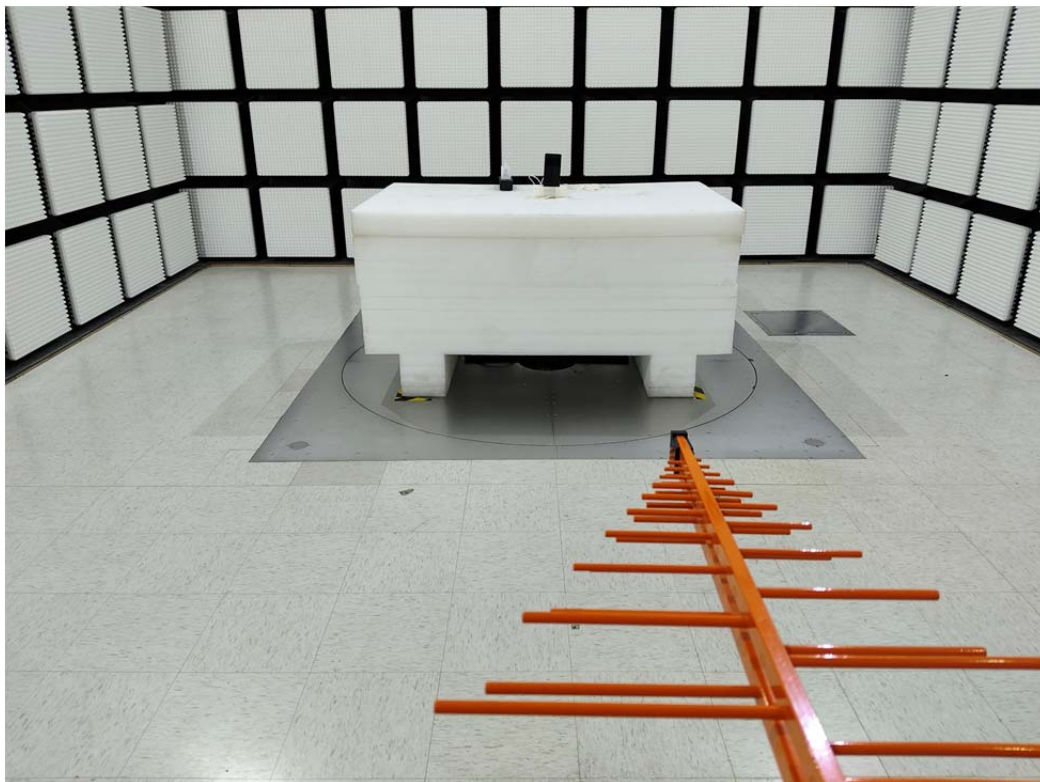
Radiated Emission 30 MHz-1 GHz View Adapter
