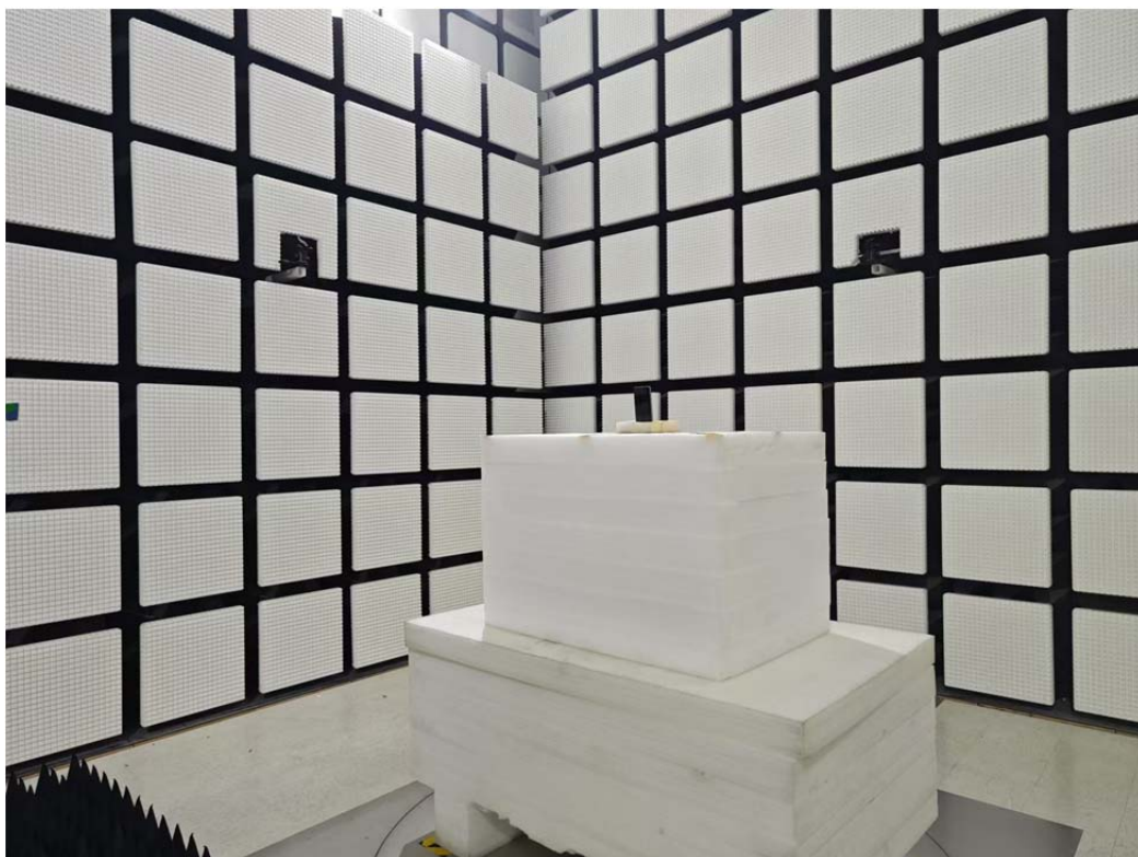
Radiated Emission Above 18-25GHz View
