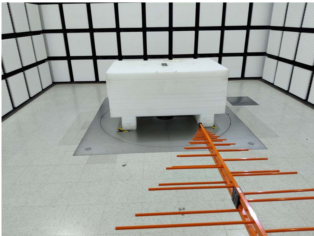
Radiated Emission 30 MHz-1 GHz View Earphone
