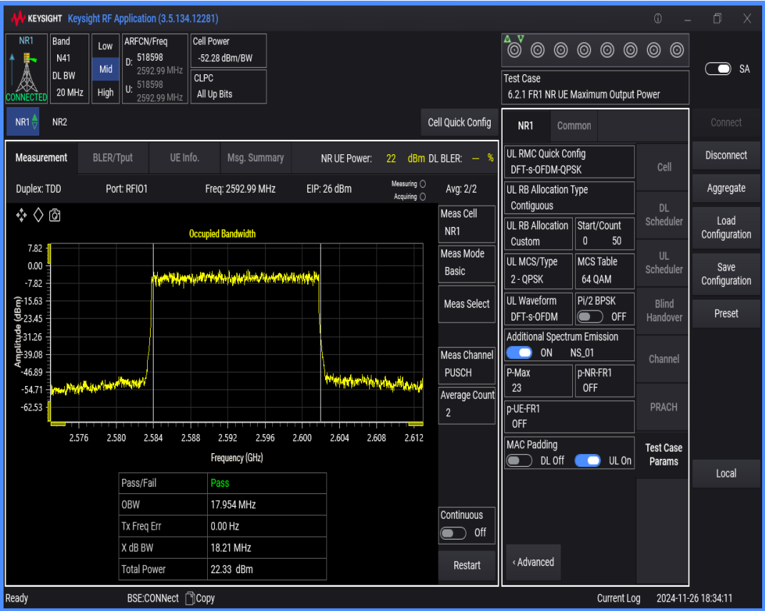
n41 SCS=30kHz DFT_QAM64 BW=50MHz Channel=518598 RB=128@0
