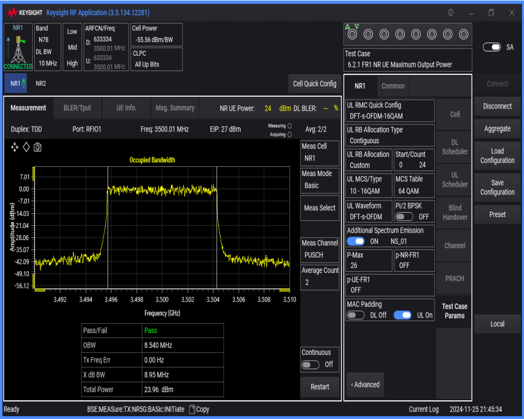
n78(3450-3550) SCS=30kHz DFT_QAM16 BW=20MHz Channel=633334 RB=50@0
