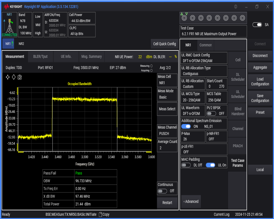
n78(3450-3550) SCS=30kHz DFT_QAM256 BW=10MHz Channel=633334 RB=24@0
