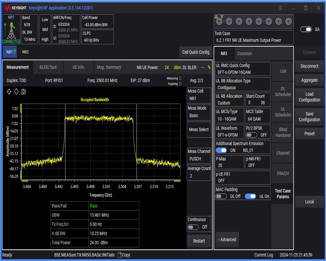
n78(3450-3550) SCS=30kHz DFT_QAM16 BW=50MHz Channel=633334 RB=128@0
