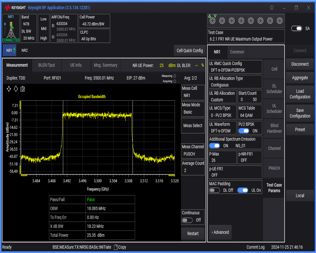
n78(3450-3550) SCS=30kHz DFT_BPSK BW=15MHz Channel=633334 RB=36@0
