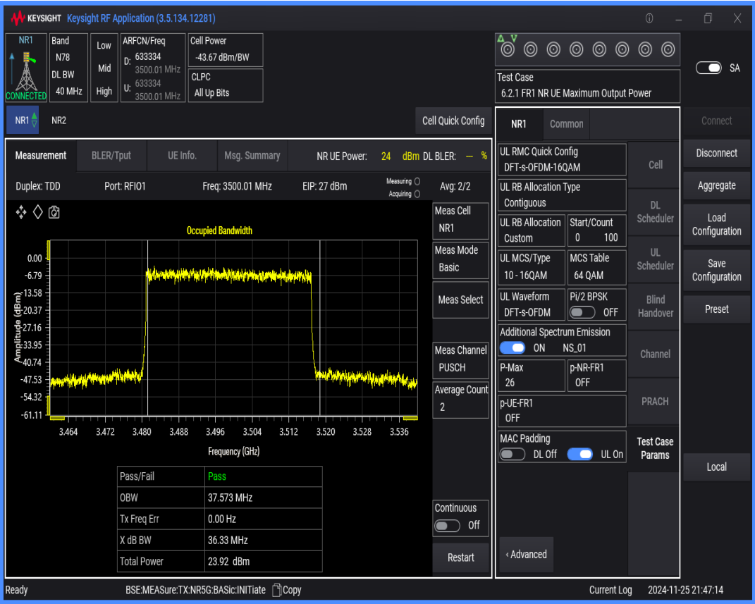
n78(3450-3550) SCS=30kHz DFT_QAM16 BW=30MHz Channel=633334 RB=75@0
