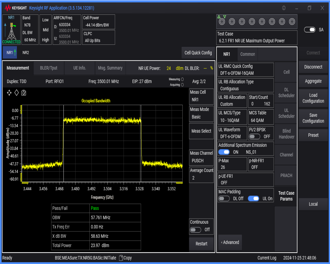
n78(3450-3550) SCS=30kHz DFT_QAM256 BW=100MHz Channel=633334 RB=270@0
