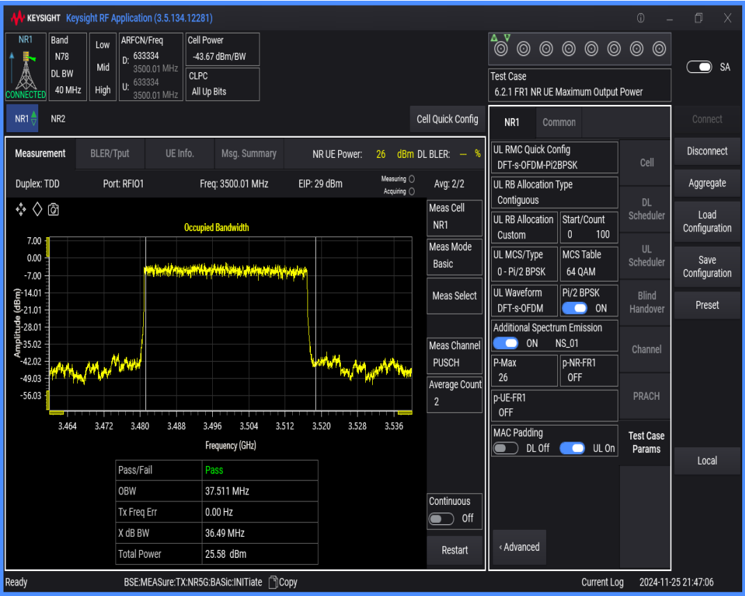
n78(3450-3550) SCS=30kHz DFT_BPSK BW=30MHz Channel=633334 RB=75@0
