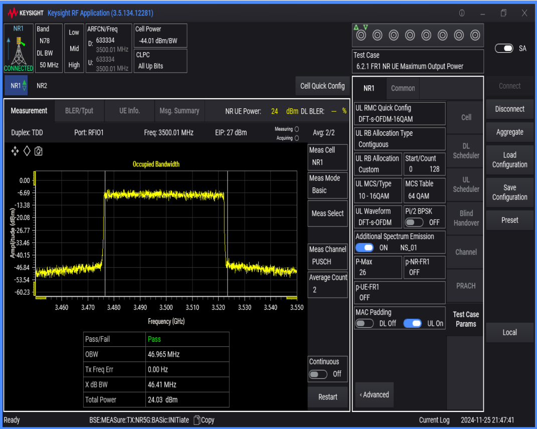
n78(3450-3550) SCS=30kHz DFT_QAM16 BW=40MHz Channel=633334 RB=100@0
