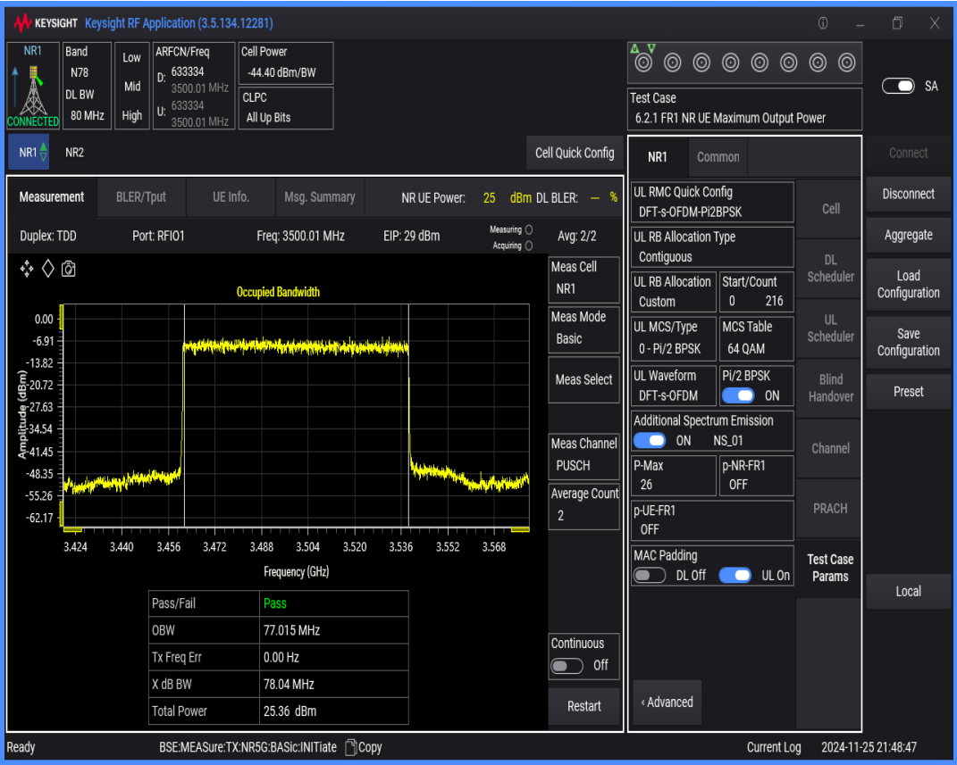
n78(3450-3550) SCS=30kHz DFT_QAM16 BW=100MHz Channel=633334 RB=270@0
