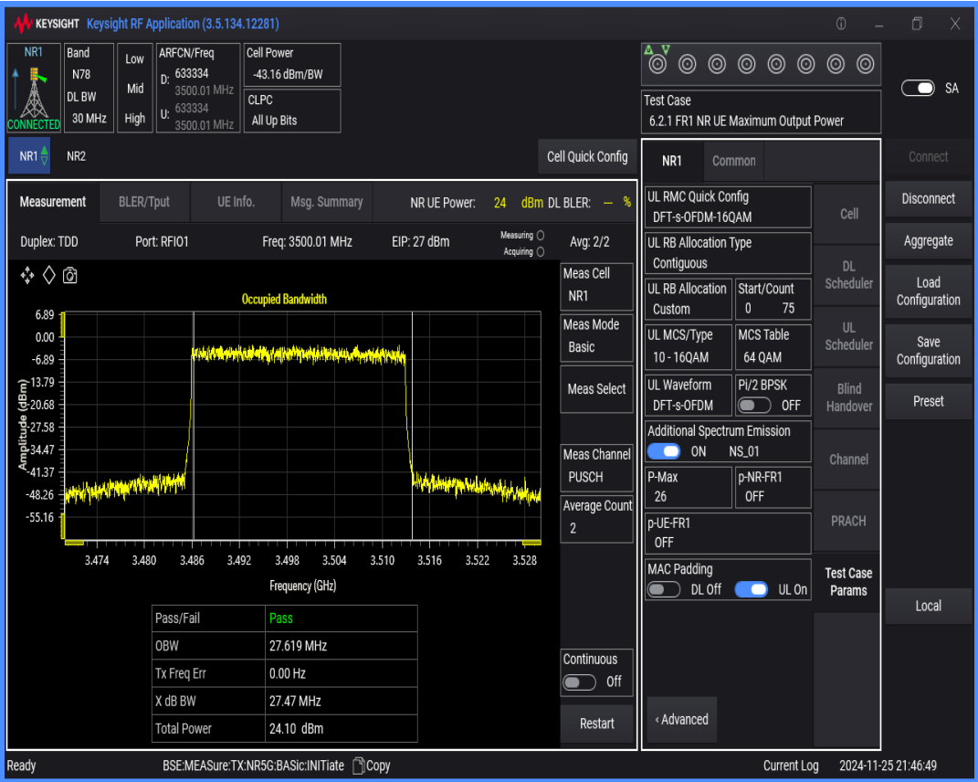
n78(3450-3550) SCS=30kHz DFT_QAM16 BW=60MHz Channel=633334 RB=162@0
