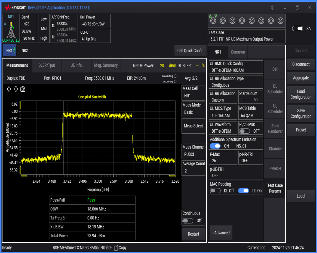
n78(3450-3550) SCS=30kHz DFT_QAM16 BW=15MHz Channel=633334 RB=36@0
