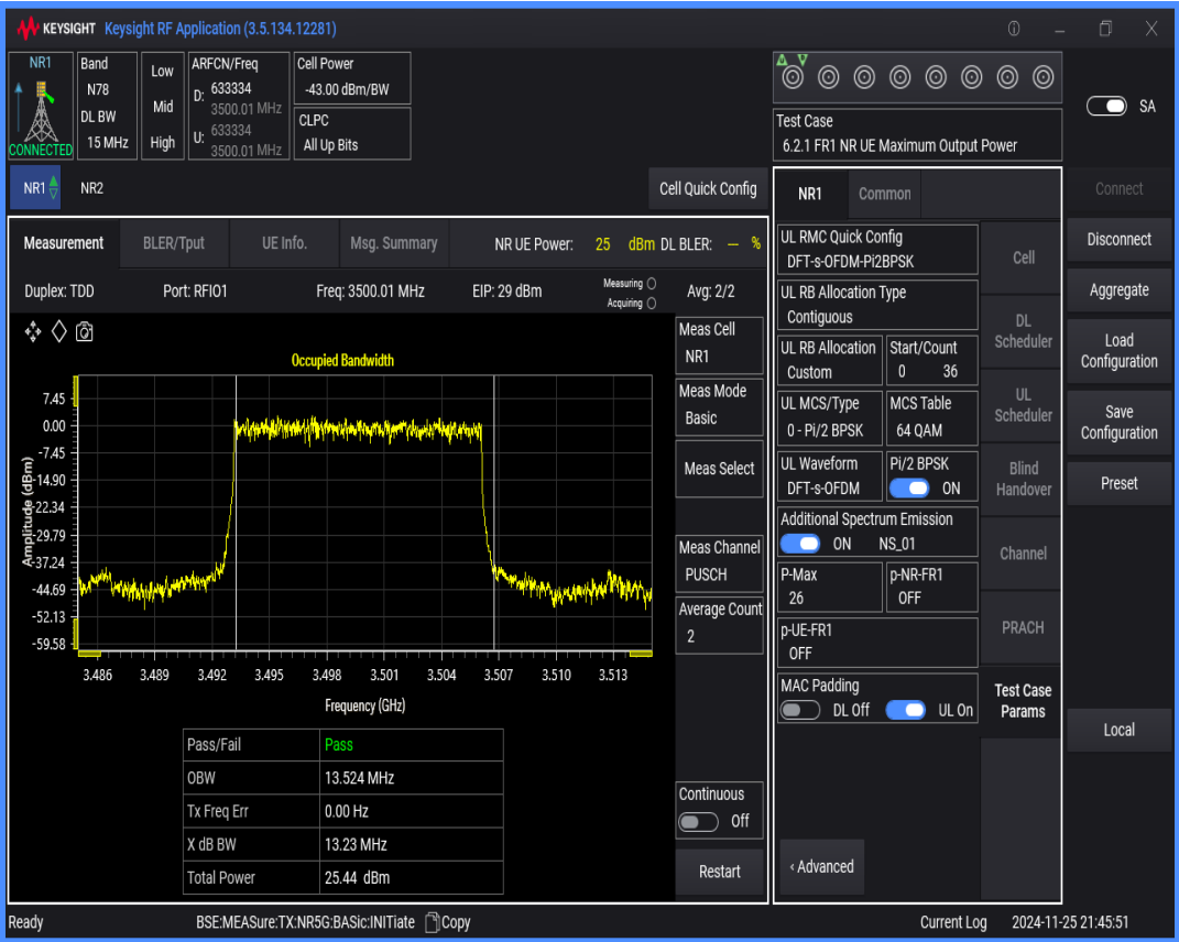
n78(3450-3550) SCS=30kHz DFT_BPSK BW=40MHz Channel=633334 RB=100@0
