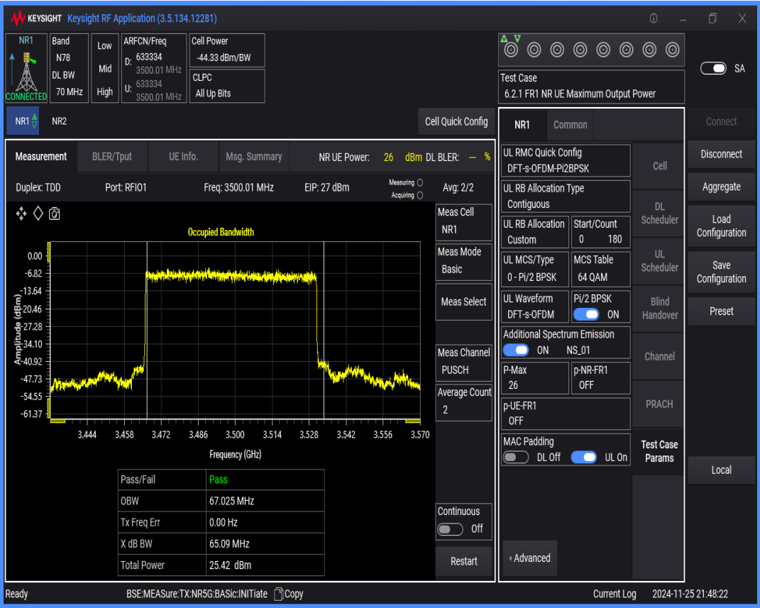
n78(3450-3550) SCS=30kHz DFT_BPSK BW=90MHz Channel=633334 RB=240@0
