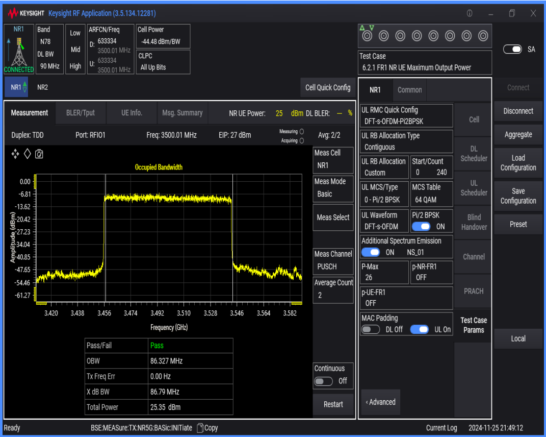
n78(3450-3550) SCS=30kHz DFT_BPSK BW=80MHz Channel=633334 RB=216@0
