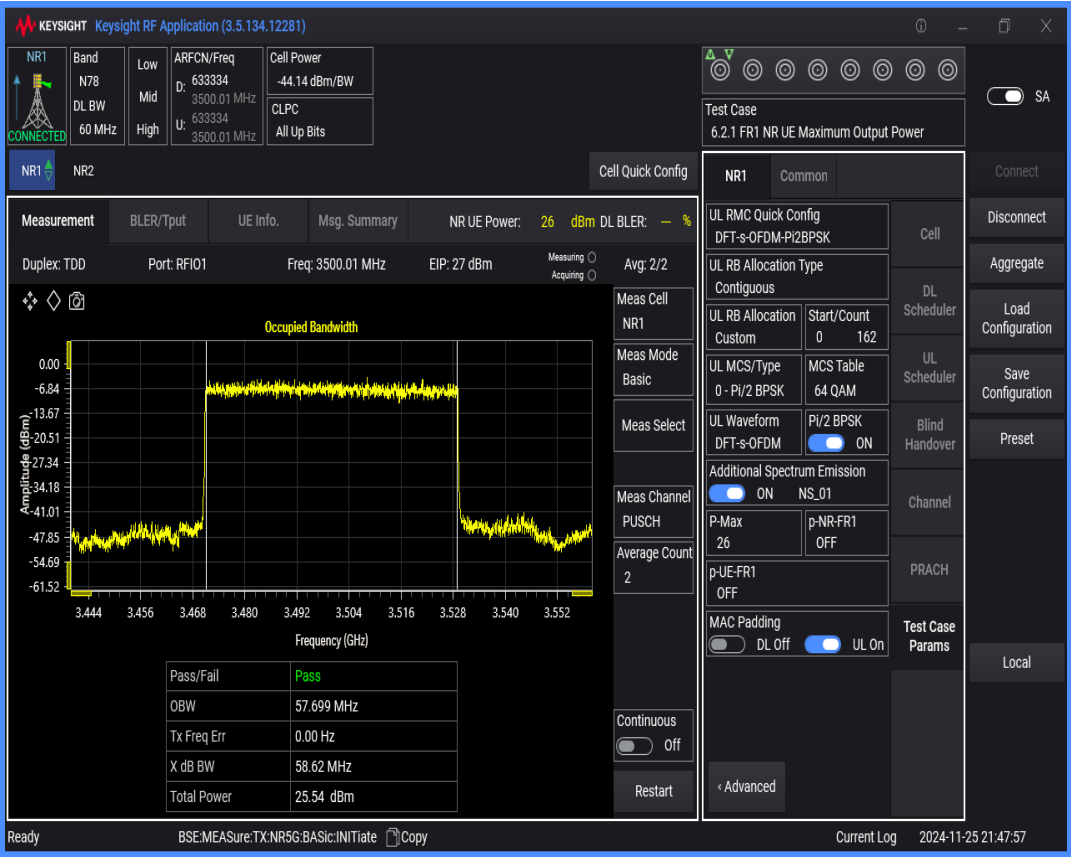
n78(3450-3550) SCS=30kHz DFT_BPSK BW=50MHz Channel=633334 RB=128@0
