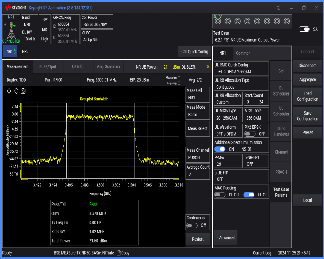
n78(3450-3550) SCS=30kHz DFT_QAM16 BW=90MHz Channel=633334 RB=240@0
