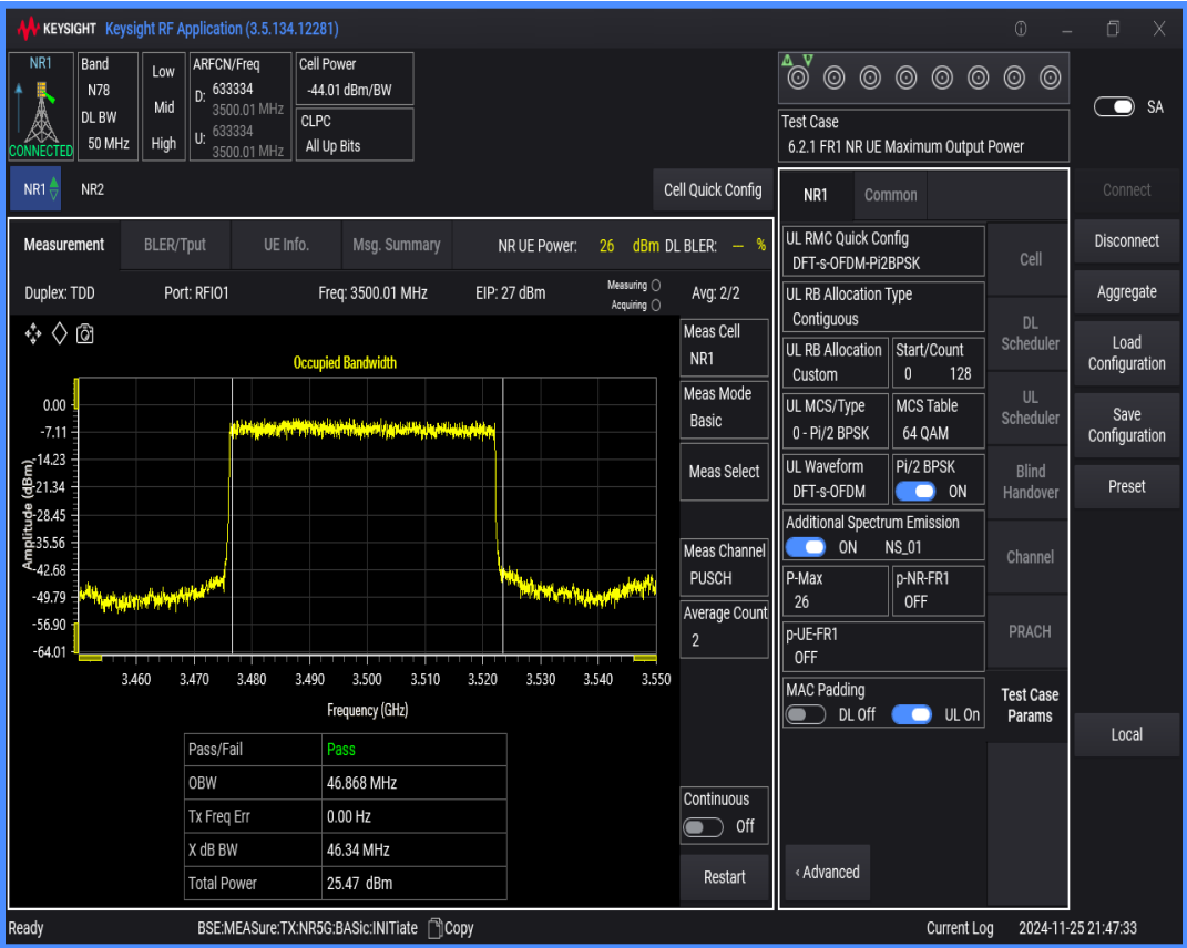
n78(3450-3550) SCS=30kHz DFT_BPSK BW=70MHz Channel=633334 RB=180@0
