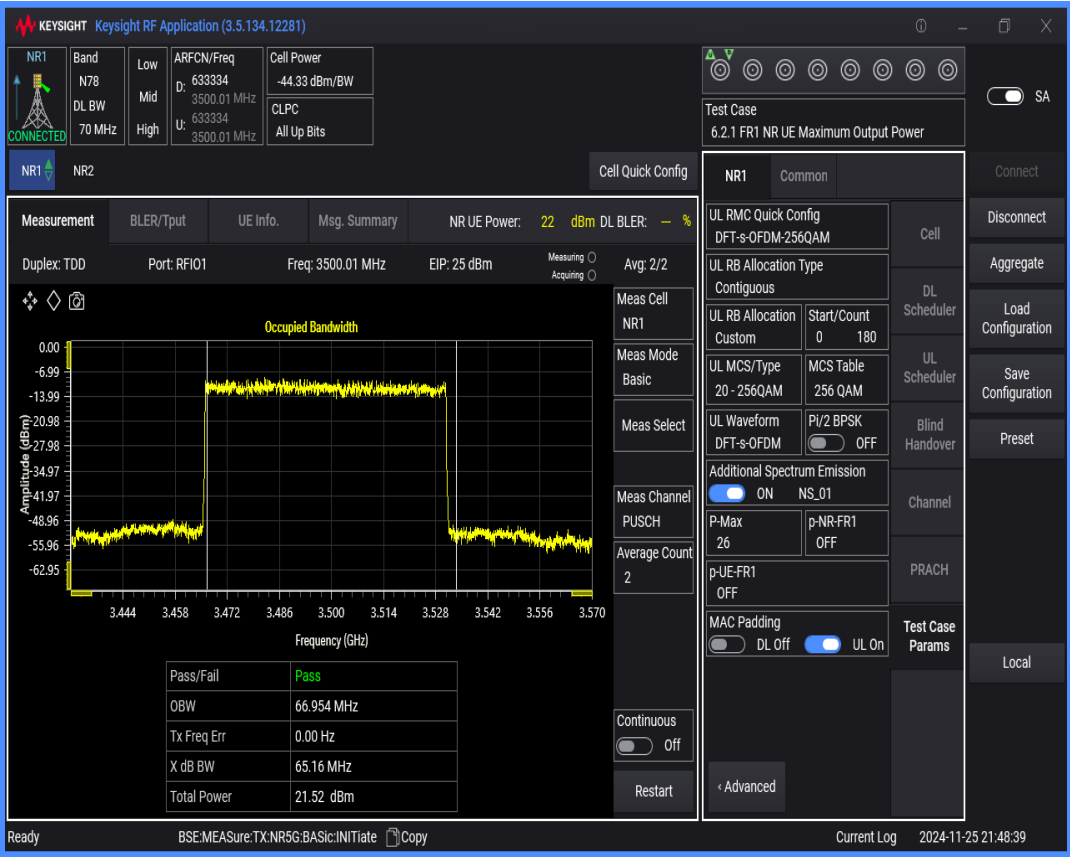
n78(3450-3550) SCS=30kHz DFT_QAM64 BW=100MHz Channel=633334 RB=270@0
