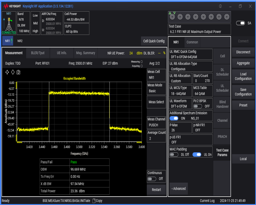
n78(3450-3550) SCS=30kHz DFT_QAM256 BW=90MHz Channel=633334 RB=240@0
