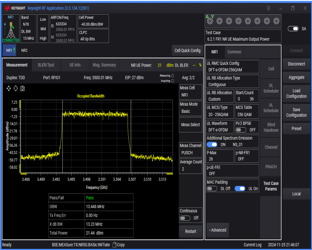
n78(3450-3550) SCS=30kHz DFT_QAM256 BW=40MHz Channel=633334 RB=100@0
