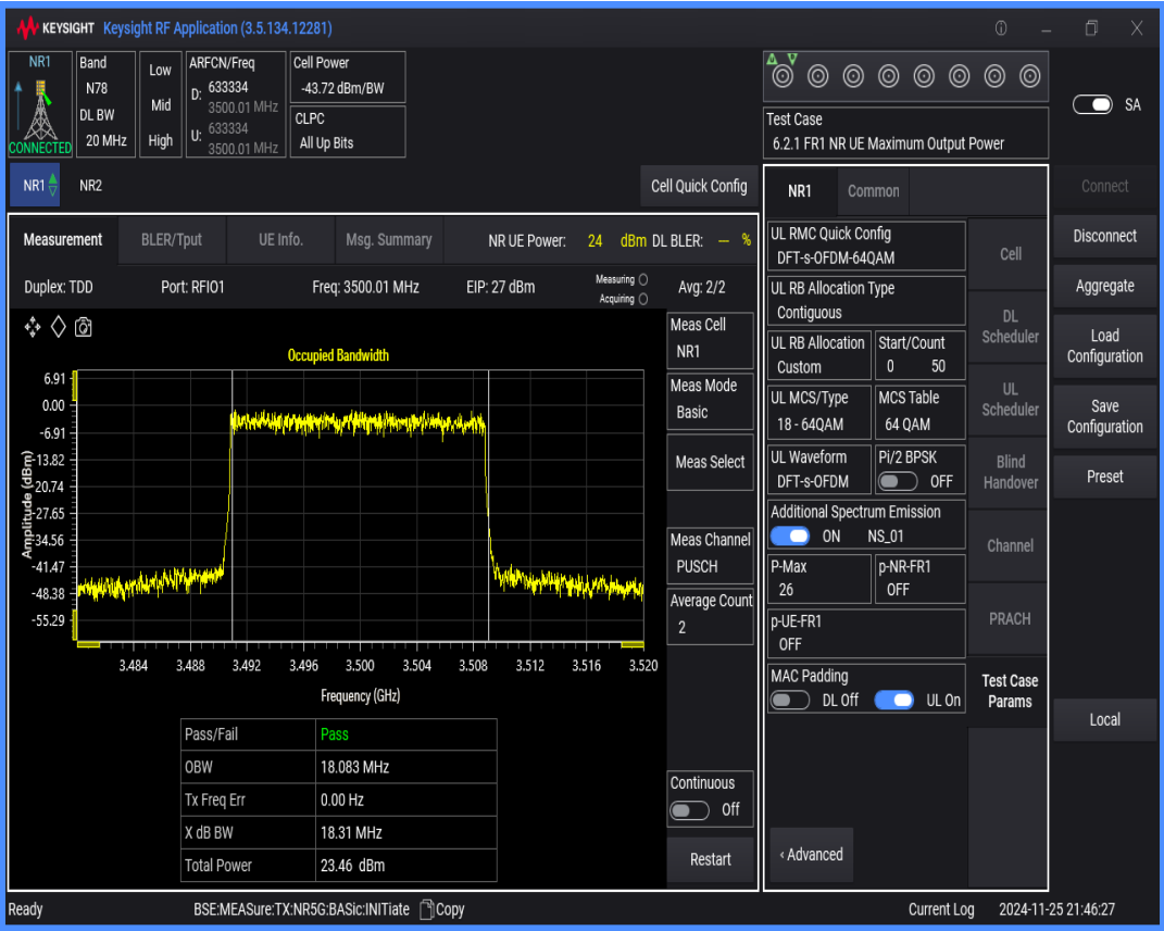
n78(3450-3550) SCS=30kHz DFT_QAM64 BW=10MHz Channel=633334 RB=24@0
