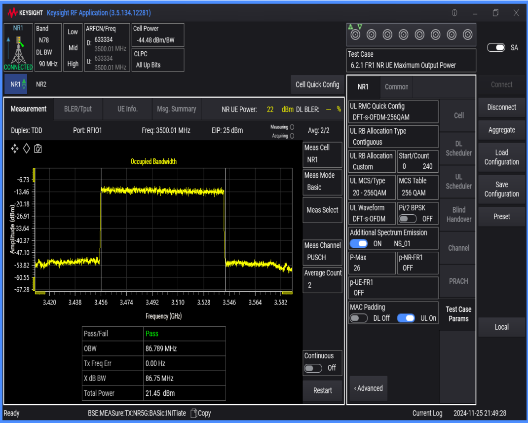
n78(3450-3550) SCS=30kHz DFT_QAM256 BW=80MHz Channel=633334 RB=216@0
