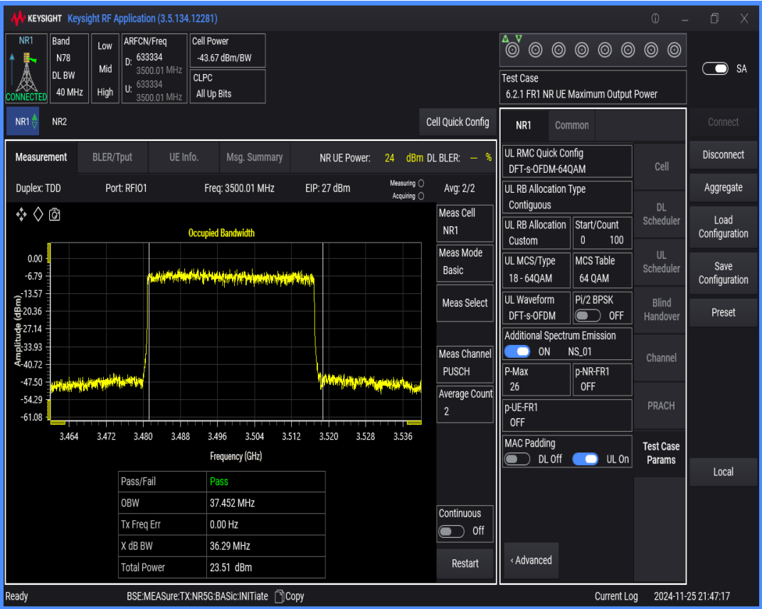
n78(3450-3550) SCS=30kHz DFT_QAM64 BW=20MHz Channel=633334 RB=50@0
