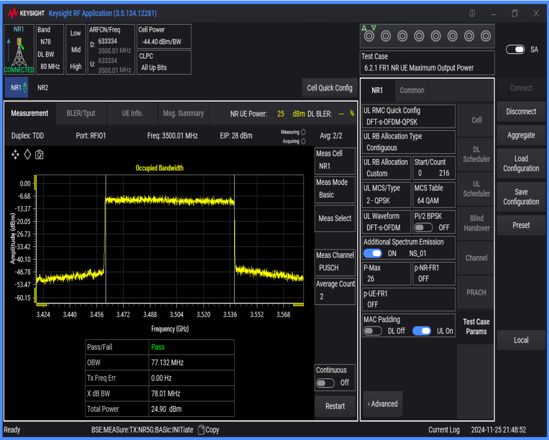
n78(3450-3550) SCS=30kHz DFT_QPSK BW=70MHz Channel=633334 RB=180@0
