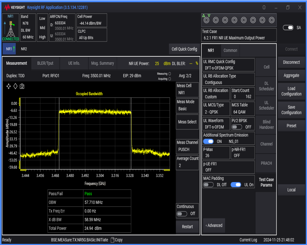
n78(3450-3550) SCS=30kHz DFT_QPSK BW=80MHz Channel=633334 RB=216@0
