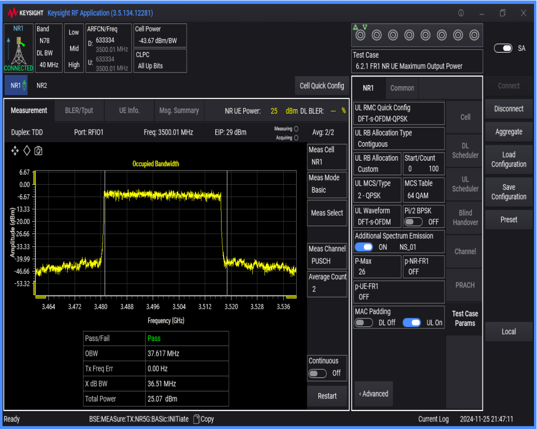
n78(3450-3550) SCS=30kHz DFT_QPSK BW=50MHz Channel=633334 RB=128@0
