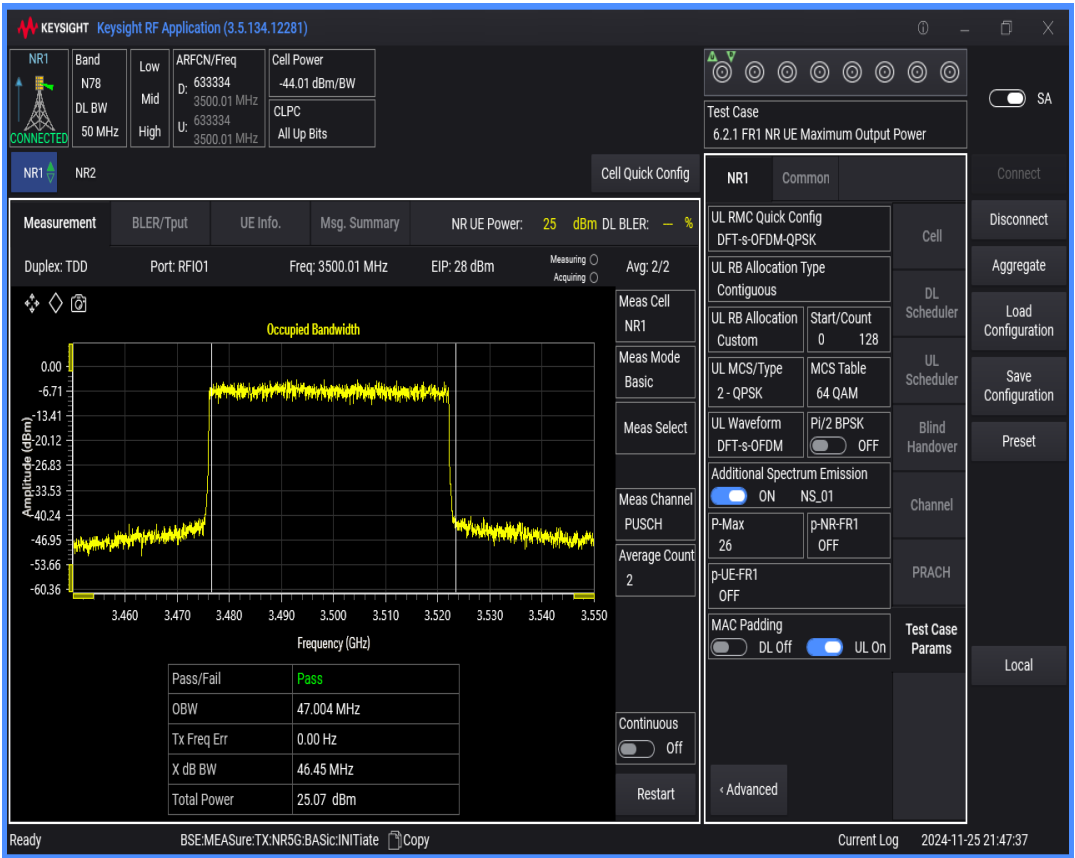
n78(3450-3550) SCS=30kHz DFT_QPSK BW=30MHz Channel=633334 RB=75@0
