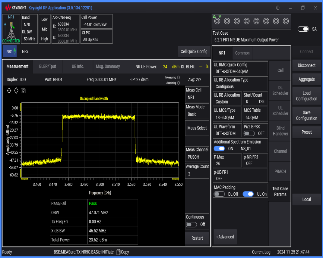
n78(3450-3550) SCS=30kHz DFT_QAM64 BW=80MHz Channel=633334 RB=216@0
