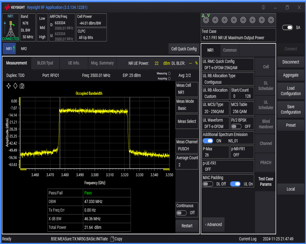
n78(3450-3550) SCS=30kHz DFT_QAM256 BW=70MHz Channel=633334 RB=180@0
