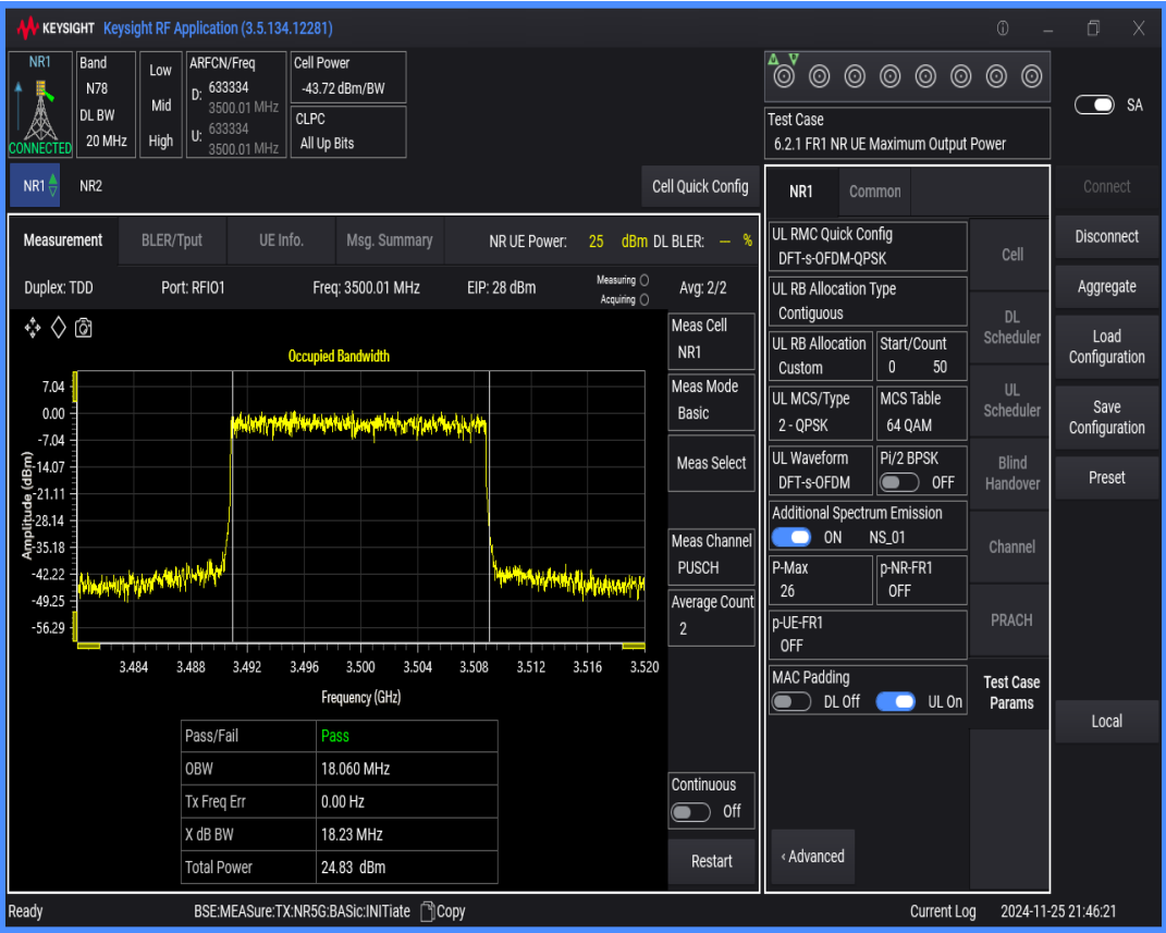
n78(3450-3550) SCS=30kHz DFT_QPSK BW=60MHz Channel=633334 RB=162@0
