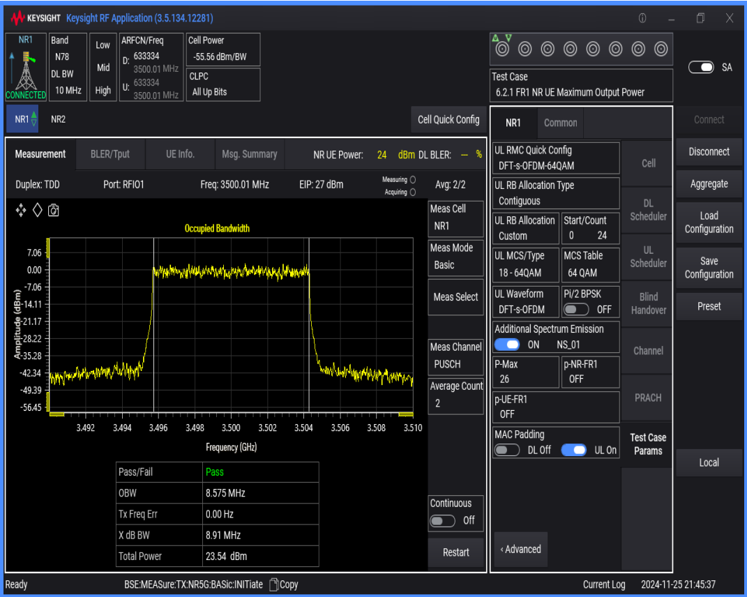
n78(3450-3550) SCS=30kHz DFT_QAM64 BW=15MHz Channel=633334 RB=36@0
