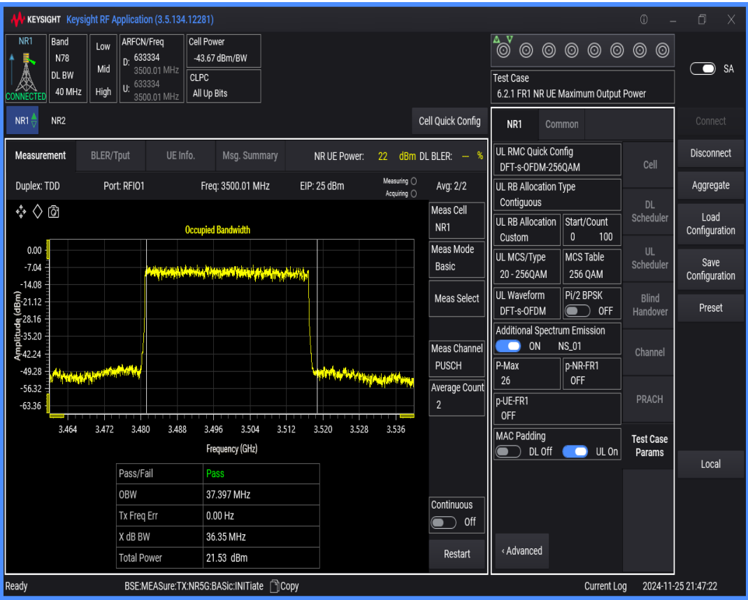
n78(3450-3550) SCS=30kHz DFT_QAM256 BW=30MHz Channel=633334 RB=75@0
