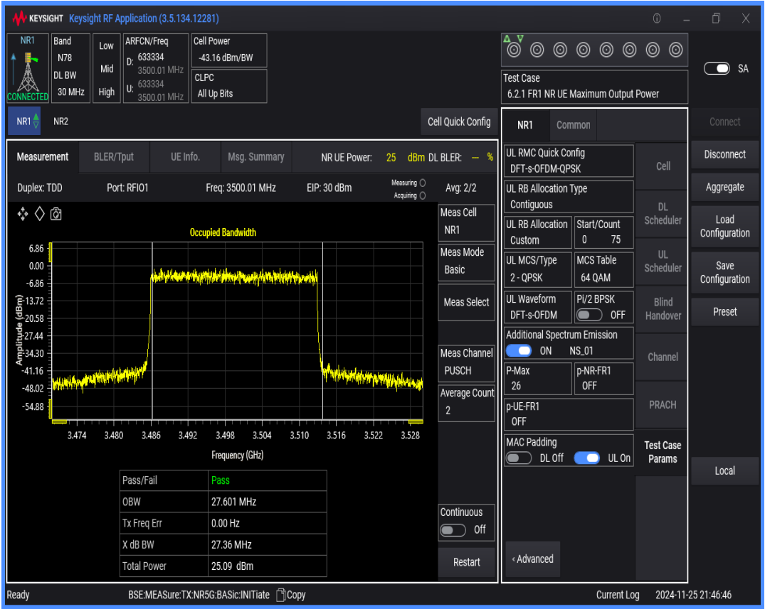
n78(3450-3550) SCS=30kHz DFT_QPSK BW=15MHz Channel=633334 RB=36@0
