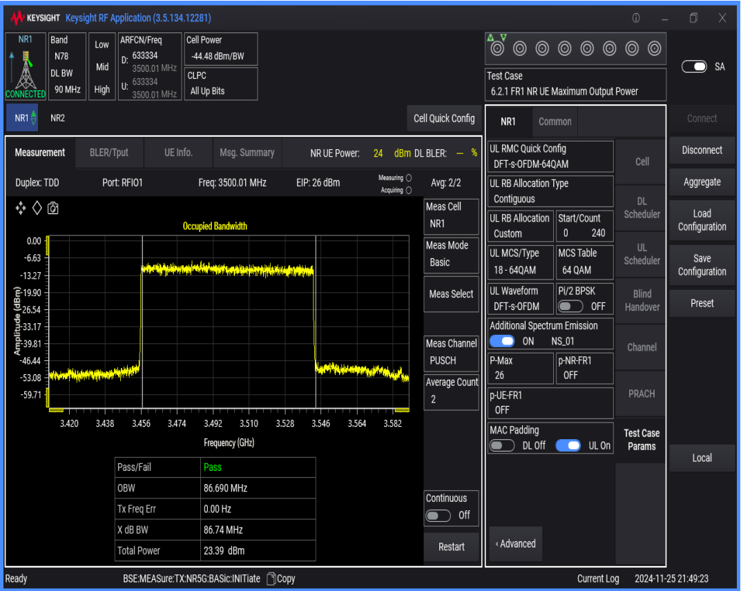
n78(3450-3550) SCS=30kHz DFT_QPSK BW=40MHz Channel=633334 RB=100@0
