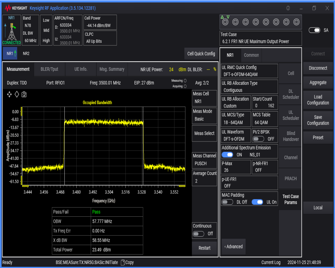
n78(3450-3550) SCS=30kHz DFT_QAM64 BW=50MHz Channel=633334 RB=128@0
