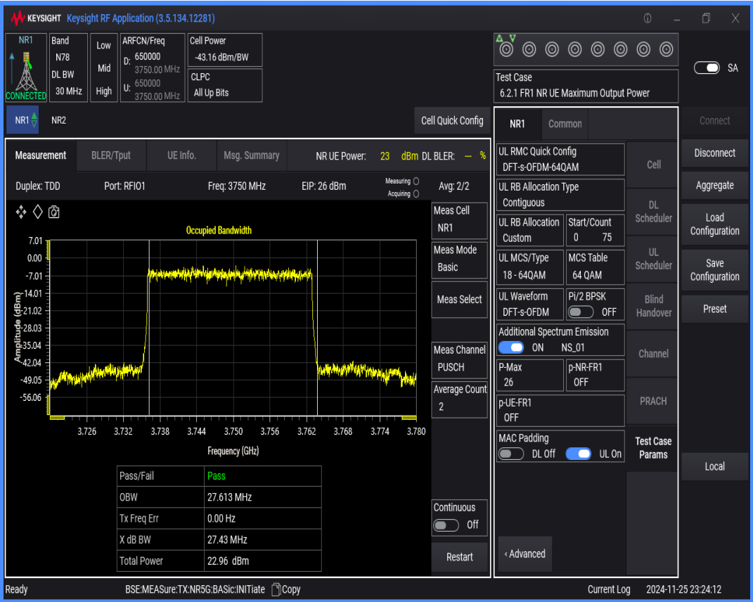
n78(3700-3800) SCS=30kHz DFT_QAM64 BW=15MHz Channel=650000 RB=36@0
