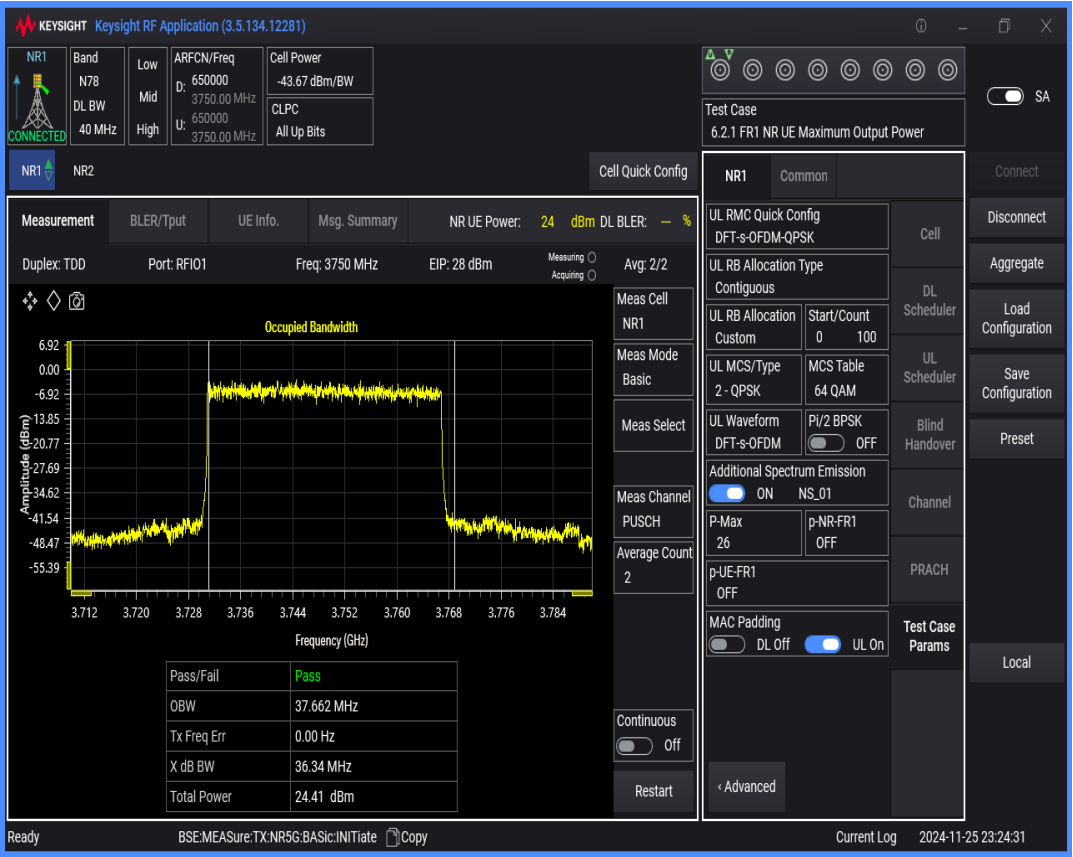
n78(3700-3800) SCS=30kHz DFT_QPSK BW=70MHz Channel=650000 RB=180@0
