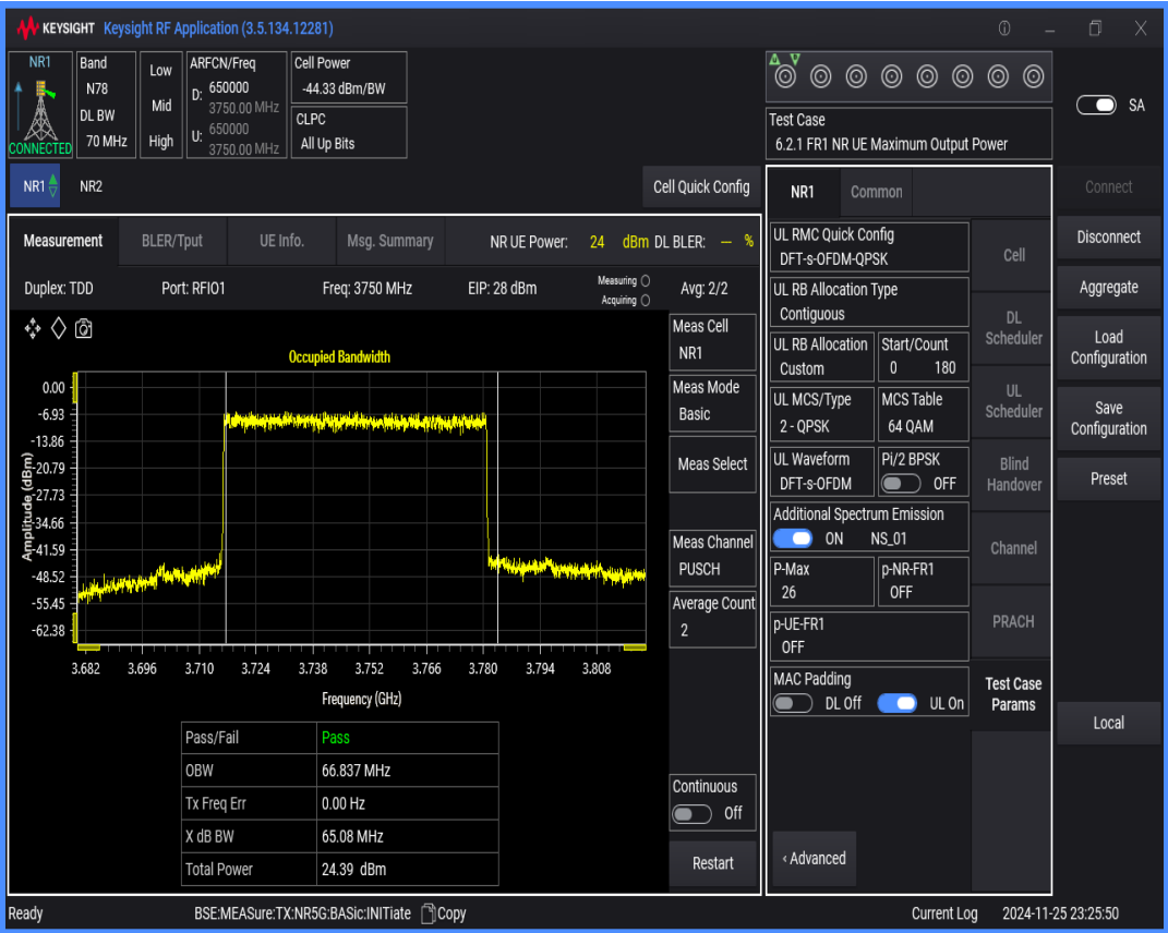
n78(3700-3800) SCS=30kHz DFT_QPSK BW=60MHz Channel=650000 RB=162@0
