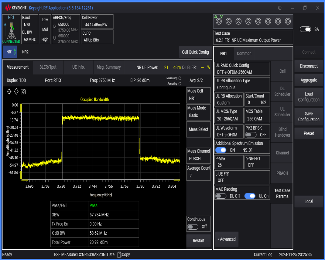
n78(3700-3800) SCS=30kHz DFT_QAM256 BW=70MHz Channel=650000 RB=180@0
