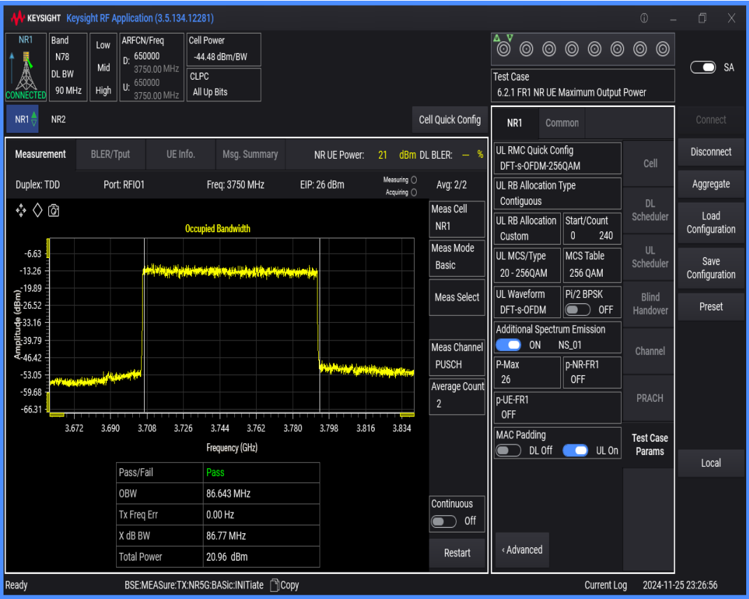
n78(3700-3800) SCS=30kHz DFT_QAM256 BW=80MHz Channel=650000 RB=216@0
