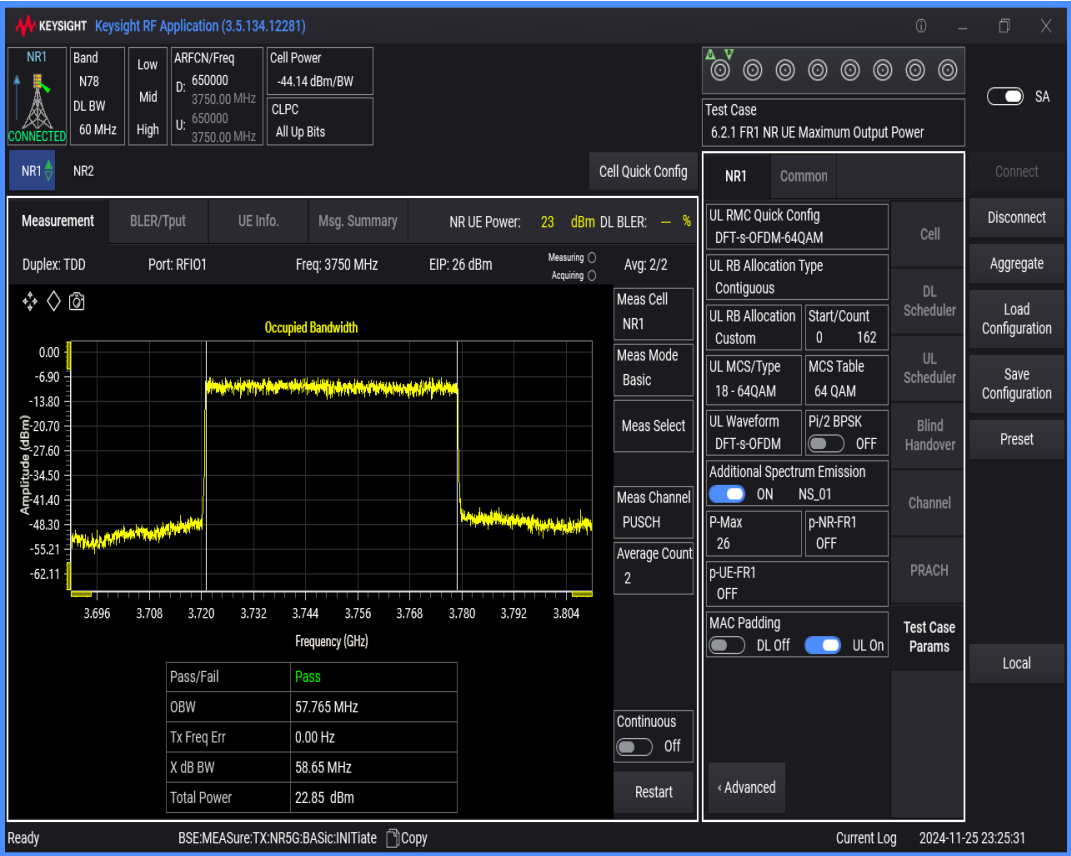
n78(3700-3800) SCS=30kHz DFT_QAM64 BW=90MHz Channel=650000 RB=240@0
