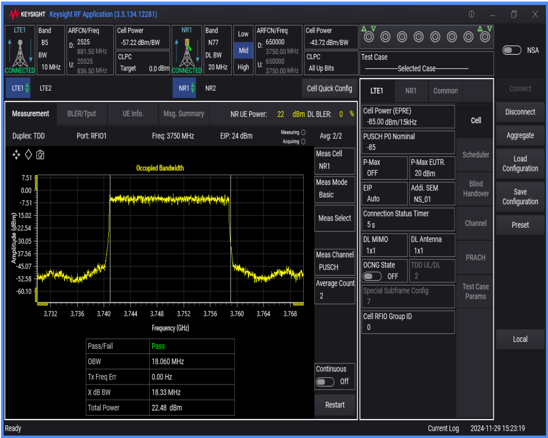
n77 SCS=30kHz DFT_BPSK BW=40MHz Channel=650000 RB=100@0
