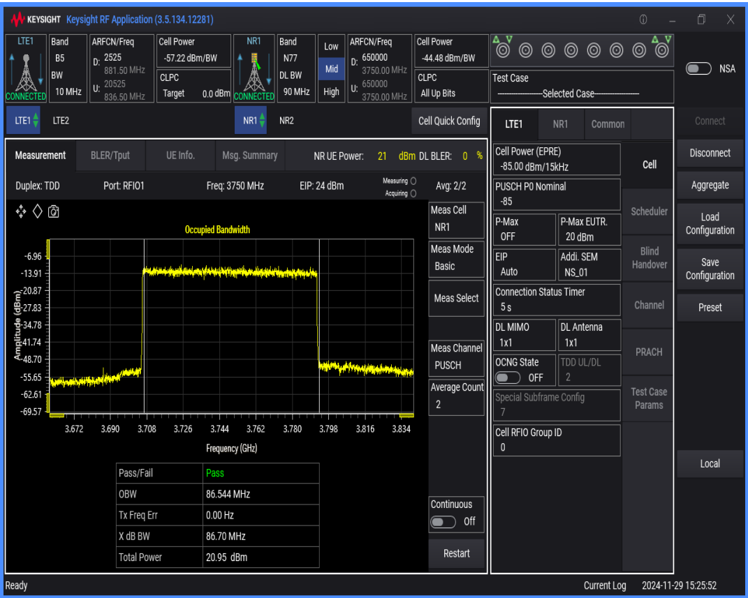
n77 SCS=30kHz DFT_QAM256 BW=40MHz Channel=650000 RB=100@0
