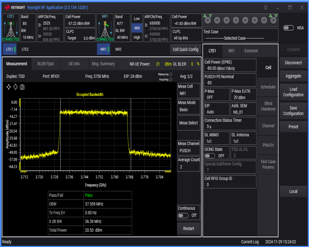
n77 SCS=30kHz DFT_QAM64 BW=20MHz Channel=650000 RB=50@0
