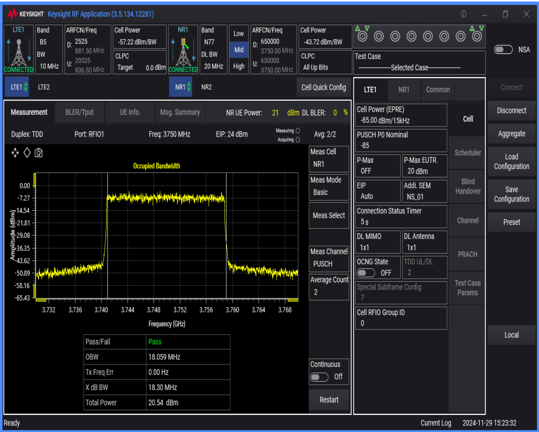
n77 SCS=30kHz DFT_QAM64 BW=100MHz Channel=650000 RB=270@0
