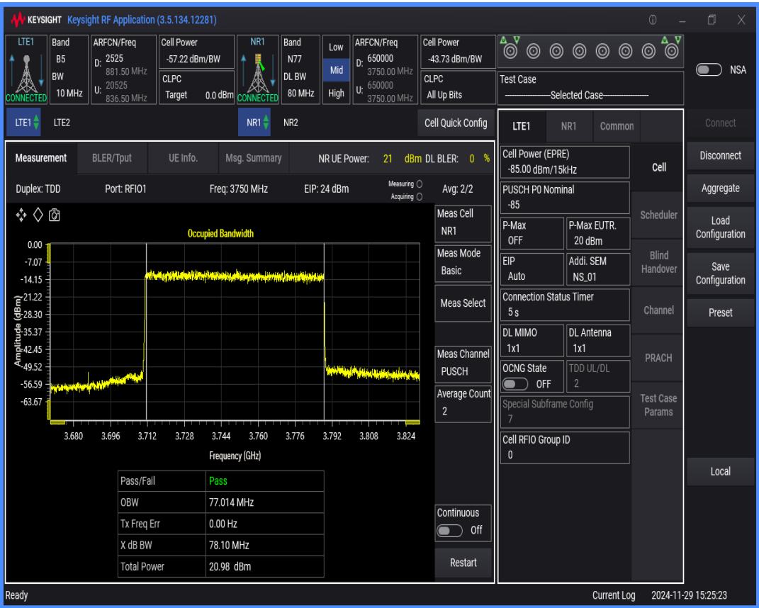
n77 SCS=30kHz DFT_QAM16 BW=90MHz Channel=650000 RB=240@0
