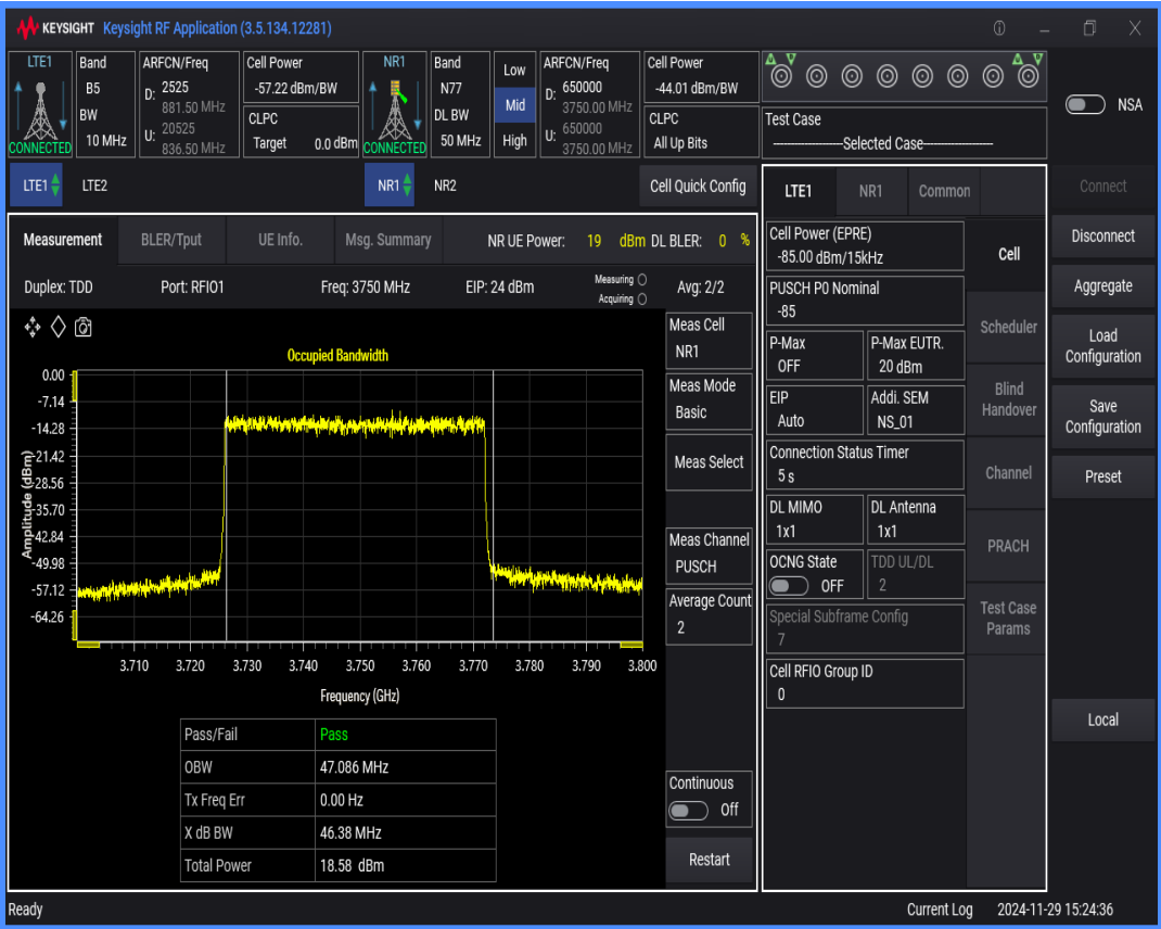
n77 SCS=30kHz DFT_QAM256 BW=90MHz Channel=650000 RB=240@0
