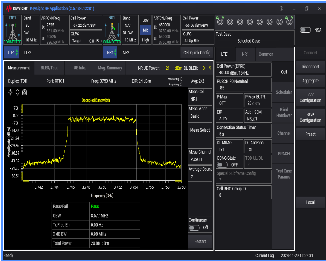
n77 SCS=30kHz DFT_QAM16 BW=100MHz Channel=650000 RB=270@0
