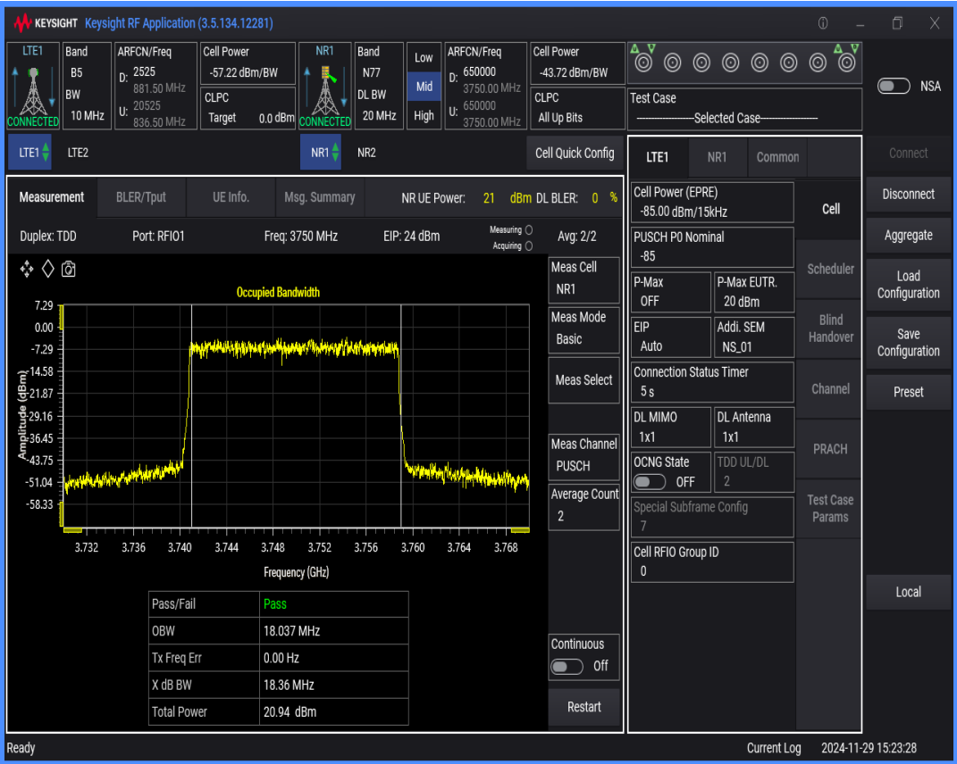
n77 SCS=30kHz DFT_QAM16 BW=15MHz Channel=650000 RB=36@0
