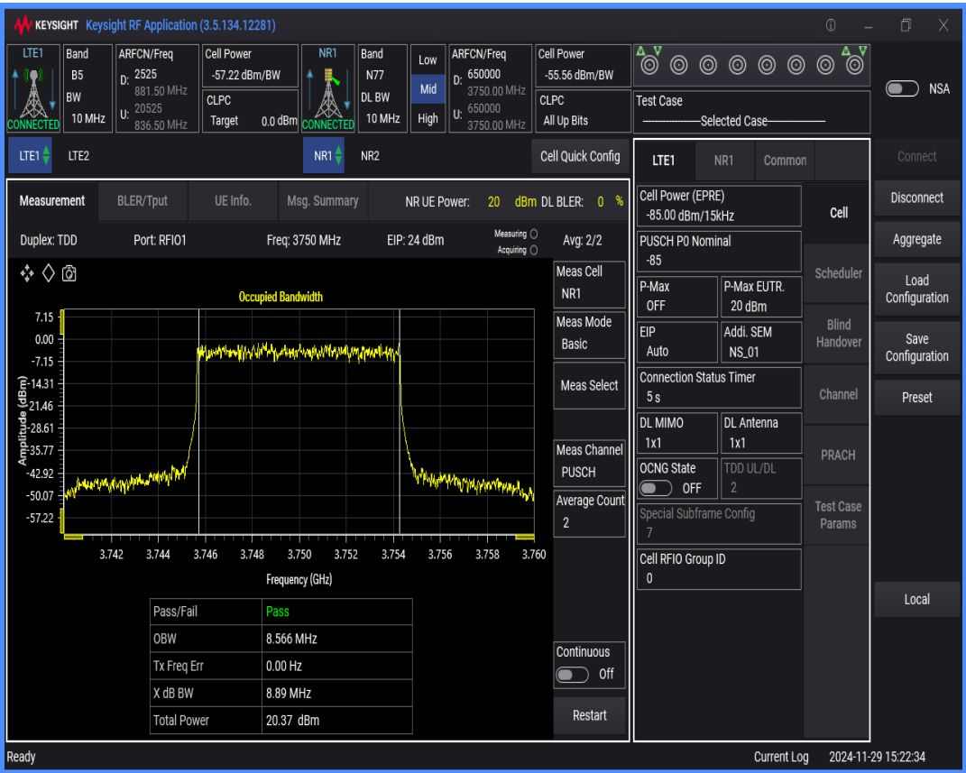
n77 SCS=30kHz DFT_QAM64 BW=100MHz Channel=650000 RB=270@0
