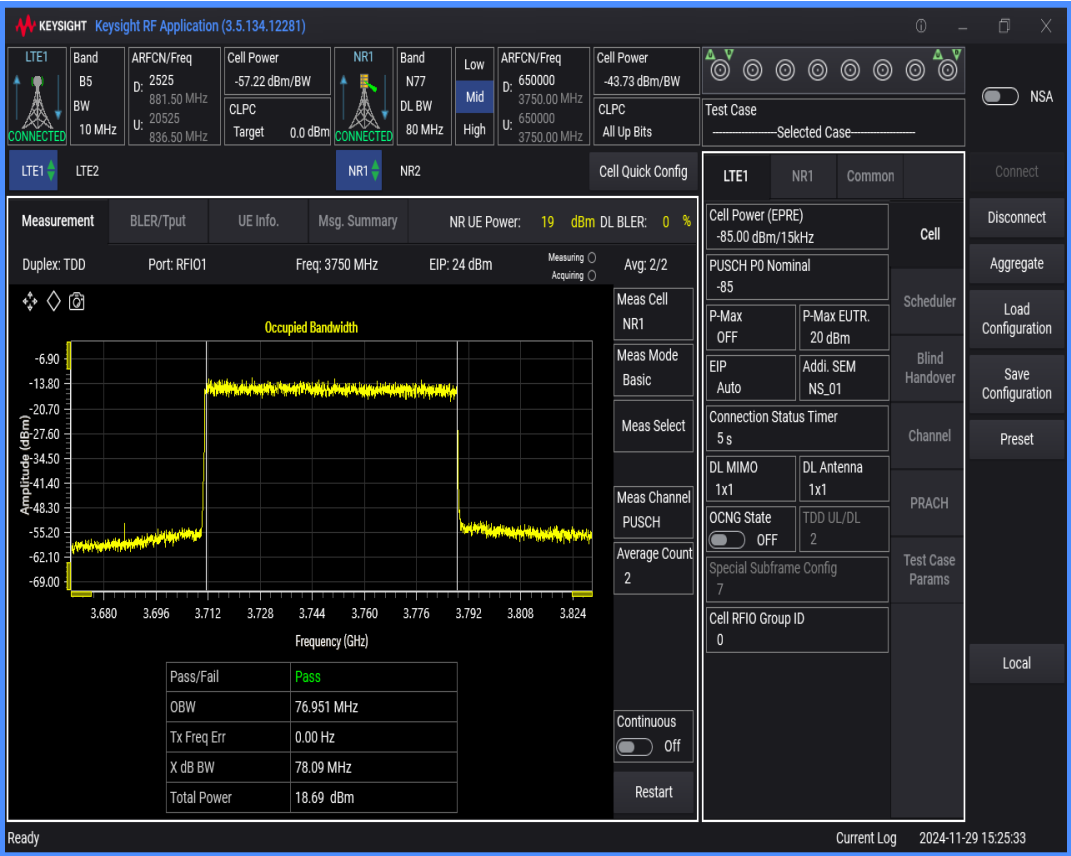
n77 SCS=30kHz DFT_QAM64 BW=10MHz Channel=650000 RB=24@0
