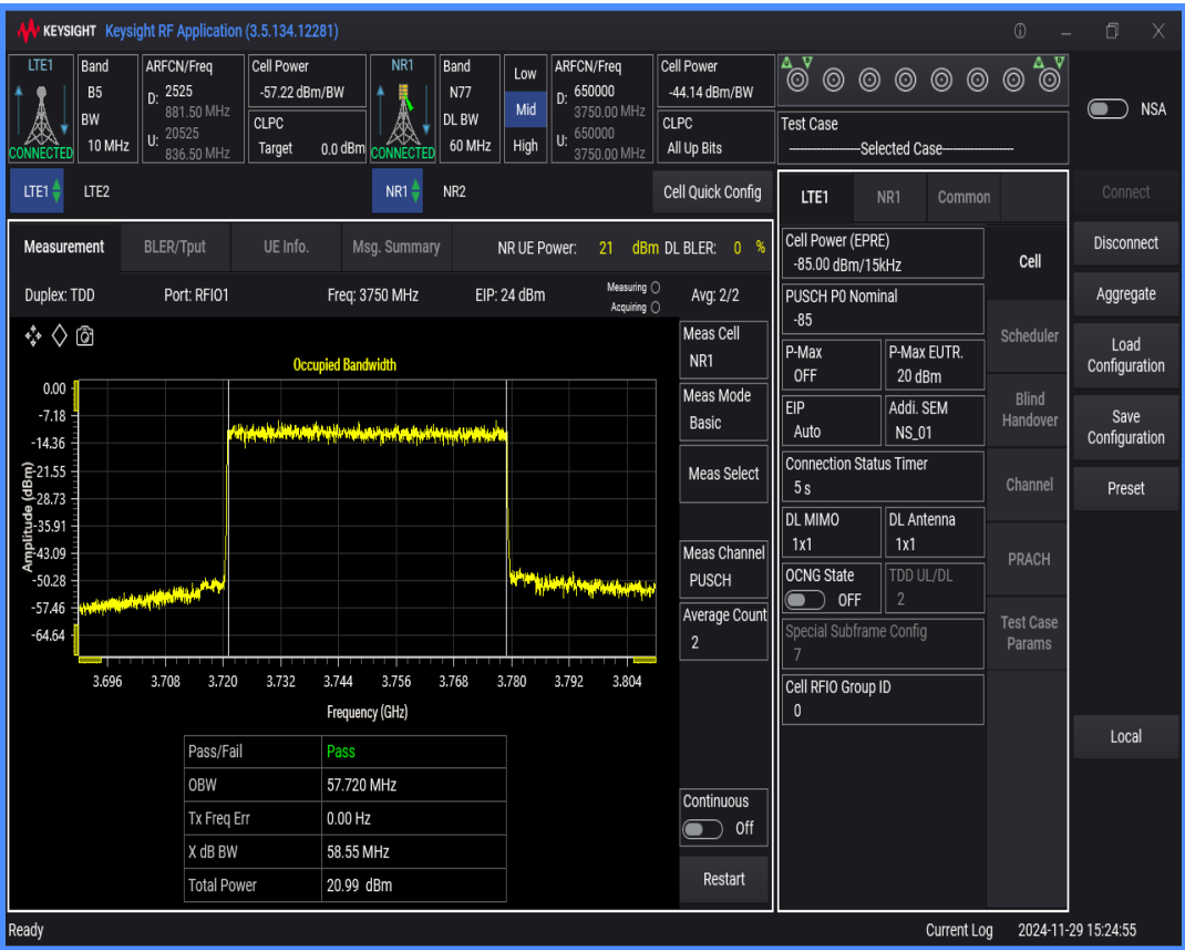
n77 SCS=30kHz DFT_QAM256 BW=90MHz Channel=650000 RB=240@0
