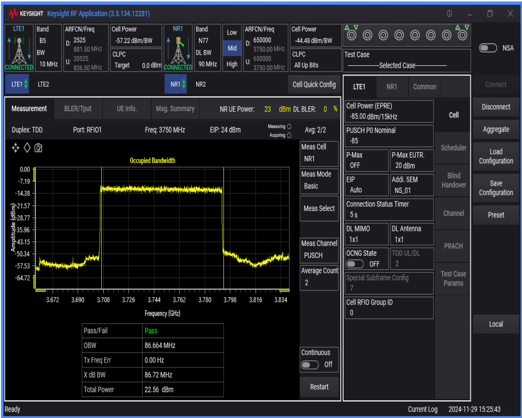
n77 SCS=30kHz DFT_QAM16 BW=100MHz Channel=650000 RB=270@0
