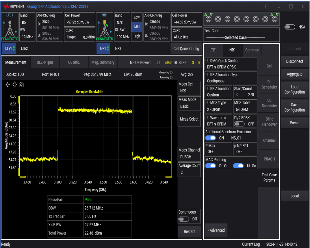
n78 SCS=30kHz DFT_QAM64 BW=90MHz Channel=636666 RB=240@0
