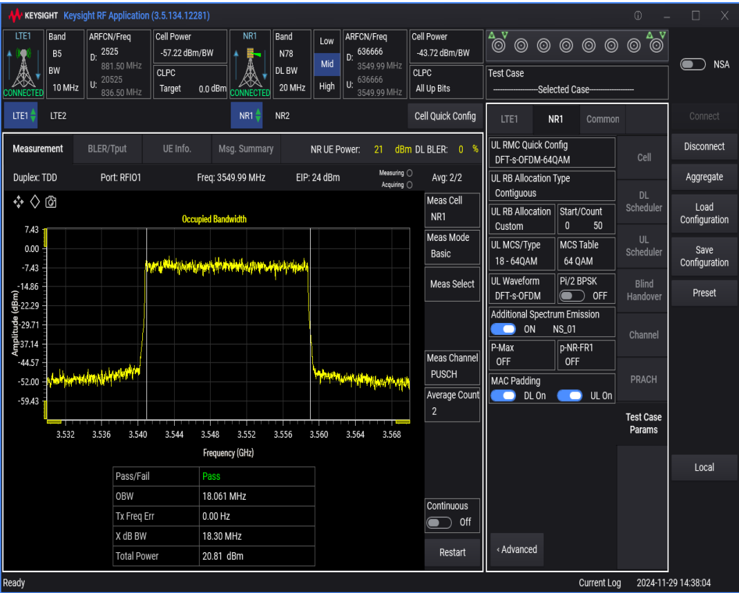
n78 SCS=30kHz DFT_QPSK BW=40MHz Channel=636666 RB=100@0
