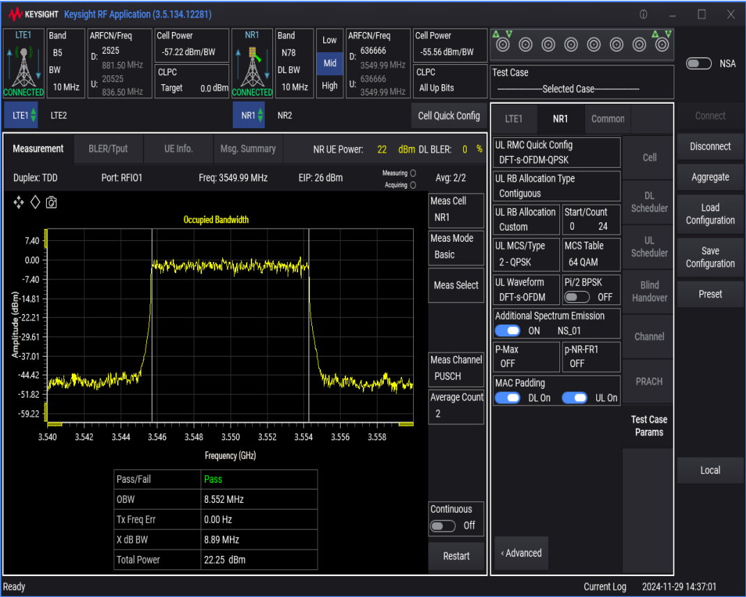
n78 SCS=30kHz DFT_QPSK BW=90MHz Channel=636666 RB=240@0
