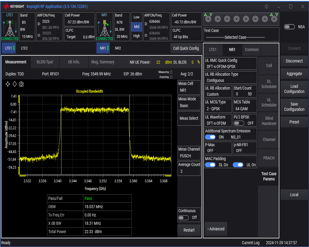
n78 SCS=30kHz DFT_QPSK BW=60MHz Channel=636666 RB=162@0
