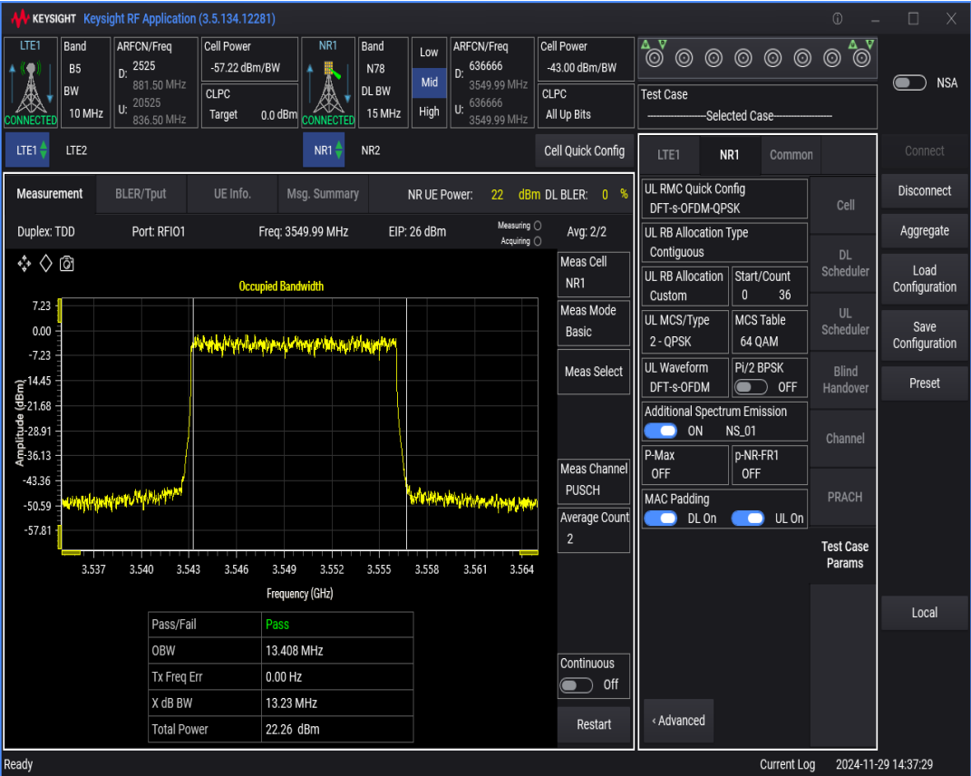
n78 SCS=30kHz DFT_QPSK BW=10MHz Channel=636666 RB=24@0
