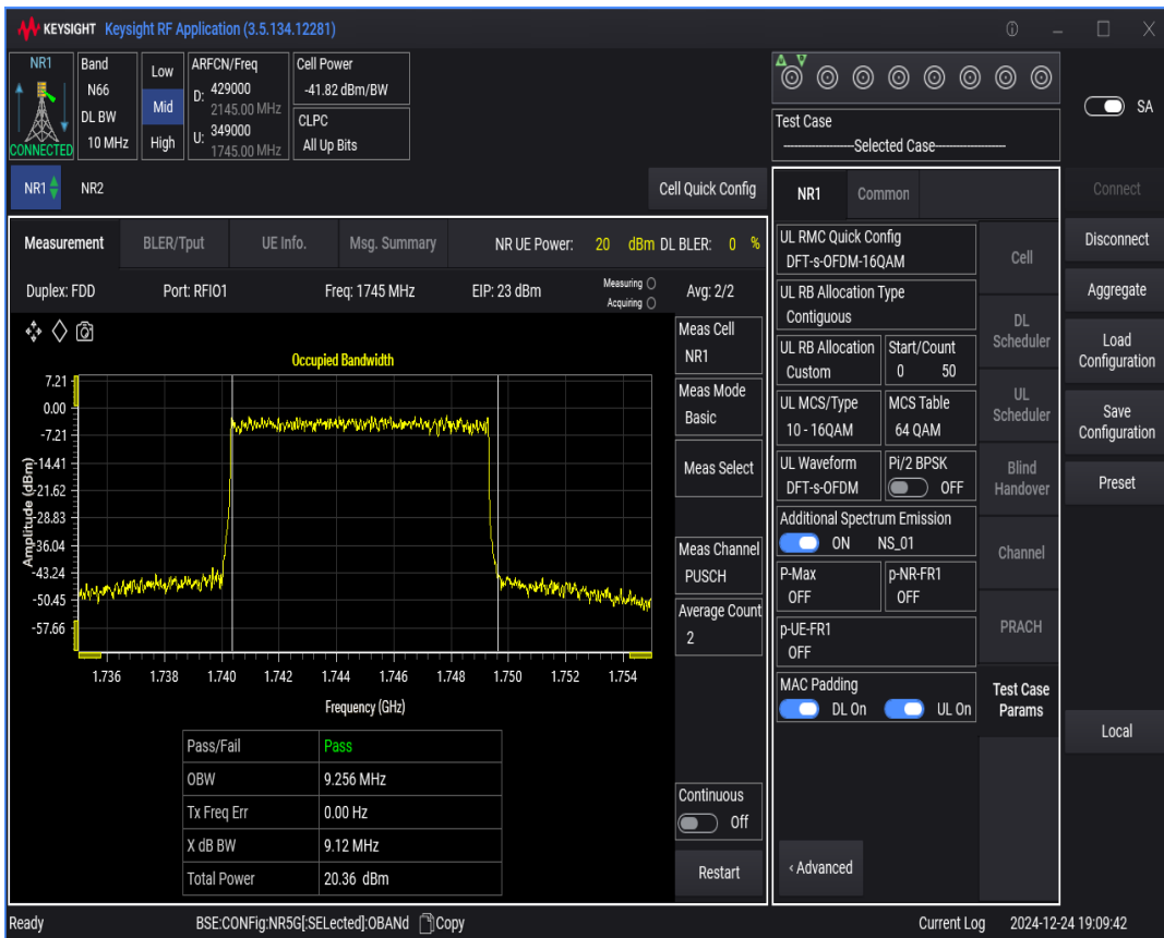
n66 SCS=15kHz DFT_QAM16 BW=15MHz Channel=349000 RB=75@0
