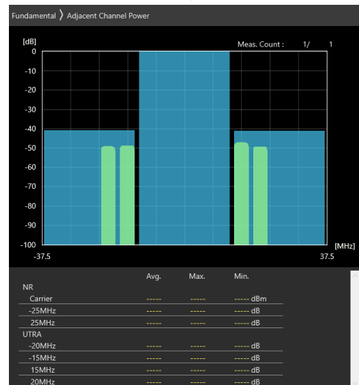
25MHz_15kHz_3687.5MHz_DFT-s-OFDM 16 QAM_RB1@132 -40.87 dB,-41.17 dB
