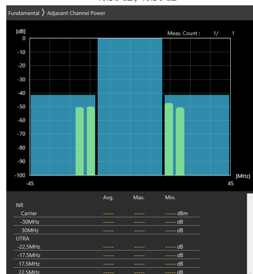
30MHz_15kHz_3685MHz_DFT-s-OFDM \pi/2 BPSK_RB1@159 -41.38 dB,-41.51 dB
