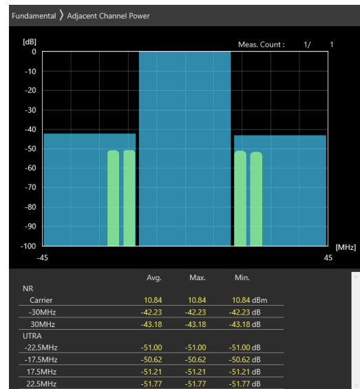
30MHz_15kHz_3565MHz_DFT-s-OFDM QPSK_RB80@40 -42.3 dB,-43.15 dB
