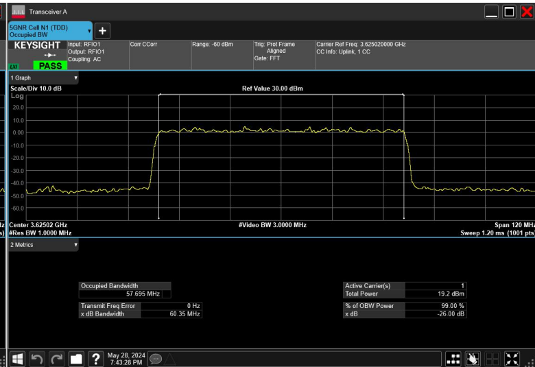
60MHz_30kHz_3625MHz_DFT-s-OFDM16QAM_RB162@0
