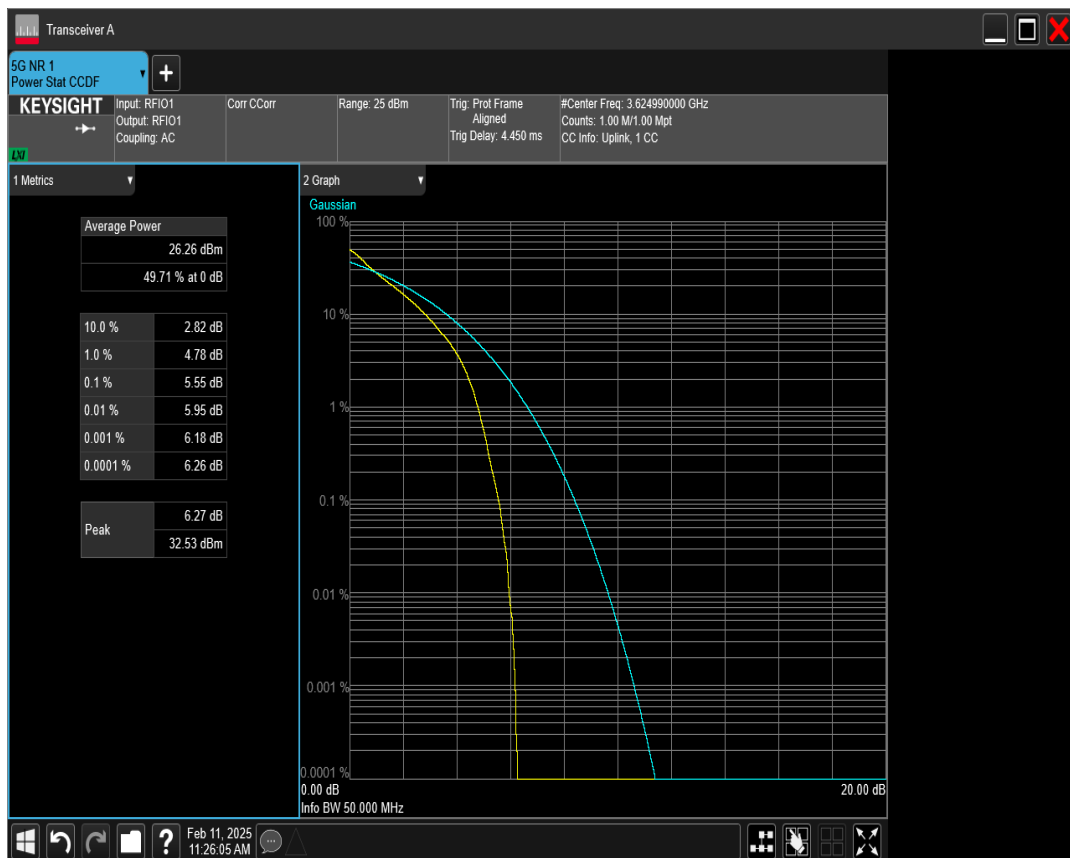
n77(3550-3700) SCS=30kHz DFT_QAM16 BW=50MHz Channel=641666 RB=128@0
