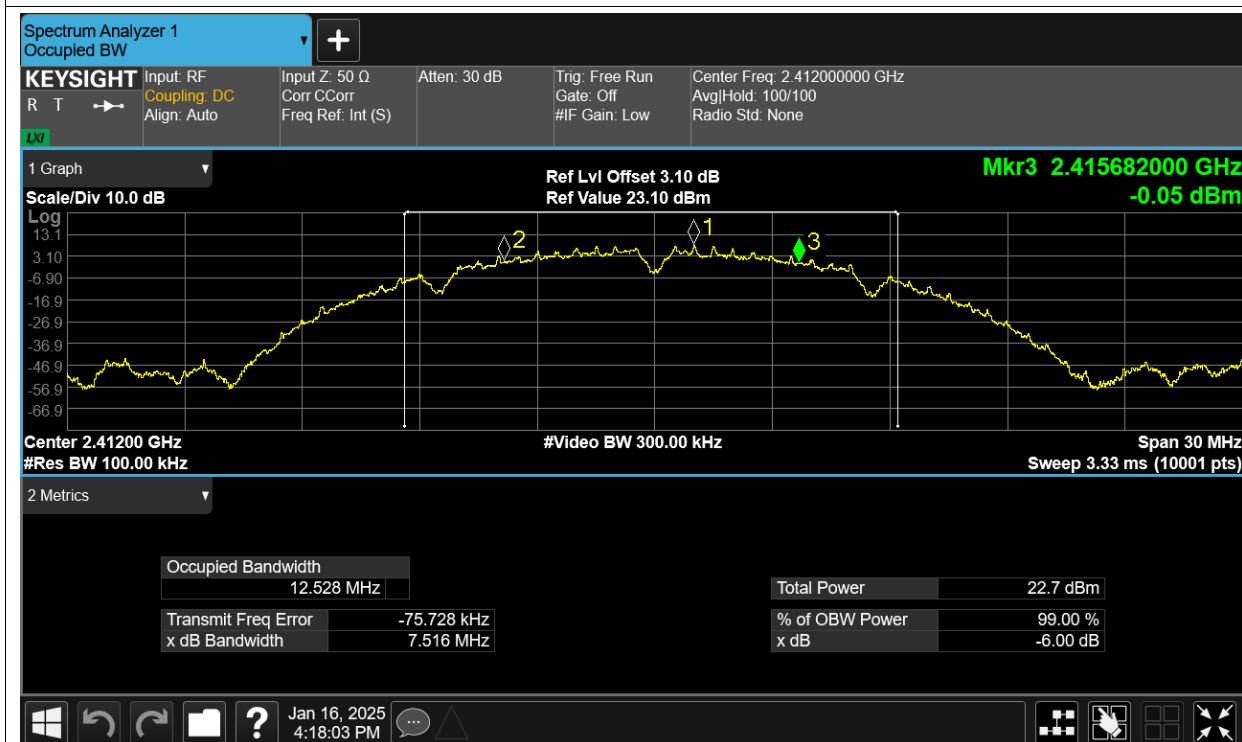
-6dB Bandwidth NVNT b 2437MHz Ant13
