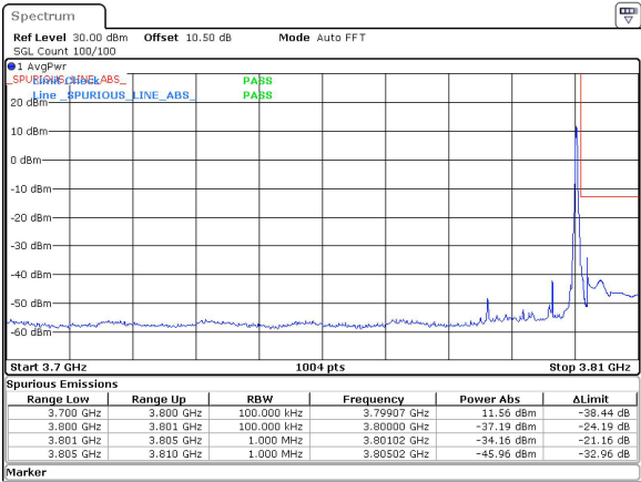
10MHz_30kHz_3795MHz_DFT-s-OFDM QPSK_RB1@23&-34.16 dBm
