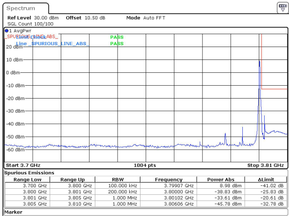
15MHz_30kHz_3792.5MHz_DFT-s-OFDM QPSK_RB1@37&-33.61 dBm
