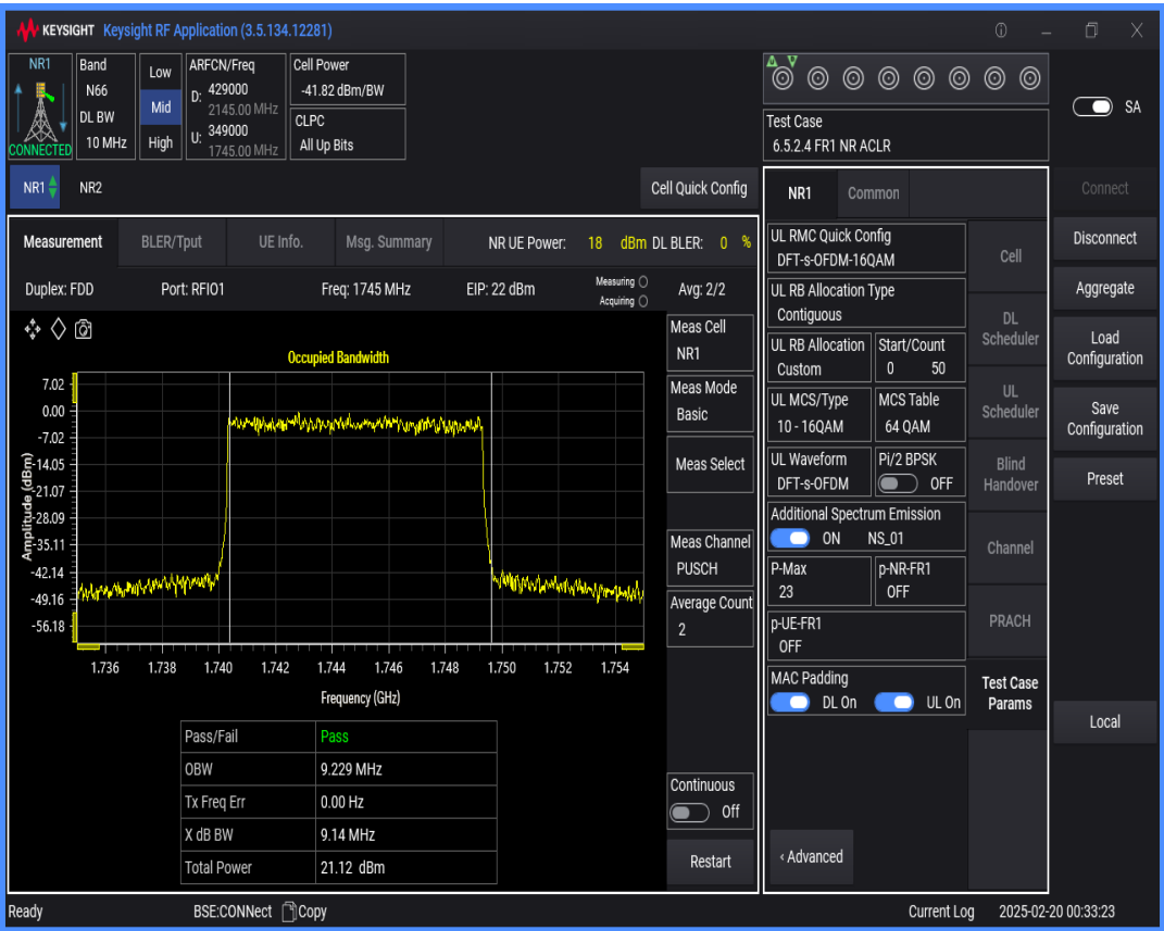
n66 SCS=15kHz DFT_QAM16 BW=15MHz Channel=349000 RB=75@0
