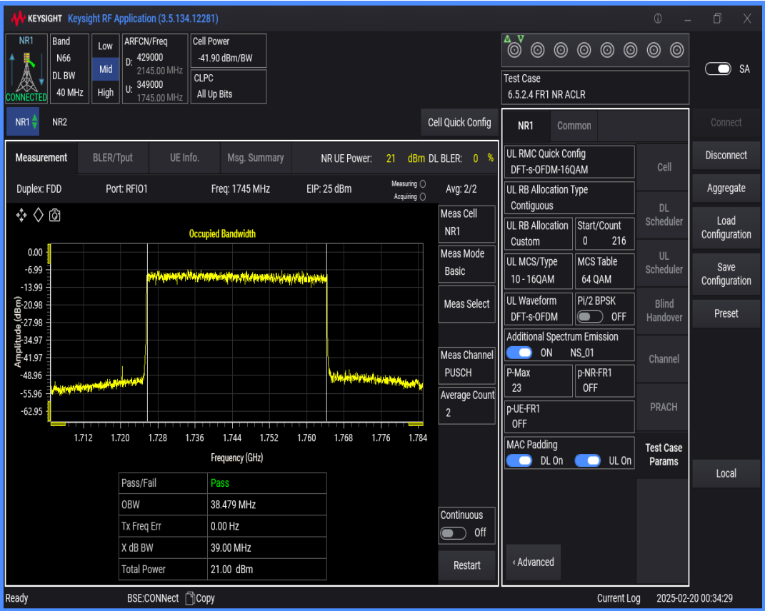
n66 SCS=15kHz DFT_QAM16 BW=5MHz Channel=349000 RB=25@0
