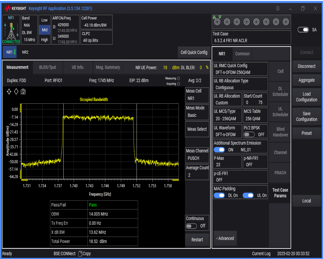
n66 SCS=15kHz DFT_QAM256 BW=40MHz Channel=349000 RB=216@0
