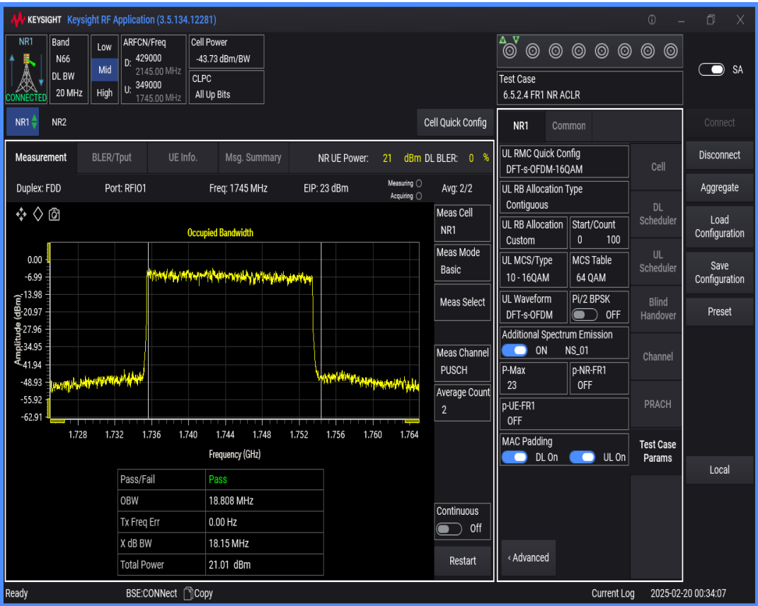
n66 SCS=15kHz DFT_QAM16 BW=40MHz Channel=349000 RB=216@0
