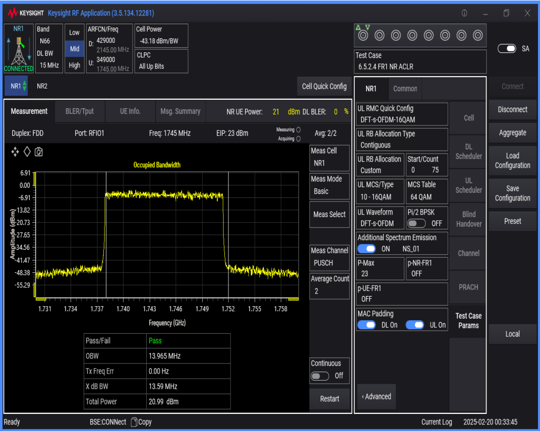
n66 SCS=15kHz DFT_QAM16 BW=20MHz Channel=349000 RB=100@0
