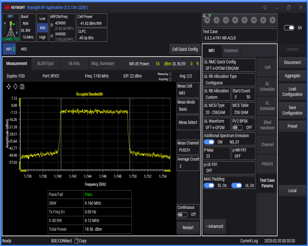
n66 SCS=15kHz DFT_QAM256 BW=15MHz Channel=349000 RB=75@0
