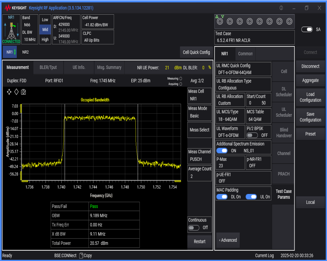
n66 SCS=15kHz DFT_QAM256 BW=5MHz Channel=349000 RB=25@0
