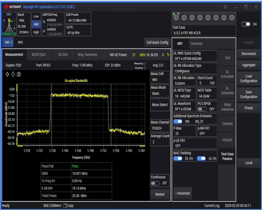
n66 SCS=15kHz DFT_QAM64 BW=15MHz Channel=349000 RB=75@0
