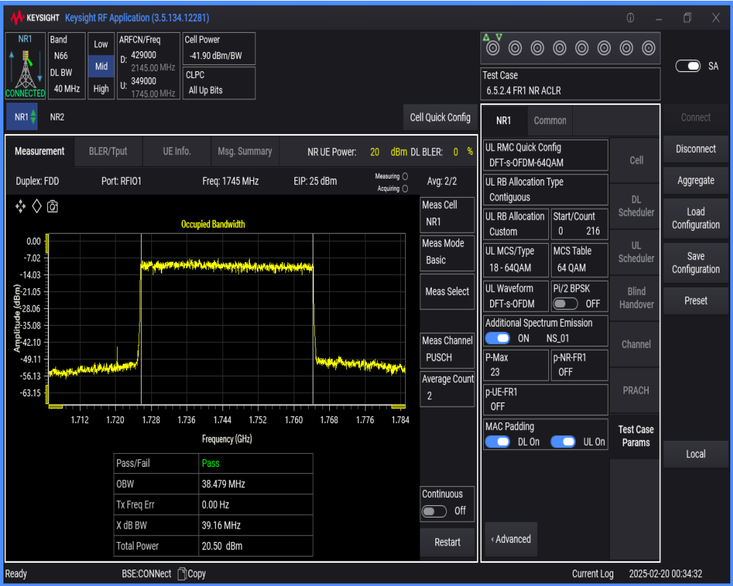
n66 SCS=15kHz DFT_QAM64 BW=20MHz Channel=349000 RB=100@0
