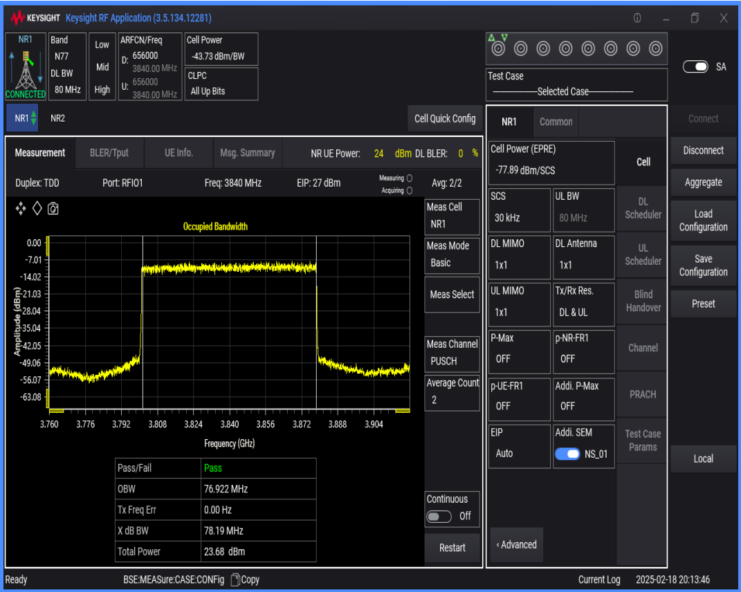
n77(3700-3980) SCS=30kHz DFT_BPSK BW=60MHz Channel=656000 RB=162@0
