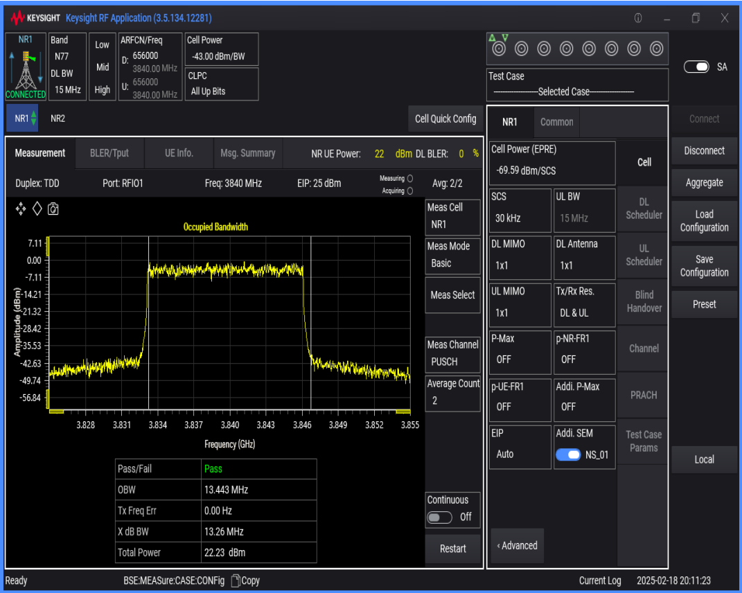
n77(3700-3980) SCS=30kHz DFT_QAM16 BW=10MHz Channel=656000 RB=24@0
