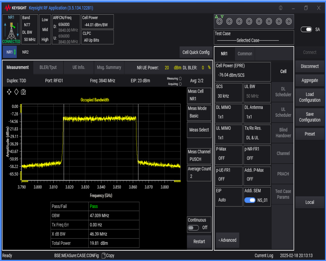
n77(3700-3980) SCS=30kHz DFT_QAM256 BW=60MHz Channel=656000 RB=162@0
