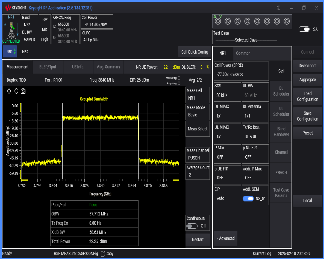
n77(3700-3980) SCS=30kHz DFT_QAM16 BW=50MHz Channel=656000 RB=128@0
