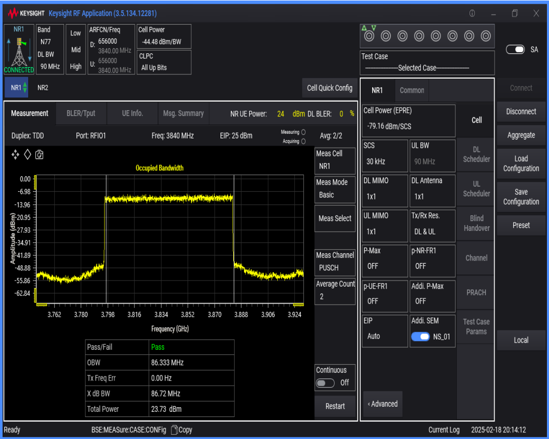
n77(3700-3980) SCS=30kHz DFT_QAM16 BW=100MHz Channel=656000 RB=270@0
