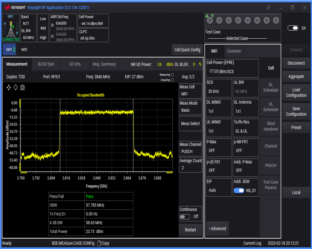
n77(3700-3980) SCS=30kHz DFT_BPSK BW=90MHz Channel=656000 RB=240@0
