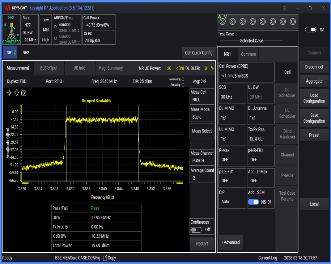
n77(3700-3980) SCS=30kHz DFT_QAM256 BW=30MHz Channel=656000 RB=75@0
