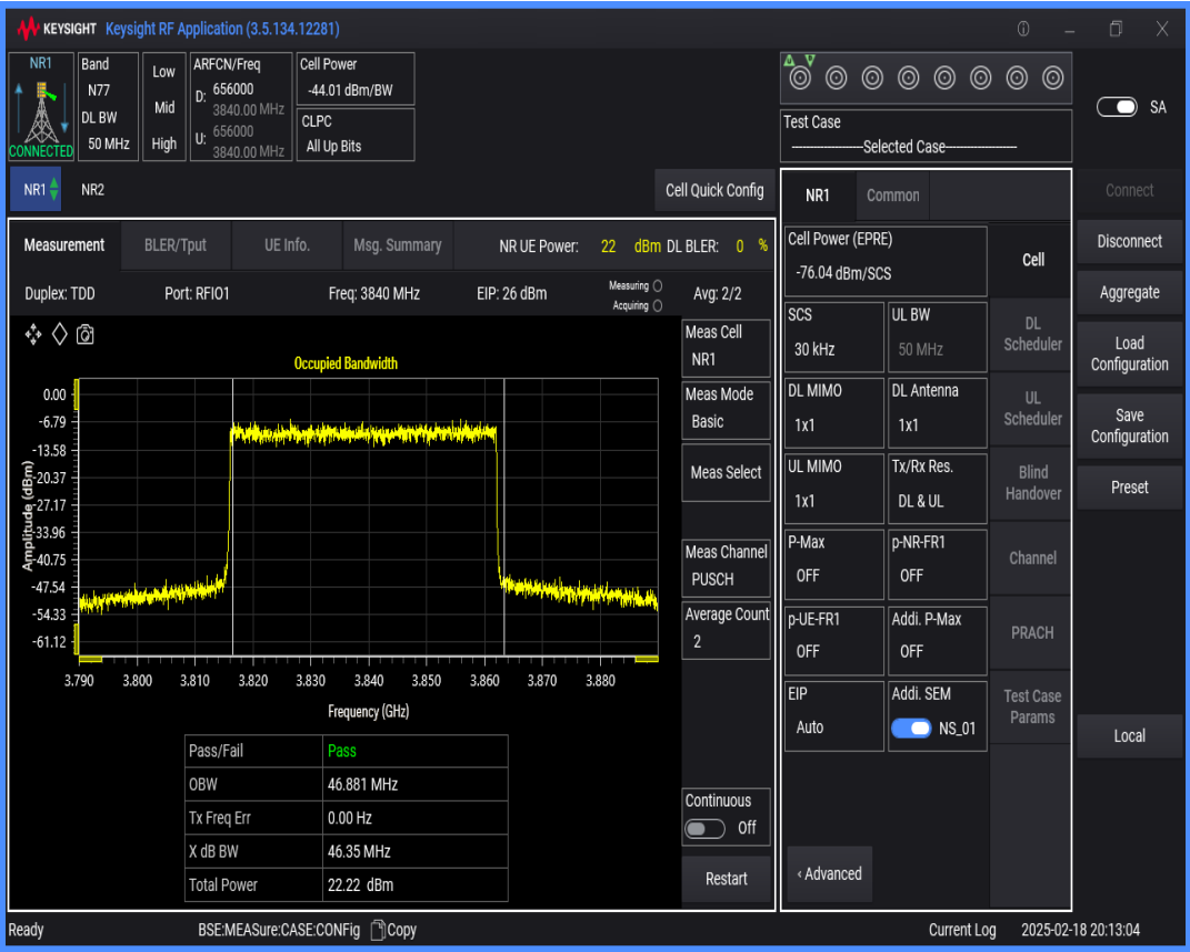
n77(3700-3980) SCS=30kHz DFT_QAM16 BW=40MHz Channel=656000 RB=100@0
