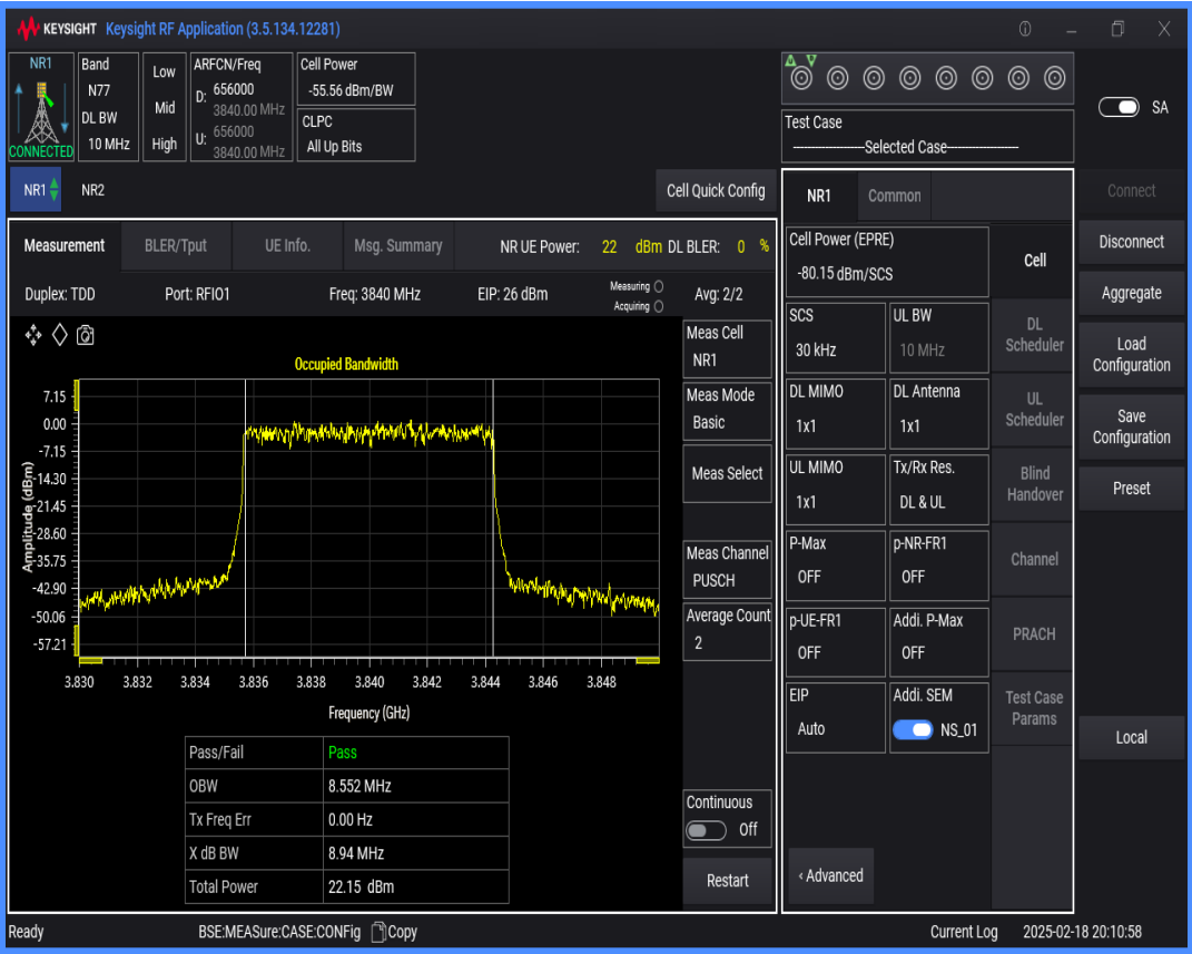
n77(3700-3980) SCS=30kHz DFT_QAM16 BW=30MHz Channel=656000 RB=75@0
