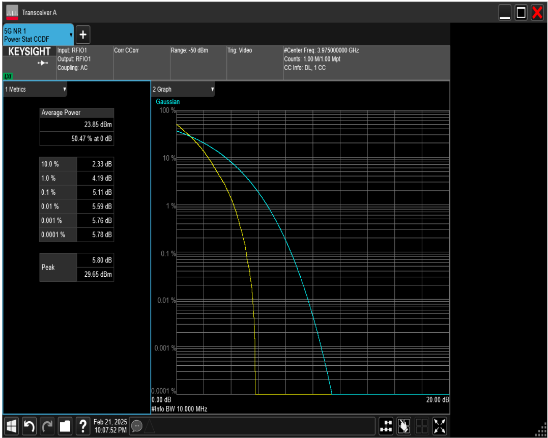
n77(3700-3980) SCS=30kHz DFT_QPSK BW=15MHz Channel=647168 RB=36@0
