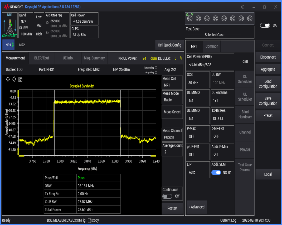
n77(3700-3980) SCS=30kHz DFT_BPSK BW=15MHz Channel=656000 RB=36@0
