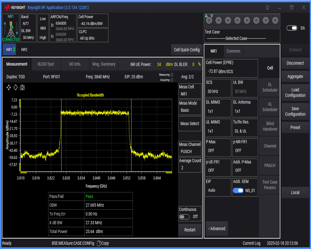
n77(3700-3980) SCS=30kHz DFT_BPSK BW=40MHz Channel=656000 RB=100@0
