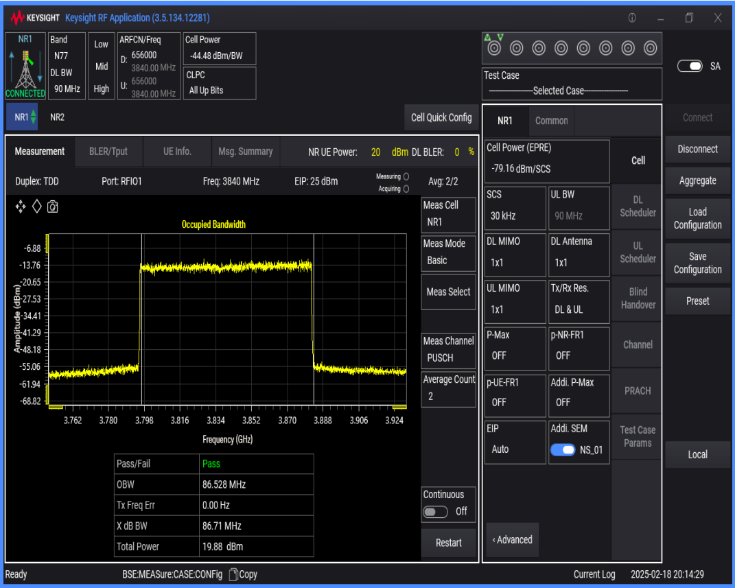
n77(3700-3980) SCS=30kHz DFT_QAM256 BW=80MHz Channel=656000 RB=216@0
