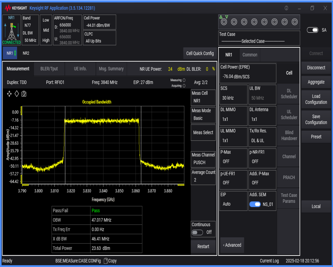
n77(3700-3980) SCS=30kHz DFT_BPSK BW=80MHz Channel=656000 RB=216@0
