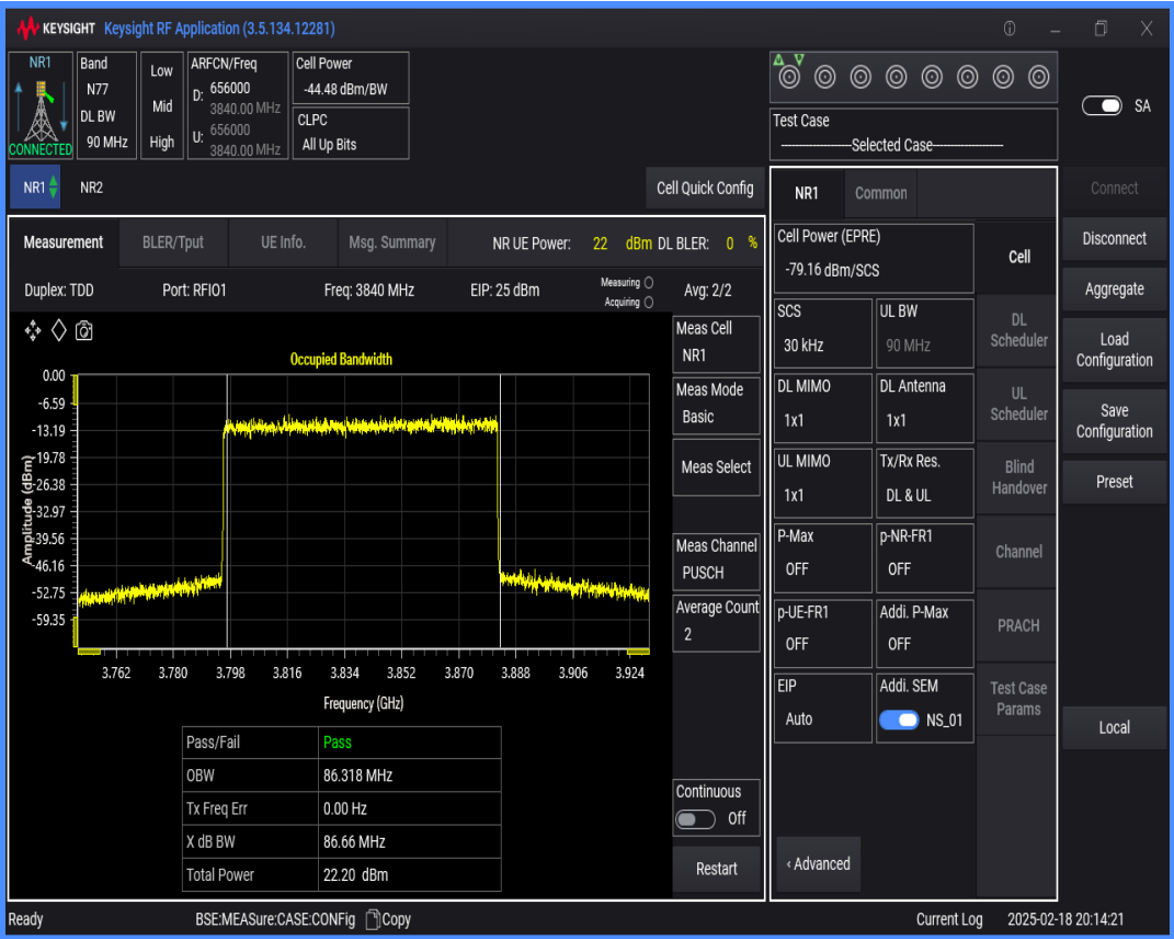
n77(3700-3980) SCS=30kHz DFT_QAM256 BW=15MHz Channel=656000 RB=36@0
