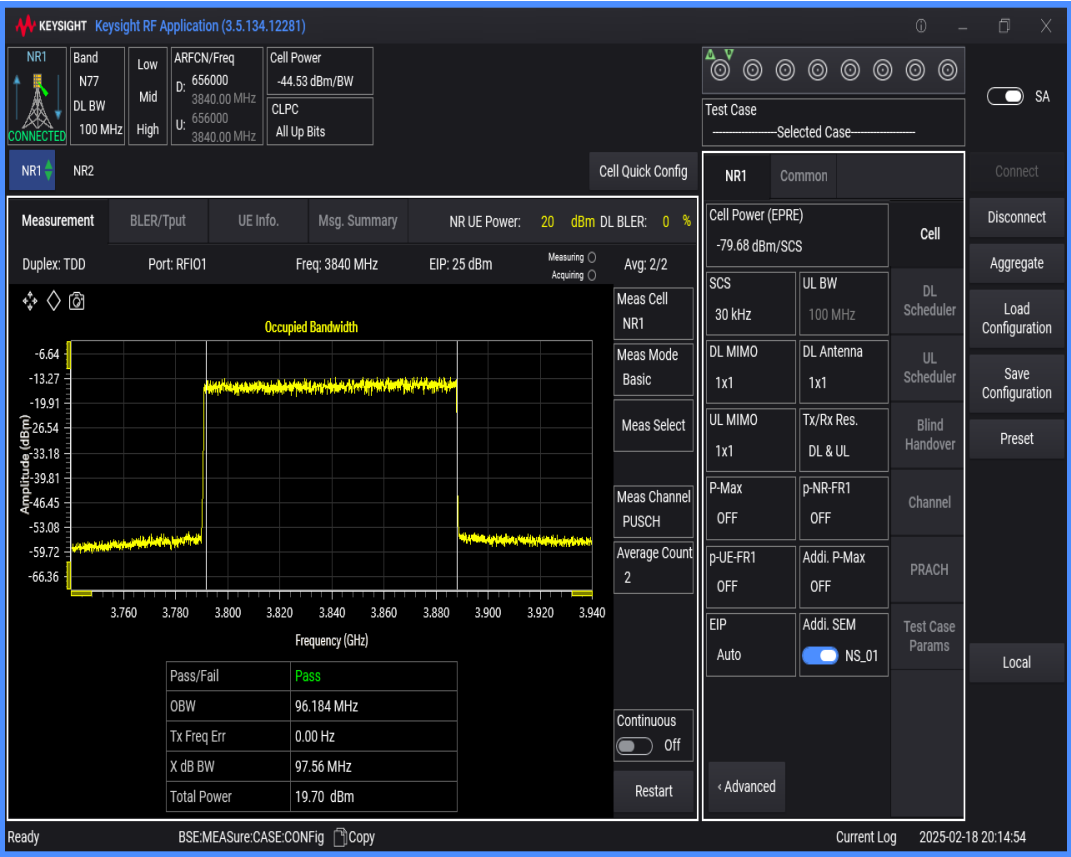
n77(3700-3980) SCS=30kHz DFT_QAM256 BW=50MHz Channel=656000 RB=128@0
