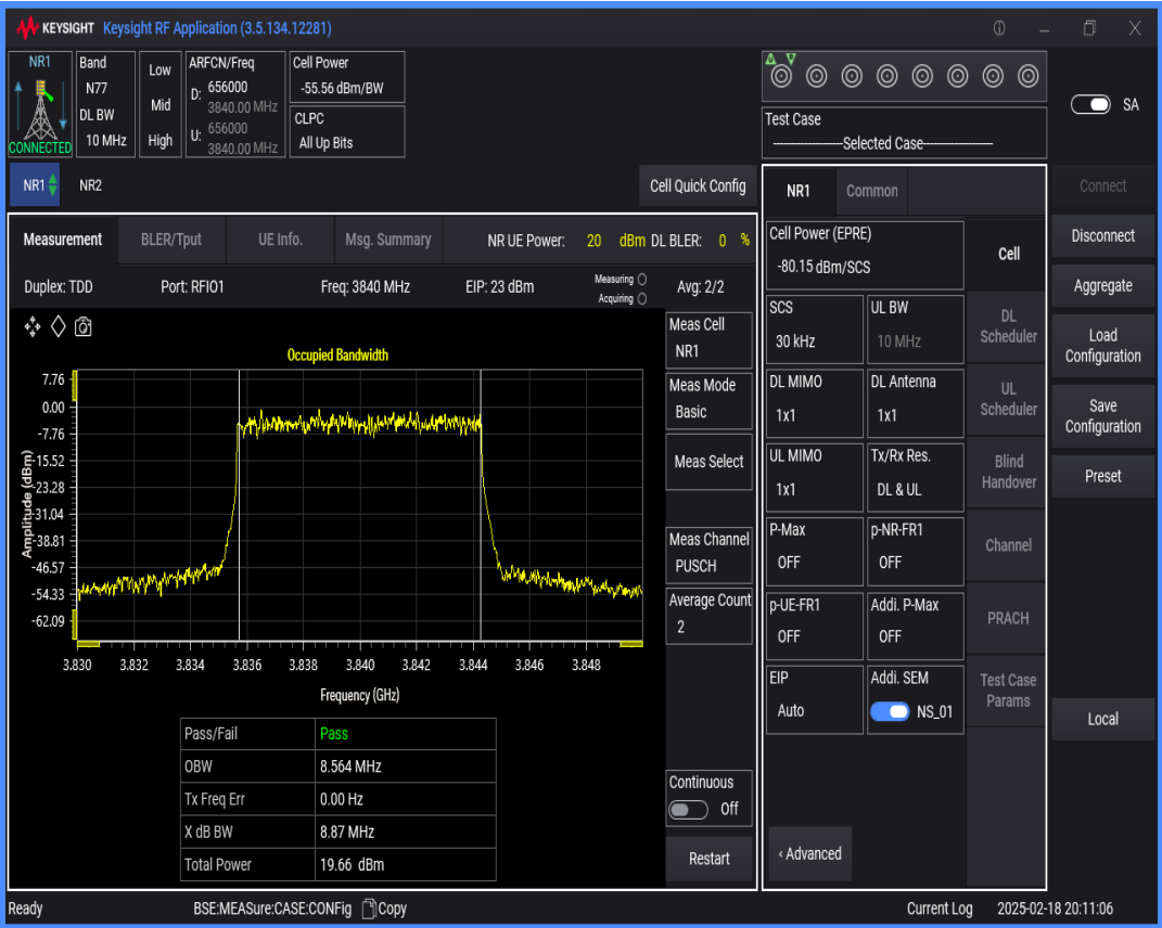
n77(3700-3980) SCS=30kHz DFT_QAM256 BW=100MHz Channel=656000 RB=270@0
