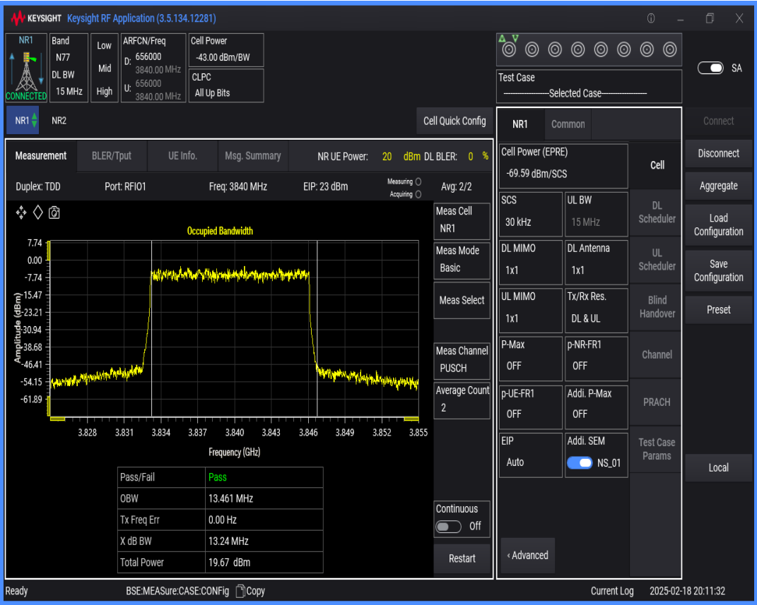
n77(3700-3980) SCS=30kHz DFT_QAM256 BW=10MHz Channel=656000 RB=24@0
