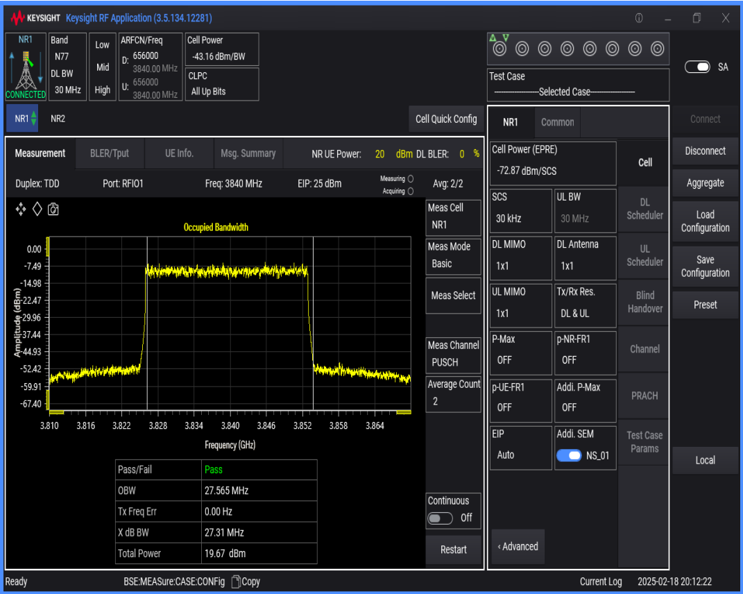
n77(3700-3980) SCS=30kHz DFT_QAM256 BW=90MHz Channel=656000 RB=240@0
