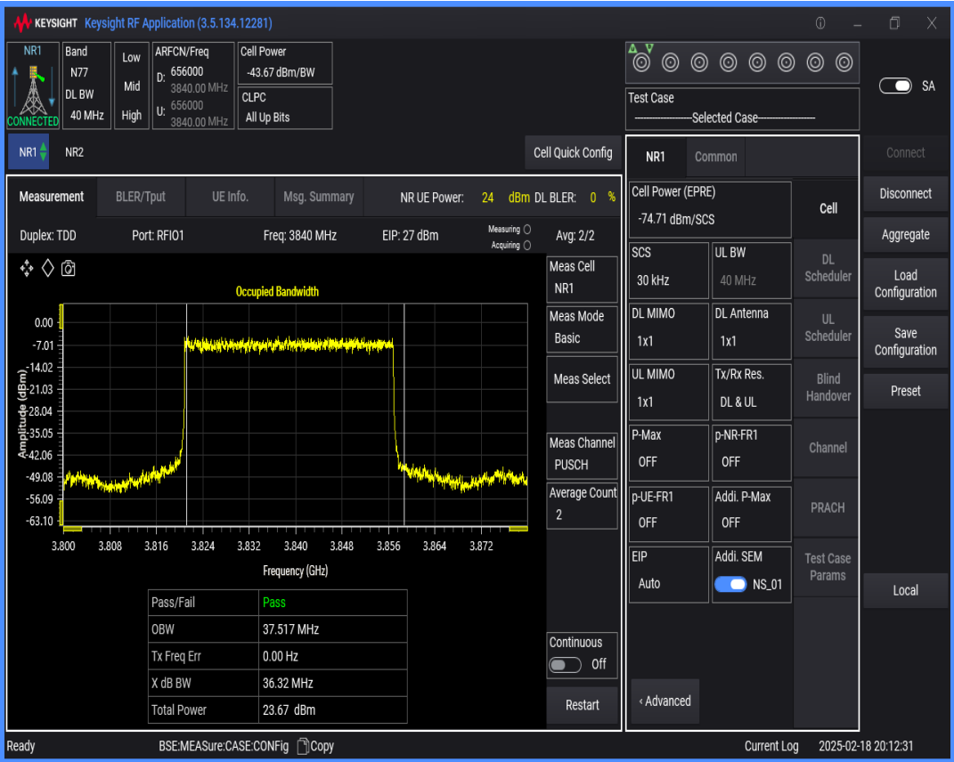
n77(3700-3980) SCS=30kHz DFT_BPSK BW=50MHz Channel=656000 RB=128@0
