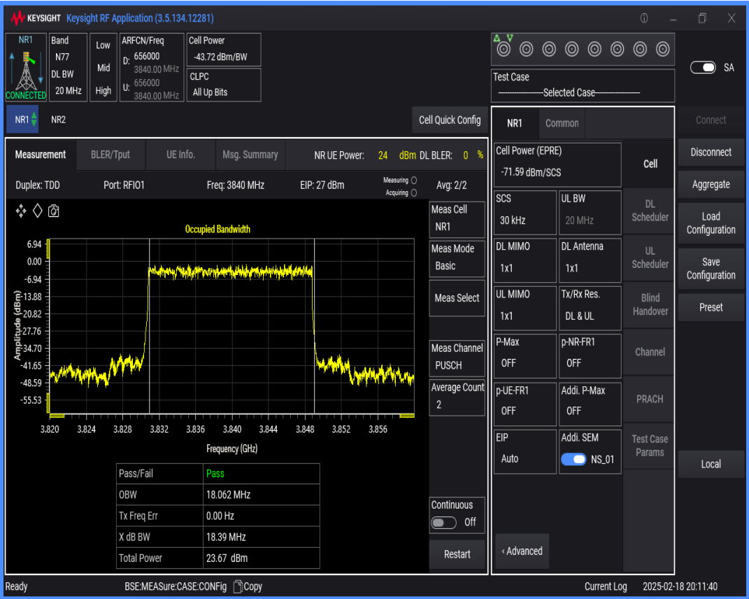
n77(3700-3980) SCS=30kHz DFT_BPSK BW=30MHz Channel=656000 RB=75@0
