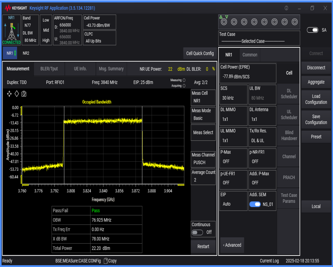
n77(3700-3980) SCS=30kHz DFT_QAM16 BW=90MHz Channel=656000 RB=240@0
