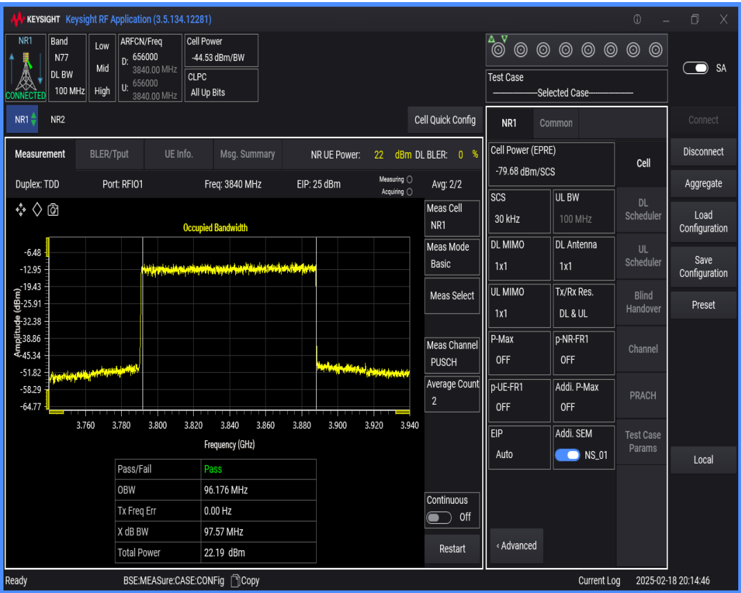
n77(3700-3980) SCS=30kHz DFT_QAM16 BW=15MHz Channel=656000 RB=36@0
