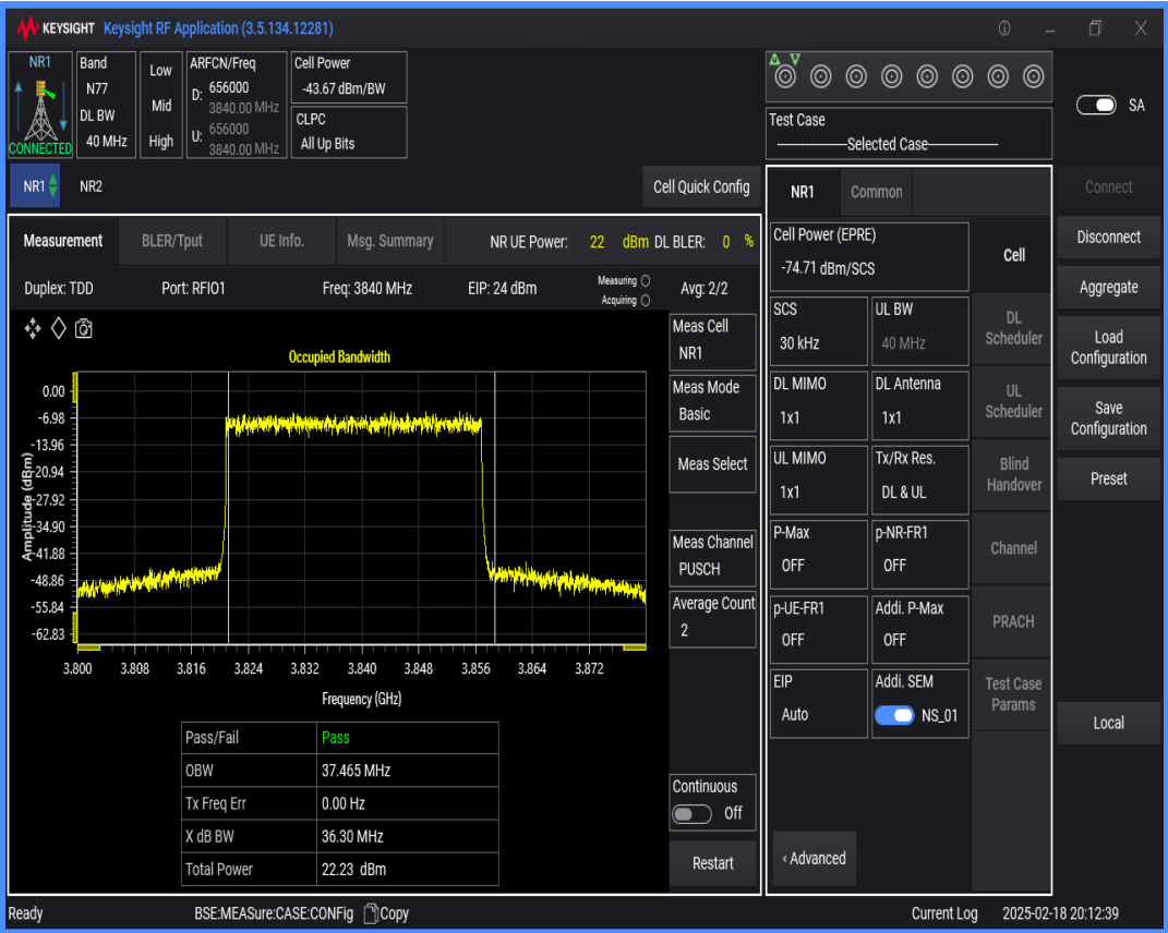
n77(3700-3980) SCS=30kHz DFT_QAM16 BW=80MHz Channel=656000 RB=216@0
