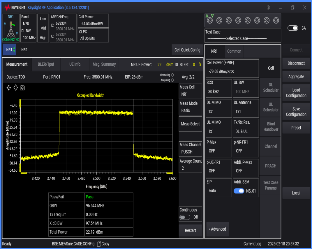
n78(3450-3550) SCS=30kHz DFT_QAM64 BW=10MHz Channel=633334 RB=24@0
