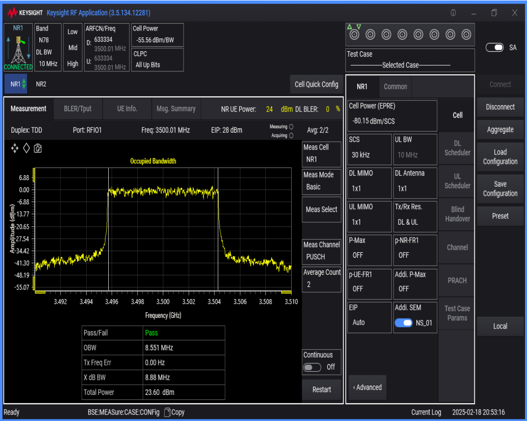
n78(3450-3550) SCS=30kHz DFT_QPSK BW=100MHz Channel=633334 RB=270@0
