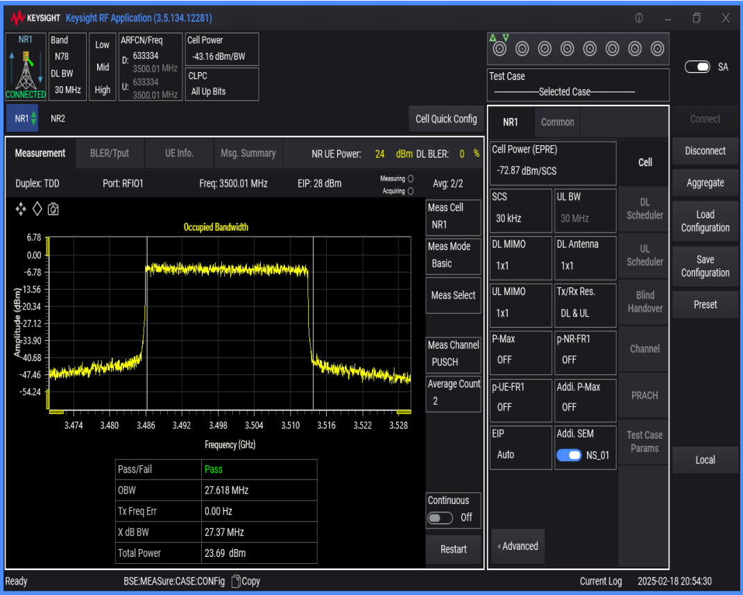
n78(3450-3550) SCS=30kHz DFT_QPSK BW=60MHz Channel=633334 RB=162@0
