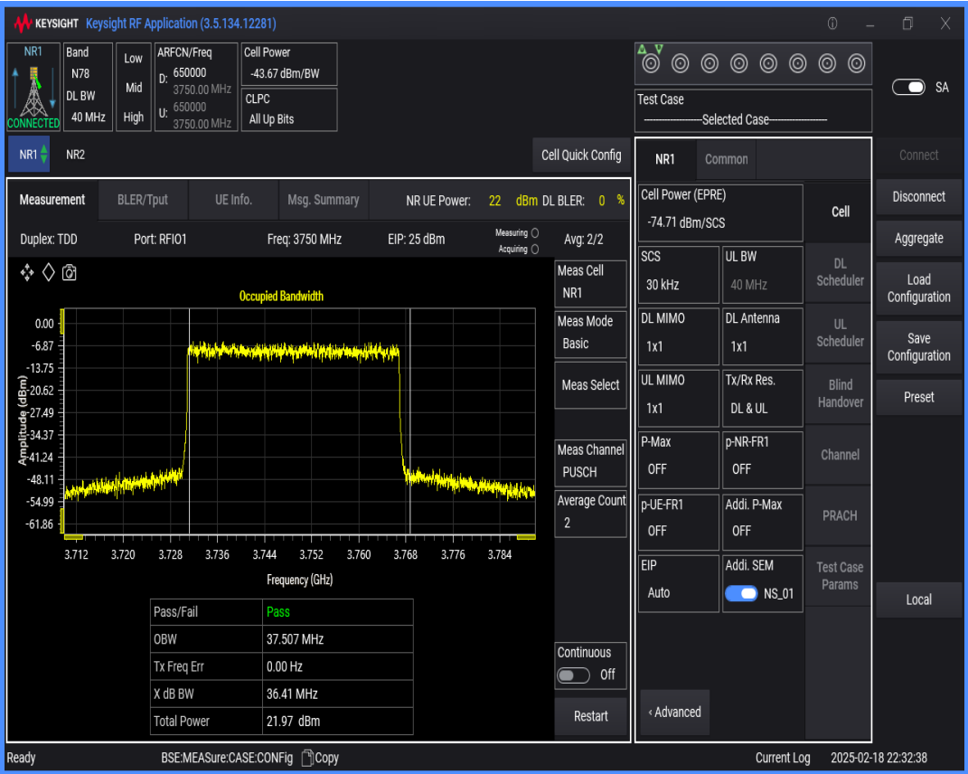
n78(3700-3800) SCS=30kHz DFT_QAM16 BW=60MHz Channel=650000 RB=162@0
