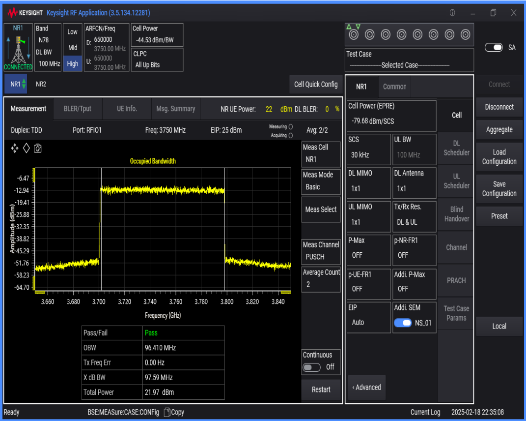
n78(3700-3800) SCS=30kHz DFT_QAM16 BW=10MHz Channel=650000 RB=24@0
