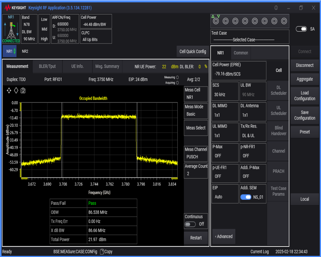
n78(3700-3800) SCS=30kHz DFT_QAM16 BW=80MHz Channel=650000 RB=216@0
