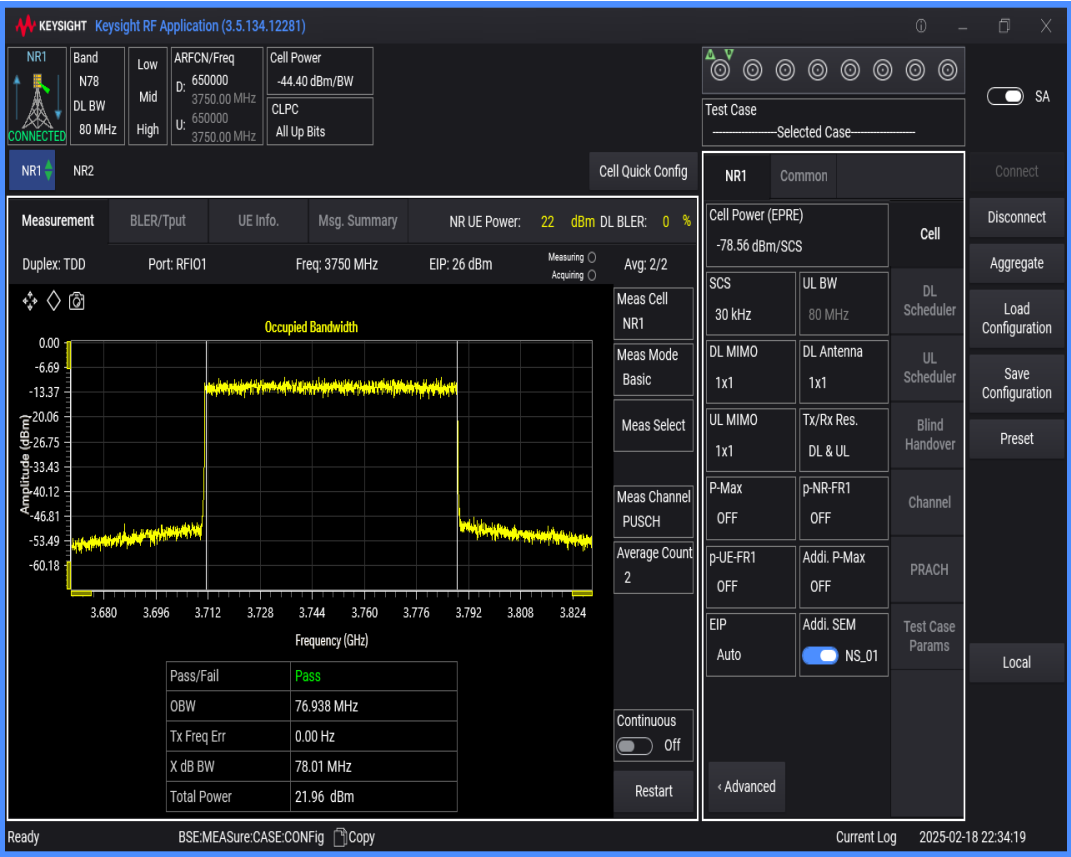
n78(3700-3800) SCS=30kHz DFT_QAM256 BW=15MHz Channel=650000 RB=36@0
