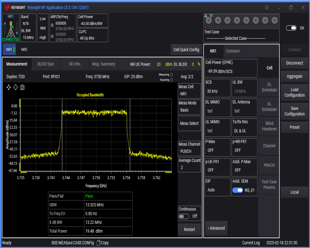
n78(3700-3800) SCS=30kHz DFT_QAM256 BW=10MHz Channel=650000 RB=24@0
