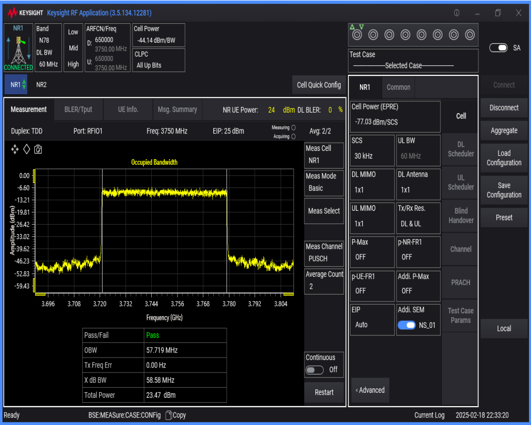
n78(3700-3800) SCS=30kHz DFT_BPSK BW=90MHz Channel=650000 RB=240@0
