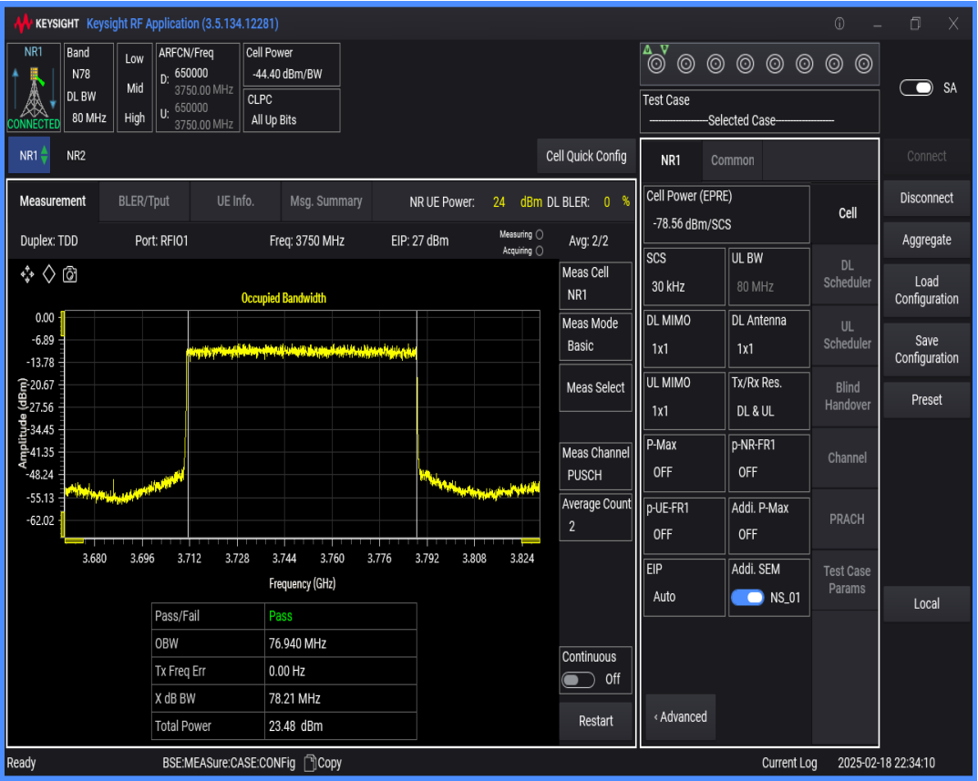
n78(3700-3800) SCS=30kHz DFT_QAM16 BW=100MHz Channel=650000 RB=270@0
