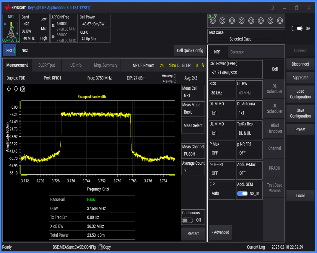
n78(3700-3800) SCS=30kHz DFT_BPSK BW=70MHz Channel=650000 RB=180@0
