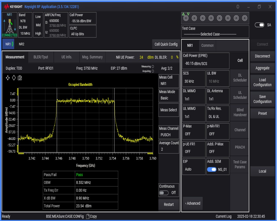
n78(3700-3800) SCS=30kHz DFT_BPSK BW=15MHz Channel=650000 RB=36@0
