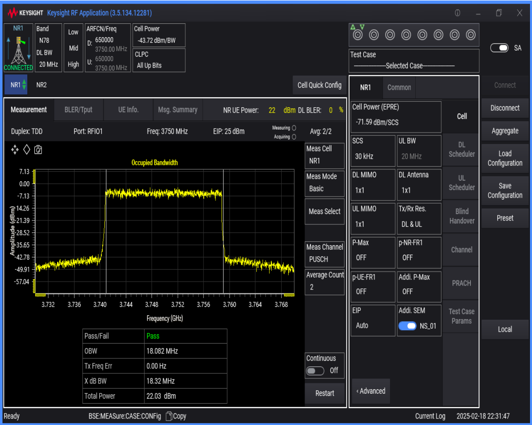
n78(3700-3800) SCS=30kHz DFT_QAM16 BW=50MHz Channel=650000 RB=128@0
