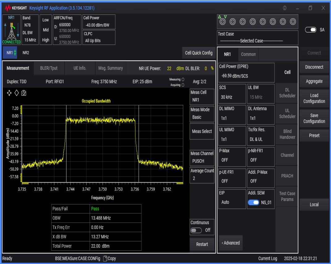
n78(3700-3800) SCS=30kHz DFT_QAM16 BW=30MHz Channel=650000 RB=75@0
