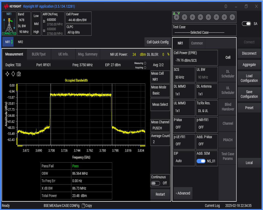
n78(3700-3800) SCS=30kHz DFT_BPSK BW=80MHz Channel=650000 RB=216@0
