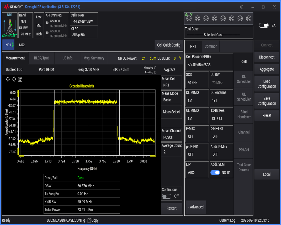
n78(3700-3800) SCS=30kHz DFT_BPSK BW=60MHz Channel=650000 RB=162@0
