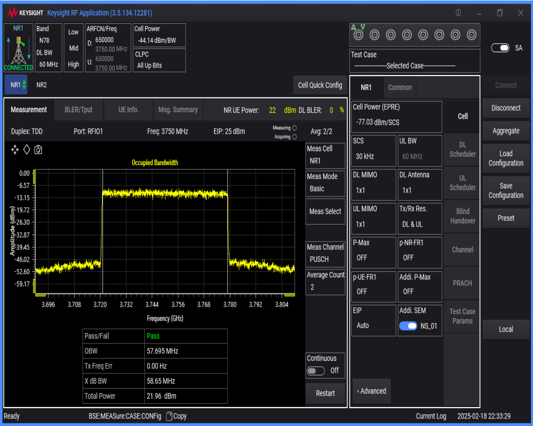
n78(3700-3800) SCS=30kHz DFT_QAM16 BW=70MHz Channel=650000 RB=180@0
