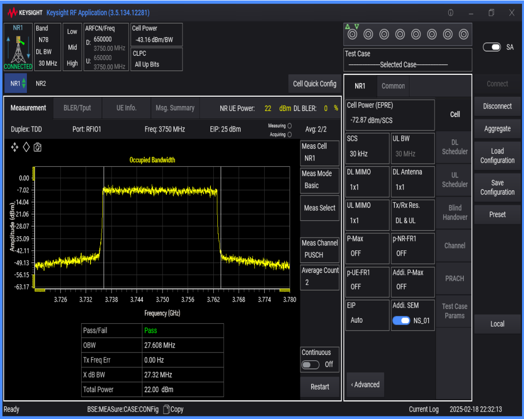
n78(3700-3800) SCS=30kHz DFT_QAM16 BW=20MHz Channel=650000 RB=50@0
