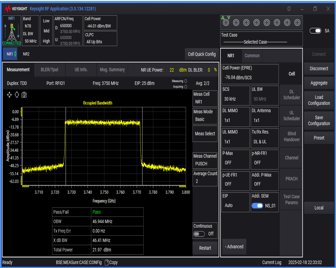
n78(3700-3800) SCS=30kHz DFT_QAM16 BW=40MHz Channel=650000 RB=100@0
