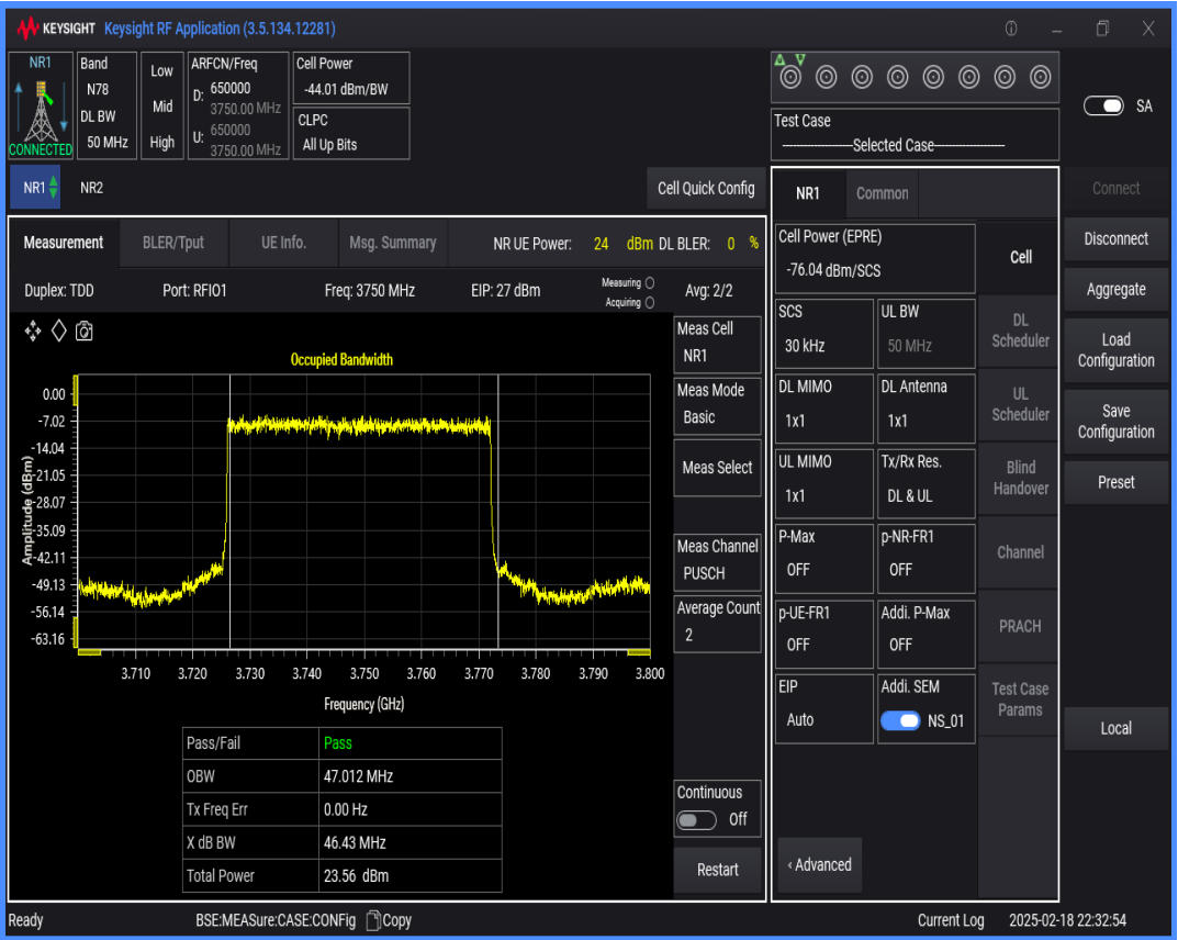
n78(3700-3800) SCS=30kHz DFT_BPSK BW=40MHz Channel=650000 RB=100@0
