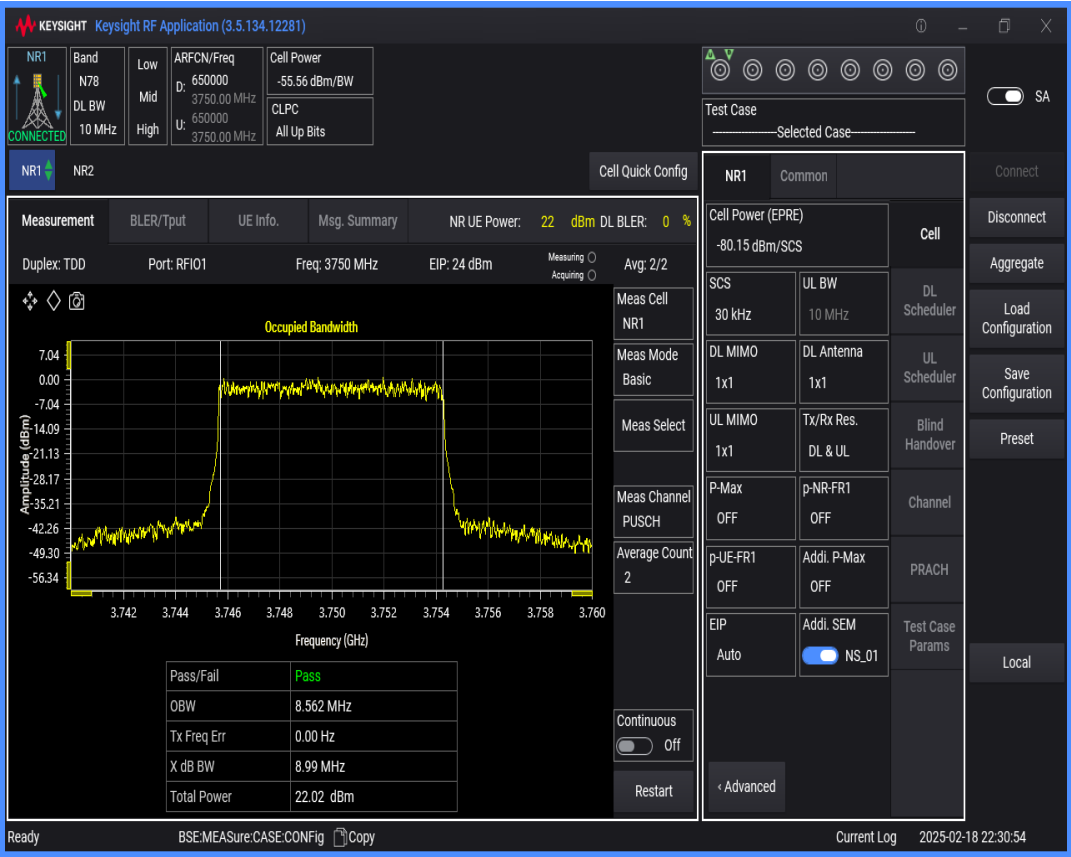
n78(3700-3800) SCS=30kHz DFT_QAM16 BW=15MHz Channel=650000 RB=36@0
