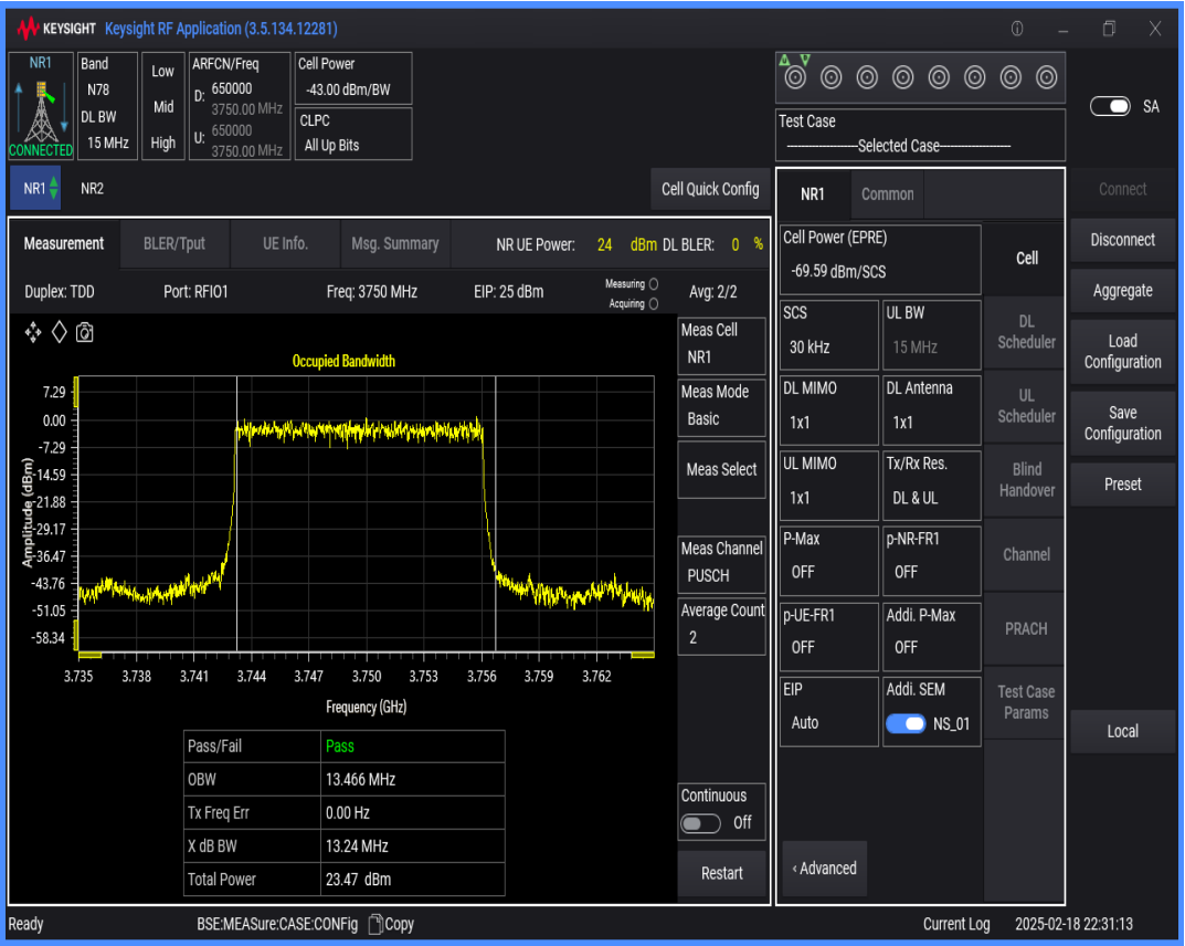
n78(3700-3800) SCS=30kHz DFT_BPSK BW=30MHz Channel=650000 RB=75@0
