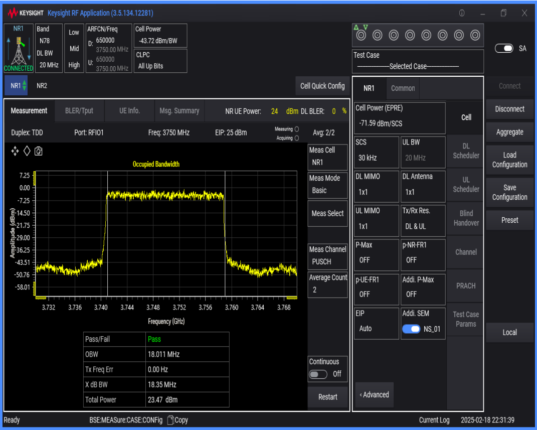
n78(3700-3800) SCS=30kHz DFT_BPSK BW=50MHz Channel=650000 RB=128@0
