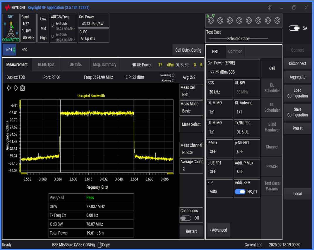
n77(3550-3700) SCS=30kHz DFT_QAM256 BW=40MHz Channel=641666 RB=100@0
