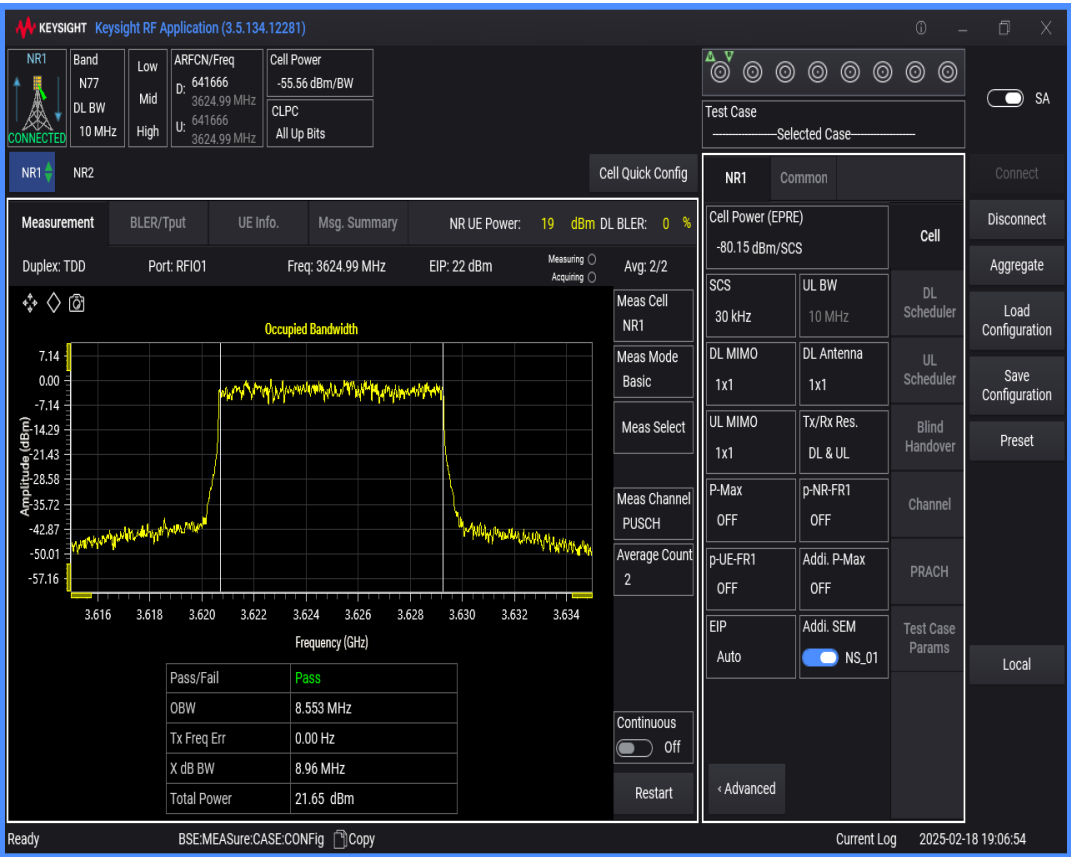
n77(3550-3700) SCS=30kHz DFT_QAM64 BW=15MHz Channel=641666 RB=36@0
