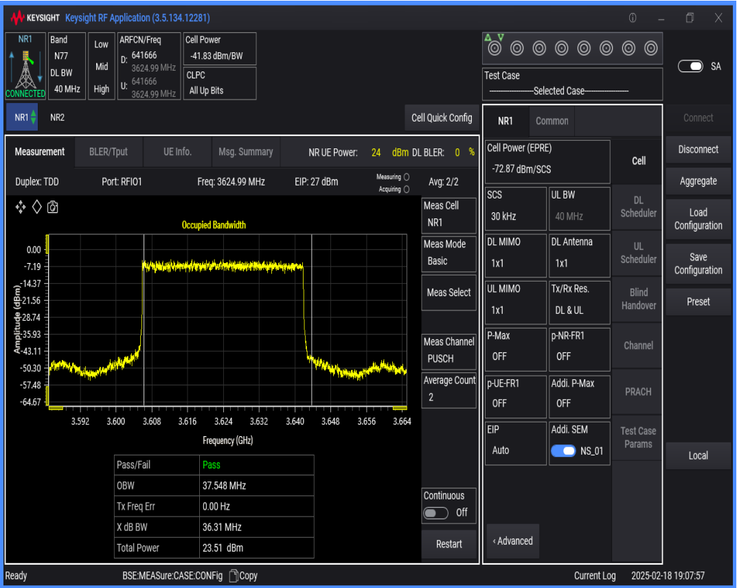
n77(3550-3700) SCS=30kHz DFT_BPSK BW=60MHz Channel=641666 RB=162@0
