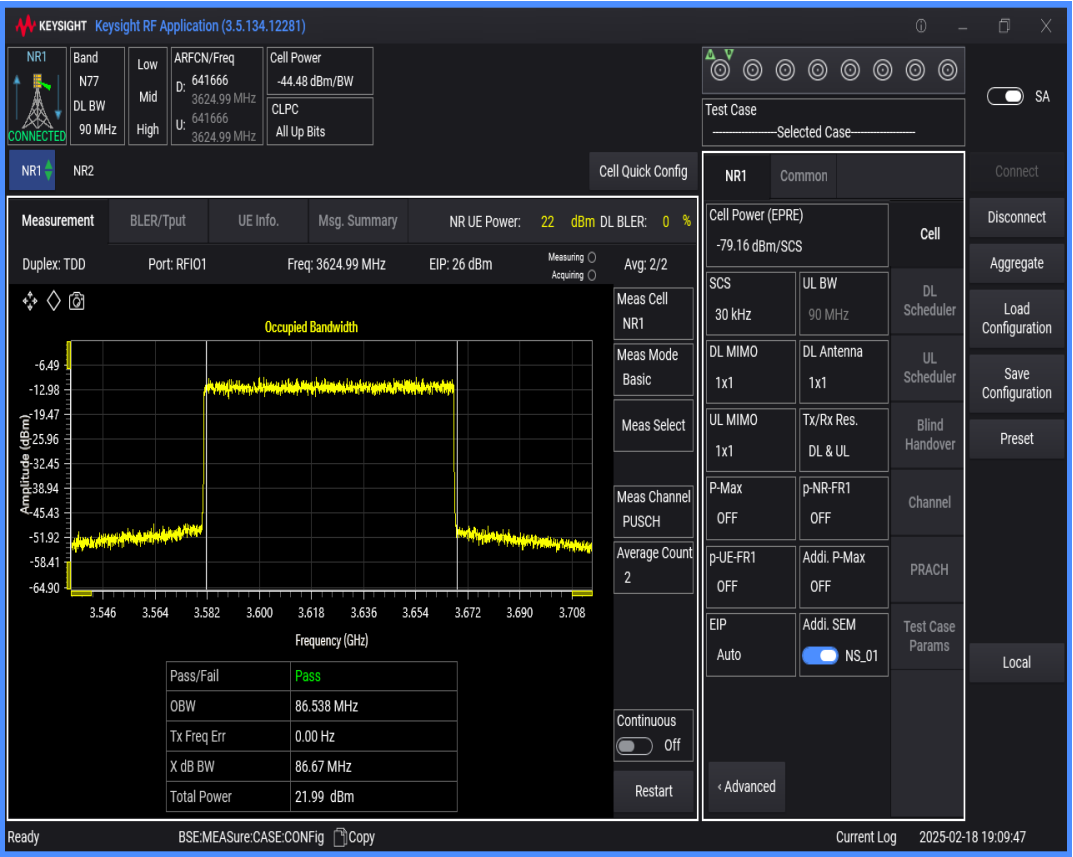
n77(3550-3700) SCS=30kHz DFT_QAM16 BW=80MHz Channel=641666 RB=216@0
