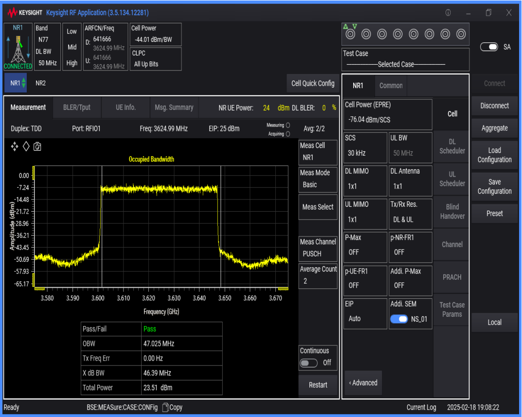
n77(3550-3700) SCS=30kHz DFT_BPSK BW=40MHz Channel=641666 RB=100@0
