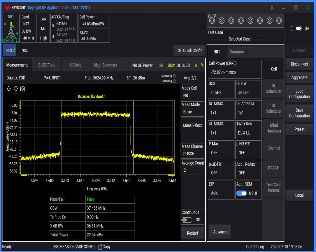
n77(3550-3700) SCS=30kHz DFT_QAM16 BW=90MHz Channel=641666 RB=240@0
