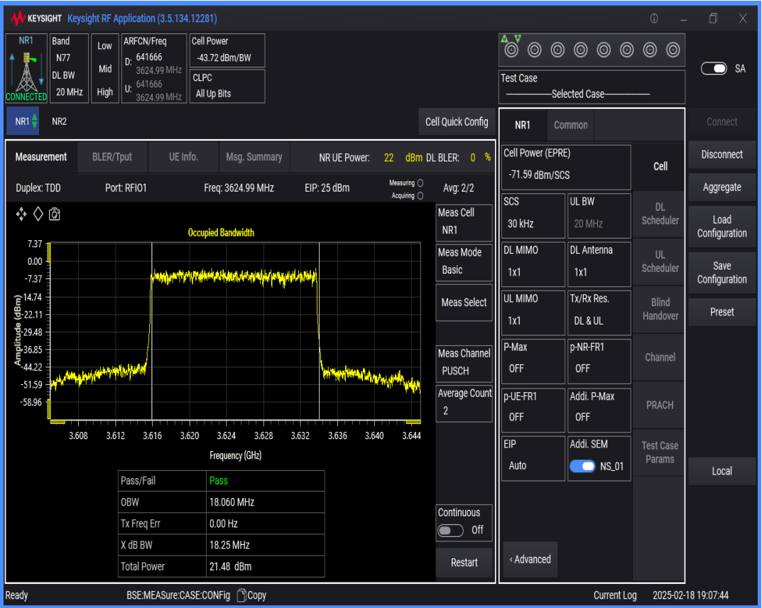
n77(3550-3700) SCS=30kHz DFT_QAM64 BW=40MHz Channel=641666 RB=100@0
