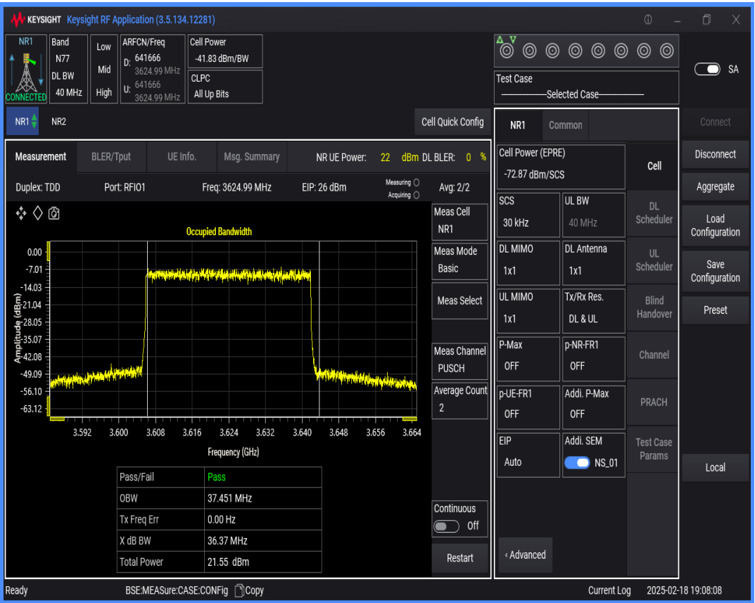
n77(3550-3700) SCS=30kHz DFT_QPSK BW=10MHz Channel=641666 RB=24@0
