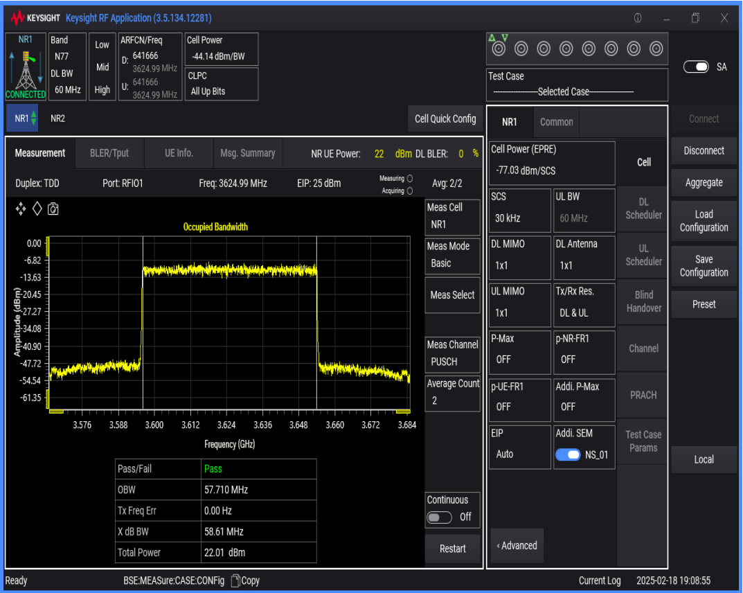
n77(3550-3700) SCS=30kHz DFT_QAM16 BW=50MHz Channel=641666 RB=128@0
