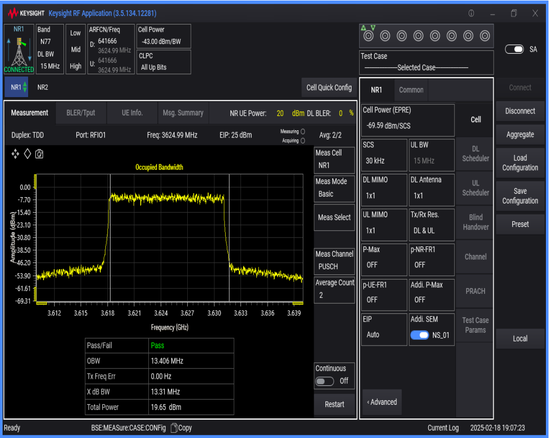
n77(3550-3700) SCS=30kHz DFT_QAM256 BW=10MHz Channel=641666 RB=24@0
