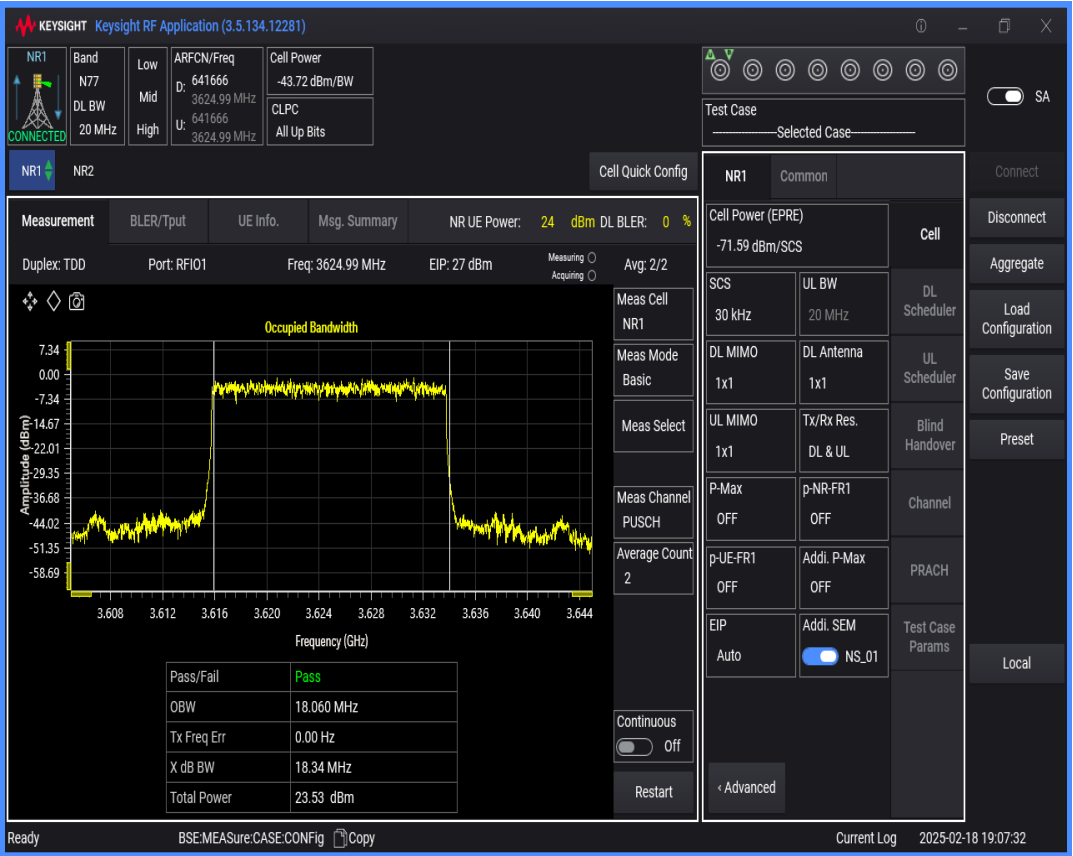
n77(3550-3700) SCS=30kHz DFT_BPSK BW=50MHz Channel=641666 RB=128@0
