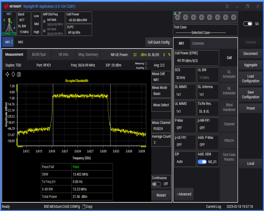
n77(3550-3700) SCS=30kHz DFT_QAM256 BW=90MHz Channel=641666 RB=240@0
