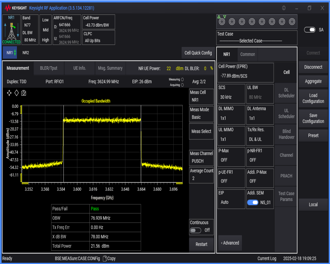
n77(3550-3700) SCS=30kHz DFT_QAM64 BW=50MHz Channel=641666 RB=128@0
