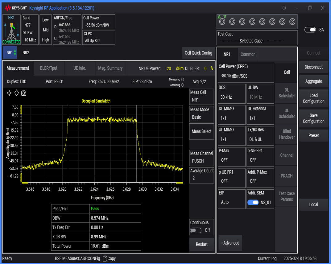
n77(3550-3700) SCS=30kHz DFT_QAM256 BW=100MHz Channel=641666 RB=270@0
