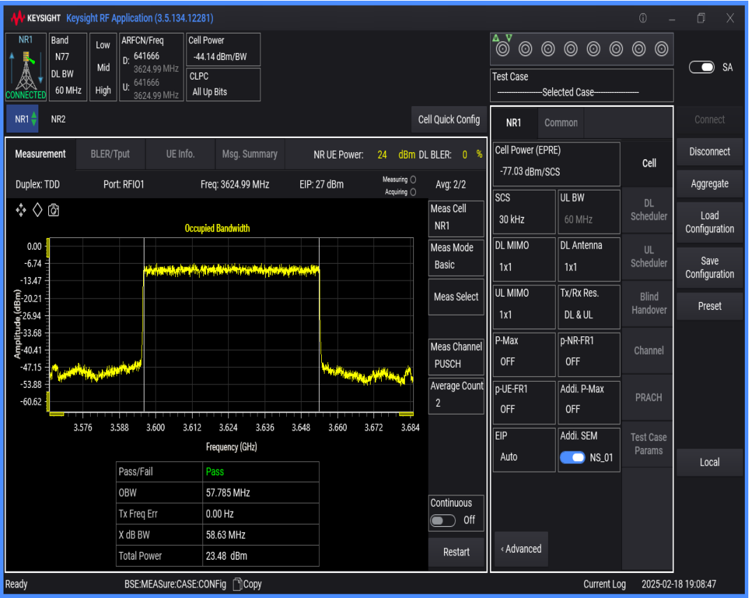
n77(3550-3700) SCS=30kHz DFT_BPSK BW=80MHz Channel=641666 RB=216@0
