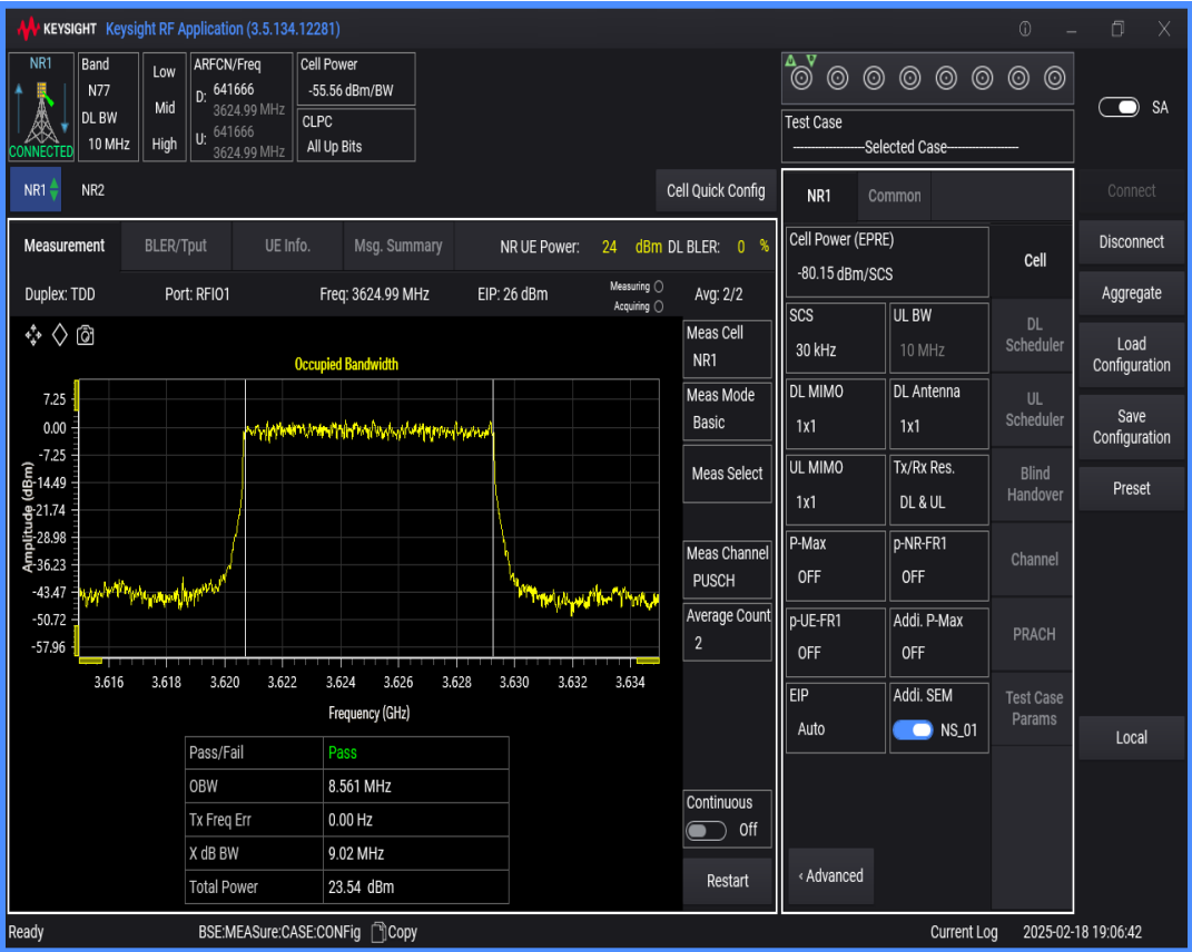
n77(3550-3700) SCS=30kHz DFT_BPSK BW=15MHz Channel=641666 RB=36@0
