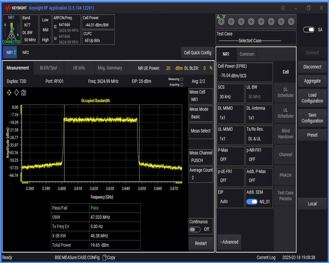
n77(3550-3700) SCS=30kHz DFT_QAM64 BW=10MHz Channel=641666 RB=24@0
