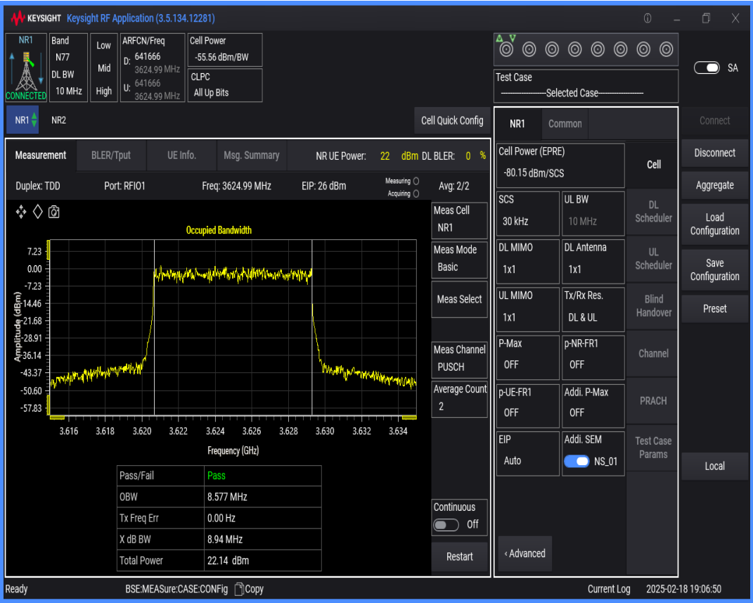
n77(3550-3700) SCS=30kHz DFT_QAM16 BW=100MHz Channel=641666 RB=270@0
