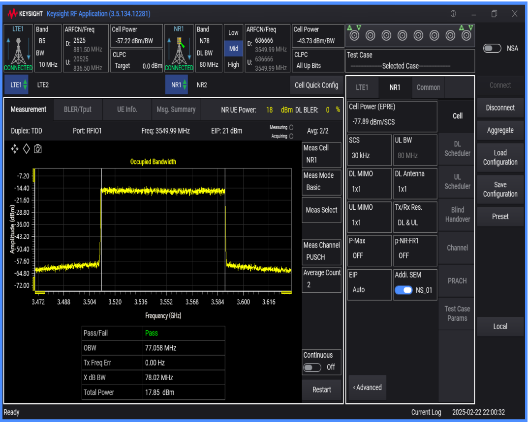
n78 SCS=30kHz DFT_QAM64 BW=100MHz Channel=636666 RB=270@0
