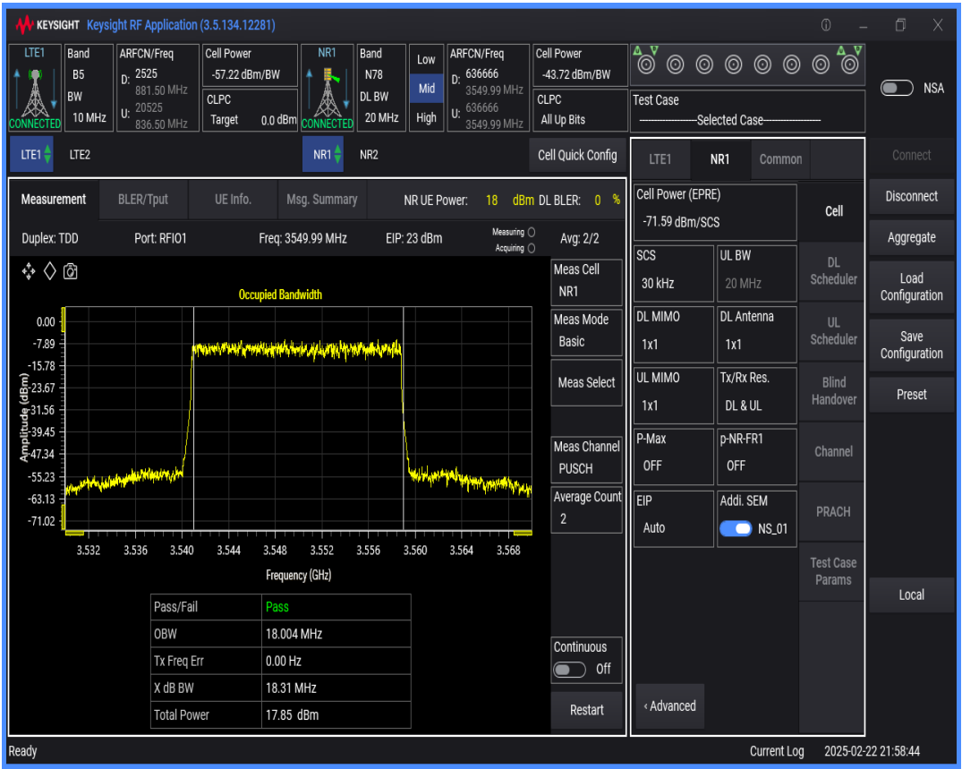
n78 SCS=30kHz DFT_QAM256 BW=60MHz Channel=636666 RB=162@0
