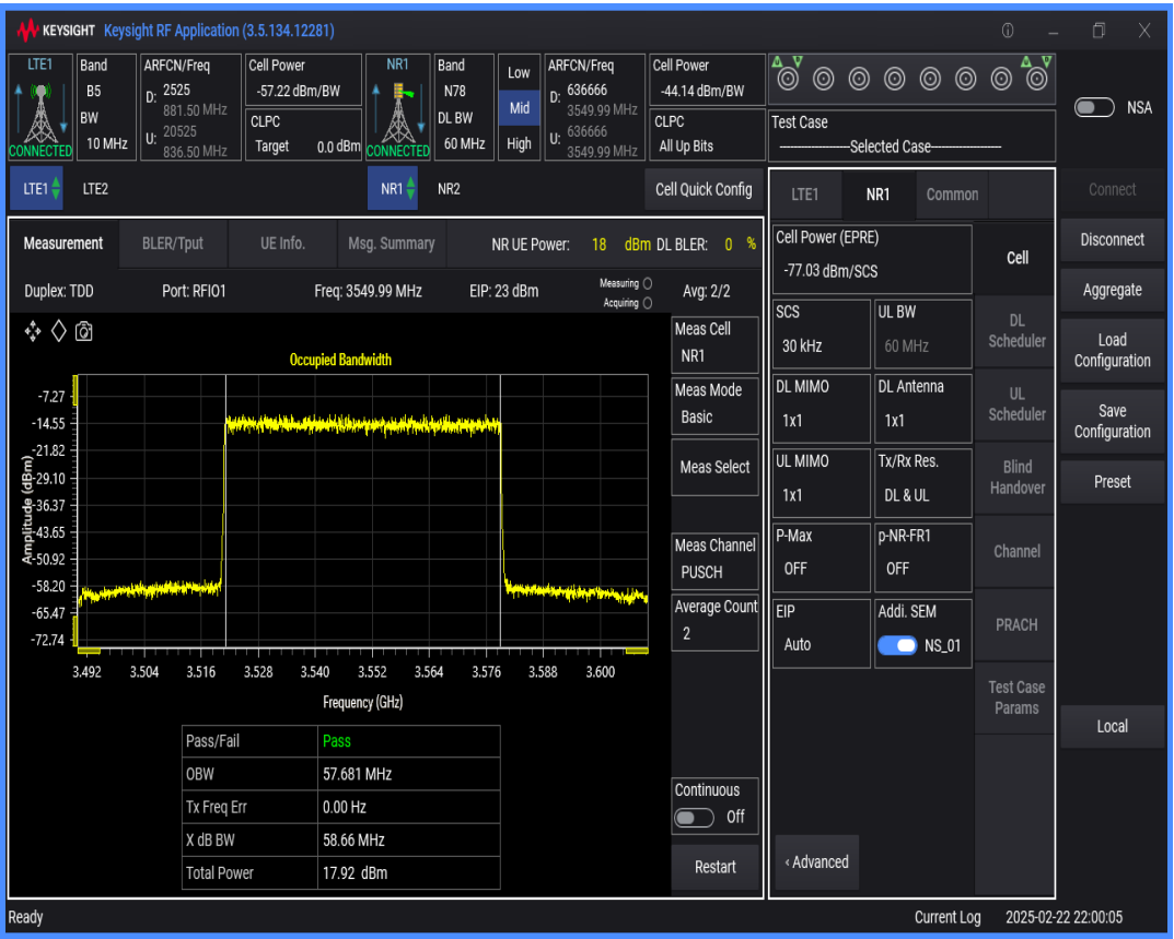
n78 SCS=30kHz DFT_QAM256 BW=80MHz Channel=636666 RB=216@0
