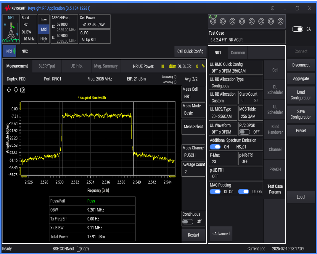
n7 SCS=15kHz DFT_QAM16 BW=5MHz Channel=507000 RB=25@0
