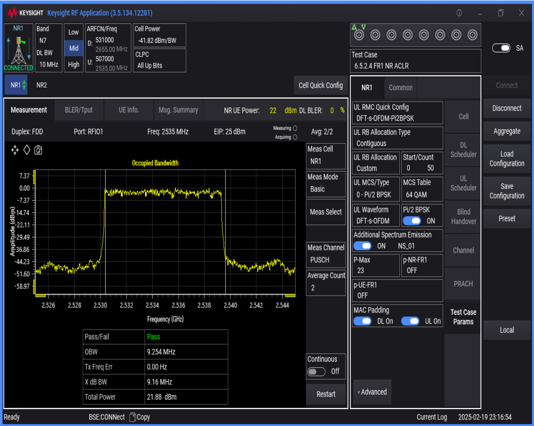
n7 SCS=15kHz DFT_BPSK BW=15MHz Channel=507000 RB=75@0
