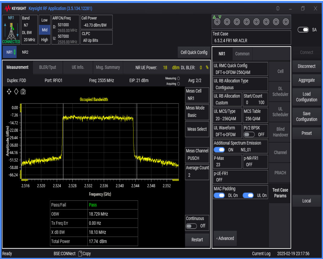
n7 SCS=15kHz DFT_QAM256 BW=15MHz Channel=507000 RB=75@0
