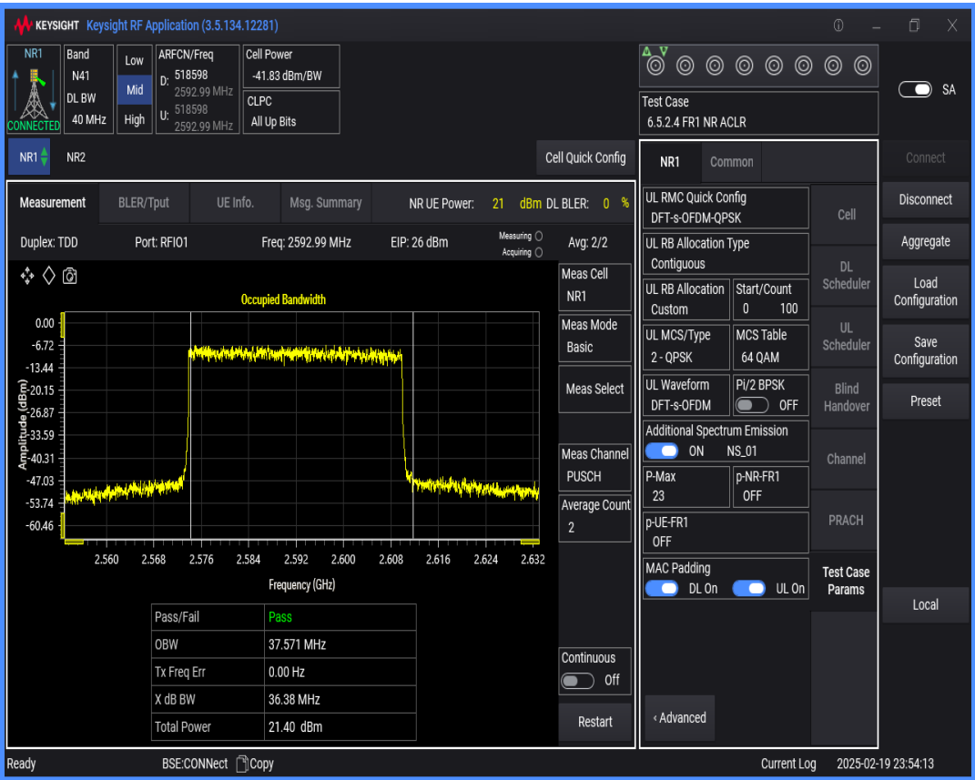
n41 SCS=30kHz DFT_QPSK BW=60MHz Channel=518598 RB=162@0
