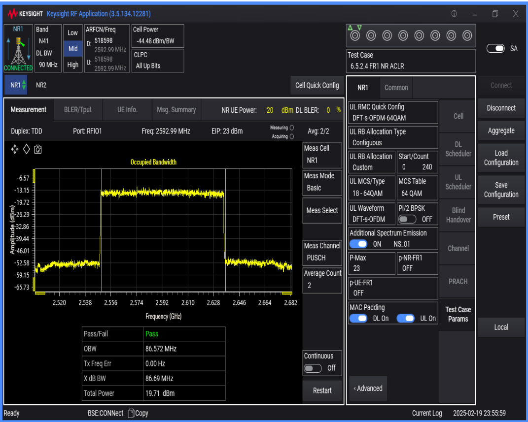
n41 SCS=30kHz DFT_QPSK BW=100MHz Channel=518598 RB=270@0
