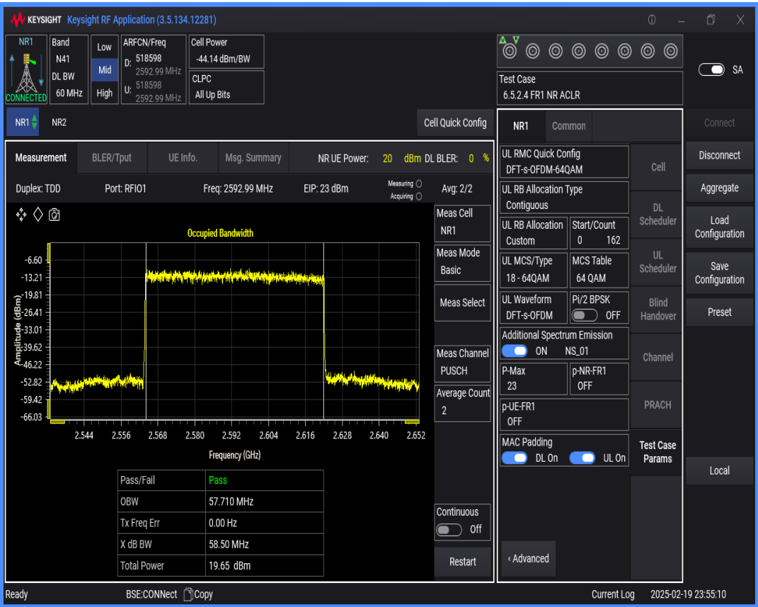
n41 SCS=30kHz DFT_QAM64 BW=80MHz Channel=518598 RB=216@0
