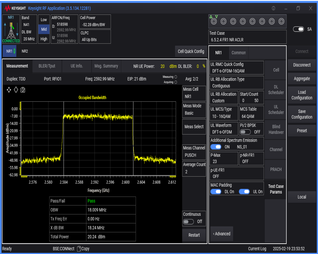
n41 SCS=30kHz DFT_QAM16 BW=100MHz Channel=518598 RB=270@0
