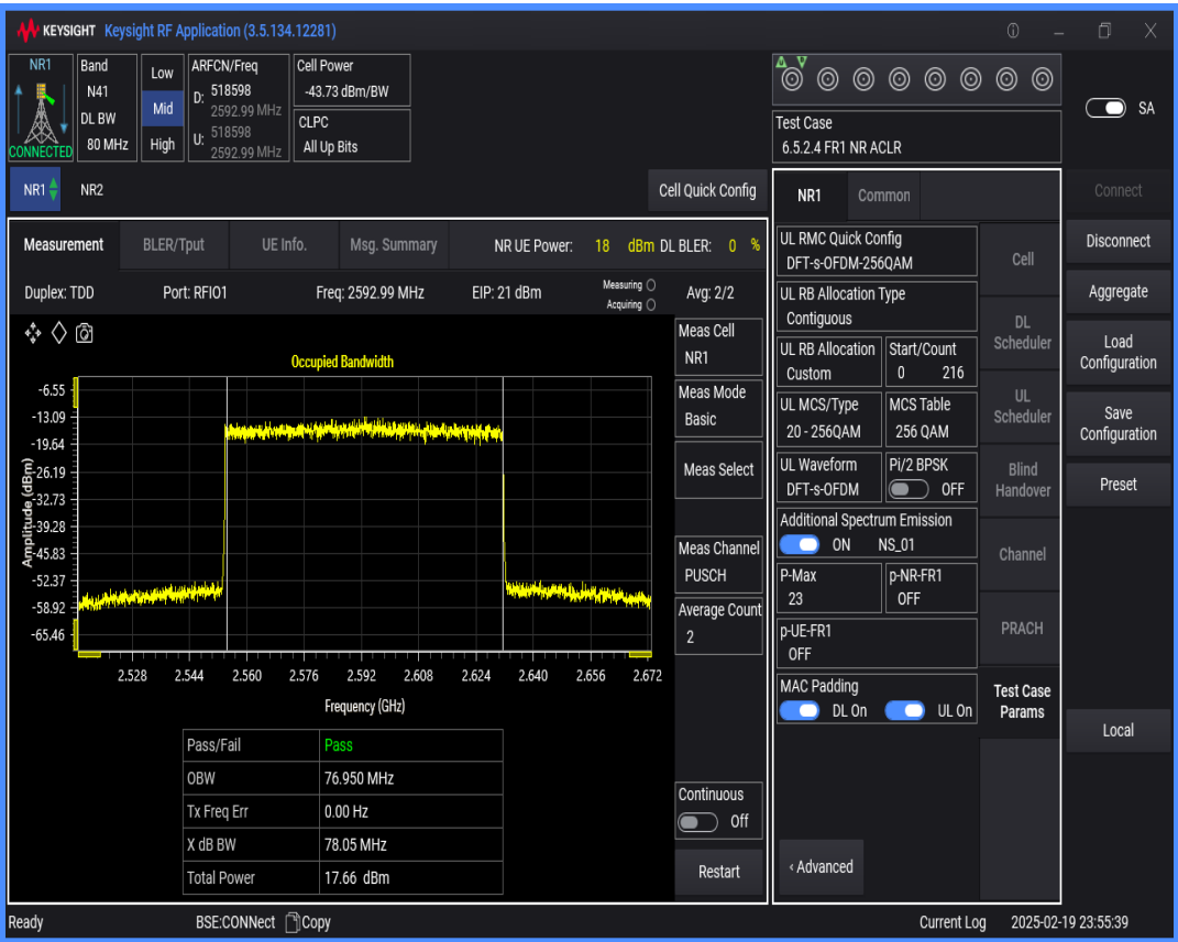
n41 SCS=30kHz DFT_QAM64 BW=100MHz Channel=518598 RB=270@0
