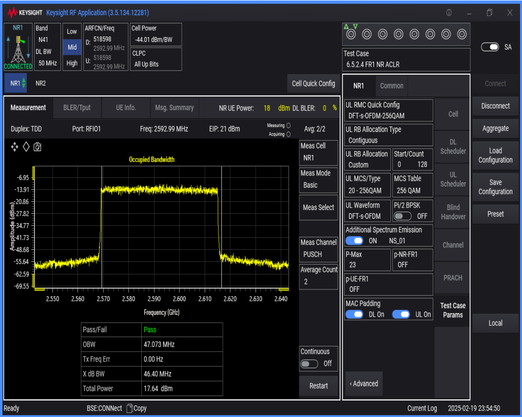
n41 SCS=30kHz DFT_QAM256 BW=80MHz Channel=518598 RB=216@0
