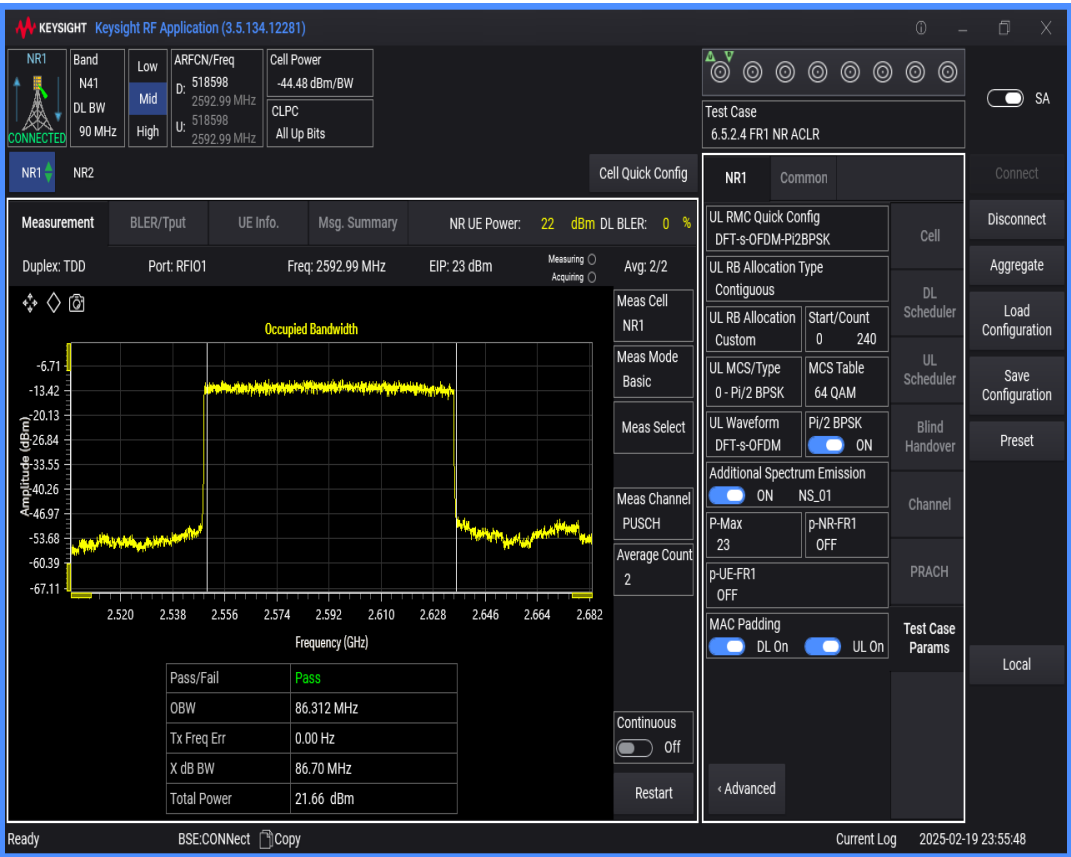
n41 SCS=30kHz DFT_BPSK BW=80MHz Channel=518598 RB=216@0
