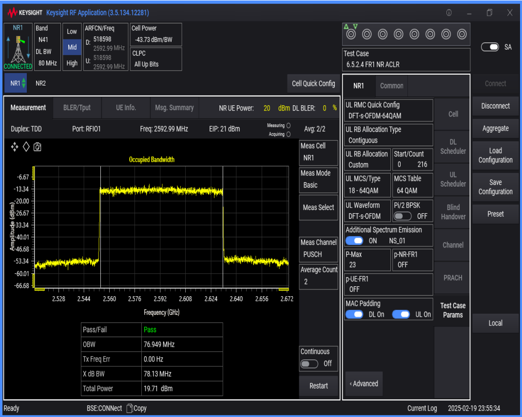
n41 SCS=30kHz DFT_QAM64 BW=90MHz Channel=518598 RB=240@0
