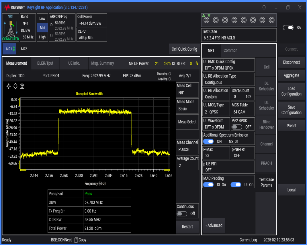
n41 SCS=30kHz DFT_QPSK BW=80MHz Channel=518598 RB=216@0
