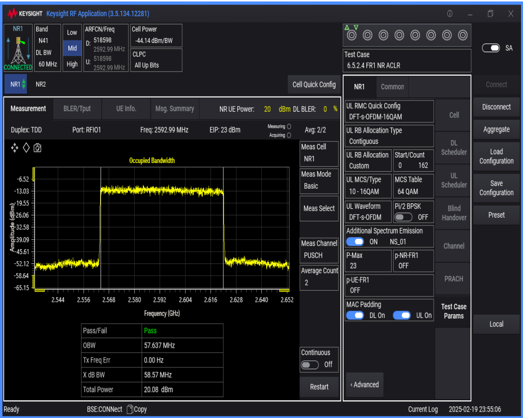
n41 SCS=30kHz DFT_QAM16 BW=90MHz Channel=518598 RB=240@0
