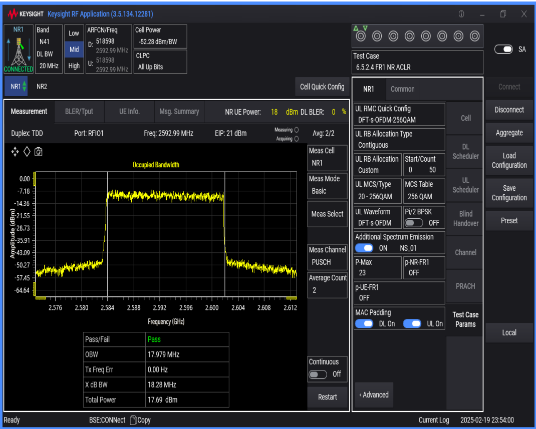
n41 SCS=30kHz DFT_QAM256 BW=40MHz Channel=518598 RB=100@0
