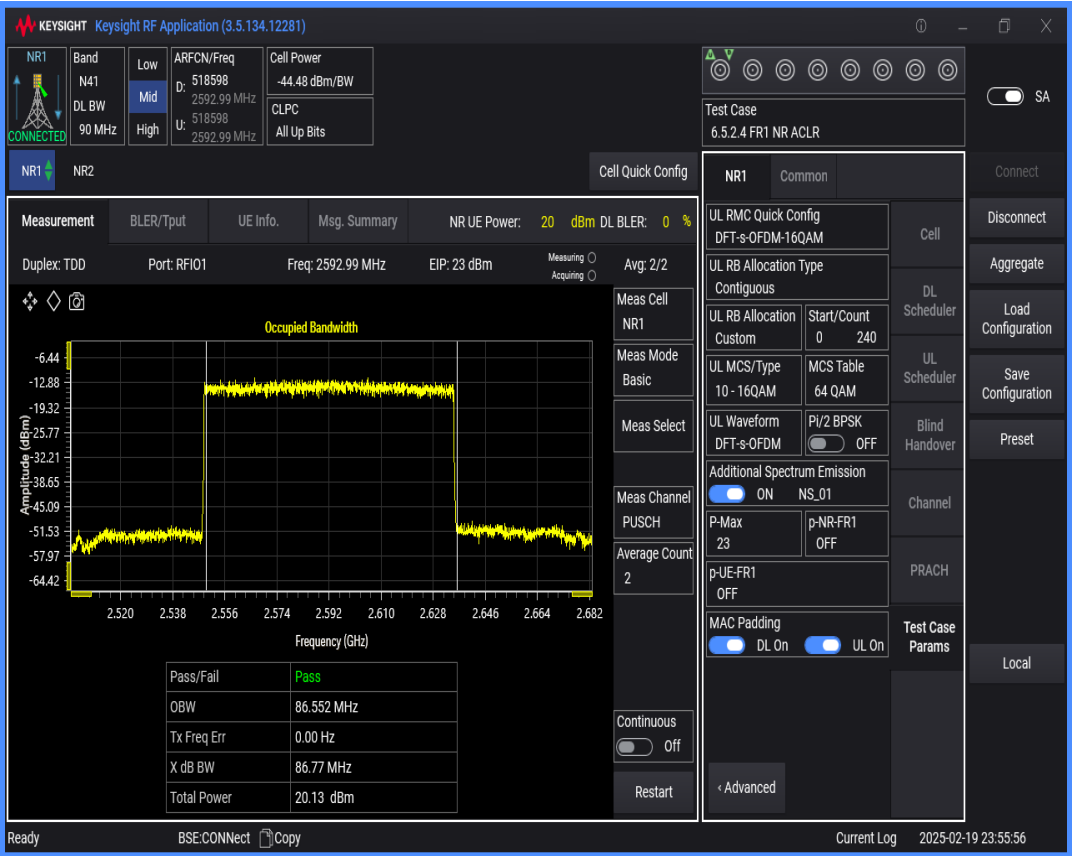
n41 SCS=30kHz DFT_QAM16 BW=80MHz Channel=518598 RB=216@0
