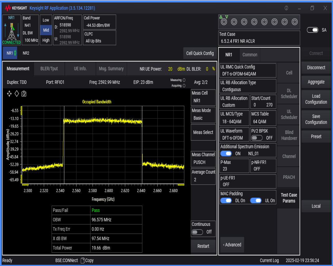
n41 SCS=30kHz DFT_QAM256 BW=90MHz Channel=518598 RB=240@0
