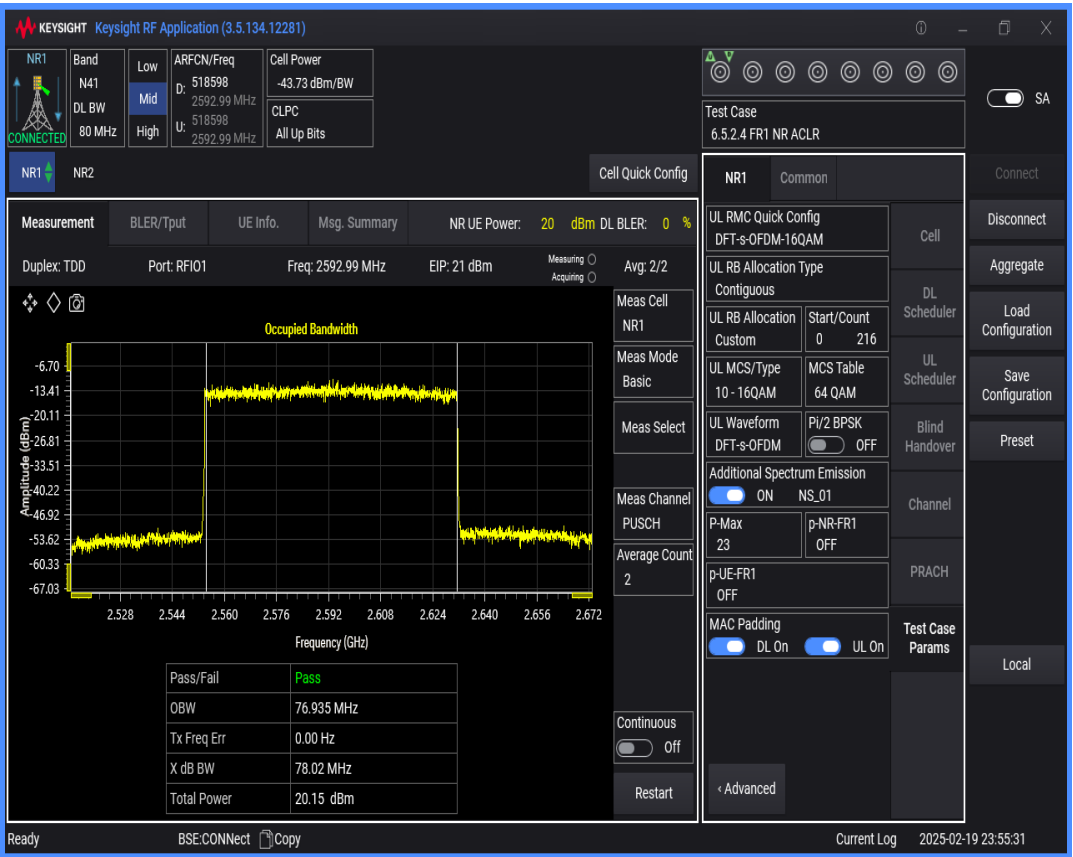
n41 SCS=30kHz DFT_QAM256 BW=100MHz Channel=518598 RB=270@0
