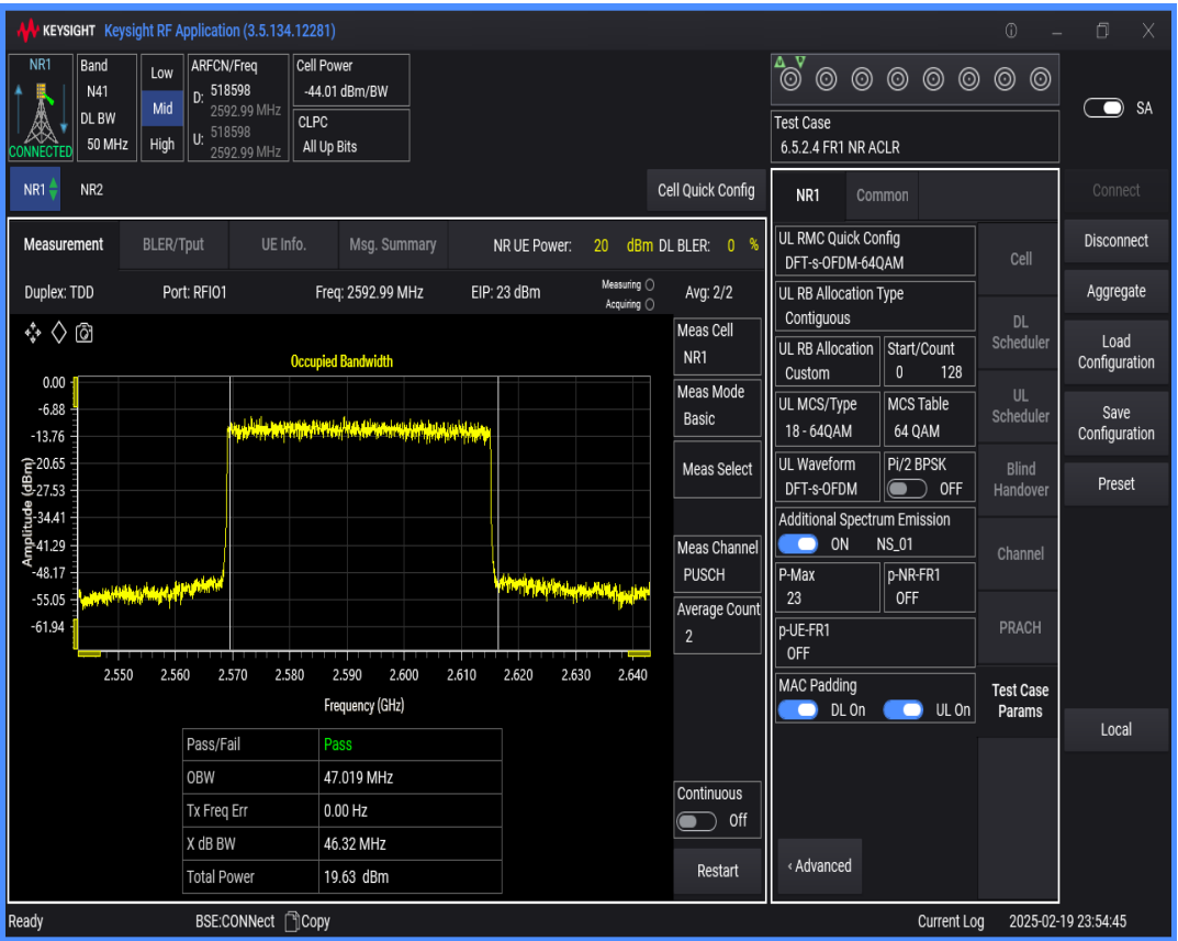
n41 SCS=30kHz DFT_QAM64 BW=40MHz Channel=518598 RB=100@0
