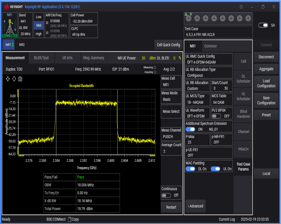
n41 SCS=30kHz DFT_QAM64 BW=50MHz Channel=518598 RB=128@0
