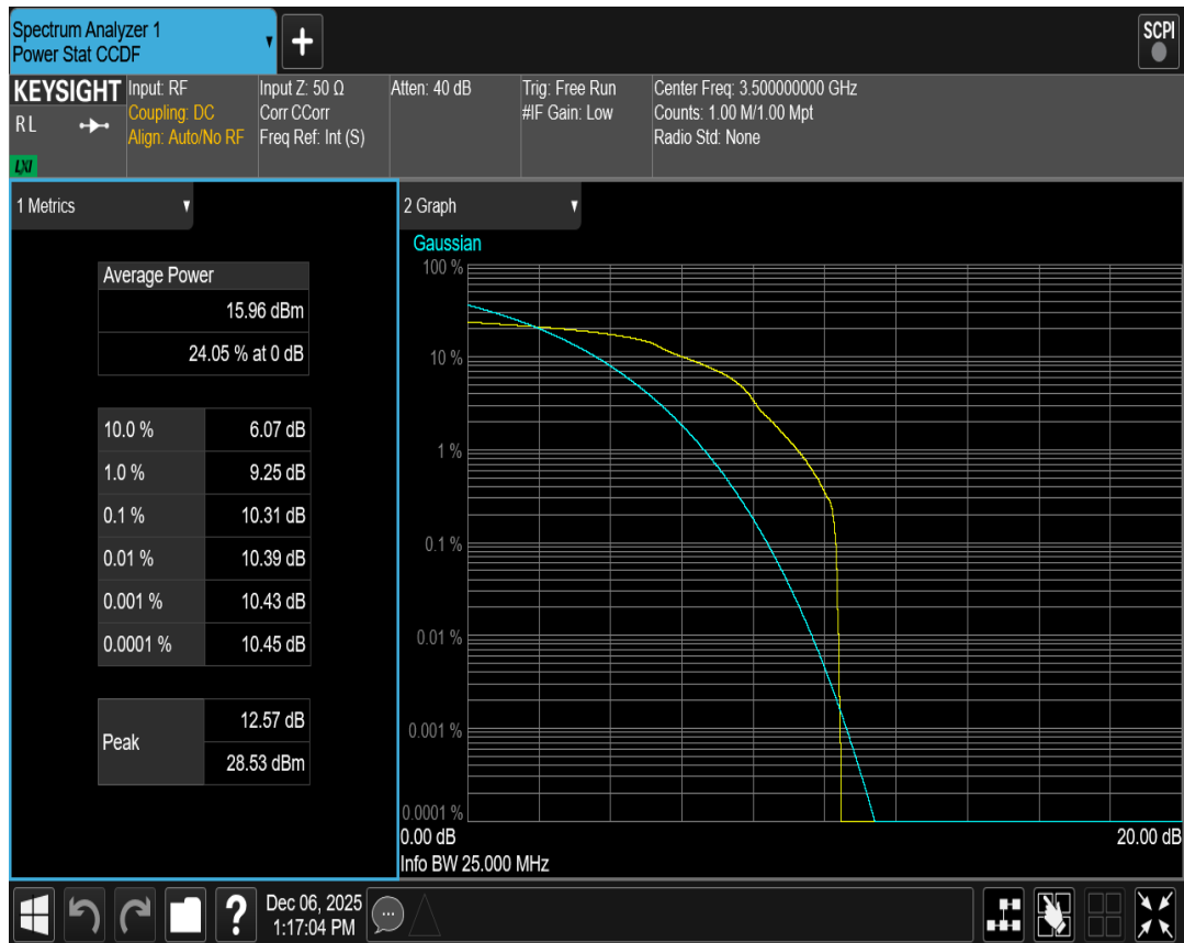
Band42(3450-3550) QPSK BW=10MHz Channel=42590 RB Size=1 Position=#0
