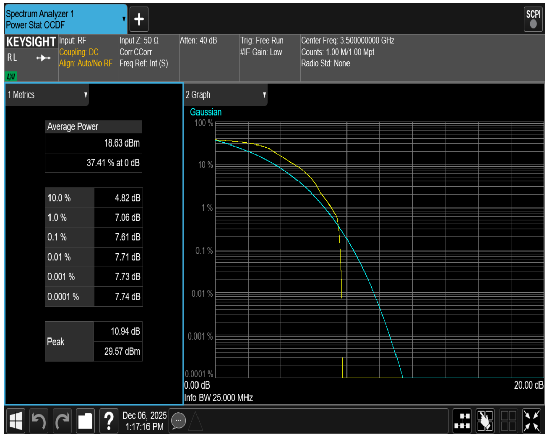
Band42(3450-3550) QPSK BW=20MHz Channel=42590 RB Size=1 Position=#0
