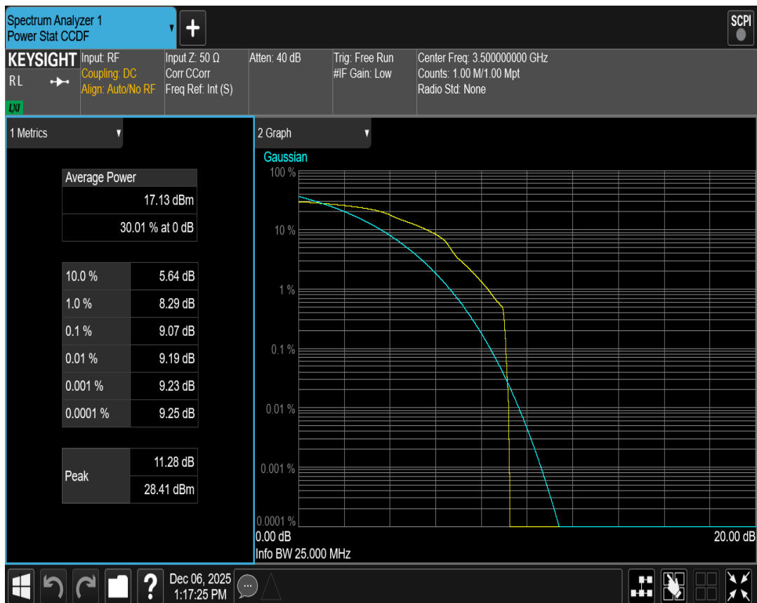
Band42(3450-3550) QAM16 BW=5MHz Channel=42590 RB Size=1 Position=#0
