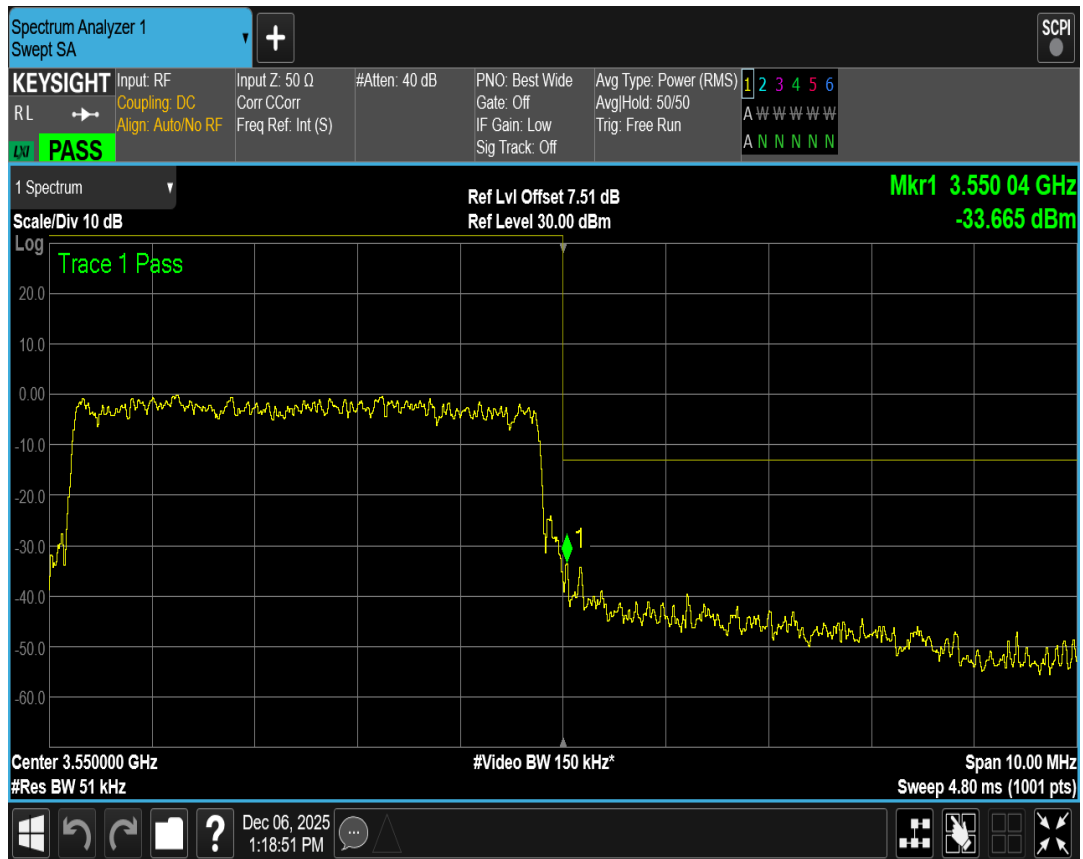
Band42(3450-3550) QPSK BW=10MHz Channel=42140 RB Size=50 Position=#0
