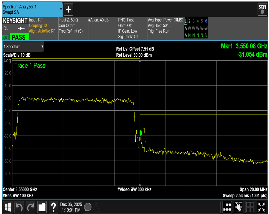
Band42(3450-3550) QPSK BW=15MHz Channel=42165 RB Size=75 Position=#0
