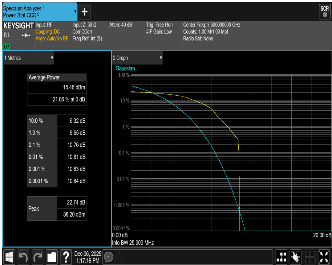
Band42(3450-3550) QAM16 BW=20MHz Channel=42590 RB Size=1 Position=#0
