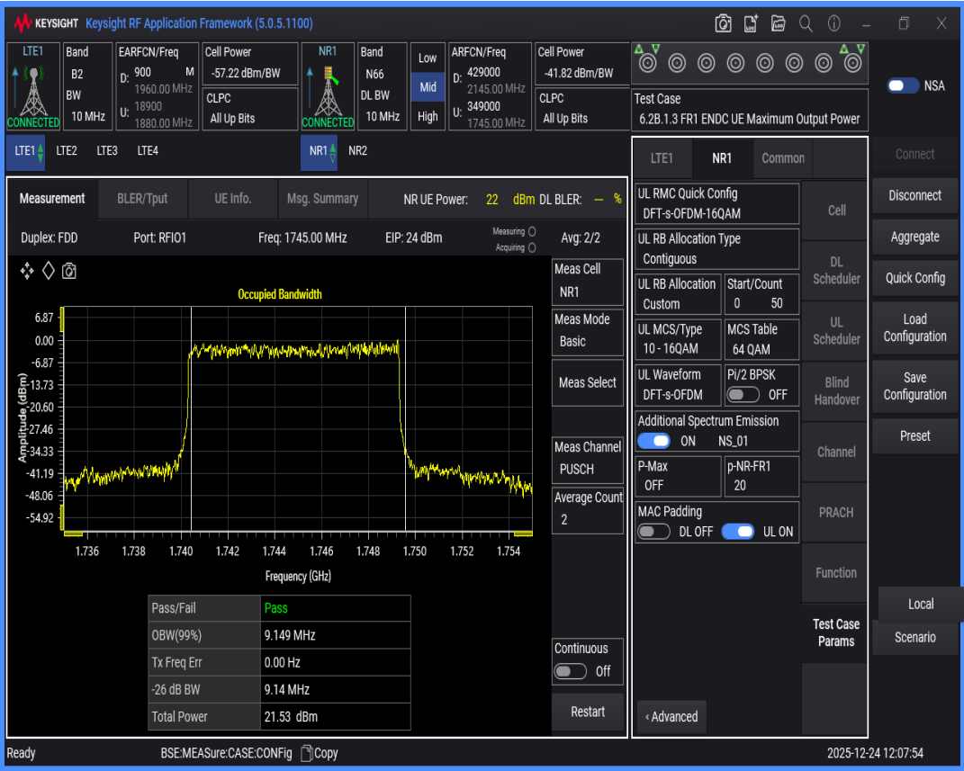
n66 SCS=15kHz DFT_QAM16 BW=15MHz Channel=349000 RB=75@0
