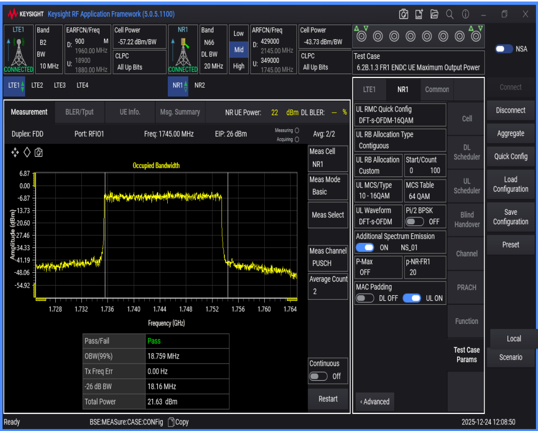
n66 SCS=15kHz DFT_QAM16 BW=40MHz Channel=349000 RB=216@0
