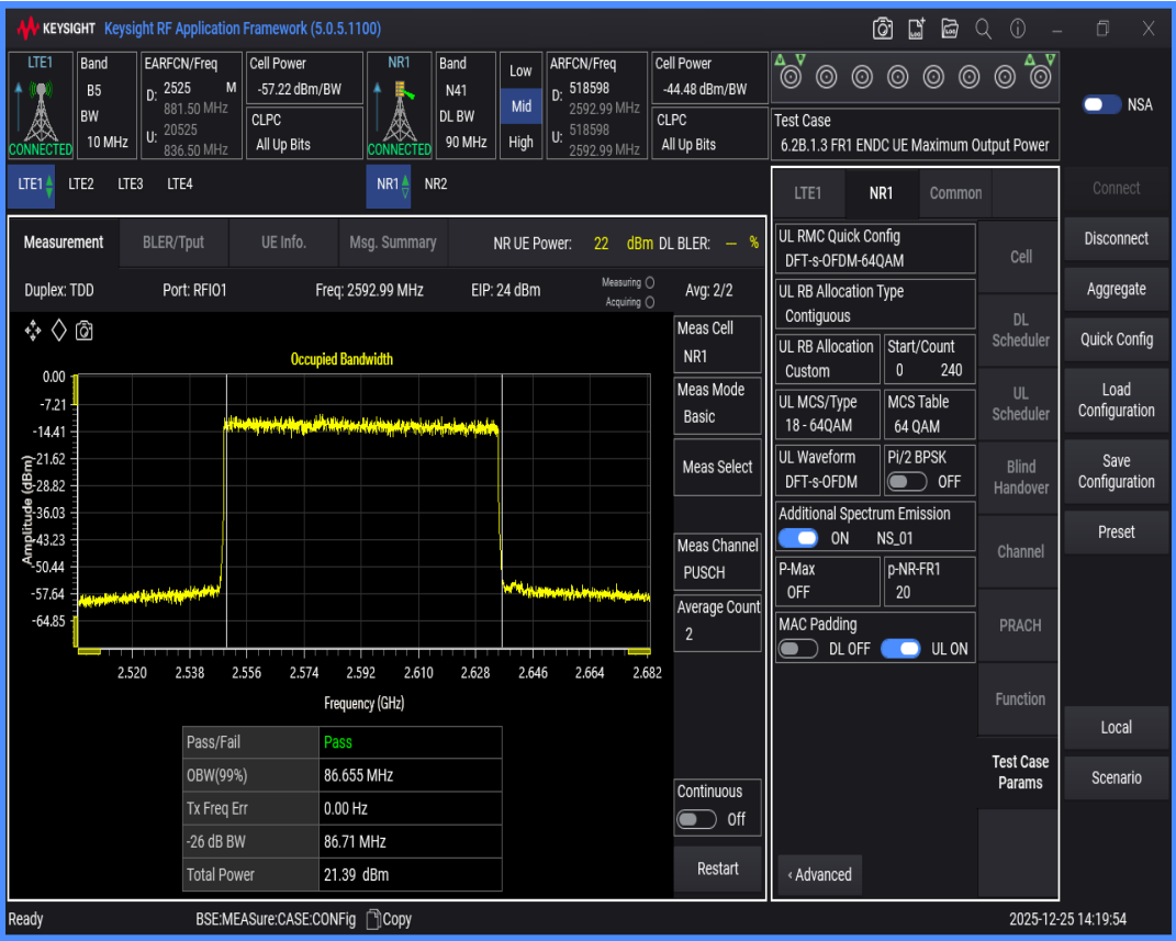
n41 SCS=30kHz DFT_QPSK BW=100MHz Channel=518598 RB=270@0
