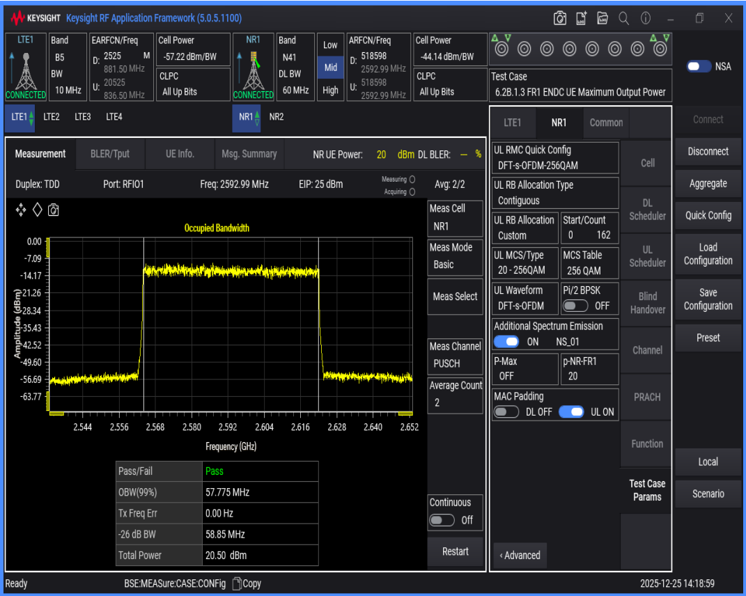
n41 SCS=30kHz DFT_QAM256 BW=80MHz Channel=518598 RB=216@0
