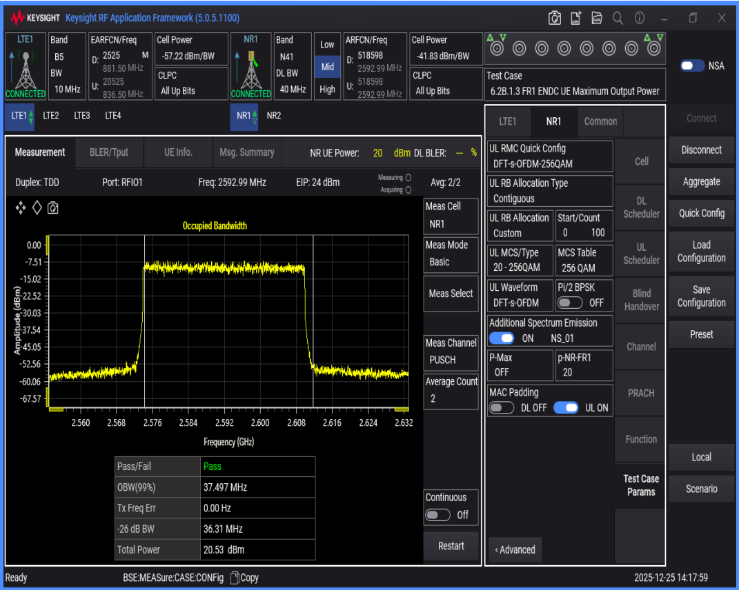
n41 SCS=30kHz DFT_QAM256 BW=50MHz Channel=518598 RB=128@0
