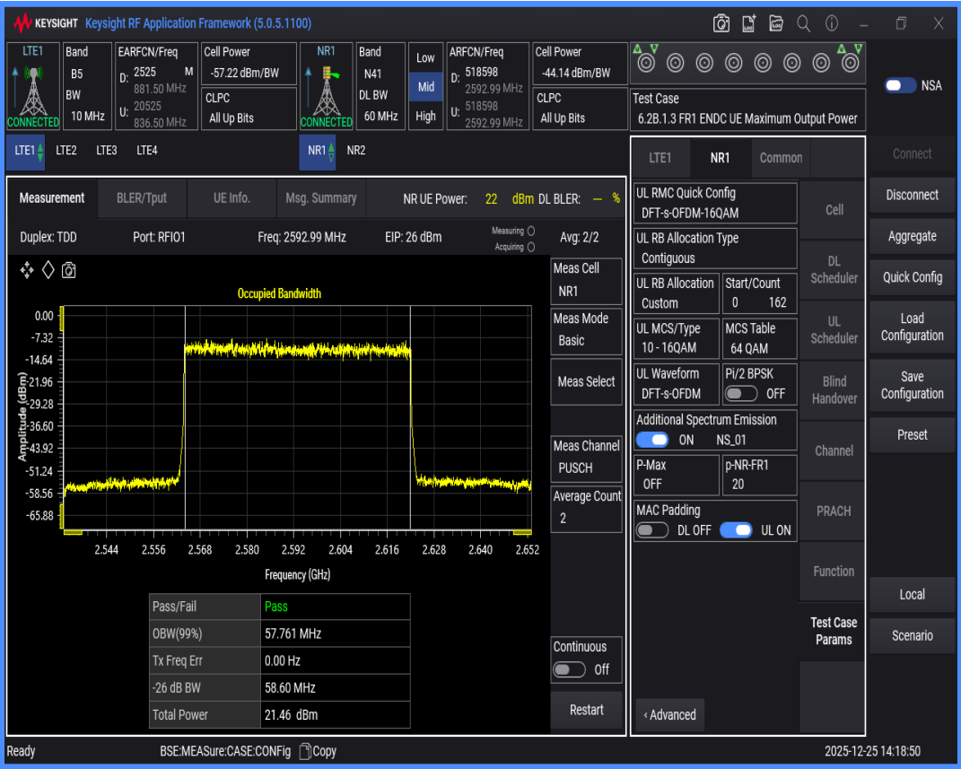
n41 SCS=30kHz DFT_QAM16 BW=80MHz Channel=518598 RB=216@0
