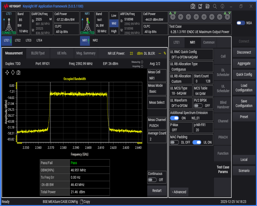
n41 SCS=30kHz DFT_QAM64 BW=60MHz Channel=518598 RB=162@0
