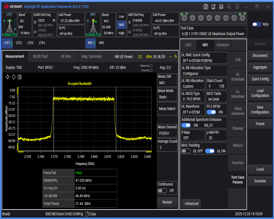
n41 SCS=30kHz DFT_BPSK BW=60MHz Channel=518598 RB=162@0
