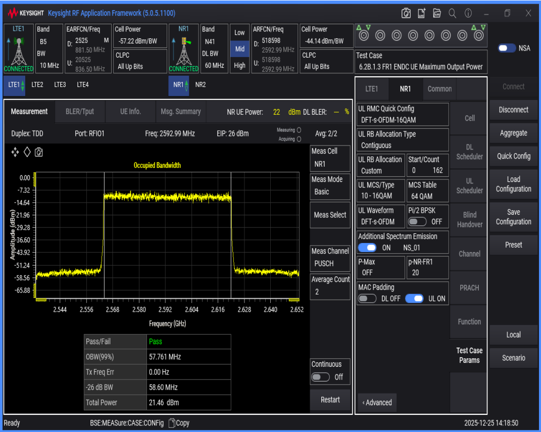
n41 SCS=30kHz DFT_QAM16 BW=80MHz Channel=518598 RB=216@0
