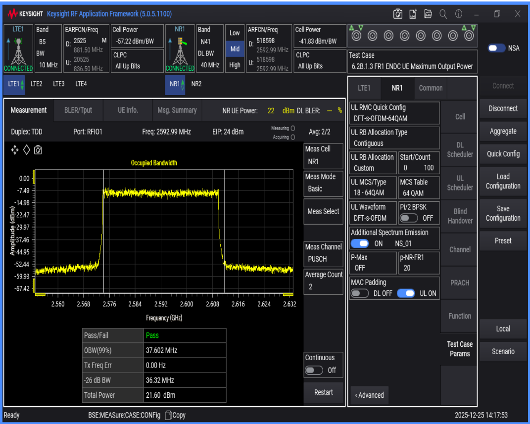
n41 SCS=30kHz DFT_QAM64 BW=50MHz Channel=518598 RB=128@0
