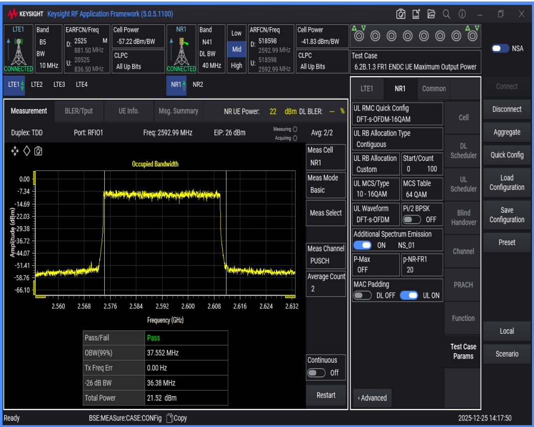
n41 SCS=30kHz DFT_QAM16 BW=50MHz Channel=518598 RB=128@0
