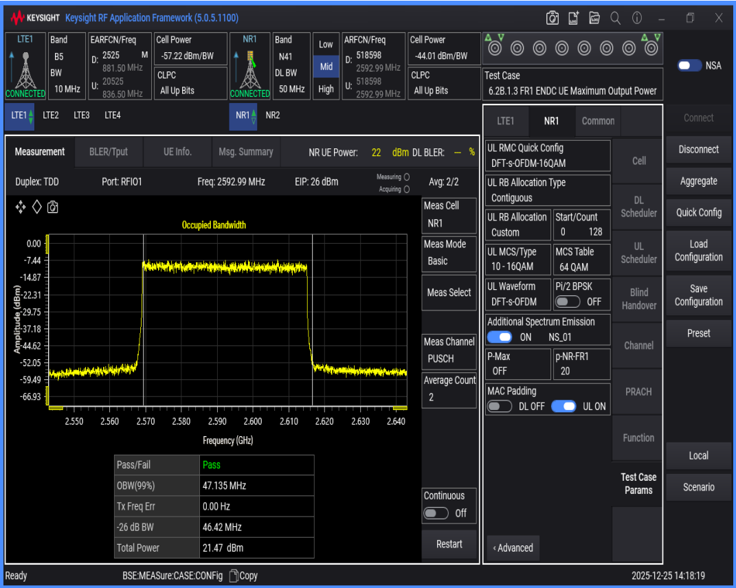
n41 SCS=30kHz DFT_QAM16 BW=60MHz Channel=518598 RB=162@0
