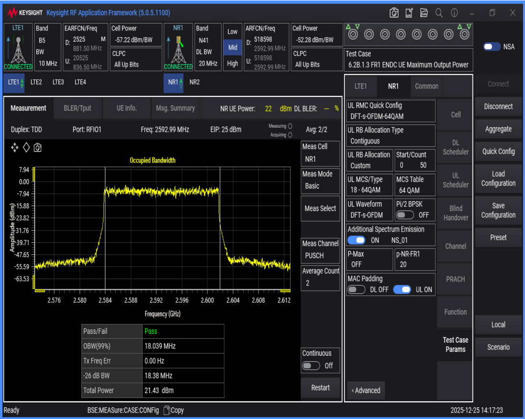
n41 SCS=30kHz DFT_QAM64 BW=40MHz Channel=518598 RB=100@0
