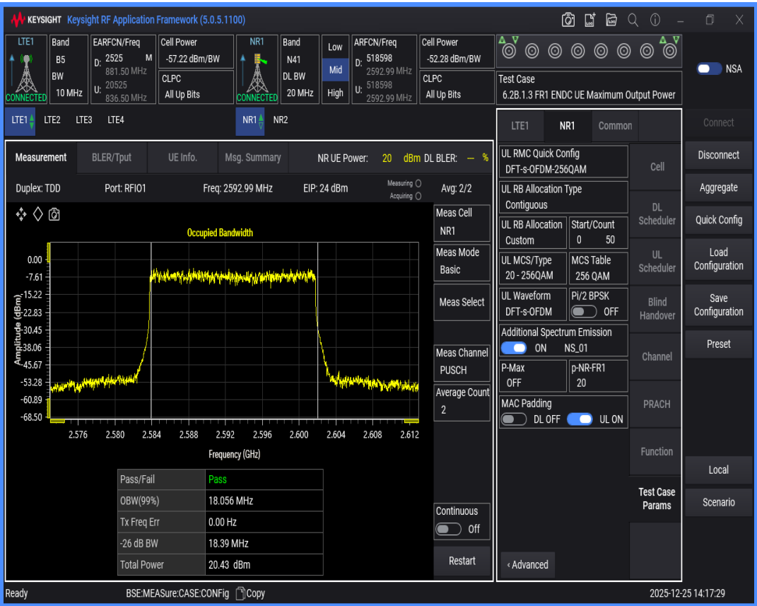
n41 SCS=30kHz DFT_QAM256 BW=40MHz Channel=518598 RB=100@0
