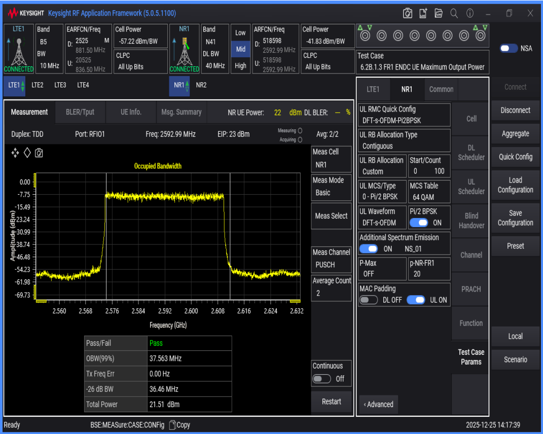
n41 SCS=30kHz DFT_BPSK BW=50MHz Channel=518598 RB=128@0
