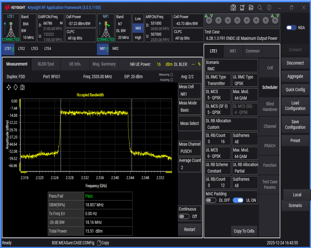
n7 SCS=15kHz DFT_QAM256 BW=5MHz Channel=507000 RB=25@0
