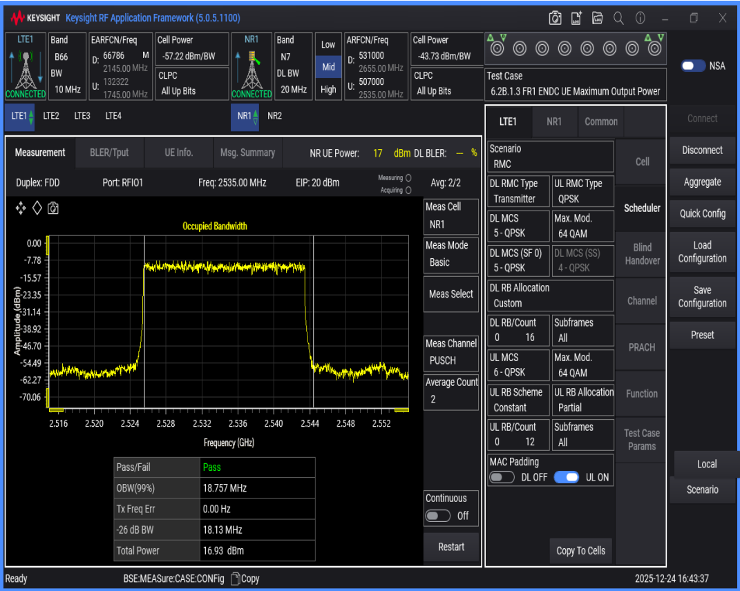
n7 SCS=15kHz DFT_BPSK BW=5MHz Channel=507000 RB=25@0
