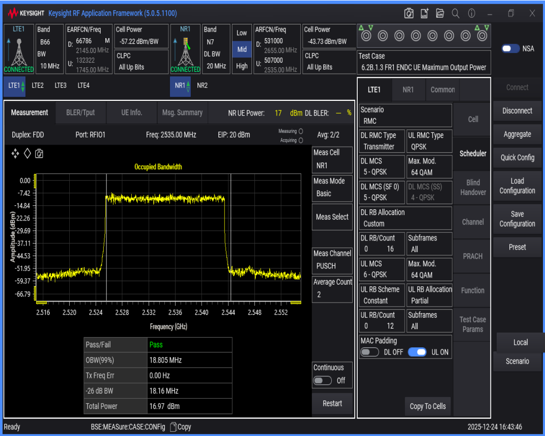
n7 SCS=15kHz DFT_QAM16 BW=5MHz Channel=507000 RB=25@0
