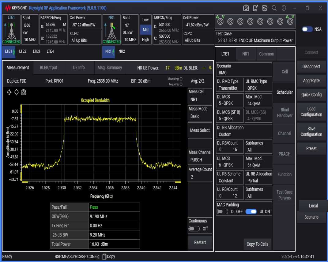
n7 SCS=15kHz DFT_BPSK BW=15MHz Channel=507000 RB=75@0
