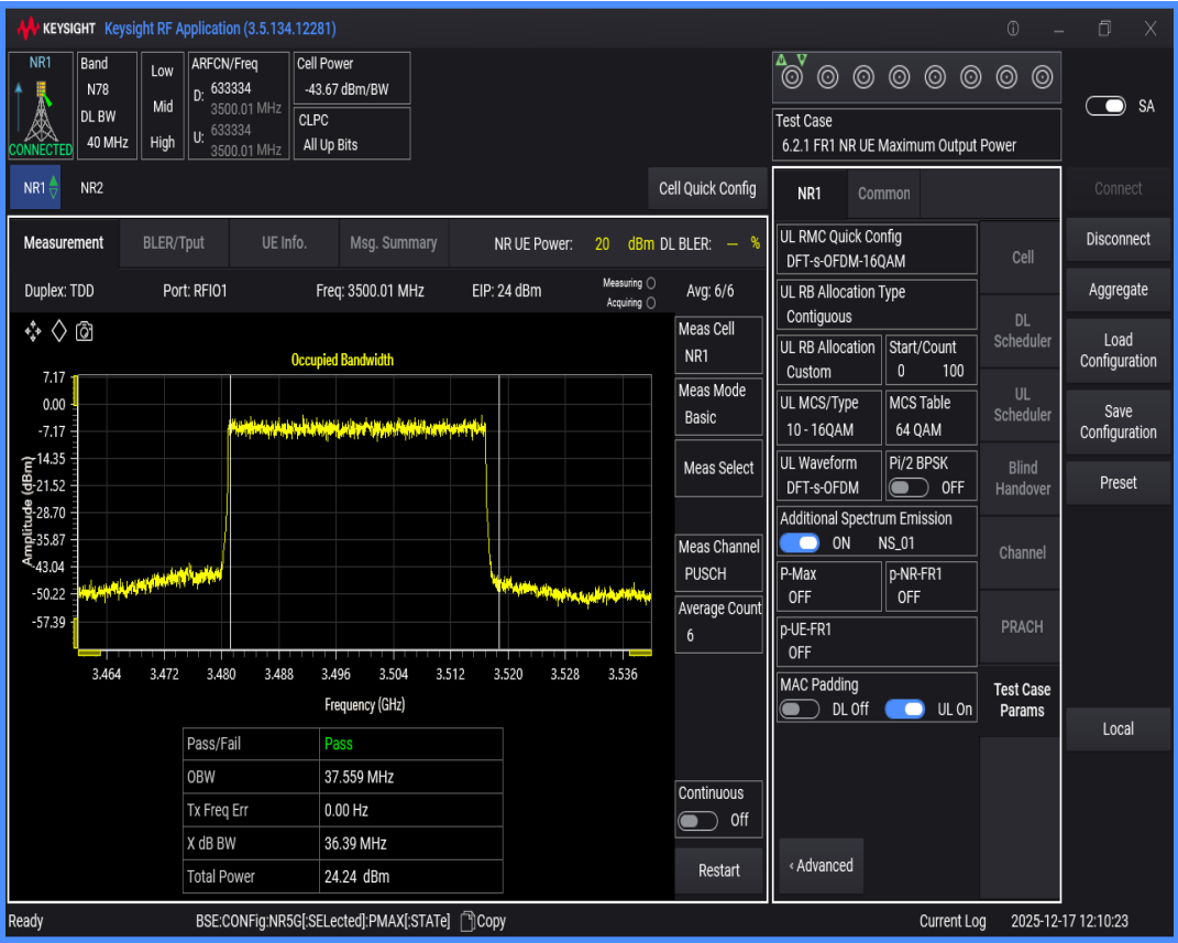
n78(3450-3550) SCS=30kHz DFT_QAM16 BW=50MHz Channel=633334 RB=128@0
