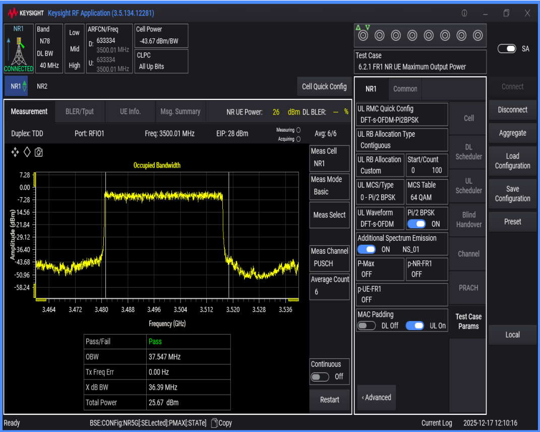
n78(3450-3550) SCS=30kHz DFT_BPSK BW=50MHz Channel=633334 RB=128@0
