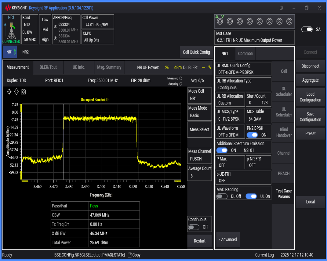
n78(3450-3550) SCS=30kHz DFT_BPSK BW=60MHz Channel=633334 RB=162@0
