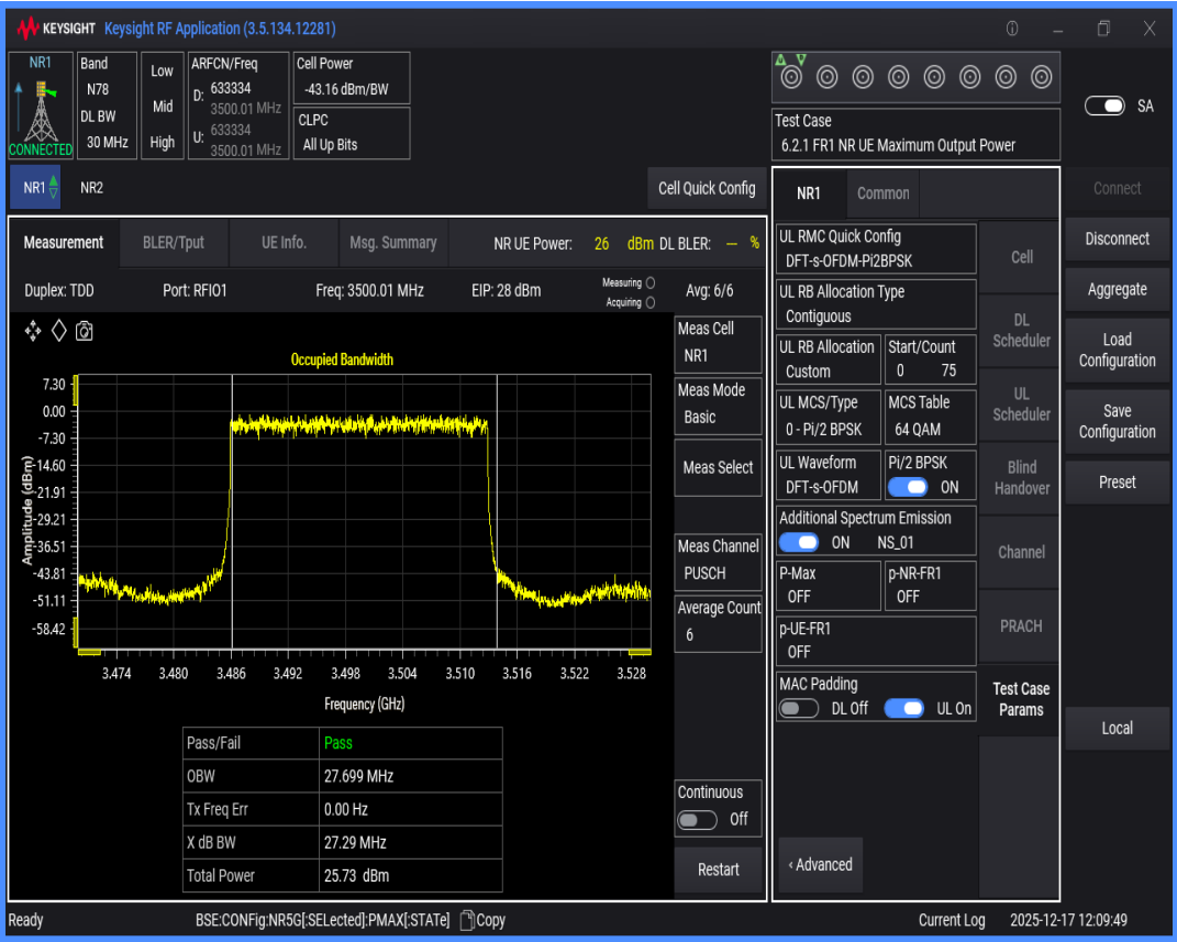
n78(3450-3550) SCS=30kHz DFT_BPSK BW=40MHz Channel=633334 RB=100@0
