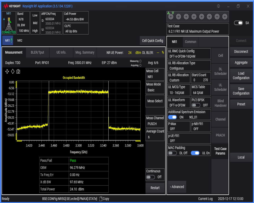
n78(3450-3550) SCS=30kHz DFT_QAM16 BW=10MHz Channel=633334 RB=24@0
