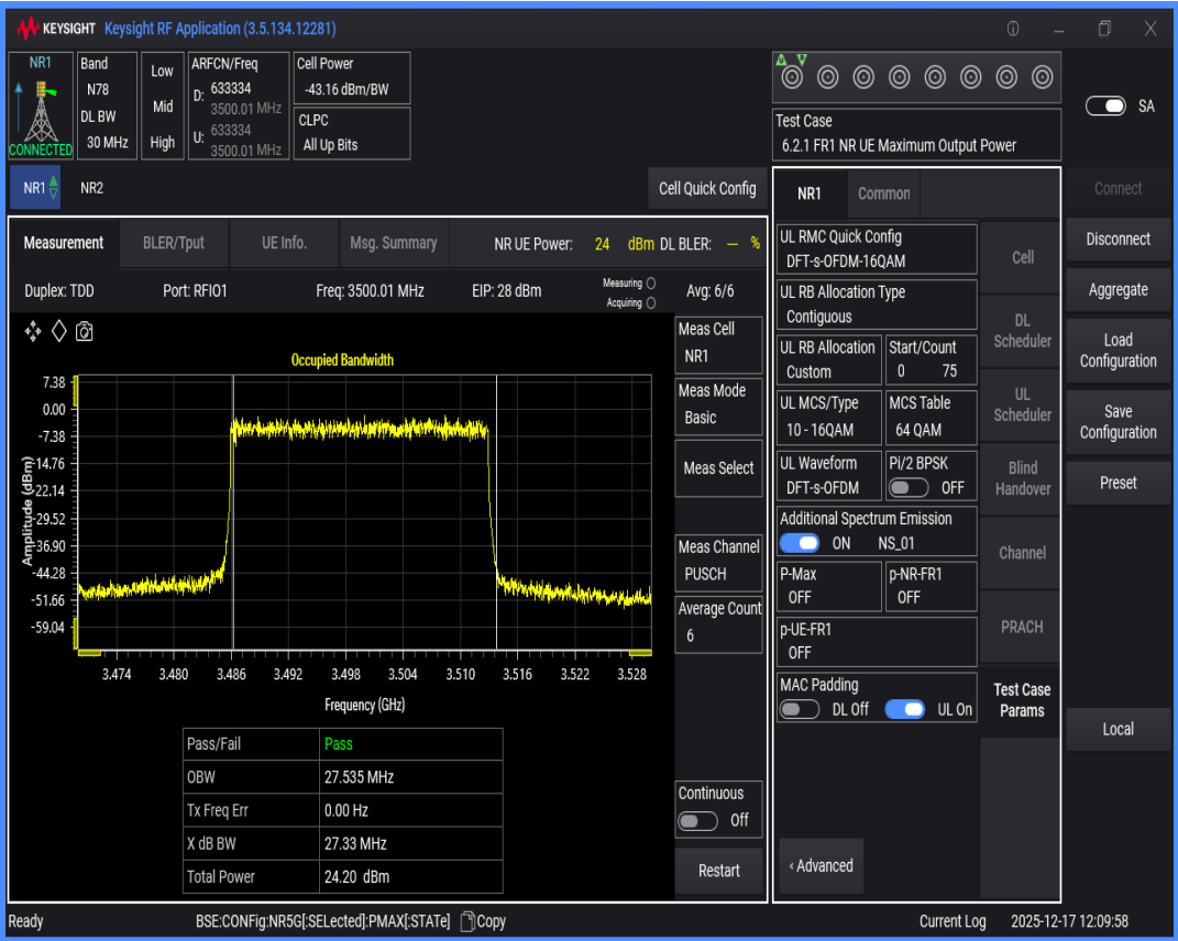
n78(3450-3550) SCS=30kHz DFT_QAM16 BW=40MHz Channel=633334 RB=100@0
