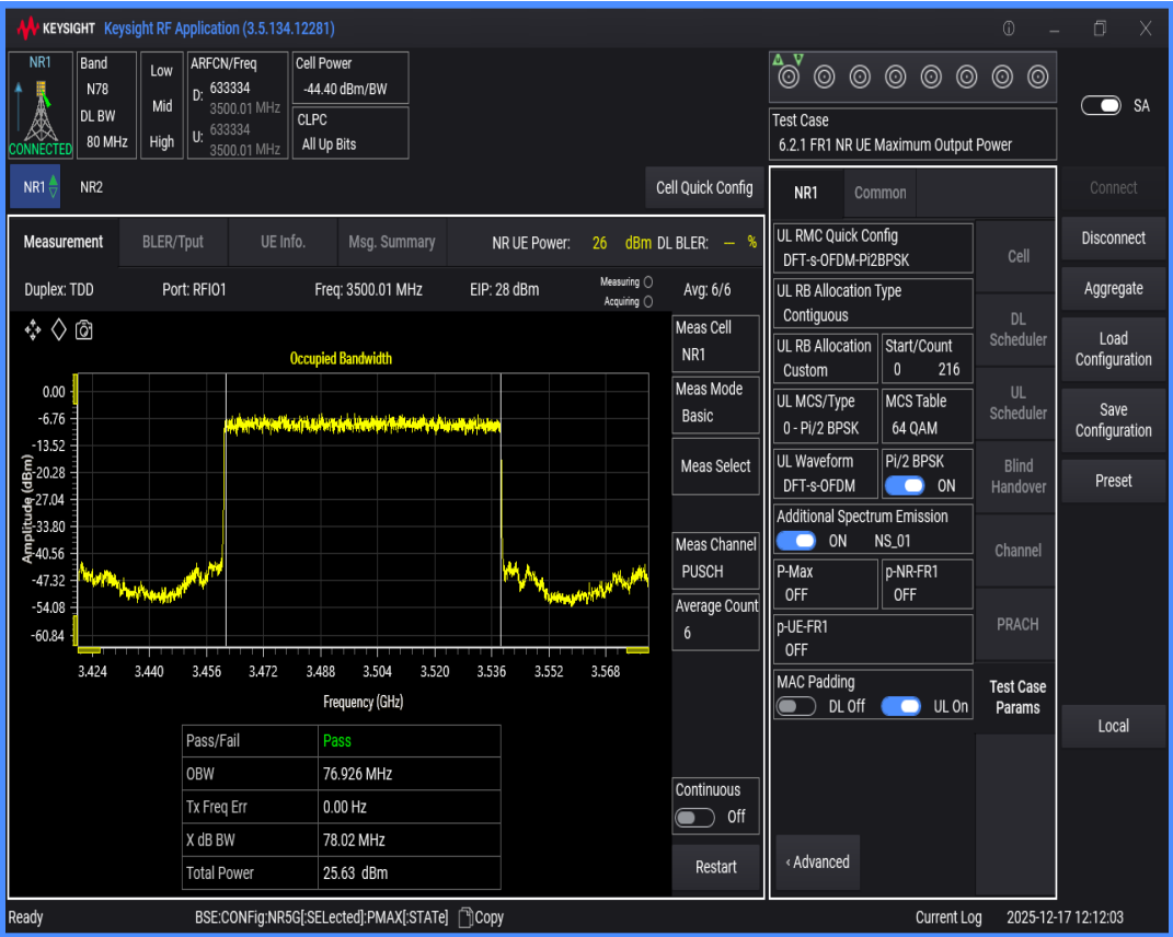
n78(3450-3550) SCS=30kHz DFT_BPSK BW=90MHz Channel=633334 RB=240@0
