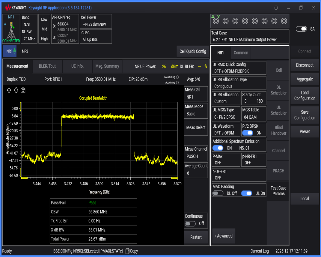
n78(3450-3550) SCS=30kHz DFT_BPSK BW=80MHz Channel=633334 RB=216@0
