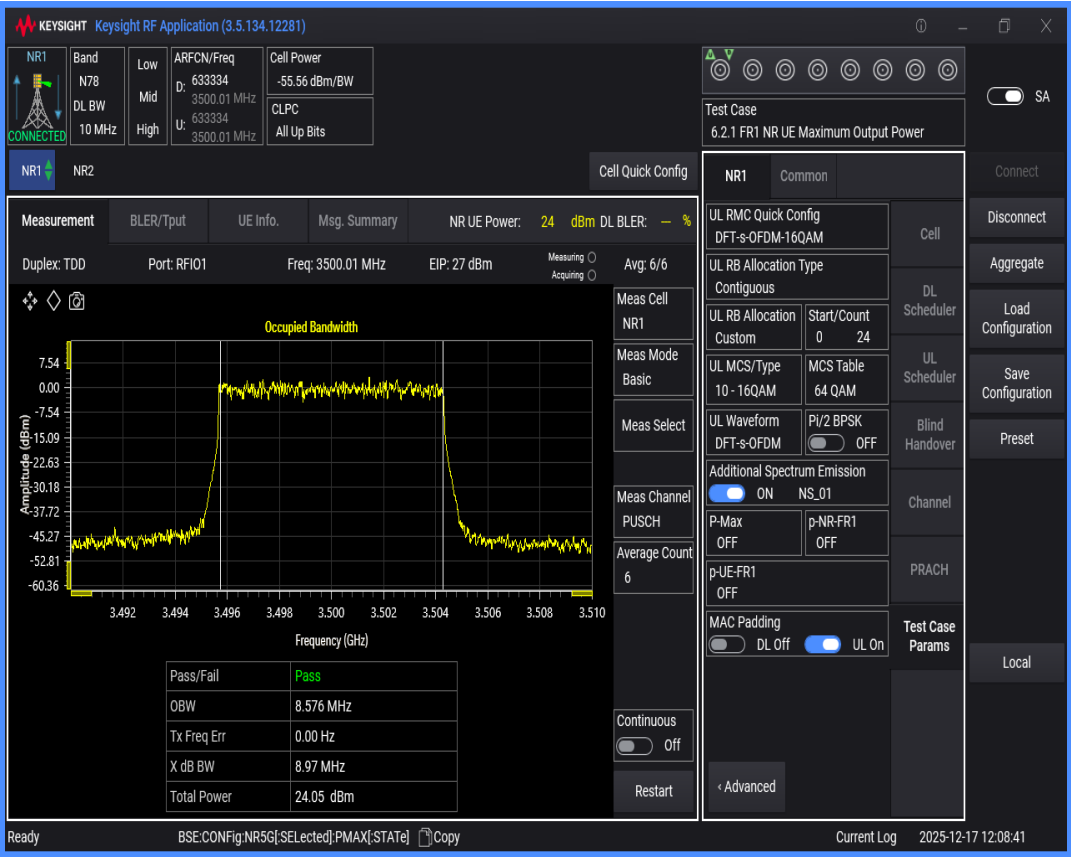
n78(3450-3550) SCS=30kHz DFT_QAM16 BW=15MHz Channel=633334 RB=36@0
