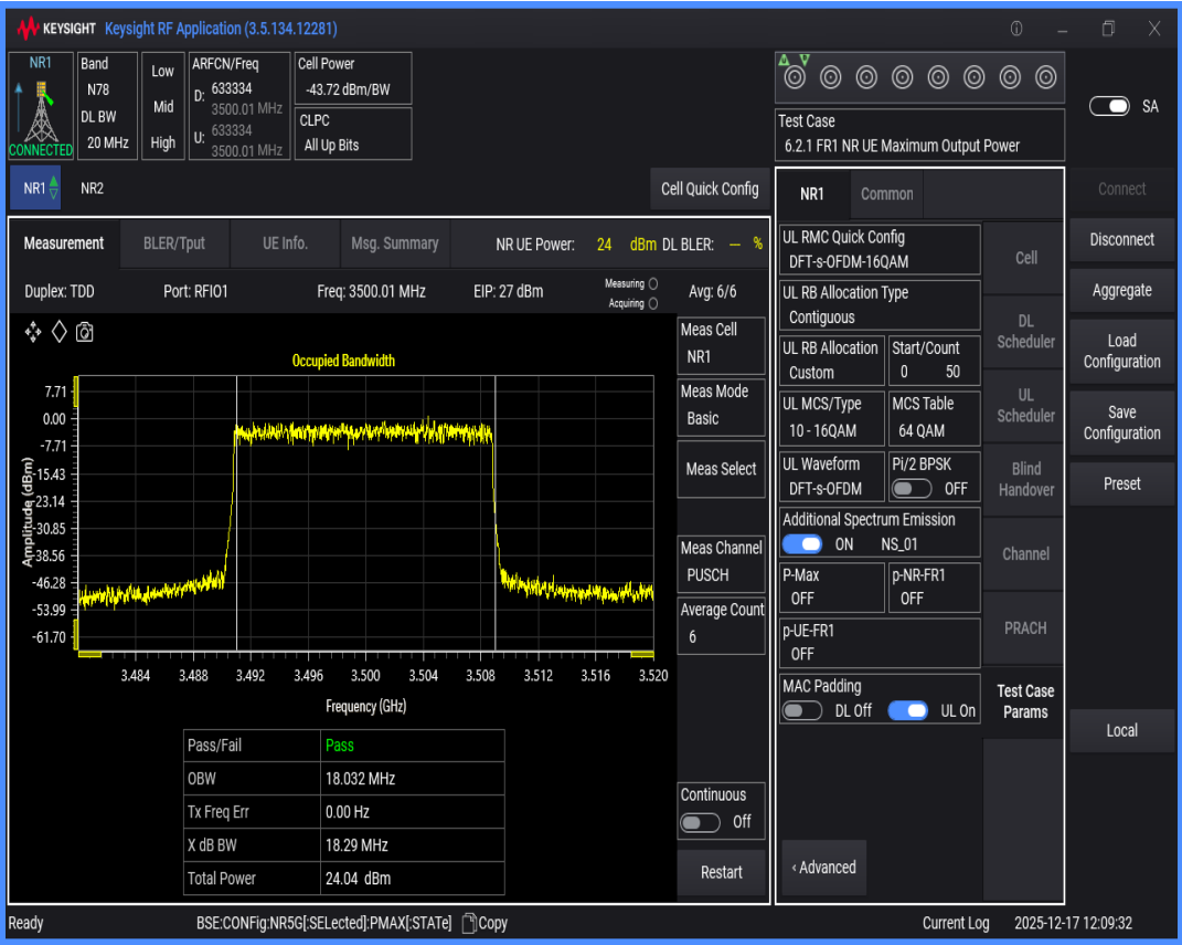
n78(3450-3550) SCS=30kHz DFT_QAM16 BW=30MHz Channel=633334 RB=75@0
