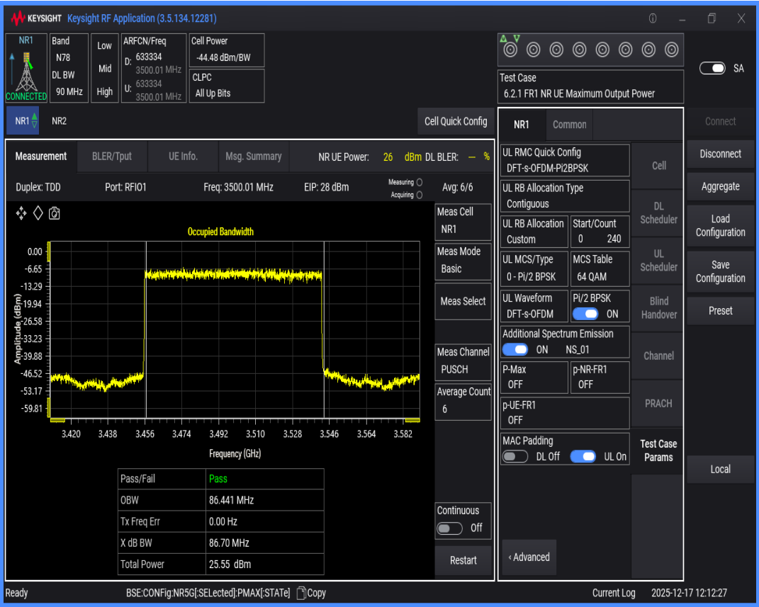
n78(3450-3550) SCS=30kHz DFT_QAM16 BW=100MHz Channel=633334 RB=270@0
