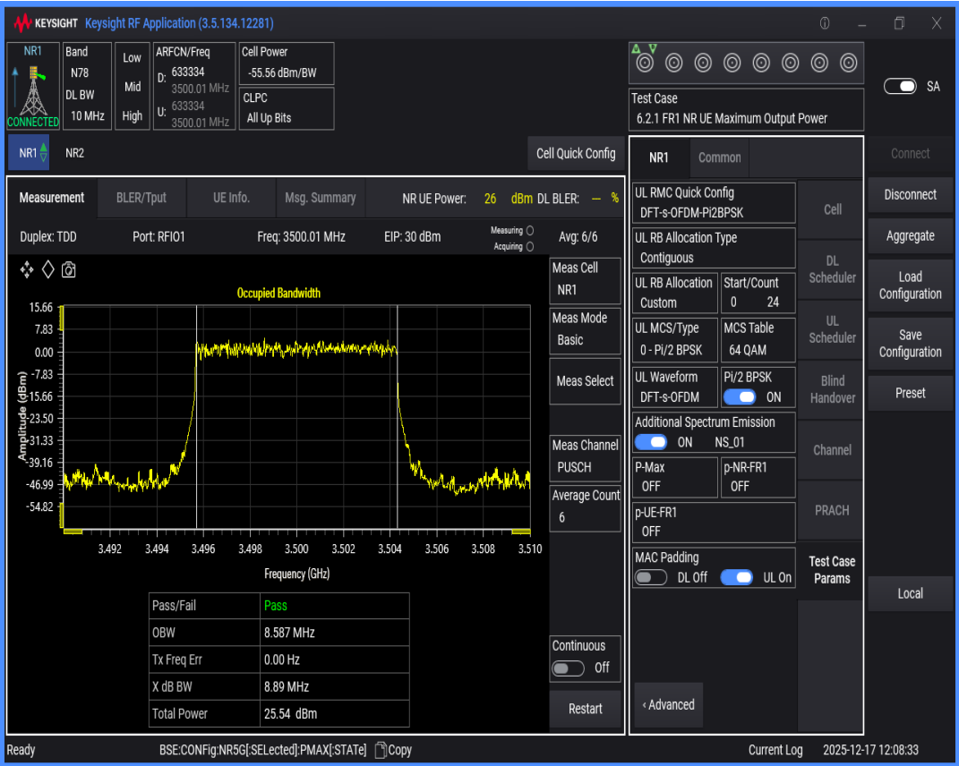
n78(3450-3550) SCS=30kHz DFT_BPSK BW=15MHz Channel=633334 RB=36@0
