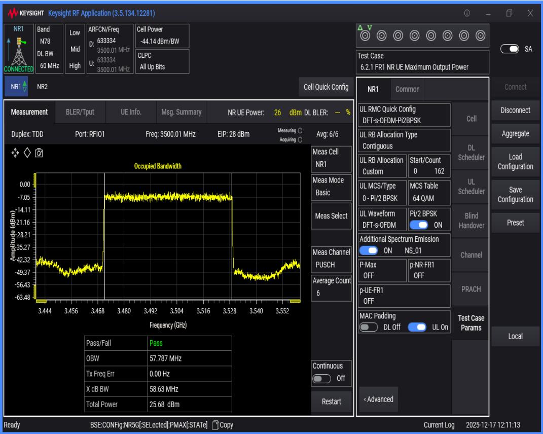
n78(3450-3550) SCS=30kHz DFT_BPSK BW=70MHz Channel=633334 RB=180@0
