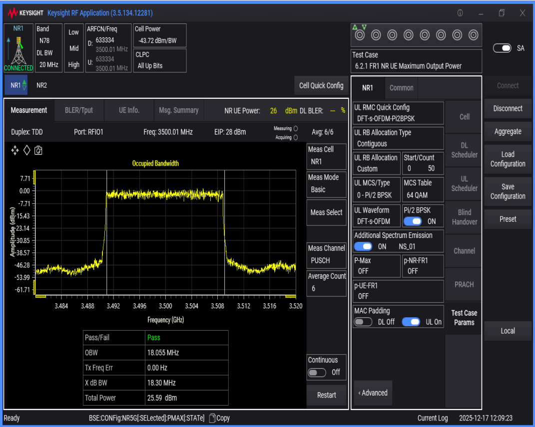
n78(3450-3550) SCS=30kHz DFT_BPSK BW=30MHz Channel=633334 RB=75@0
