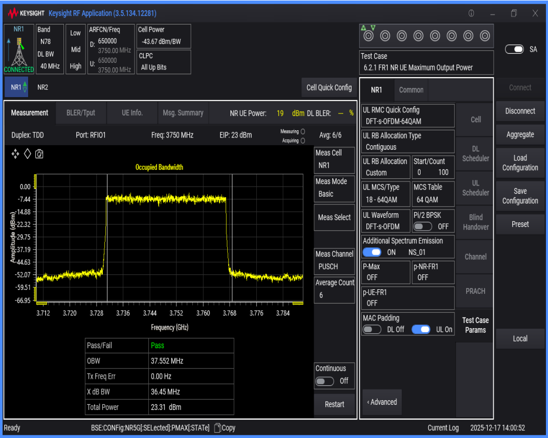
n78(3700-3800) SCS=30kHz DFT_QAM64 BW=50MHz Channel=650000 RB=128@0
