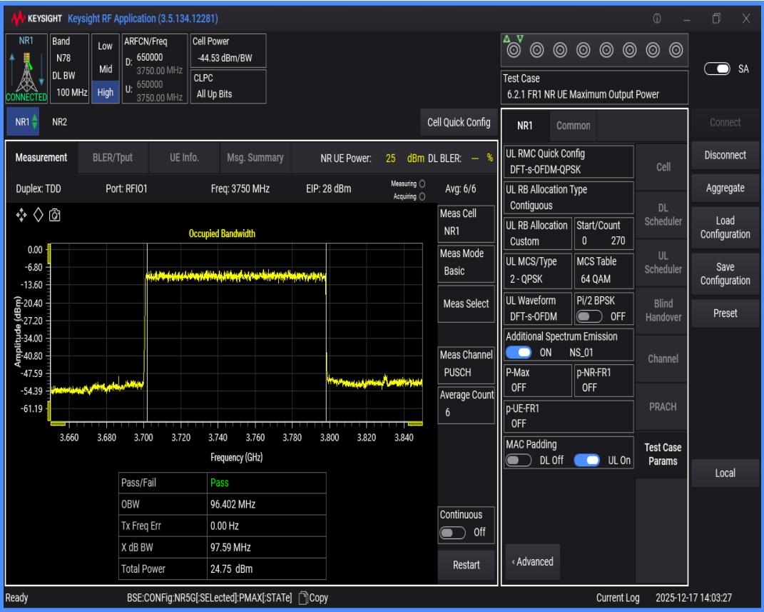
n78(3700-3800) SCS=30kHz DFT_QPSK BW=10MHz Channel=650000 RB=24@0
