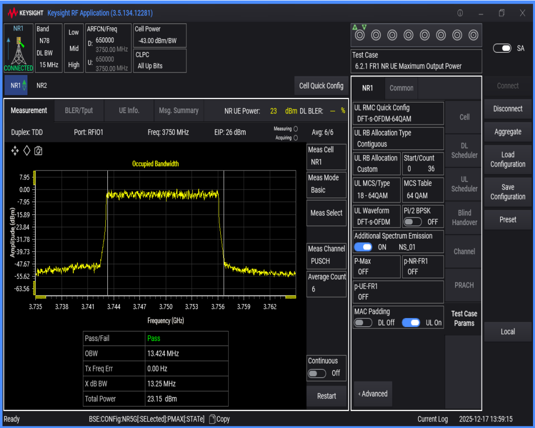
n78(3700-3800) SCS=30kHz DFT_QAM64 BW=20MHz Channel=650000 RB=50@0
