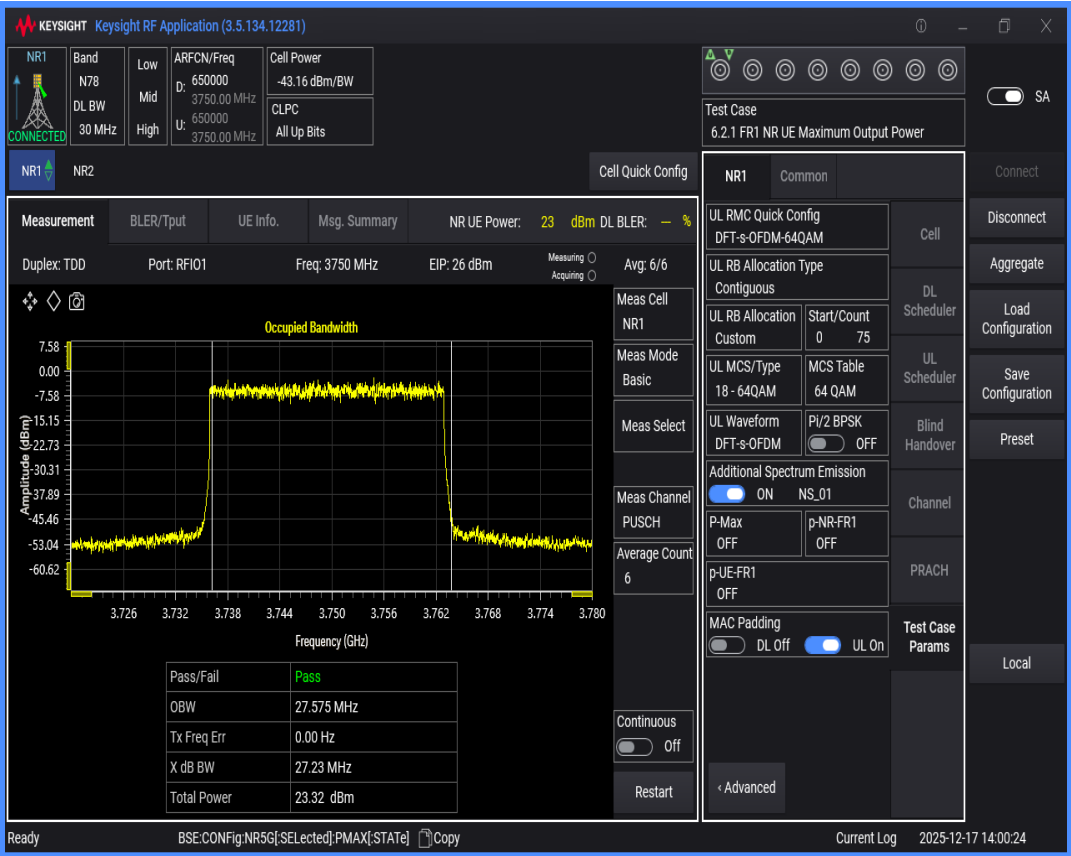
n78(3700-3800) SCS=30kHz DFT_QAM64 BW=40MHz Channel=650000 RB=100@0
