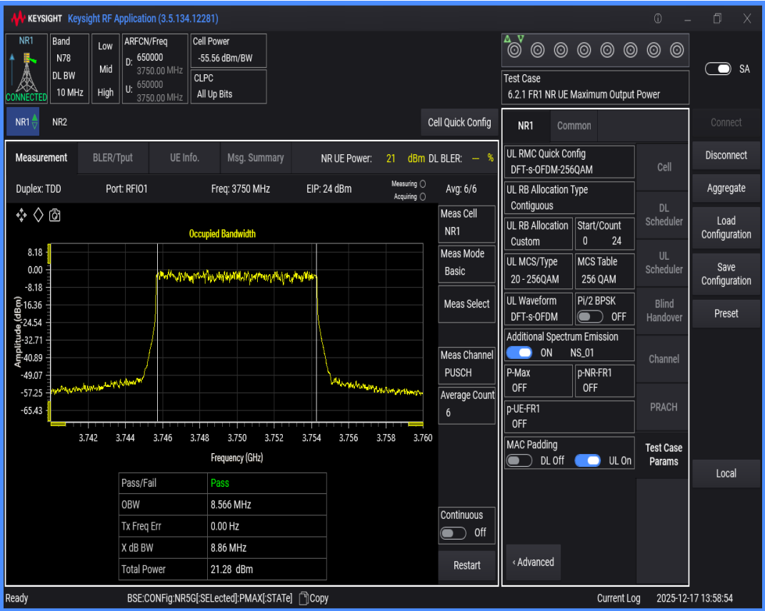
n78(3700-3800) SCS=30kHz DFT_QAM256 BW=15MHz Channel=650000 RB=36@0
