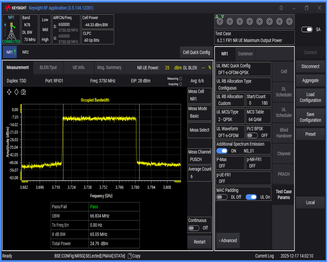
n78(3700-3800) SCS=30kHz DFT_QPSK BW=80MHz Channel=650000 RB=216@0
