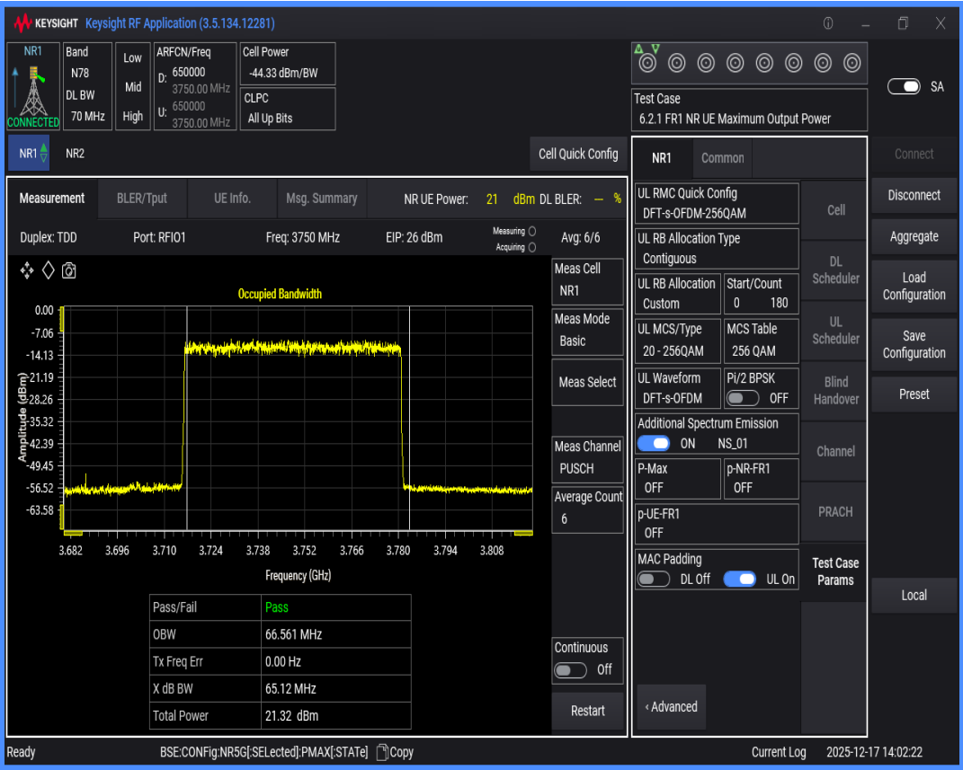
n78(3700-3800) SCS=30kHz DFT_QAM256 BW=80MHz Channel=650000 RB=216@0
