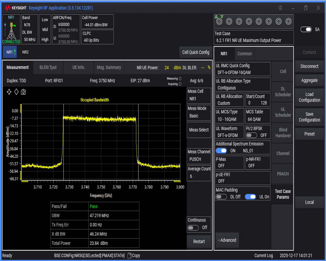
n78(3700-3800) SCS=30kHz DFT_QAM16 BW=60MHz Channel=650000 RB=162@0
