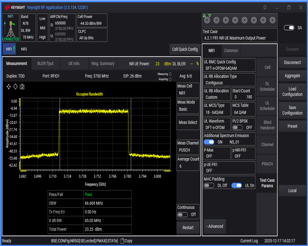
n78(3700-3800) SCS=30kHz DFT_QAM64 BW=80MHz Channel=650000 RB=216@0
