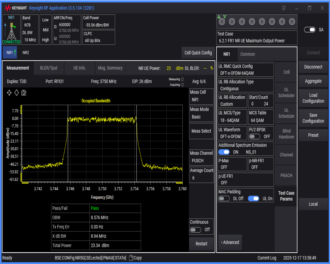
n78(3700-3800) SCS=30kHz DFT_QAM64 BW=15MHz Channel=650000 RB=36@0
