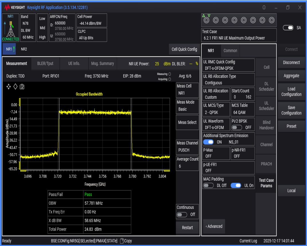
n78(3700-3800) SCS=30kHz DFT_QPSK BW=70MHz Channel=650000 RB=180@0
