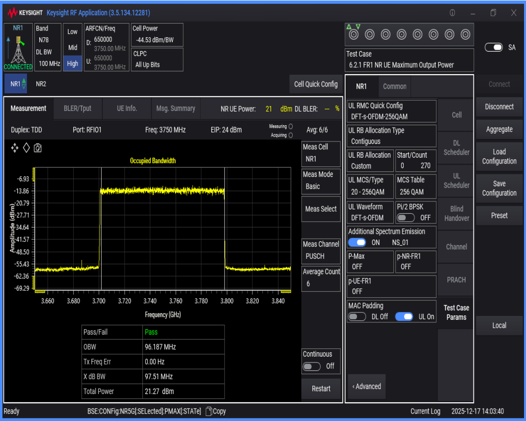
n78(3700-3800) SCS=30kHz DFT_QAM256 BW=10MHz Channel=650000 RB=24@0
