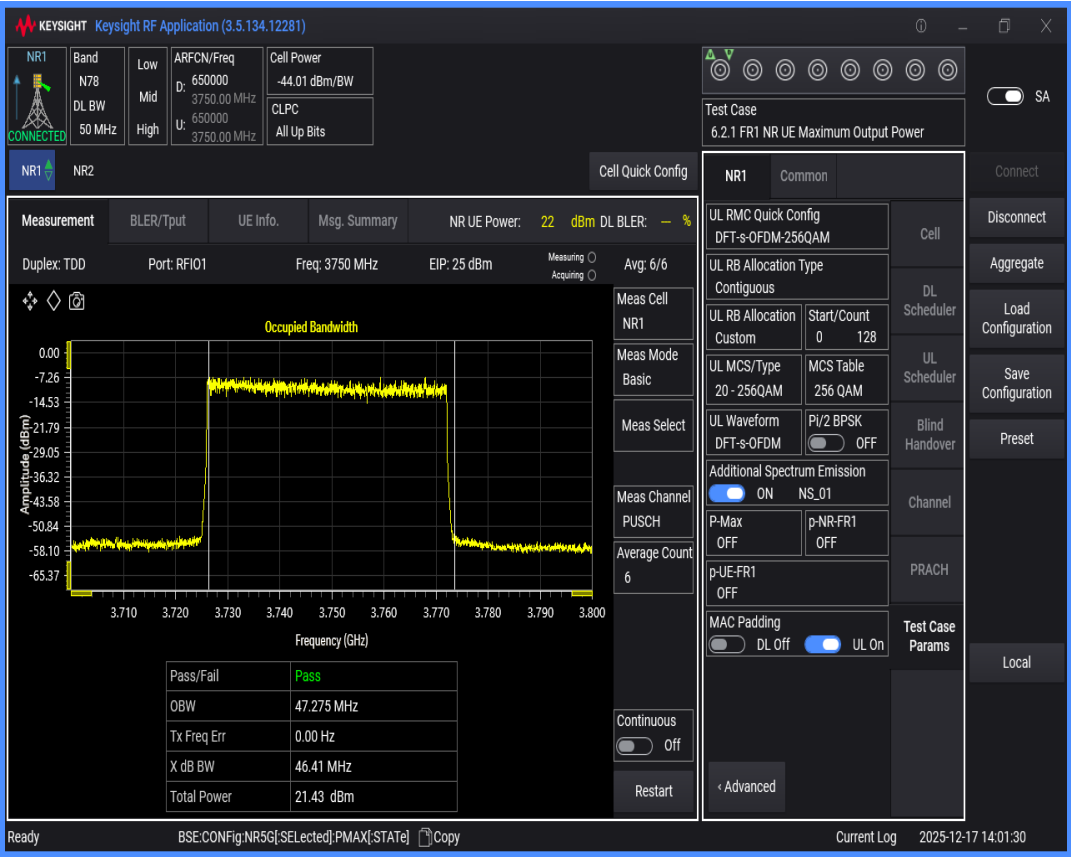
n78(3700-3800) SCS=30kHz DFT_QAM256 BW=60MHz Channel=650000 RB=162@0
