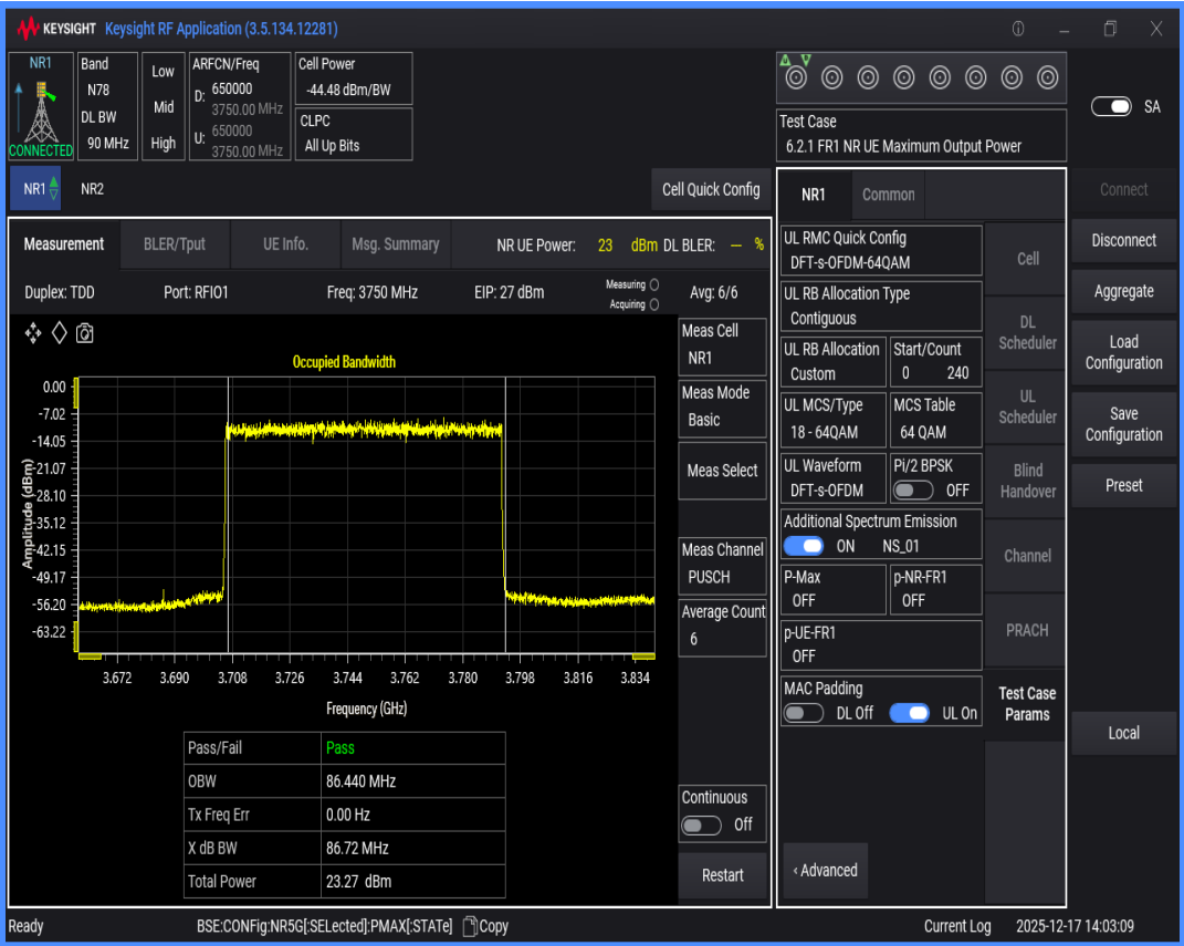
n78(3700-3800) SCS=30kHz DFT_QPSK BW=100MHz Channel=650000 RB=270@0
