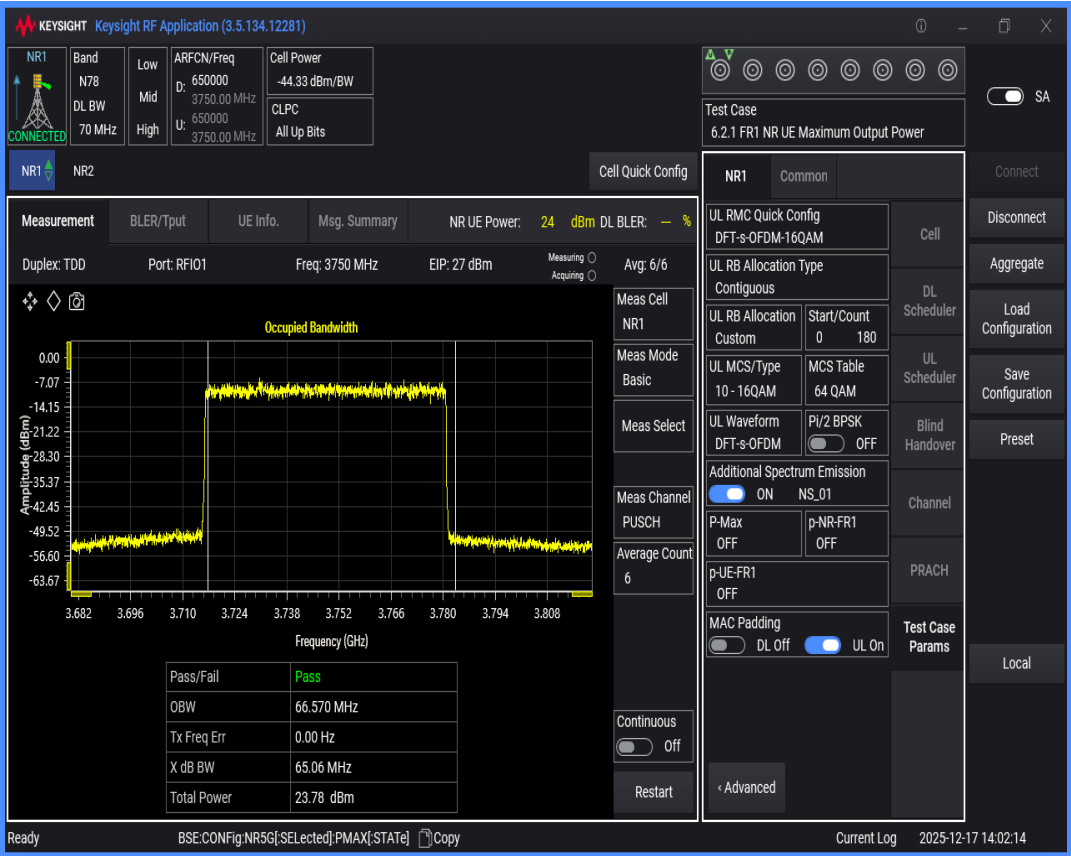
n78(3700-3800) SCS=30kHz DFT_QAM16 BW=80MHz Channel=650000 RB=216@0
