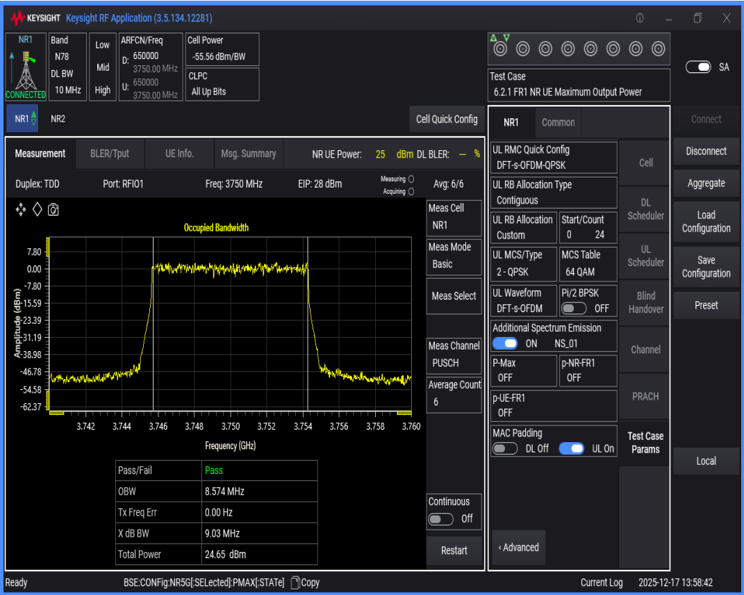
n78(3700-3800) SCS=30kHz DFT_QPSK BW=15MHz Channel=650000 RB=36@0
