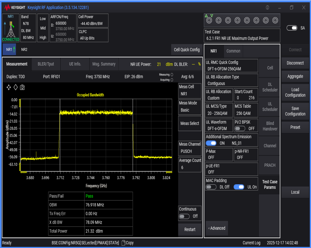
n78(3700-3800) SCS=30kHz DFT_QAM256 BW=90MHz Channel=650000 RB=240@0
