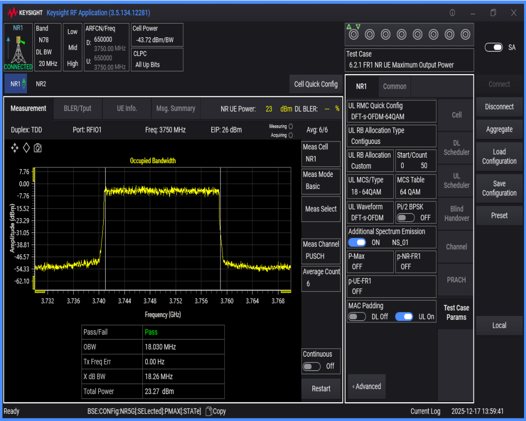
n78(3700-3800) SCS=30kHz DFT_QAM64 BW=30MHz Channel=650000 RB=75@0
