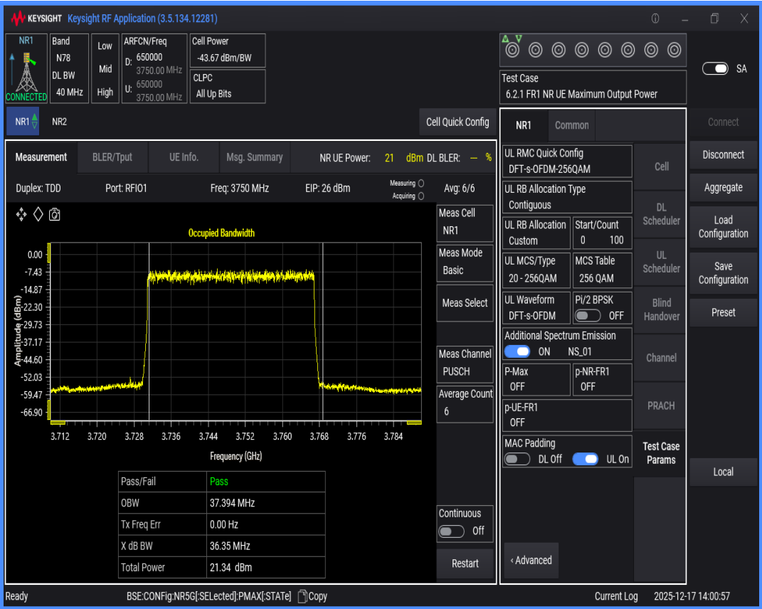
n78(3700-3800) SCS=30kHz DFT_QAM256 BW=50MHz Channel=650000 RB=128@0
