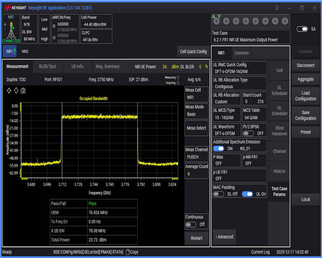
n78(3700-3800) SCS=30kHz DFT_QAM16 BW=90MHz Channel=650000 RB=240@0
