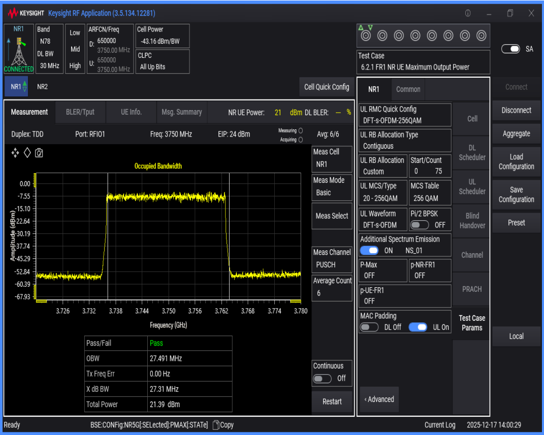
n78(3700-3800) SCS=30kHz DFT_QAM256 BW=40MHz Channel=650000 RB=100@0
