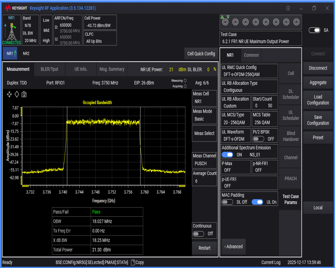
n78(3700-3800) SCS=30kHz DFT_QAM256 BW=30MHz Channel=650000 RB=75@0
