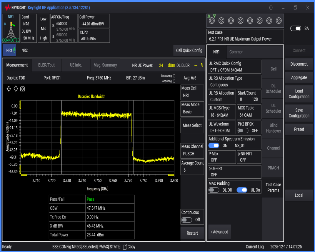
n78(3700-3800) SCS=30kHz DFT_QAM64 BW=60MHz Channel=650000 RB=162@0
