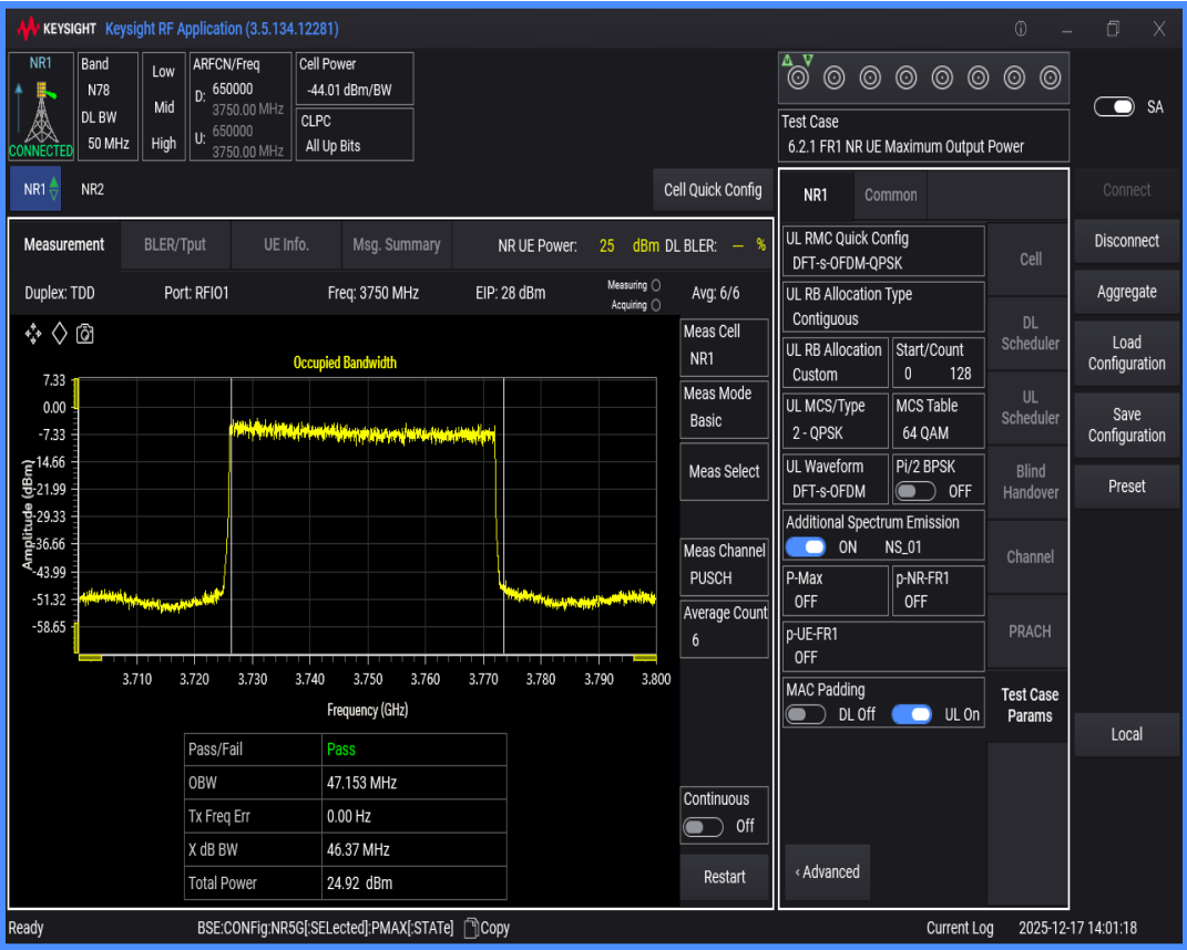
n78(3700-3800) SCS=30kHz DFT_QPSK BW=60MHz Channel=650000 RB=162@0
