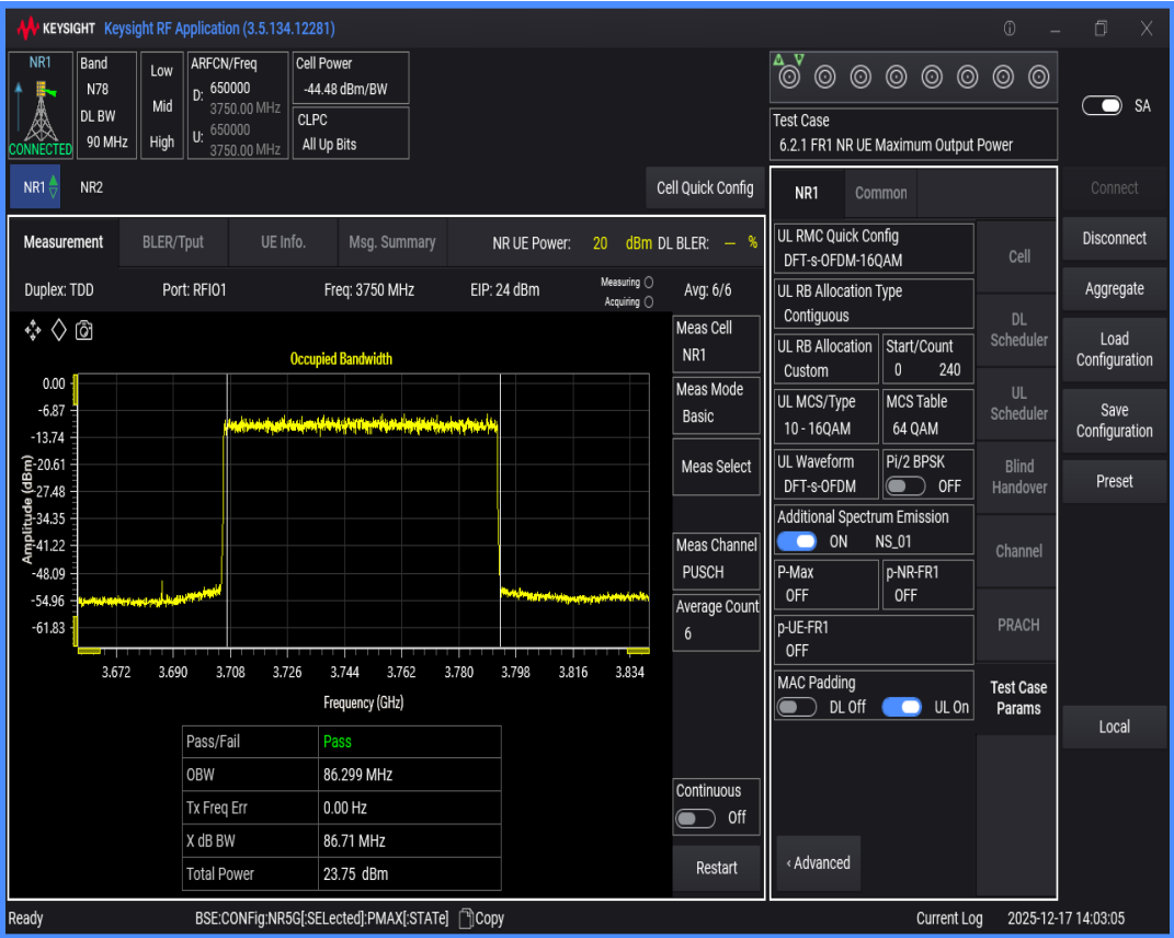
n78(3700-3800) SCS=30kHz DFT_QAM256 BW=100MHz Channel=650000 RB=270@0
