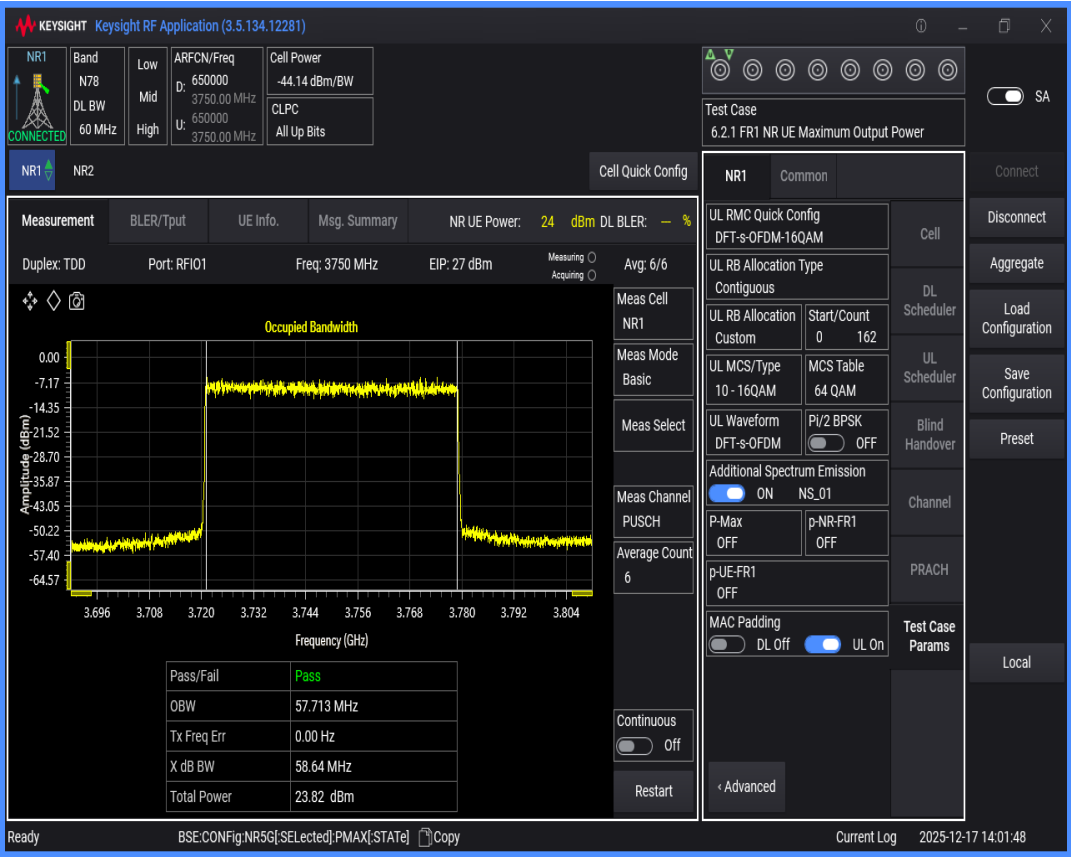
n78(3700-3800) SCS=30kHz DFT_QAM16 BW=70MHz Channel=650000 RB=180@0
