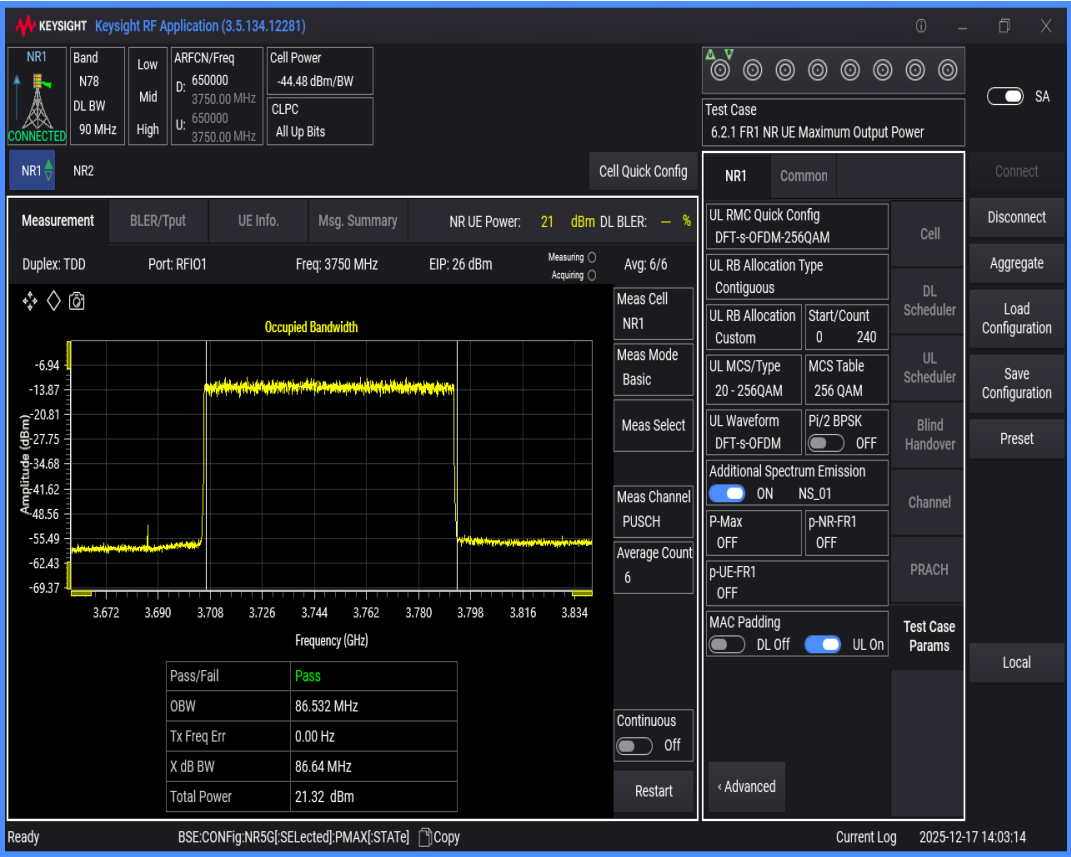
n78(3700-3800) SCS=30kHz DFT_QAM64 BW=100MHz Channel=650000 RB=270@0
