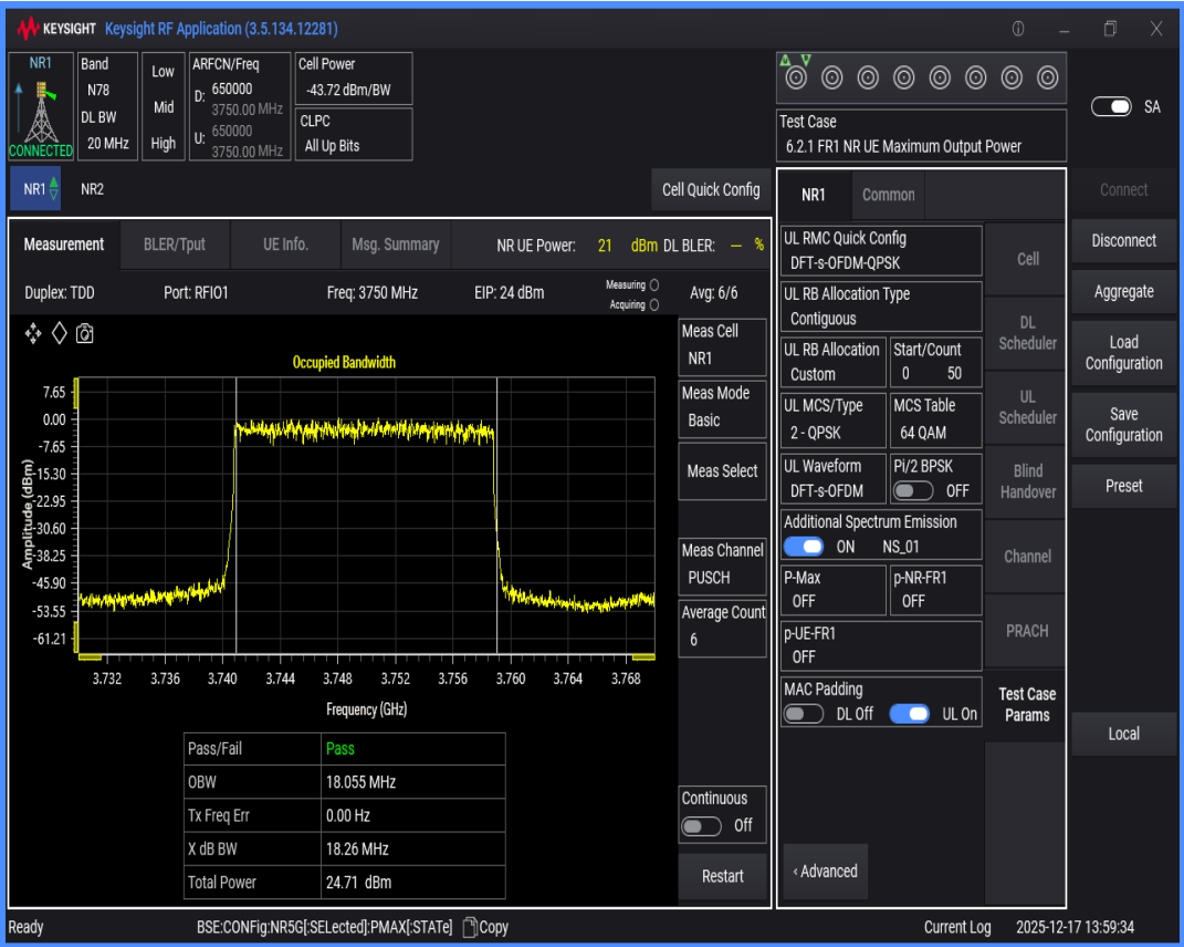
n78(3700-3800) SCS=30kHz DFT_QPSK BW=30MHz Channel=650000 RB=75@0
