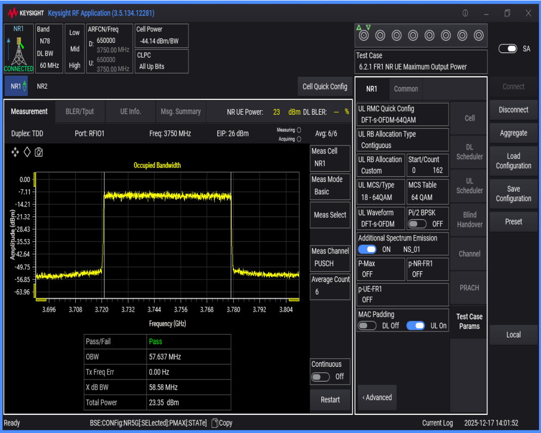
n78(3700-3800) SCS=30kHz DFT_QAM64 BW=70MHz Channel=650000 RB=180@0
