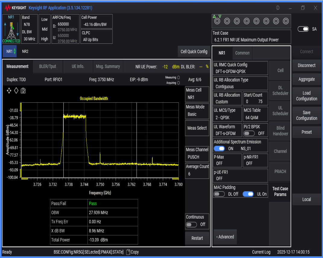
n78(3700-3800) SCS=30kHz DFT_QPSK BW=40MHz Channel=650000 RB=100@0
