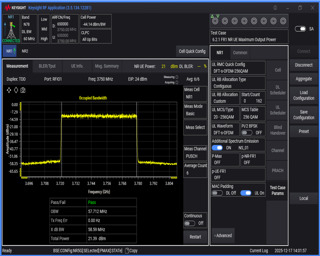
n78(3700-3800) SCS=30kHz DFT_QAM256 BW=70MHz Channel=650000 RB=180@0
