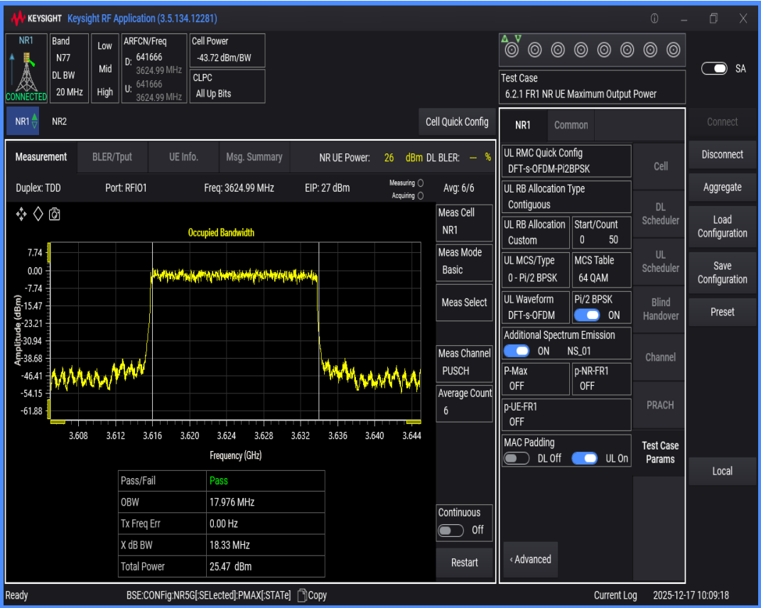
n77(3550-3700) SCS=30kHz DFT_BPSK BW=40MHz Channel=641666 RB=100@0
