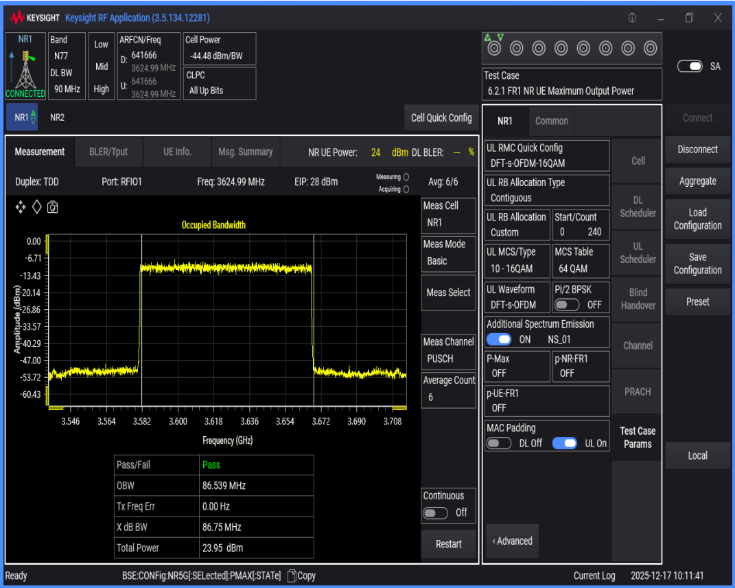
n77(3550-3700) SCS=30kHz DFT_QAM256 BW=100MHz Channel=641666 RB=270@0
