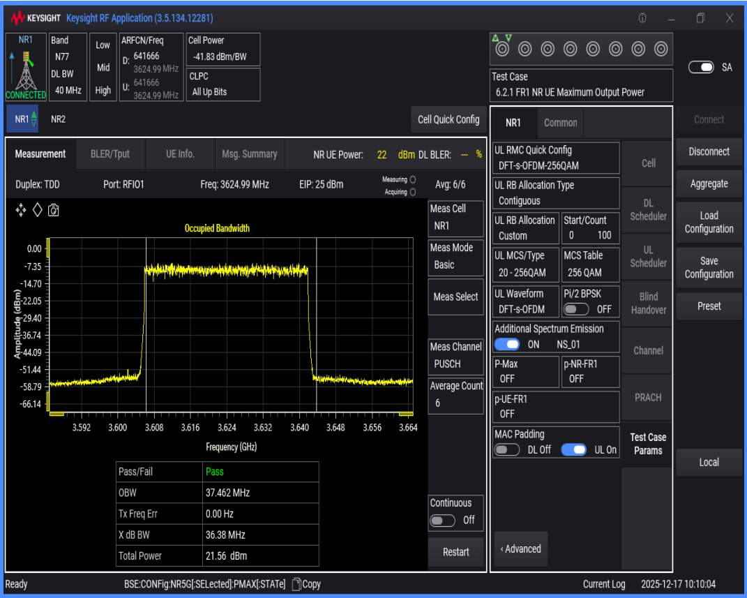
n77(3550-3700) SCS=30kHz DFT_QAM256 BW=50MHz Channel=641666 RB=128@0
