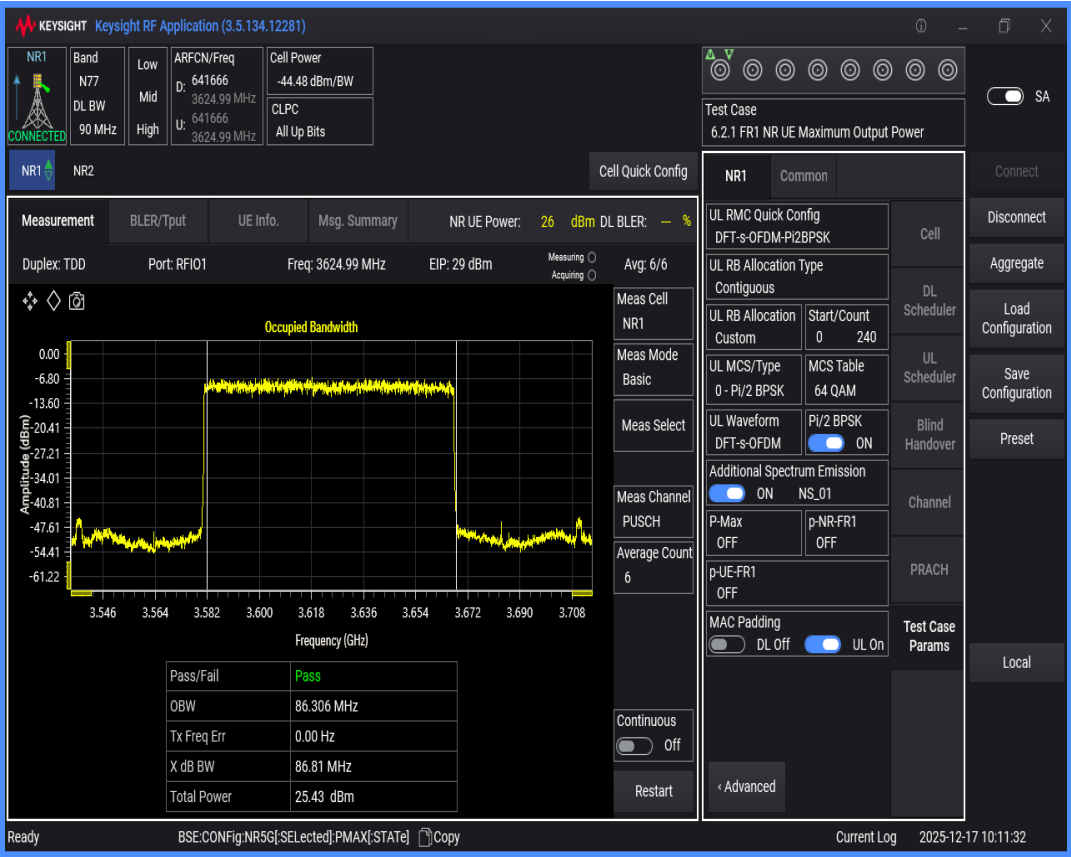
n77(3550-3700) SCS=30kHz DFT_QAM16 BW=100MHz Channel=641666 RB=270@0
