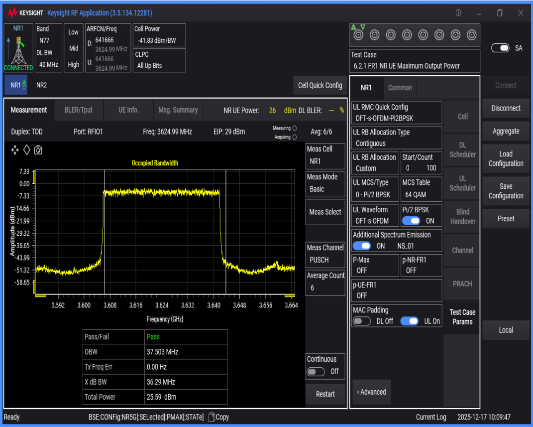
n77(3550-3700) SCS=30kHz DFT_BPSK BW=50MHz Channel=641666 RB=128@0
