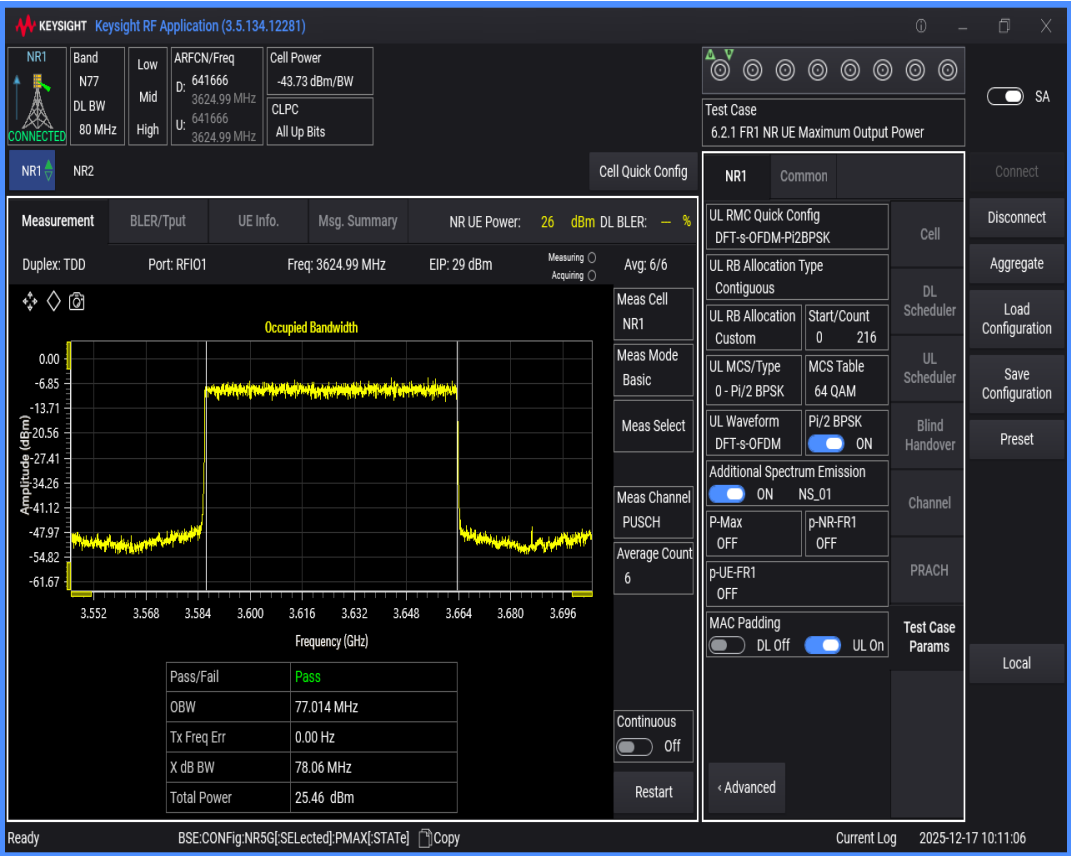
n77(3550-3700) SCS=30kHz DFT_BPSK BW=90MHz Channel=641666 RB=240@0
