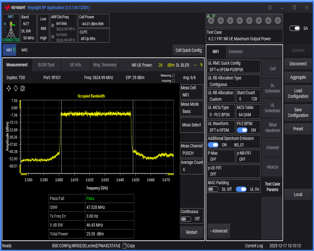
n77(3550-3700) SCS=30kHz DFT_BPSK BW=60MHz Channel=641666 RB=162@0
