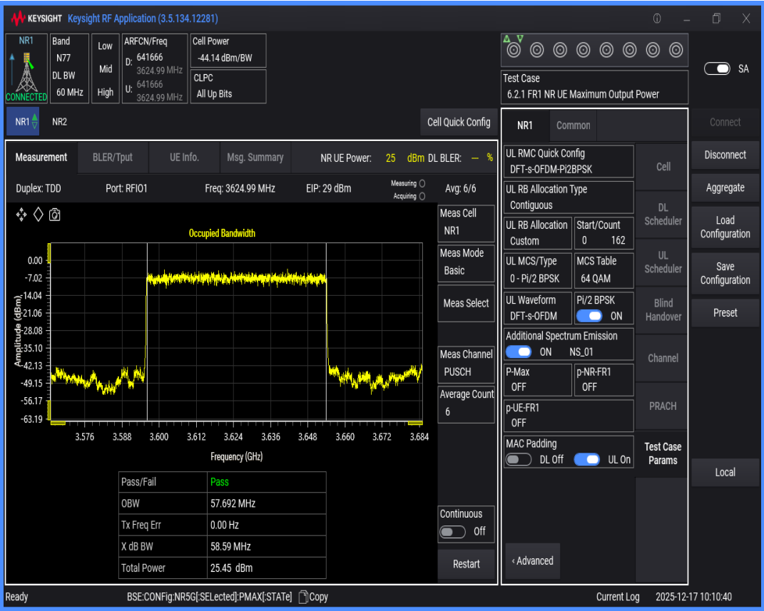
n77(3550-3700) SCS=30kHz DFT_BPSK BW=80MHz Channel=641666 RB=216@0
