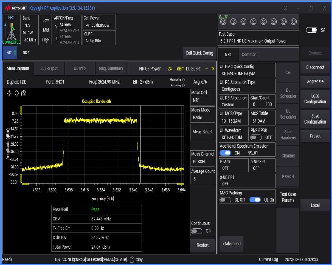
n77(3550-3700) SCS=30kHz DFT_QAM16 BW=50MHz Channel=641666 RB=128@0
