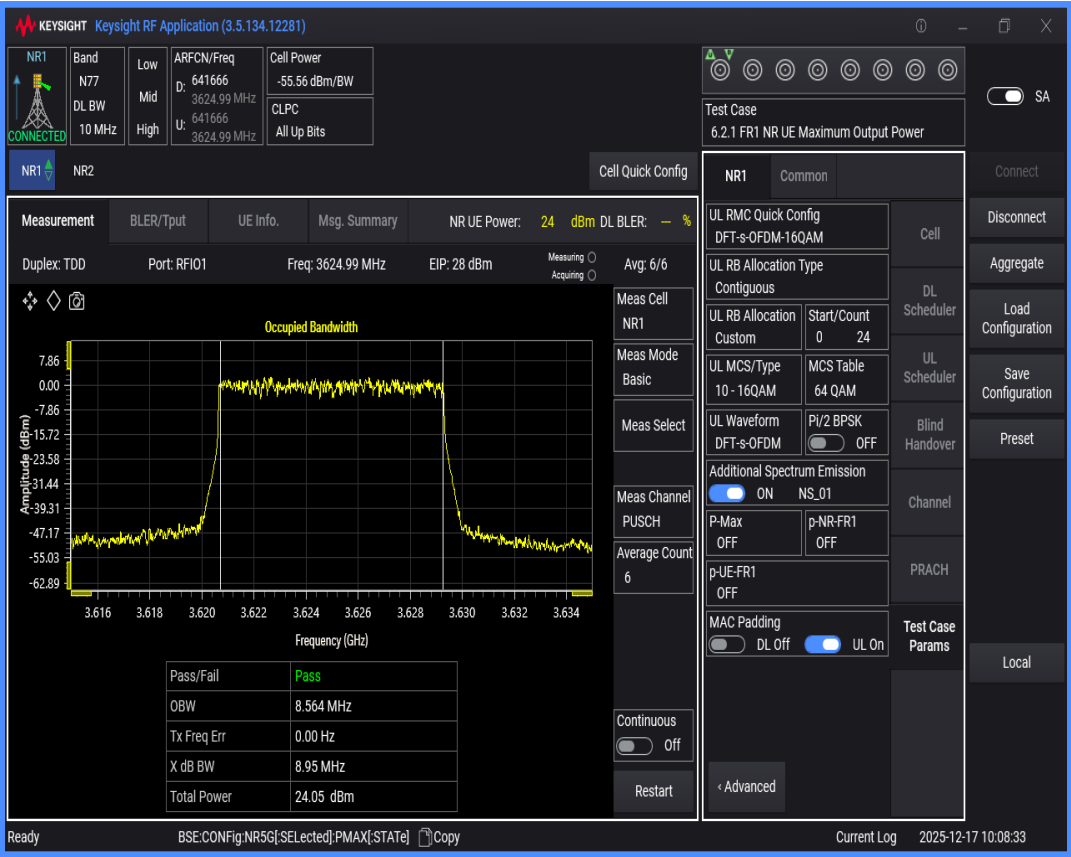
n77(3550-3700) SCS=30kHz DFT_QAM16 BW=15MHz Channel=641666 RB=36@0
