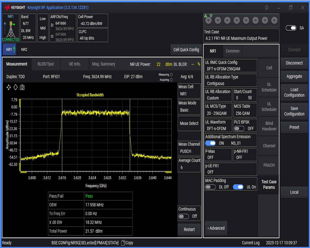
n77(3550-3700) SCS=30kHz DFT_QAM256 BW=40MHz Channel=641666 RB=100@0
