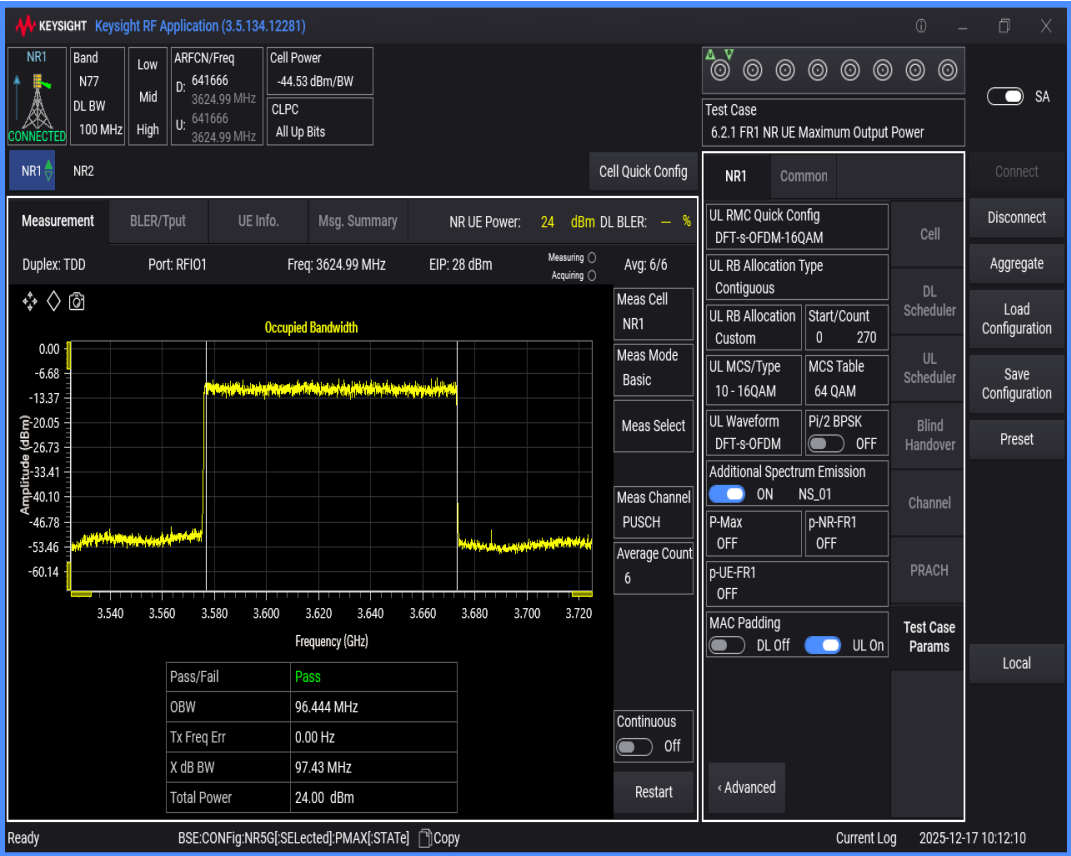
n77(3550-3700) SCS=30kHz DFT_QAM16 BW=10MHz Channel=641666 RB=24@0
