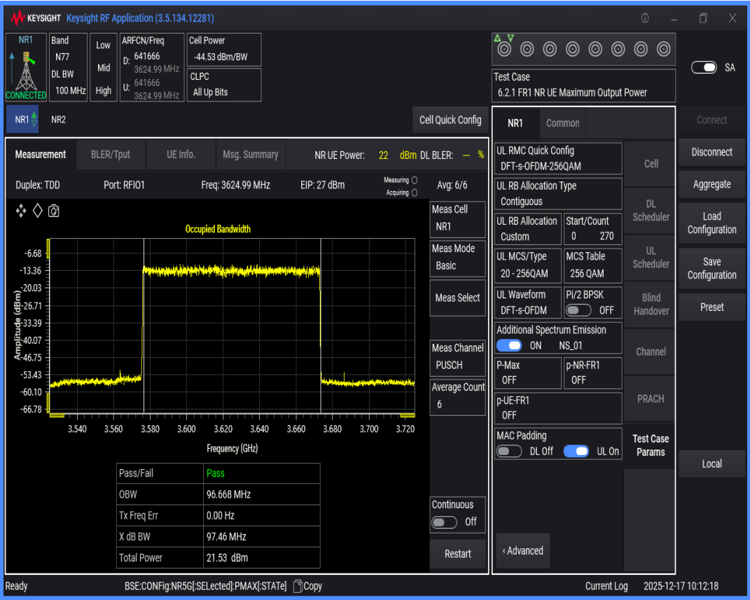
n77(3550-3700) SCS=30kHz DFT_QAM256 BW=10MHz Channel=641666 RB=24@0
