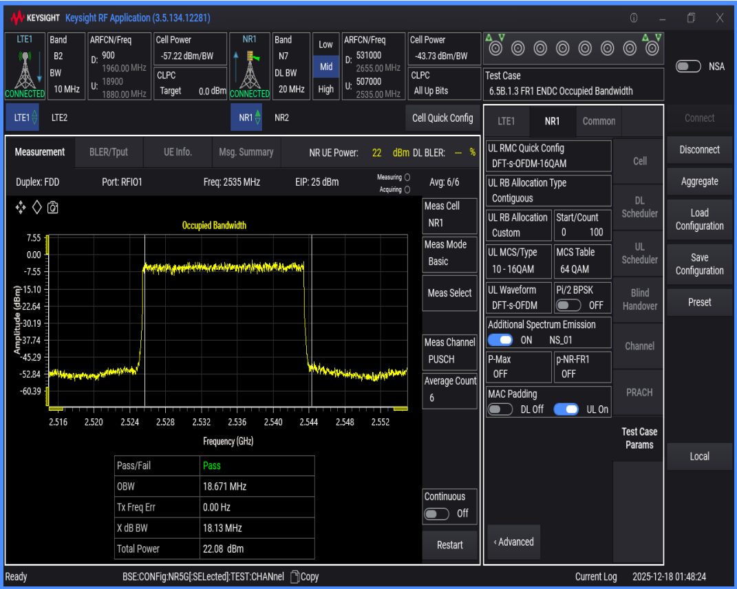
n7 SCS=15kHz DFT_QAM16 BW=5MHz Channel=507000 RB=25@0
