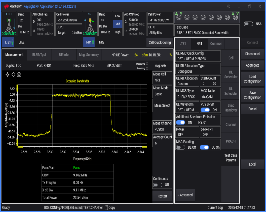
n7 SCS=15kHz DFT_BPSK BW=15MHz Channel=507000 RB=75@0
