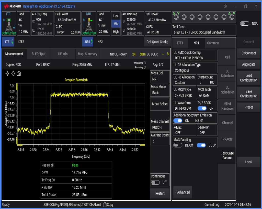
n7 SCS=15kHz DFT_BPSK BW=5MHz Channel=507000 RB=25@0
