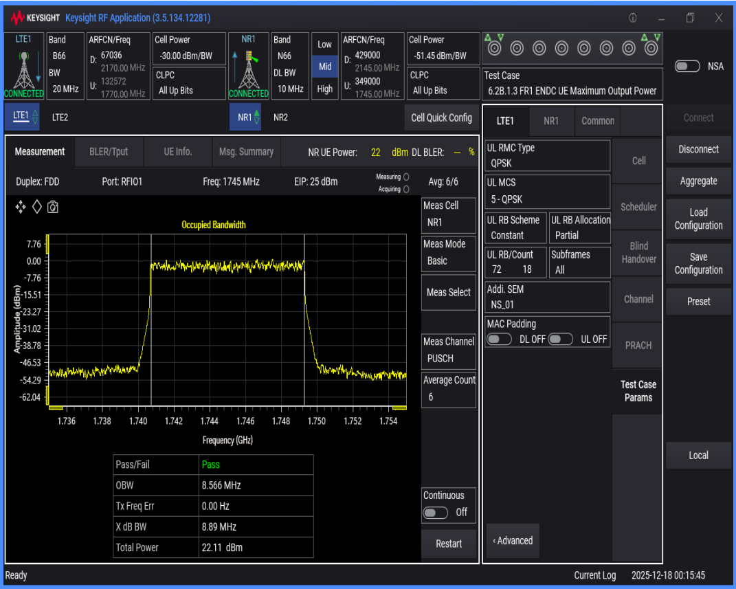
n66 SCS=30kHz DFT_QPSK BW=15MHz Channel=349000 RB=36@0
