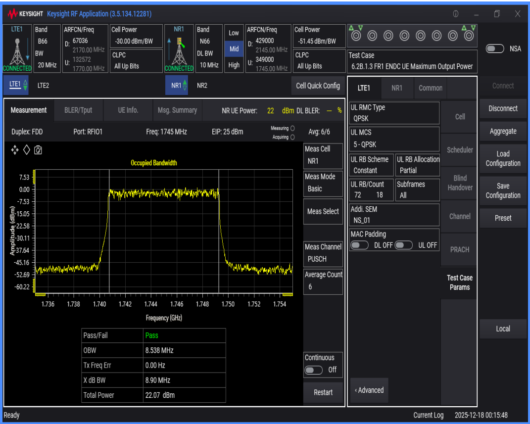
n66 SCS=30kHz DFT_QAM16 BW=15MHz Channel=349000 RB=36@0
