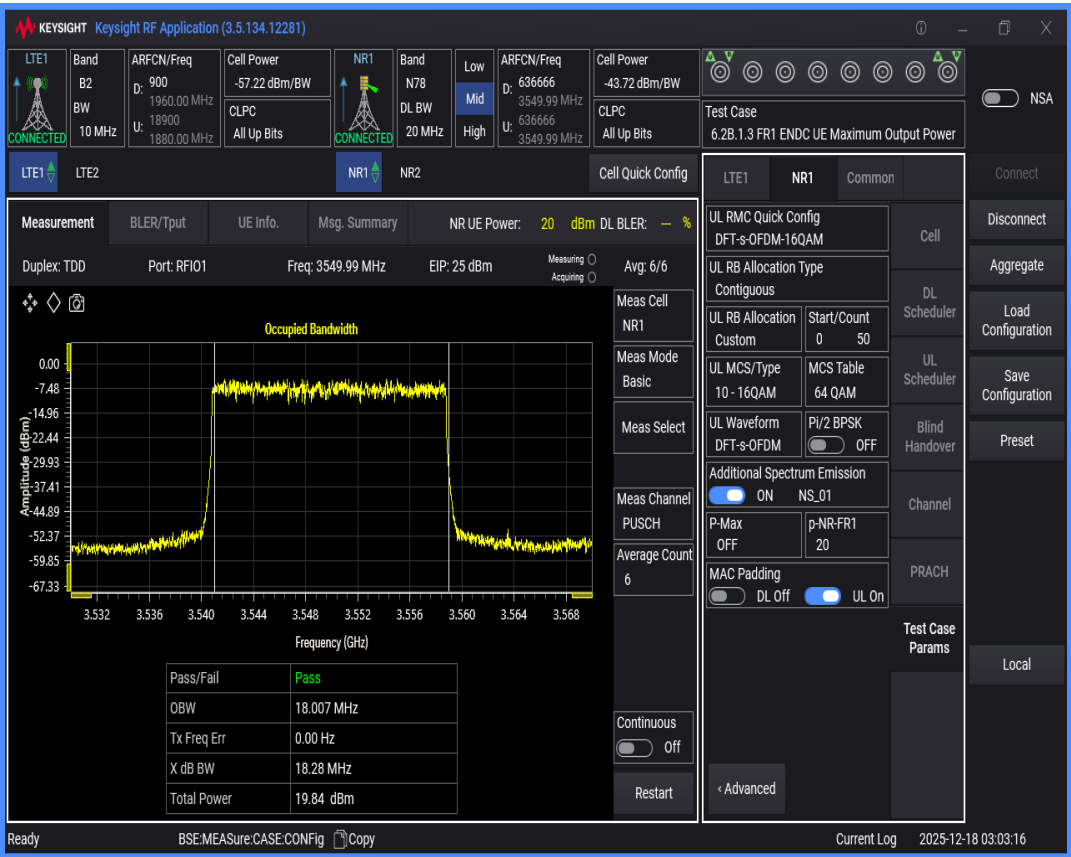
n78 SCS=30kHz DFT_QAM16 BW=40MHz Channel=636666 RB=100@0
