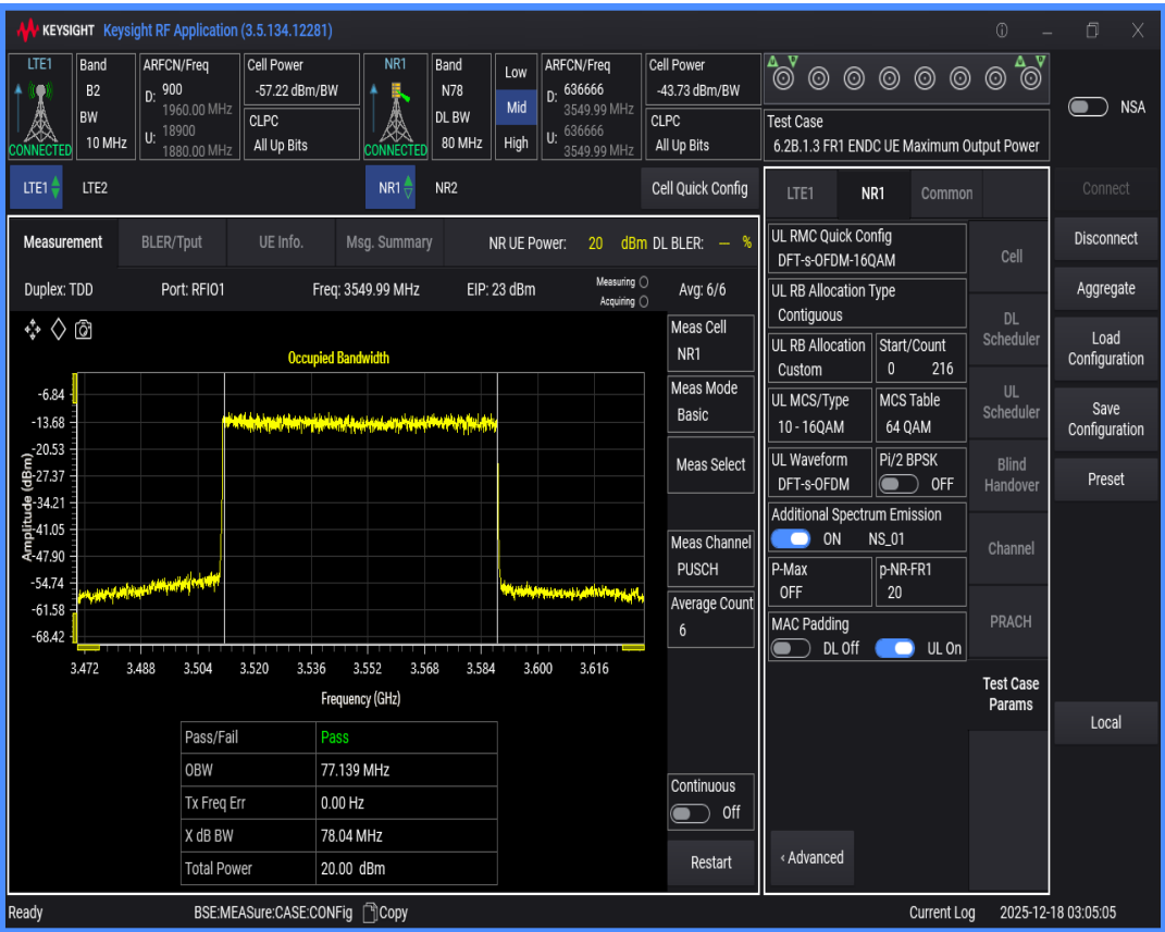
n78 SCS=30kHz DFT_QAM16 BW=90MHz Channel=636666 RB=240@0
