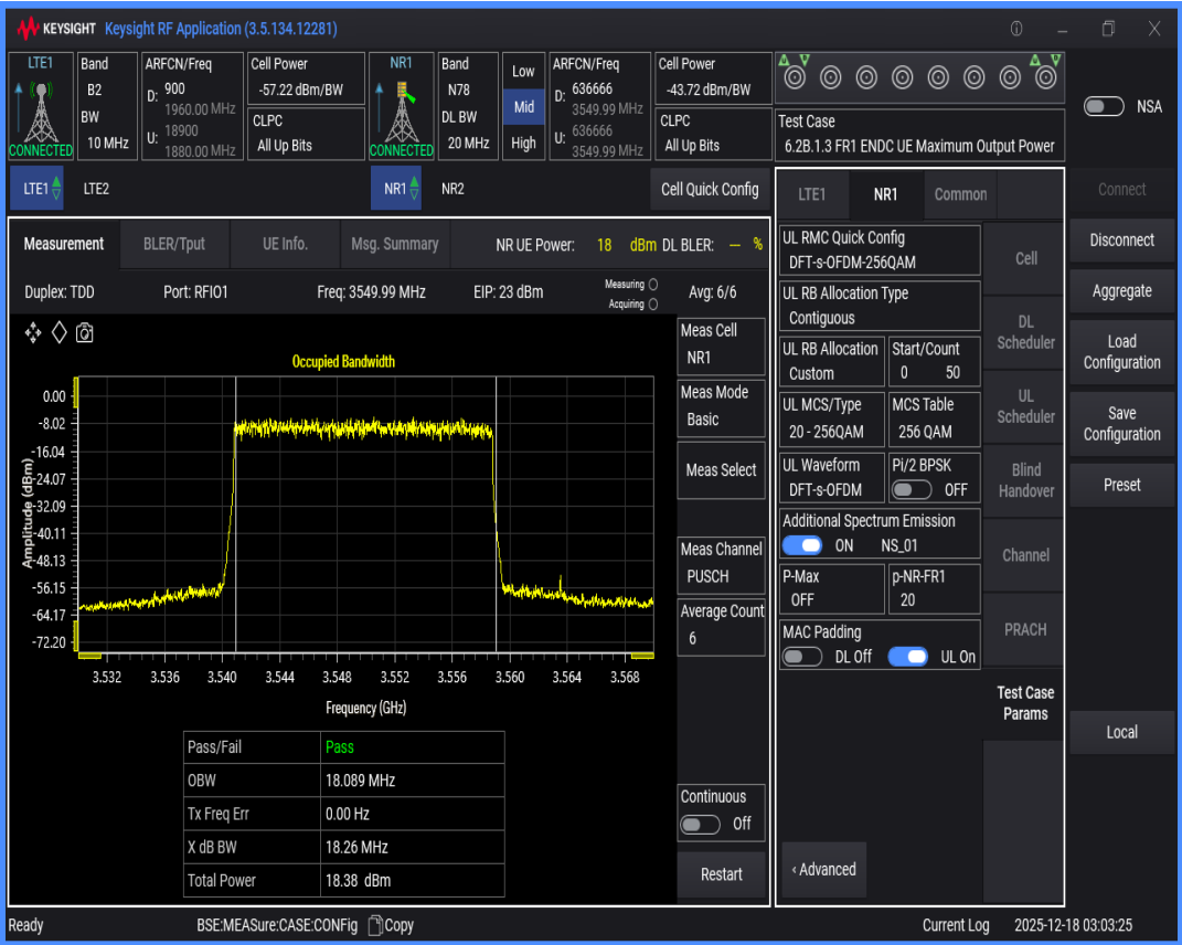
n78 SCS=30kHz DFT_QAM256 BW=40MHz Channel=636666 RB=100@0
