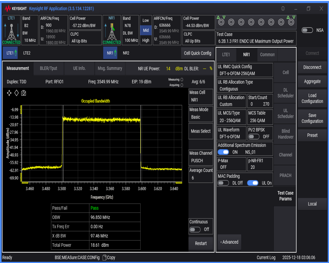
n78 SCS=30kHz DFT_QAM256 BW=10MHz Channel=636666 RB=24@0
