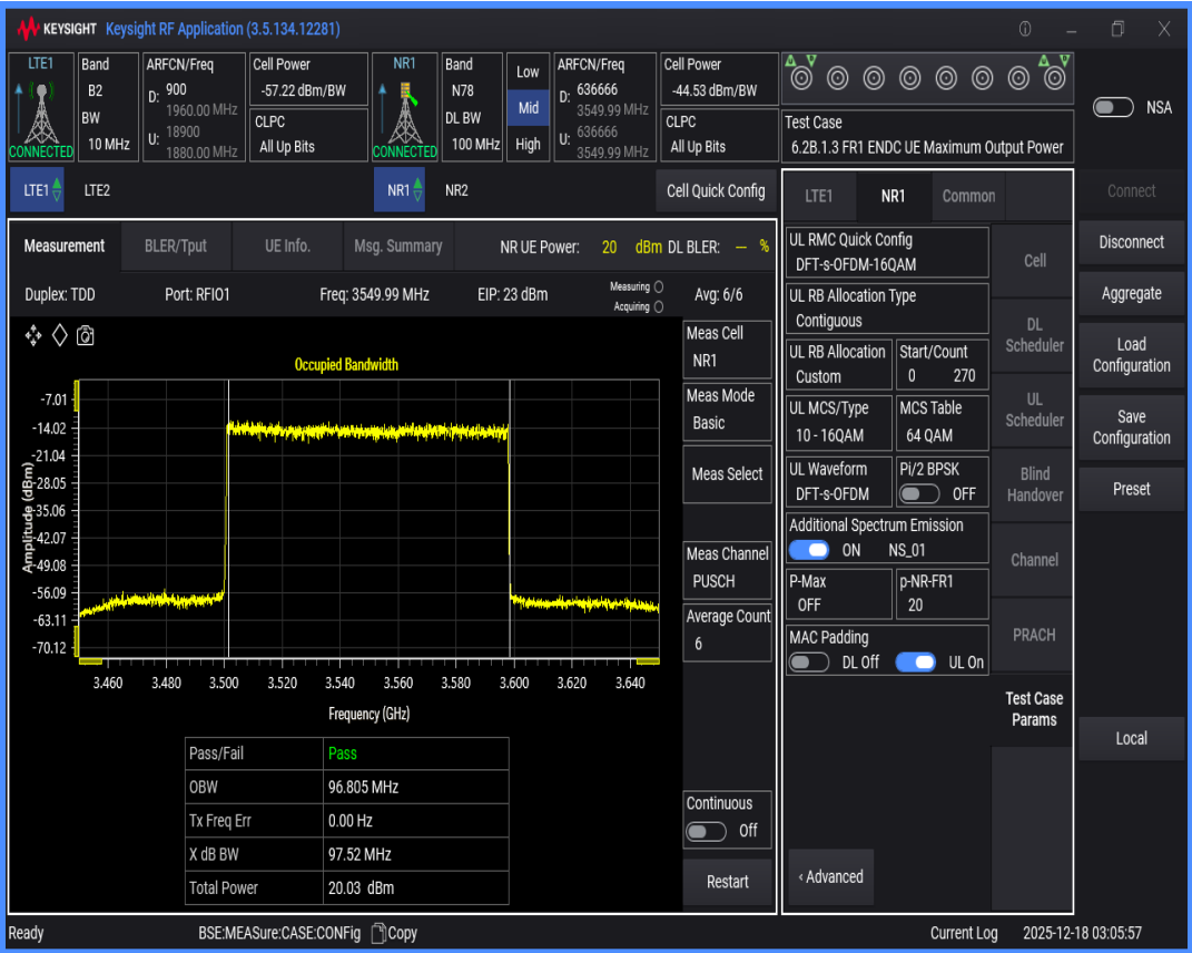
n78 SCS=30kHz DFT_QAM16 BW=10MHz Channel=636666 RB=24@0
