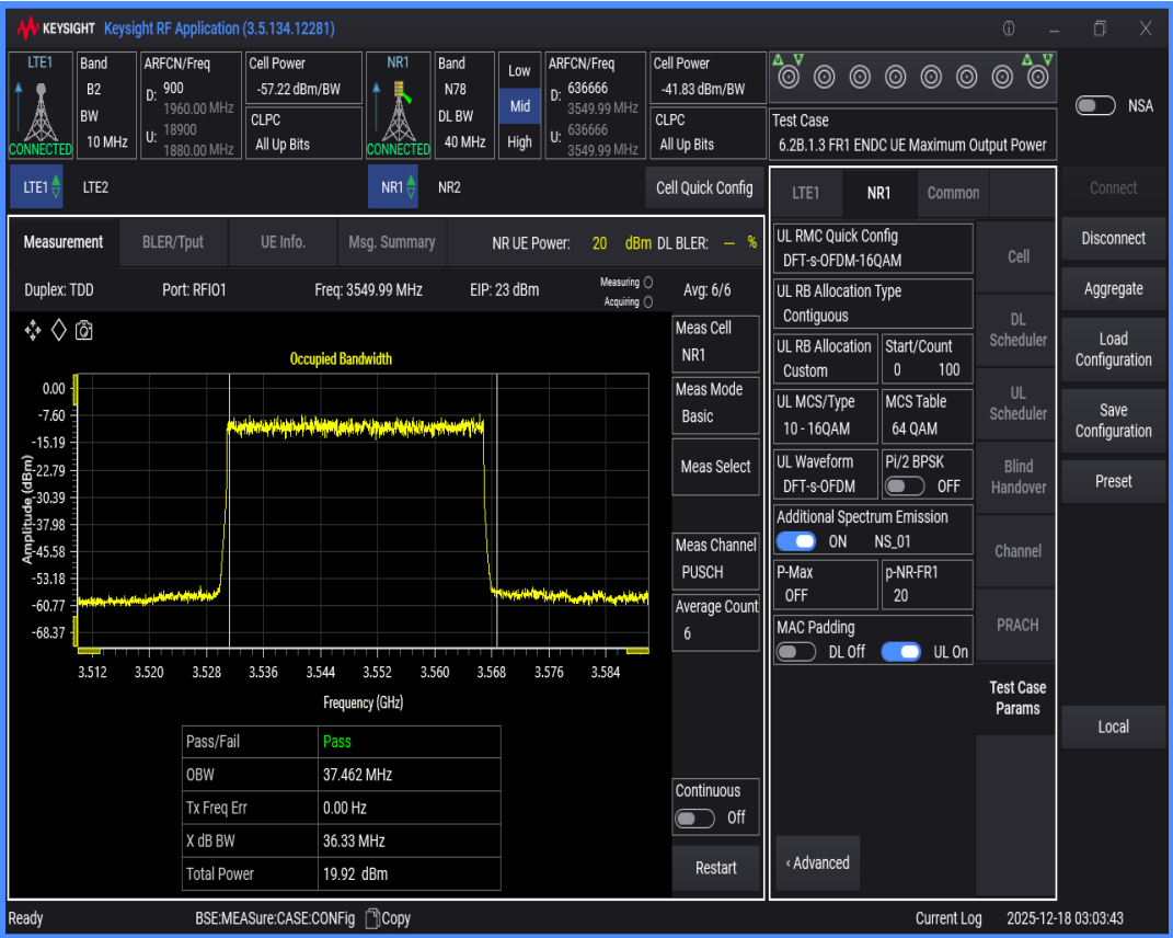
n78 SCS=30kHz DFT_QAM16 BW=50MHz Channel=636666 RB=128@0
