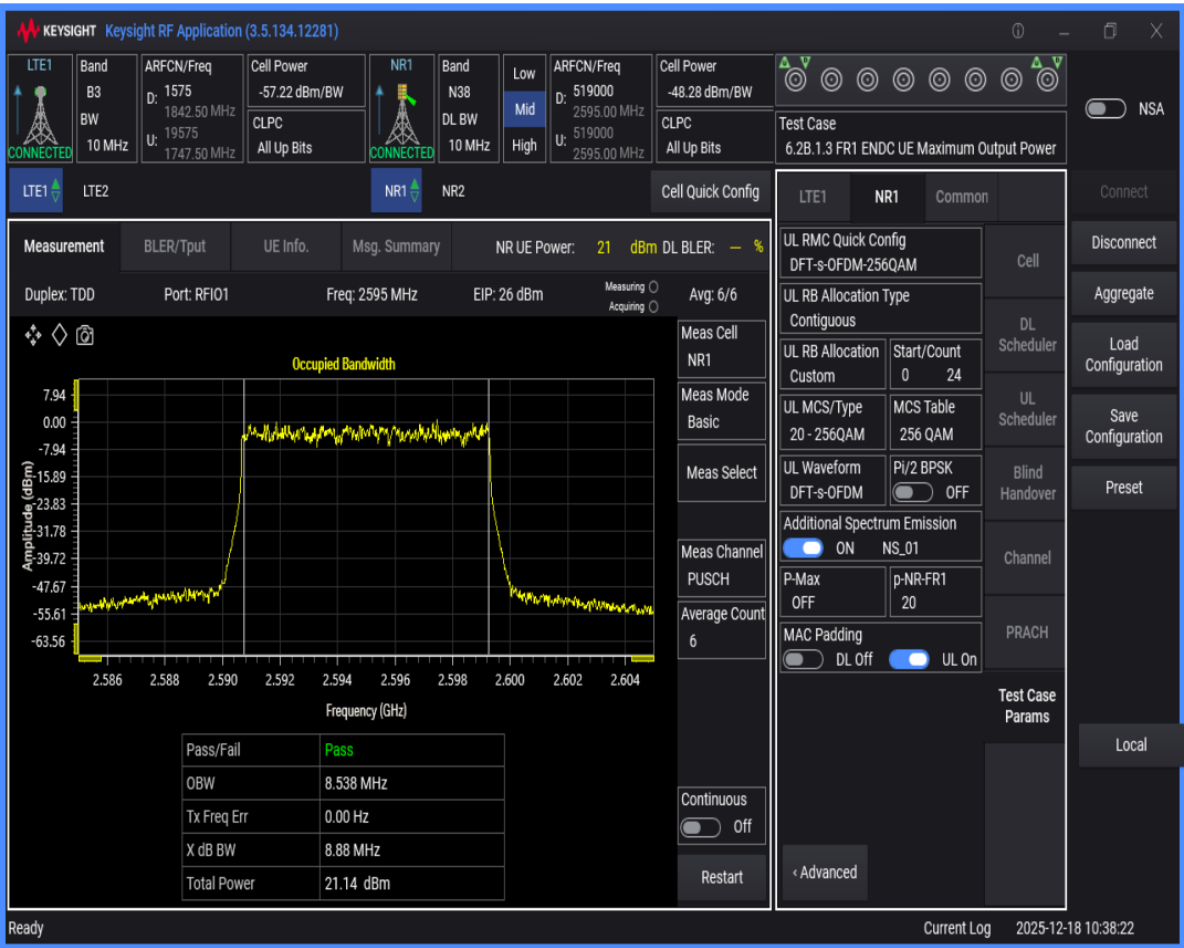
n38 SCS=30kHz DFT_QAM256 BW=15MHz Channel=519000 RB=36@0
