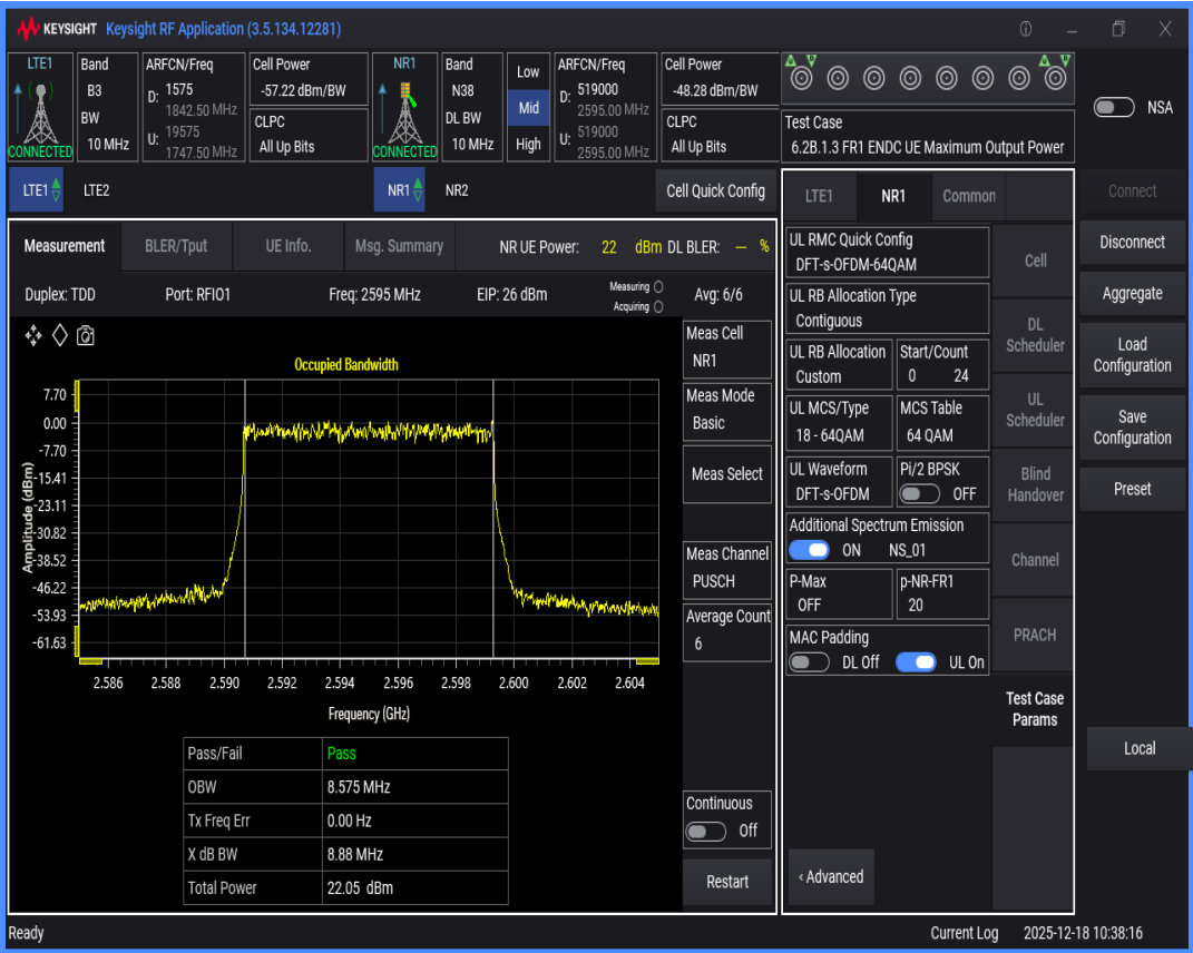
n38 SCS=30kHz DFT_QAM64 BW=15MHz Channel=519000 RB=36@0
