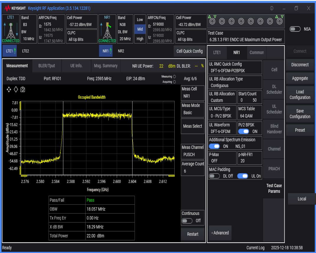
n38 SCS=30kHz DFT_QAM16 BW=10MHz Channel=519000 RB=24@0
