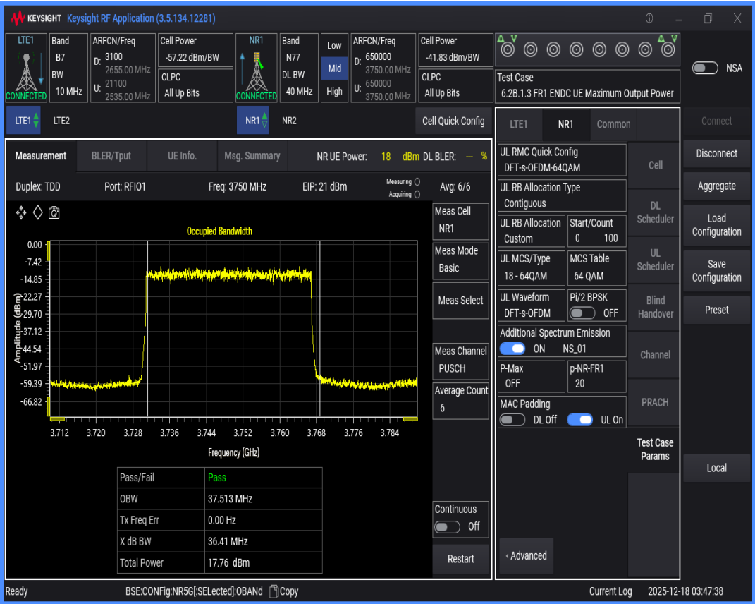
n77 SCS=30kHz DFT_QAM64 BW=50MHz Channel=650000 RB=128@0
