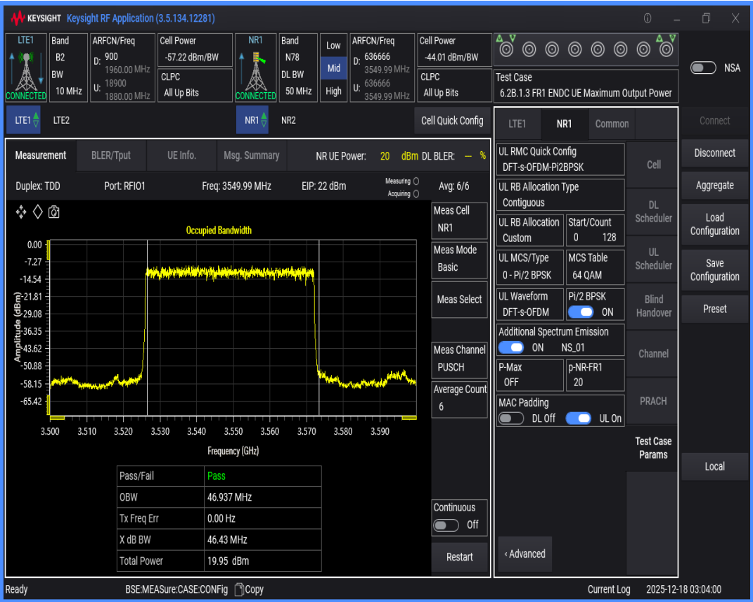
n78 SCS=30kHz DFT_BPSK BW=60MHz Channel=636666 RB=162@0
