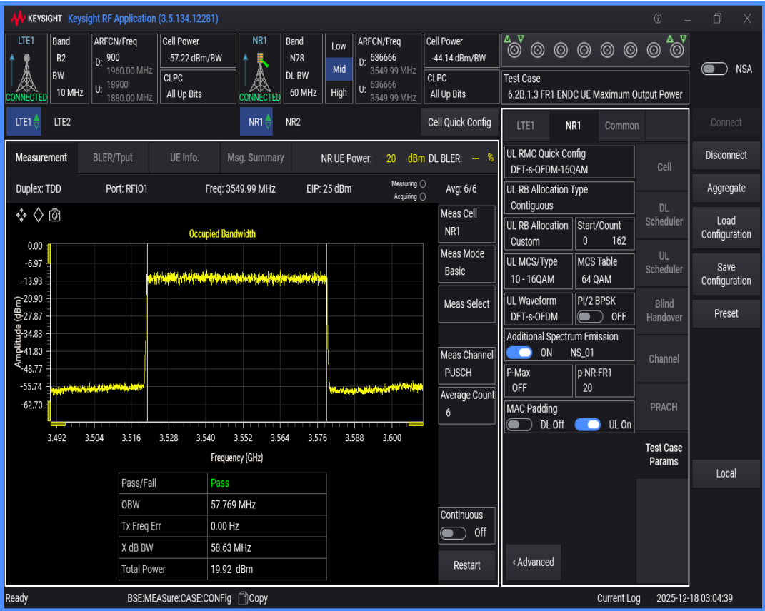
n78 SCS=30kHz DFT_QAM16 BW=80MHz Channel=636666 RB=216@0
