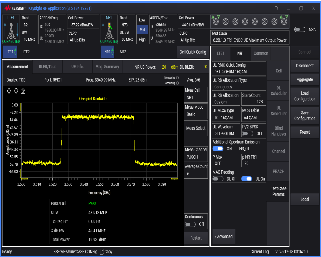
n78 SCS=30kHz DFT_QAM16 BW=60MHz Channel=636666 RB=162@0
