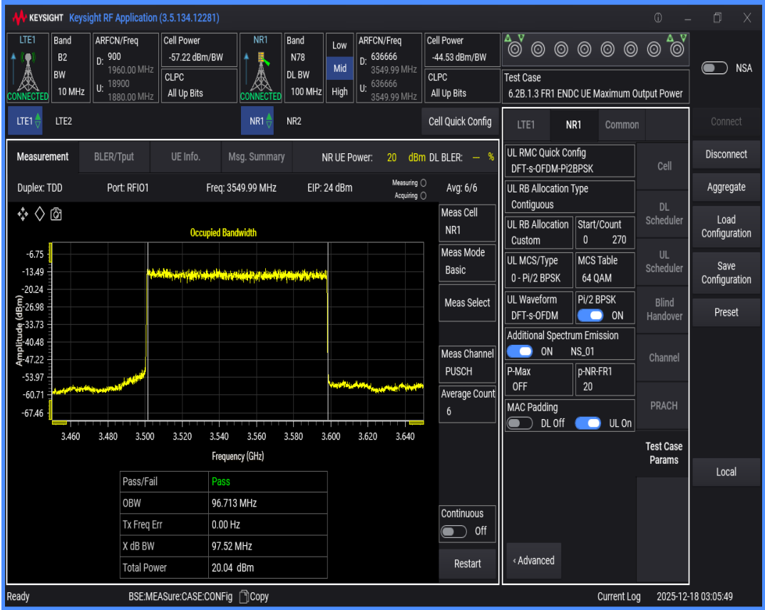
n78 SCS=30kHz DFT_BPSK BW=10MHz Channel=636666 RB=24@0
