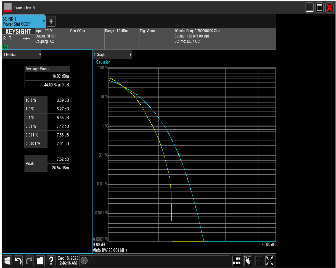
n78 SCS=30kHz DFT_QAM256 BW=40MHz Channel=621334 RB=100@0
