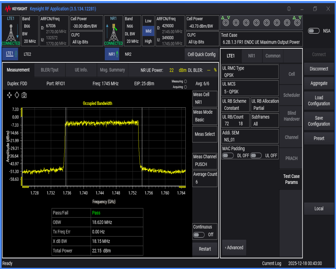
n66 SCS=15kHz DFT_QAM16 BW=40MHz Channel=349000 RB=216@0
