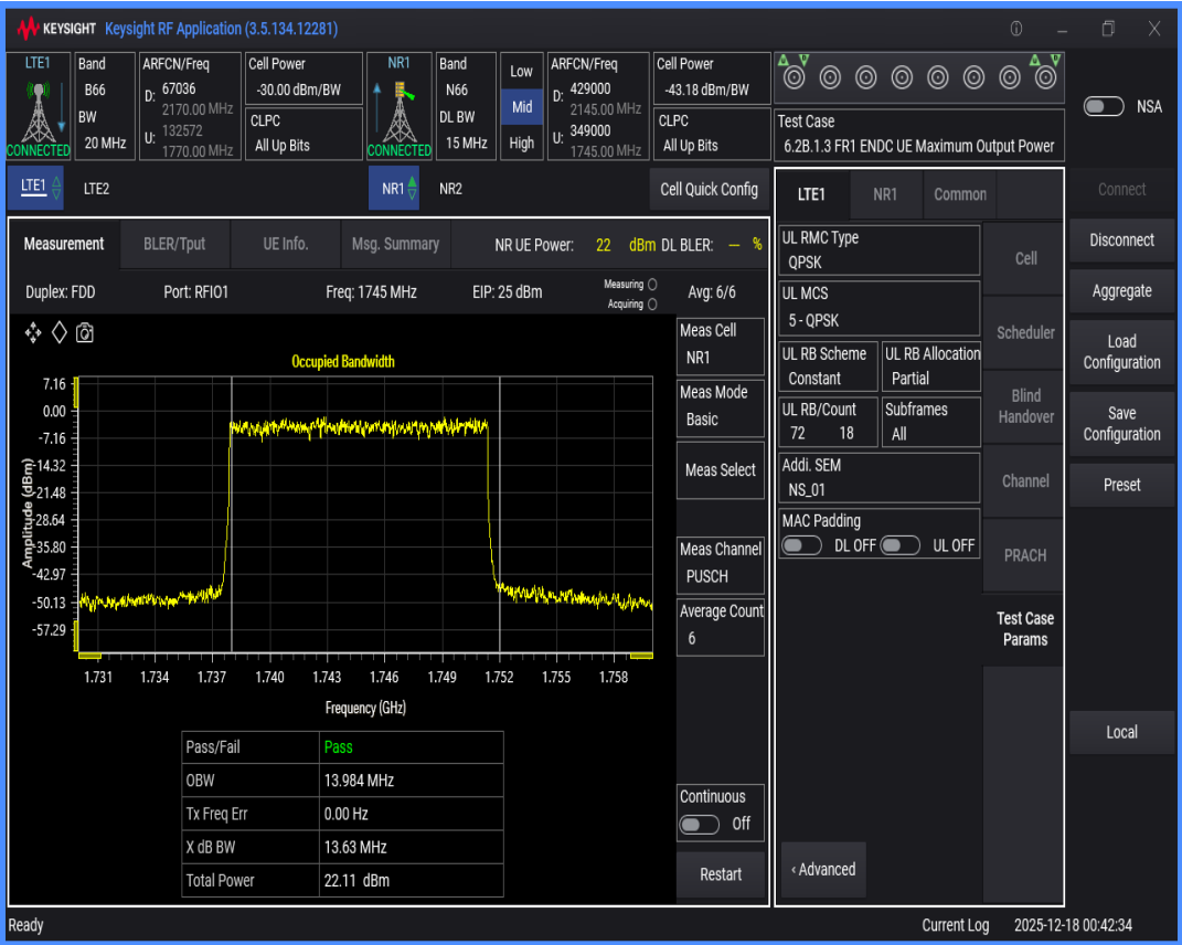
n66 SCS=15kHz DFT_QAM16 BW=20MHz Channel=349000 RB=100@0
