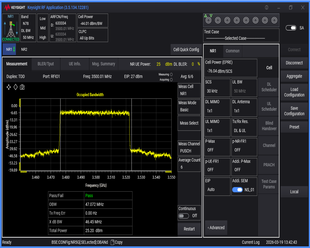
n78(3450-3550) SCS=30kHz DFT_QPSK BW=40MHz Channel=633334 RB=100@0
