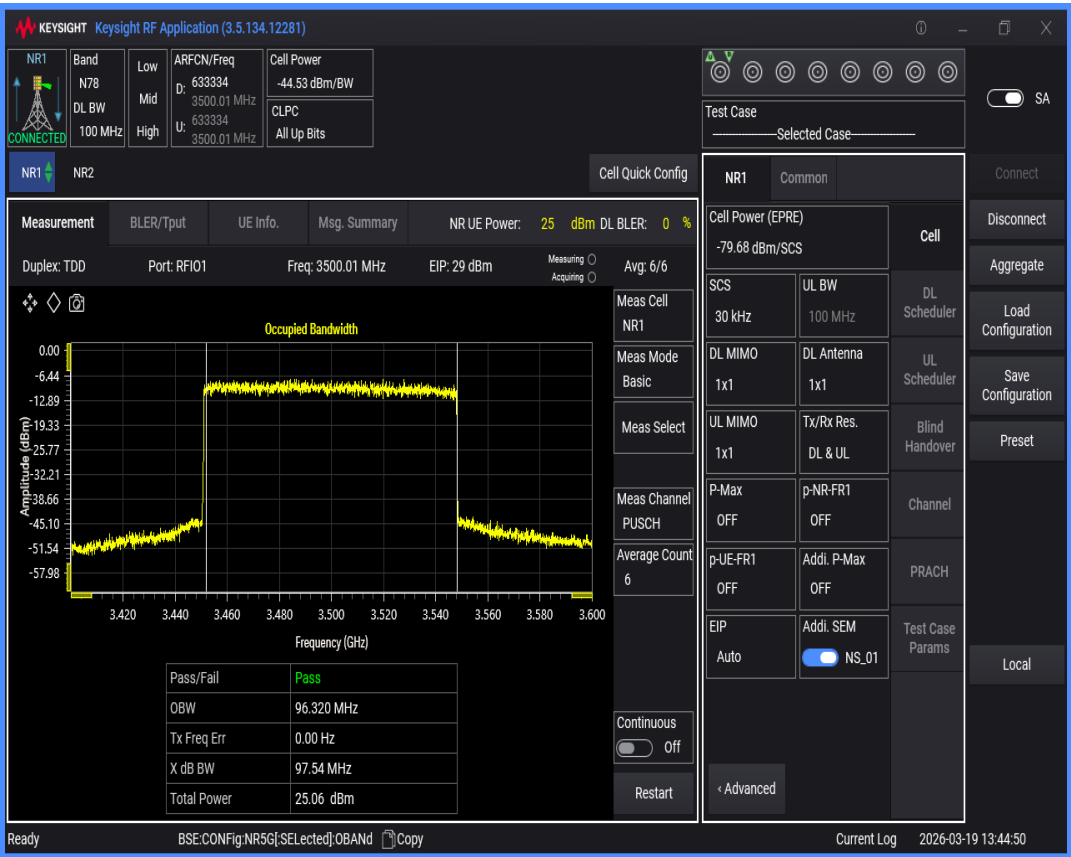
n78(3450-3550) SCS=30kHz DFT_QPSK BW=10MHz Channel=633334 RB=24@0
