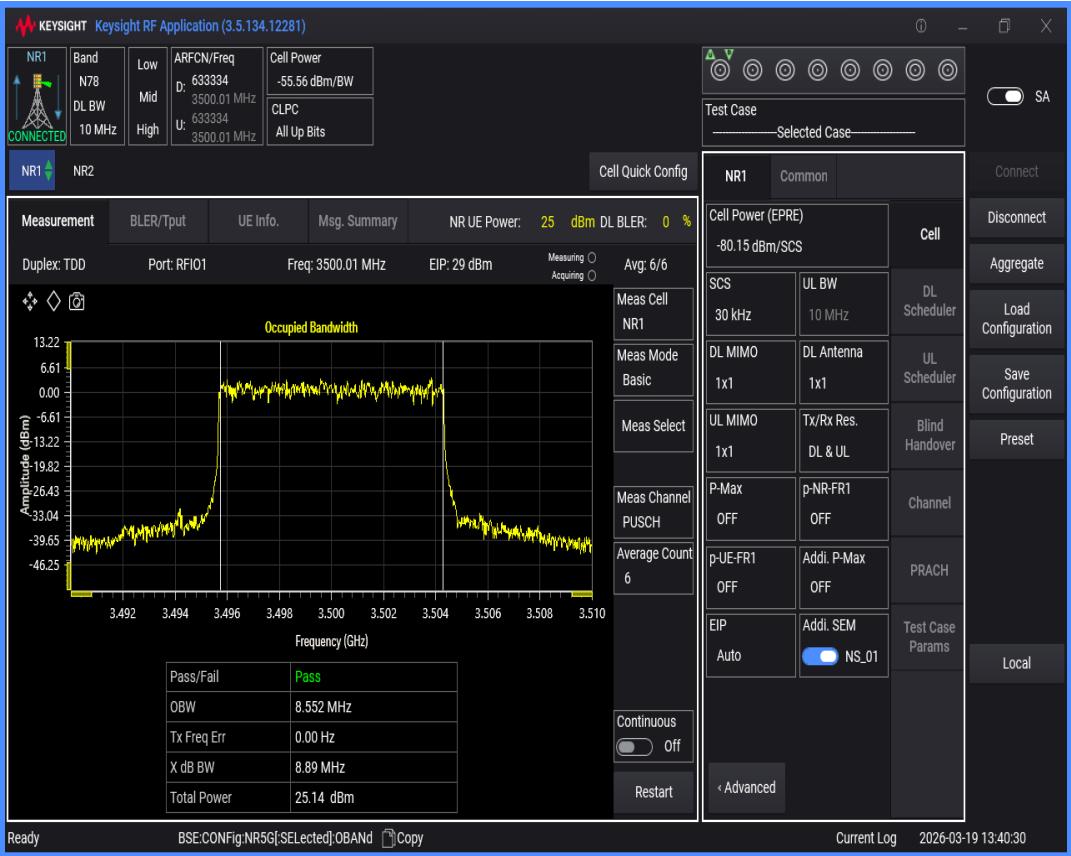
n78(3450-3550) SCS=30kHz DFT_QPSK BW=15MHz Channel=633334 RB=36@0
