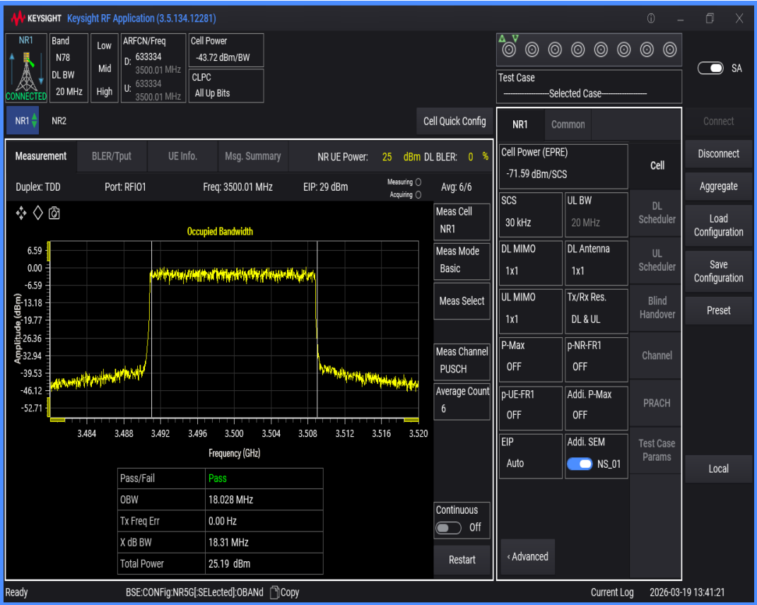
n78(3450-3550) SCS=30kHz DFT_QPSK BW=30MHz Channel=633334 RB=75@0
