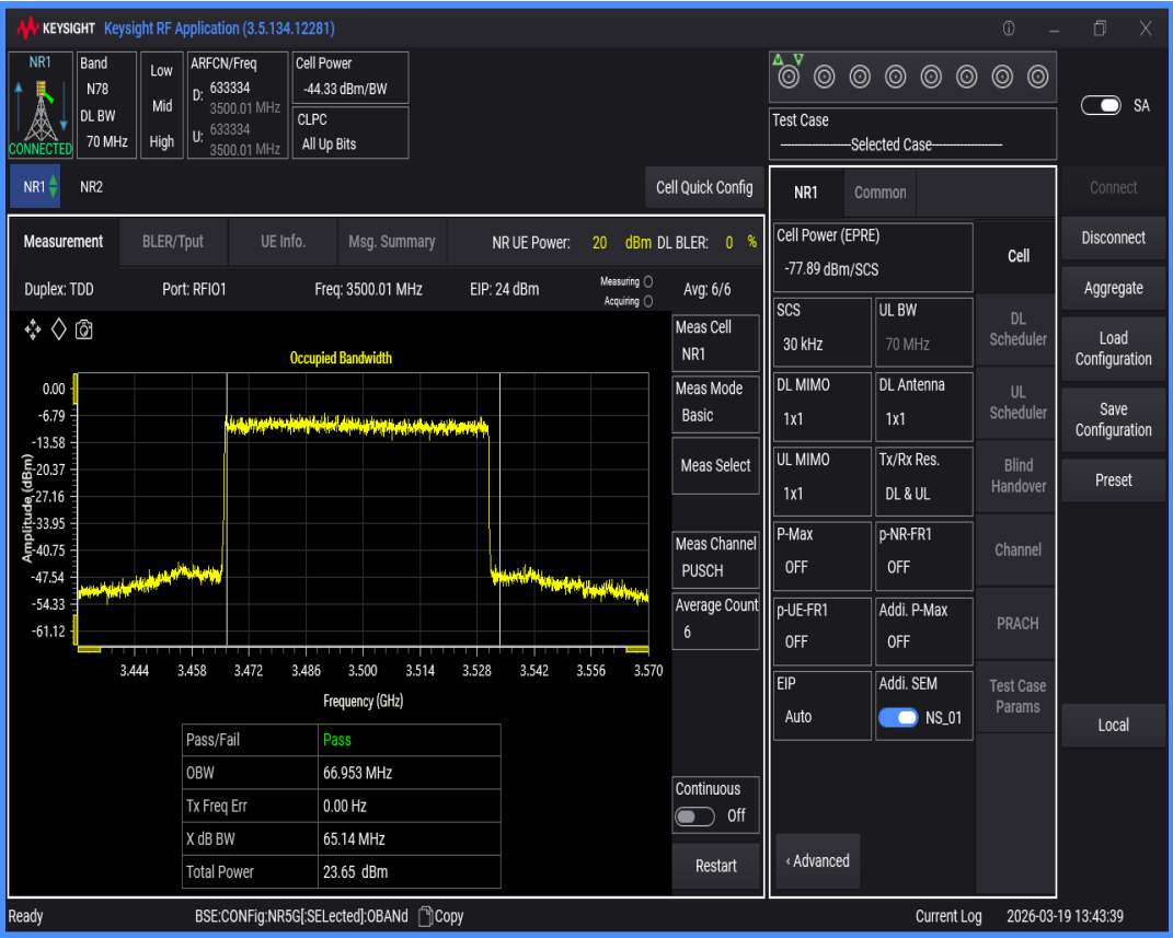
n78(3450-3550) SCS=30kHz DFT_QAM64 BW=90MHz Channel=633334 RB=240@0
