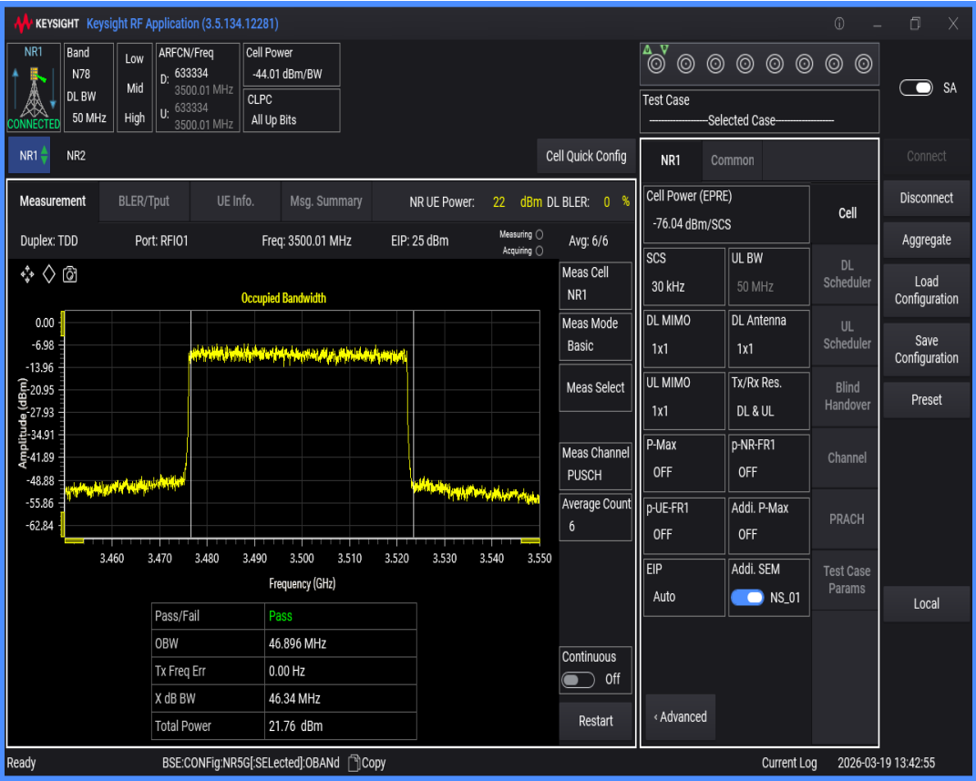
n78(3450-3550) SCS=30kHz DFT_QAM256 BW=60MHz Channel=633334 RB=162@0
