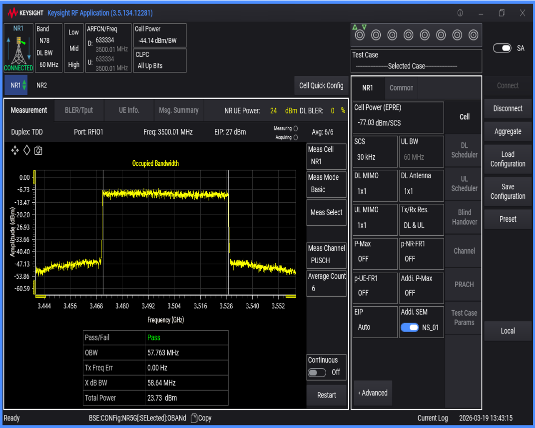
n78(3450-3550) SCS=30kHz DFT_QAM64 BW=80MHz Channel=633334 RB=216@0
