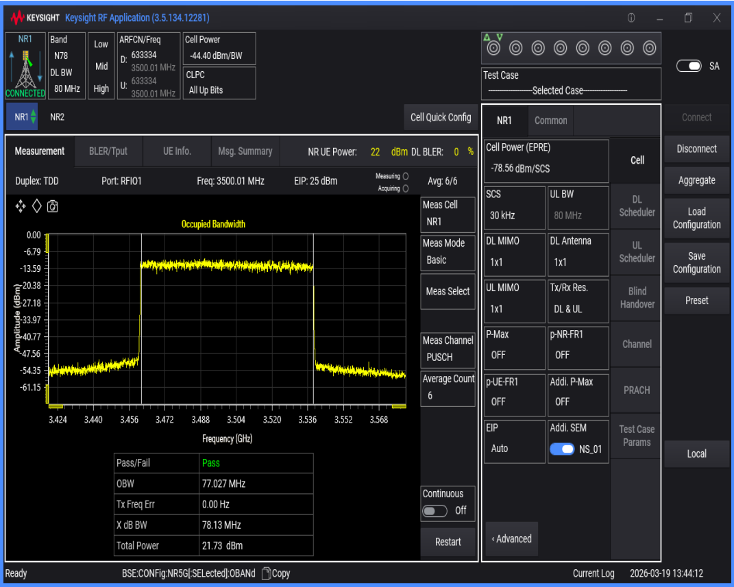
n78(3450-3550) SCS=30kHz DFT_QAM64 BW=10MHz Channel=633334 RB=24@0
