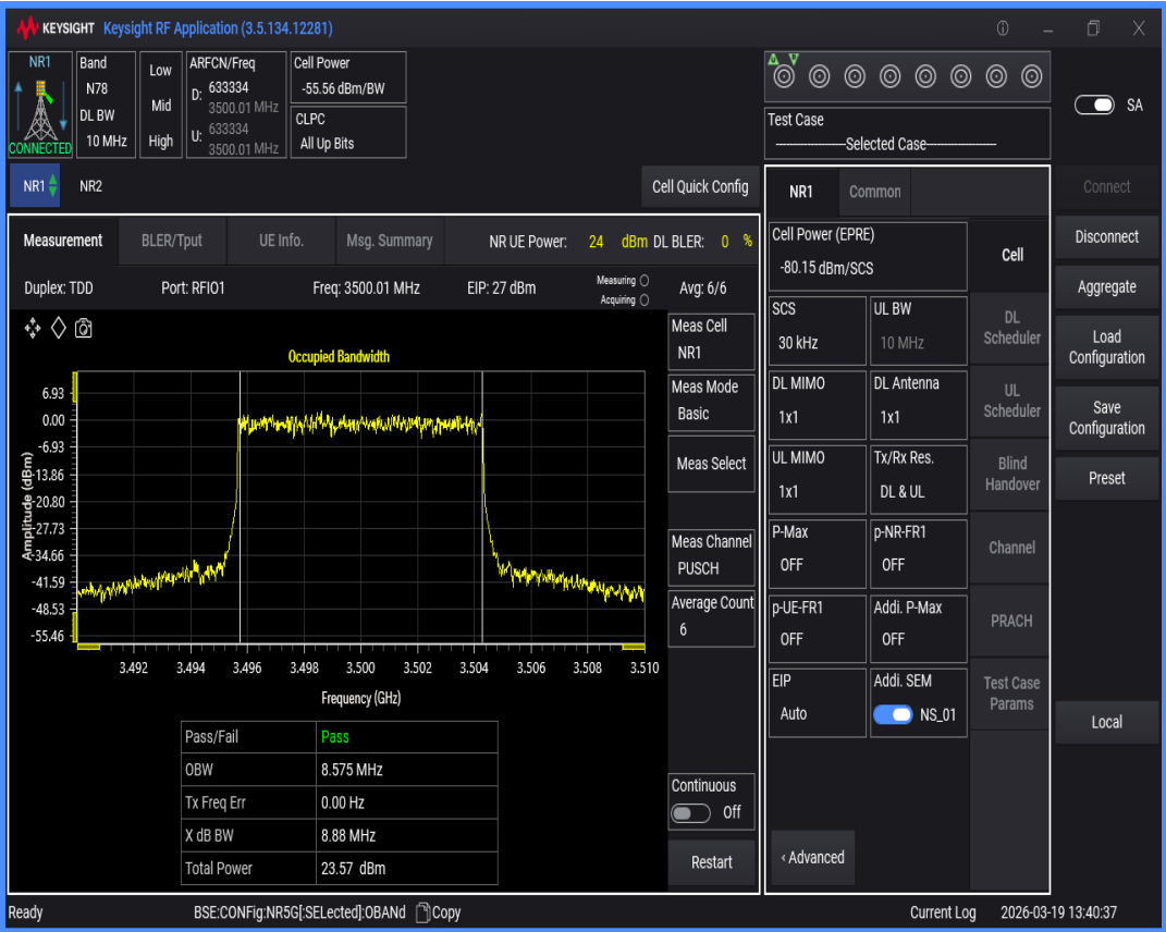
n78(3450-3550) SCS=30kHz DFT_QAM64 BW=100MHz Channel=633334 RB=270@0
