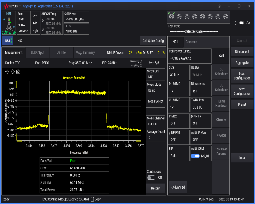
n78(3450-3550) SCS=30kHz DFT_QAM256 BW=90MHz Channel=633334 RB=240@0
