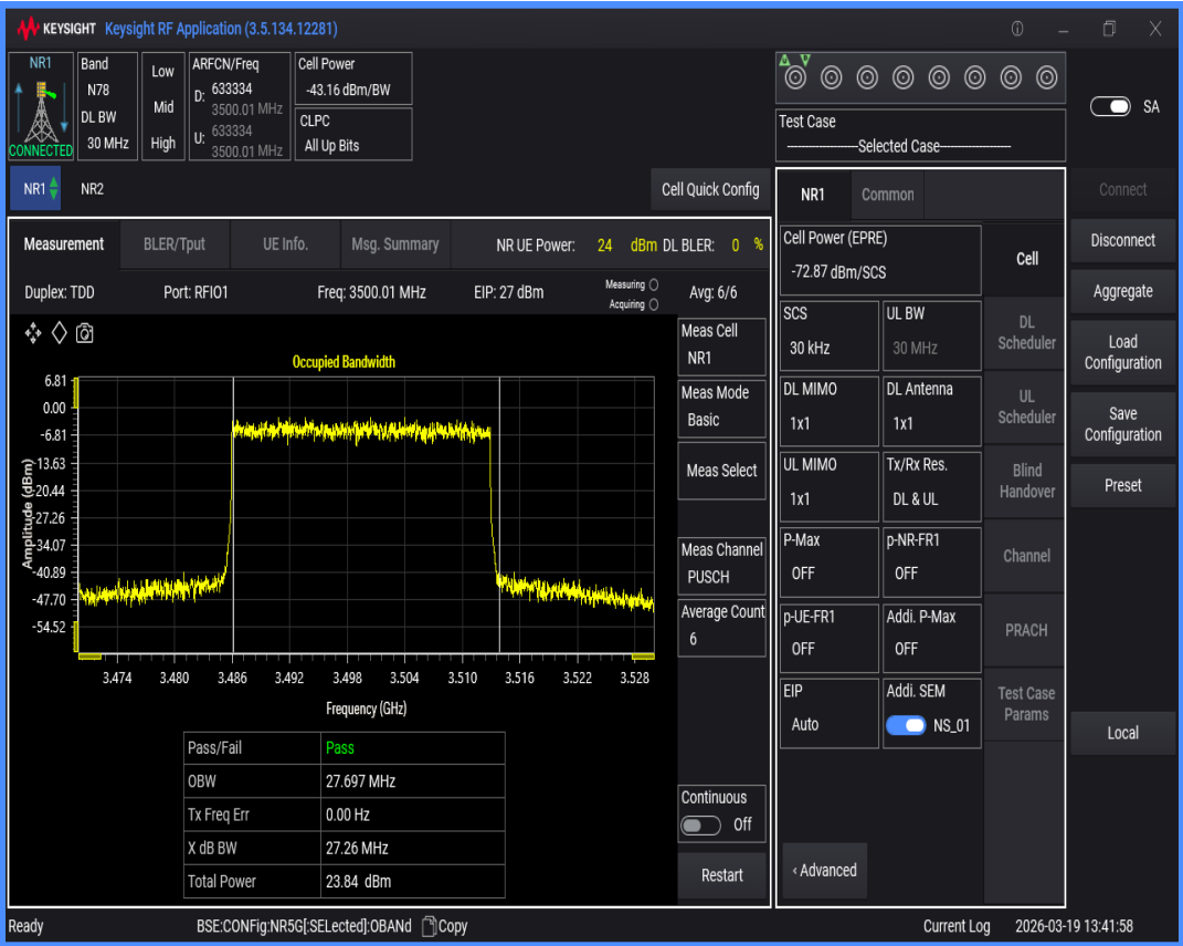
n78(3450-3550) SCS=30kHz DFT_QAM64 BW=60MHz Channel=633334 RB=162@0
