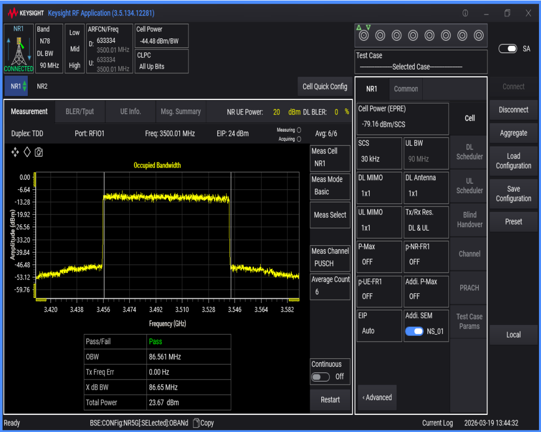
n78(3450-3550) SCS=30kHz DFT_QPSK BW=100MHz Channel=633334 RB=270@0
