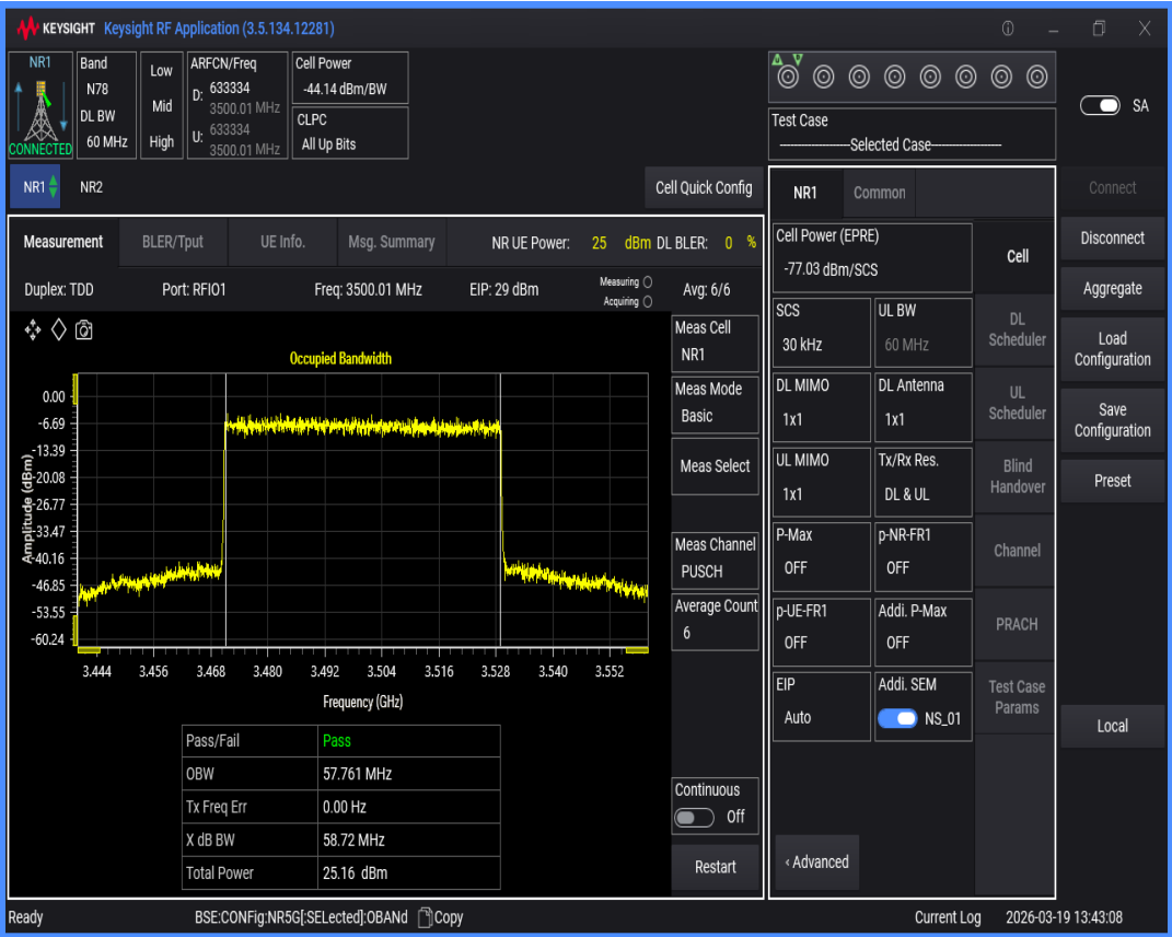
n78(3450-3550) SCS=30kHz DFT_QPSK BW=50MHz Channel=633334 RB=128@0
