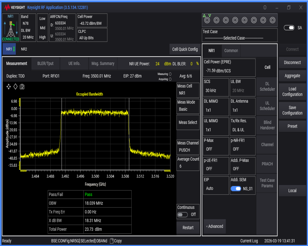
n78(3450-3550) SCS=30kHz DFT_QAM64 BW=15MHz Channel=633334 RB=36@0
