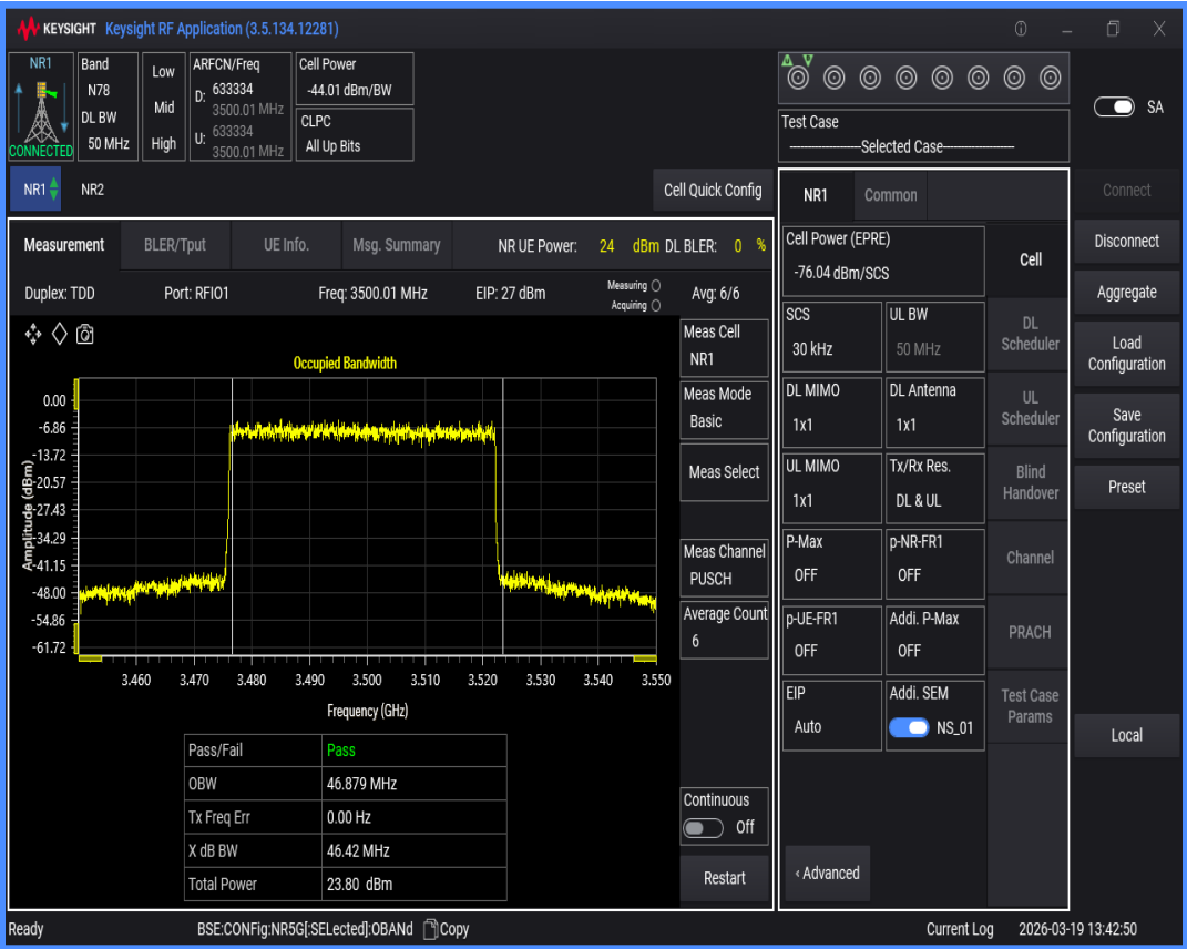
n78(3450-3550) SCS=30kHz DFT_QAM64 BW=40MHz Channel=633334 RB=100@0
