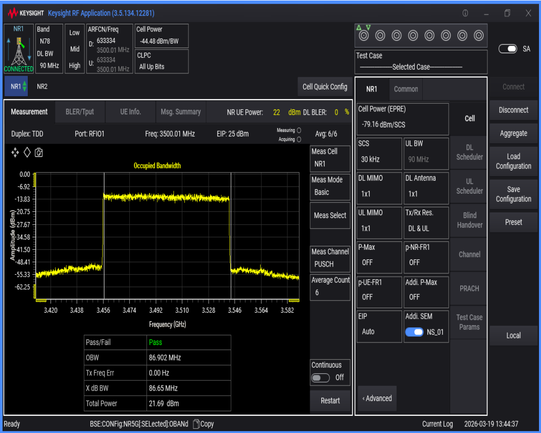
n78(3450-3550) SCS=30kHz DFT_QAM256 BW=80MHz Channel=633334 RB=216@0
