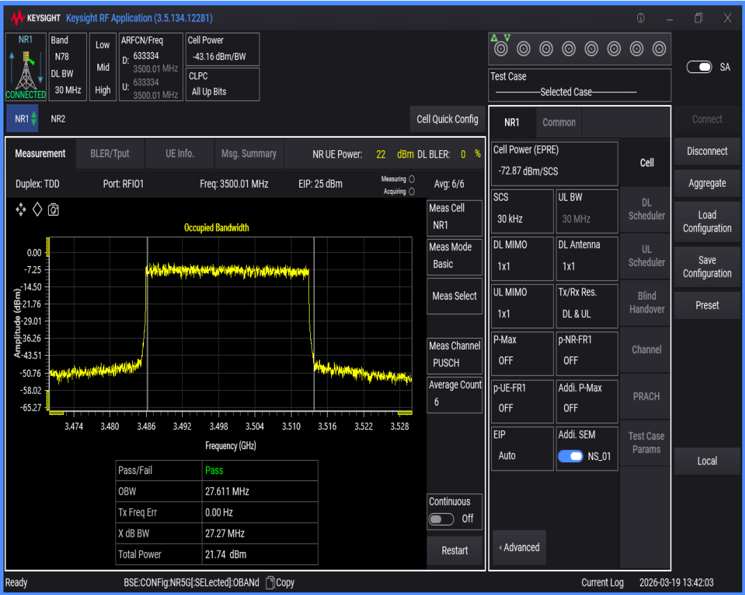
n78(3450-3550) SCS=30kHz DFT_QAM256 BW=50MHz Channel=633334 RB=128@0
