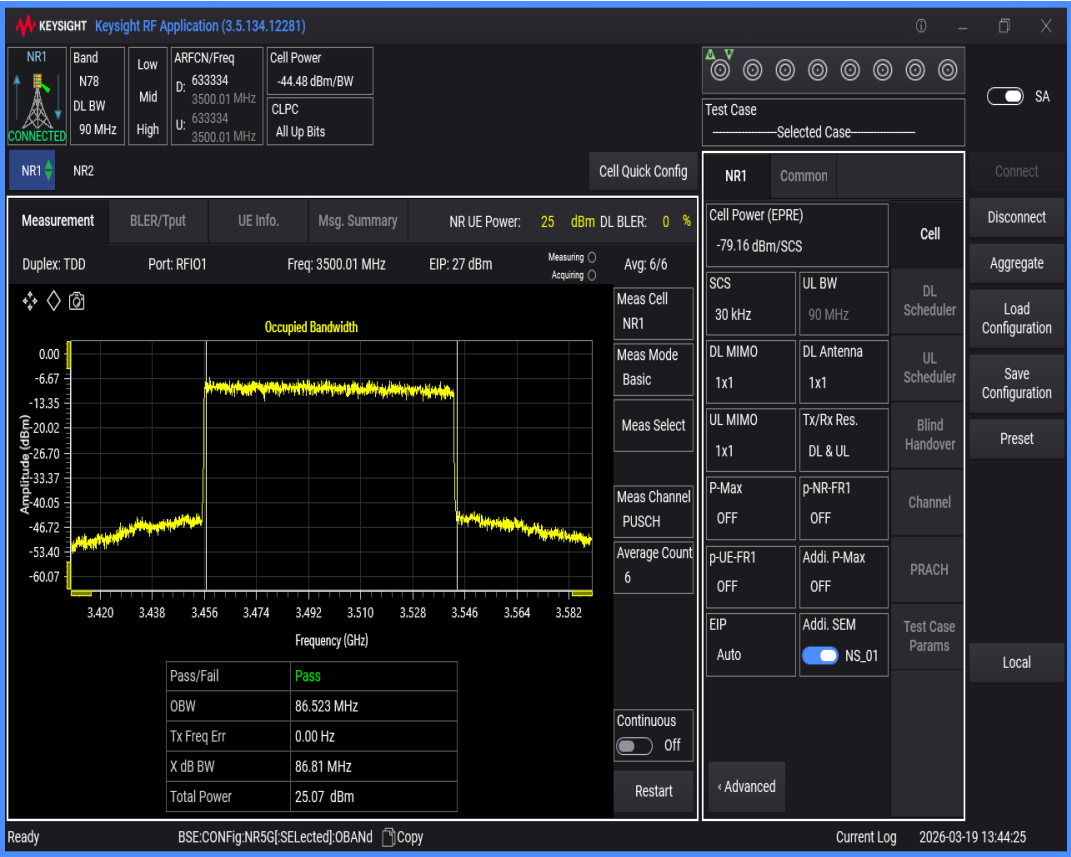
n78(3450-3550) SCS=30kHz DFT_QPSK BW=80MHz Channel=633334 RB=216@0
