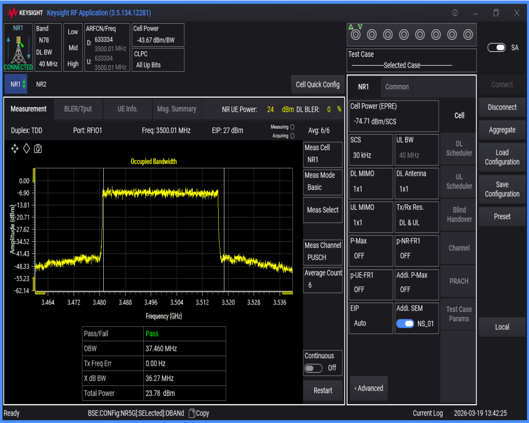
n78(3450-3550) SCS=30kHz DFT_QAM64 BW=30MHz Channel=633334 RB=75@0
