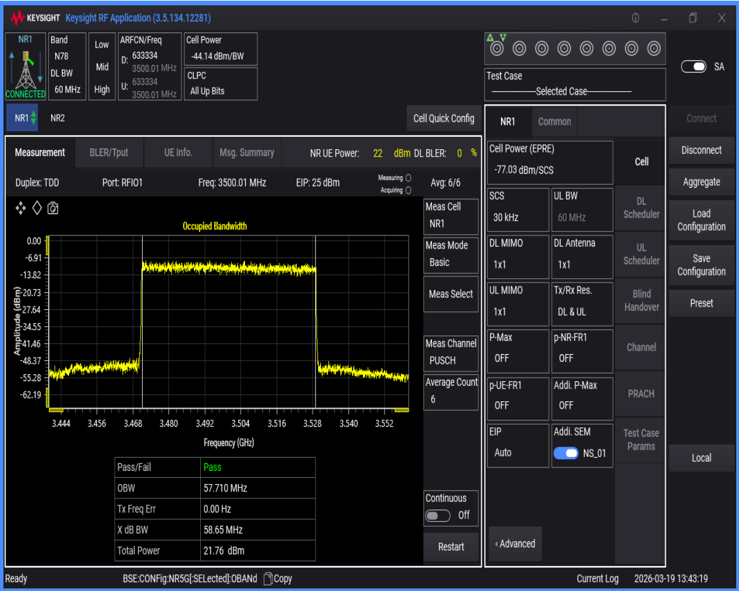
n78(3450-3550) SCS=30kHz DFT_QAM256 BW=70MHz Channel=633334 RB=180@0
