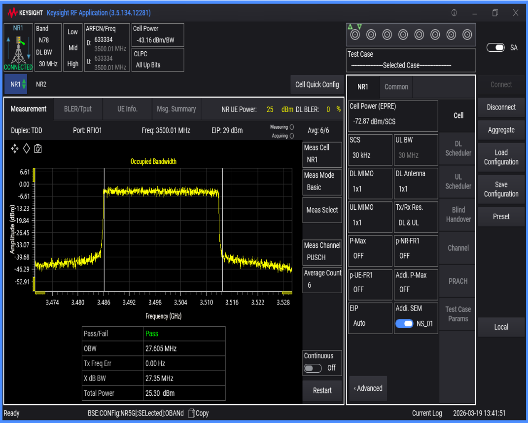
n78(3450-3550) SCS=30kHz DFT_QPSK BW=60MHz Channel=633334 RB=162@0
