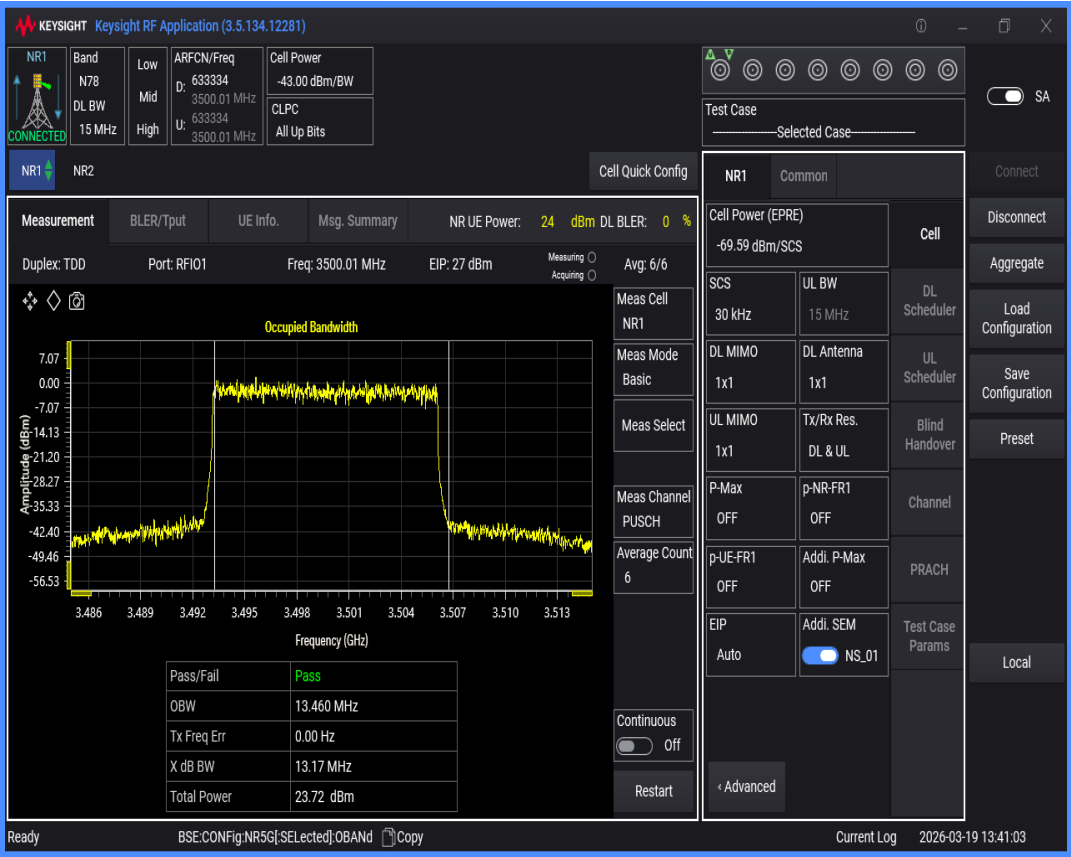
n78(3450-3550) SCS=30kHz DFT_QAM64 BW=50MHz Channel=633334 RB=128@0
