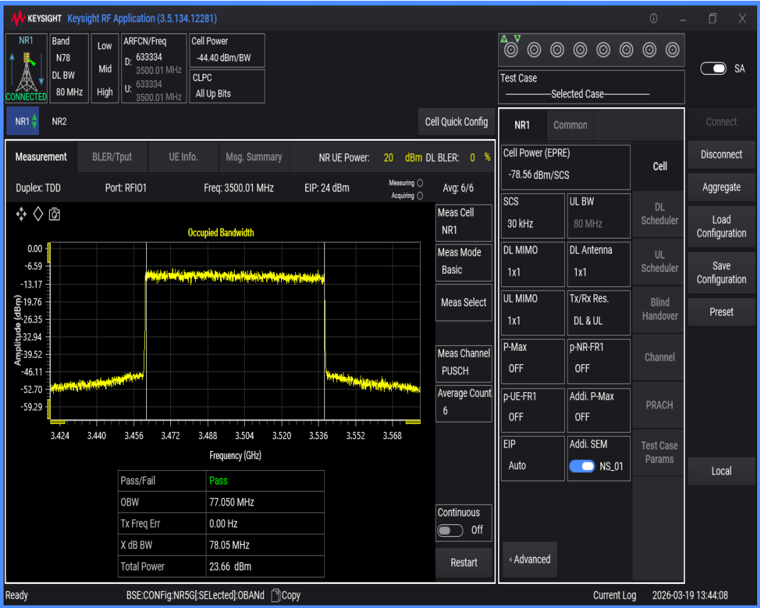
n78(3450-3550) SCS=30kHz DFT_QAM64 BW=70MHz Channel=633334 RB=180@0
