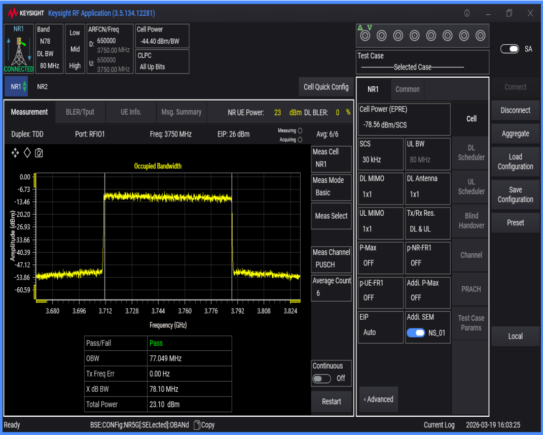
n78(3700-3800) SCS=30kHz DFT_QAM64 BW=90MHz Channel=650000 RB=240@0
