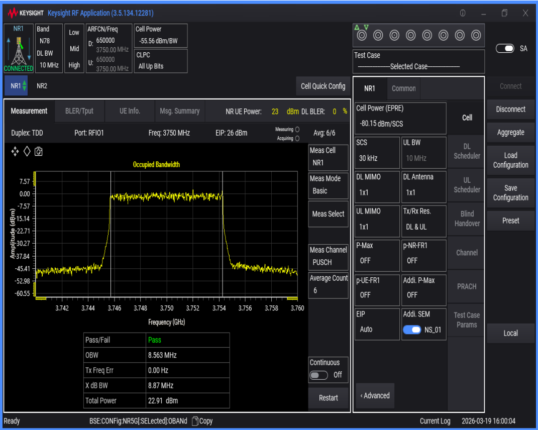
n78(3700-3800) SCS=30kHz DFT_QAM64 BW=100MHz Channel=650000 RB=270@0
