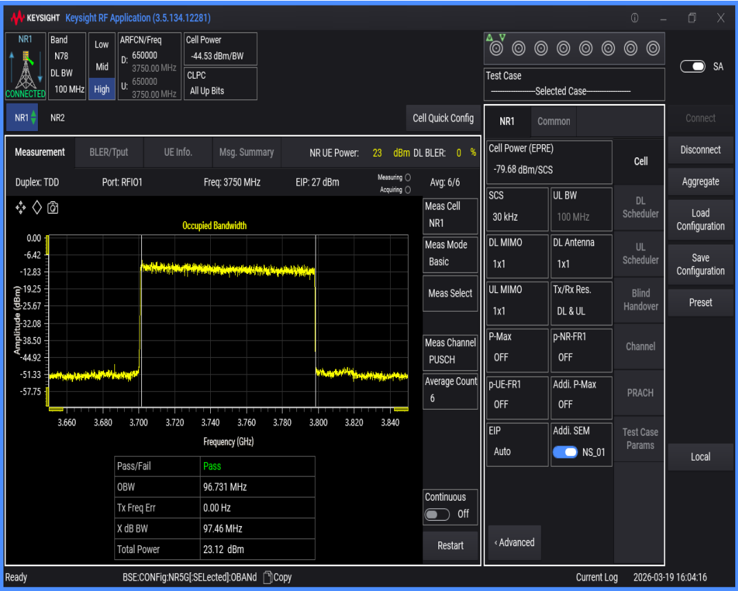
n78(3700-3800) SCS=30kHz DFT_QAM64 BW=15MHz Channel=650000 RB=36@0
