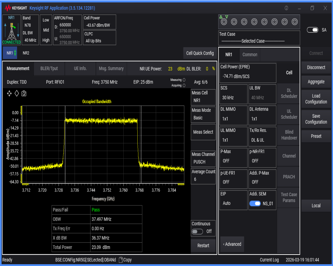
n78(3700-3800) SCS=30kHz DFT_QAM64 BW=50MHz Channel=650000 RB=128@0
