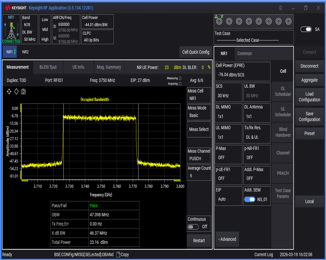
n78(3700-3800) SCS=30kHz DFT_QAM64 BW=60MHz Channel=650000 RB=162@0
