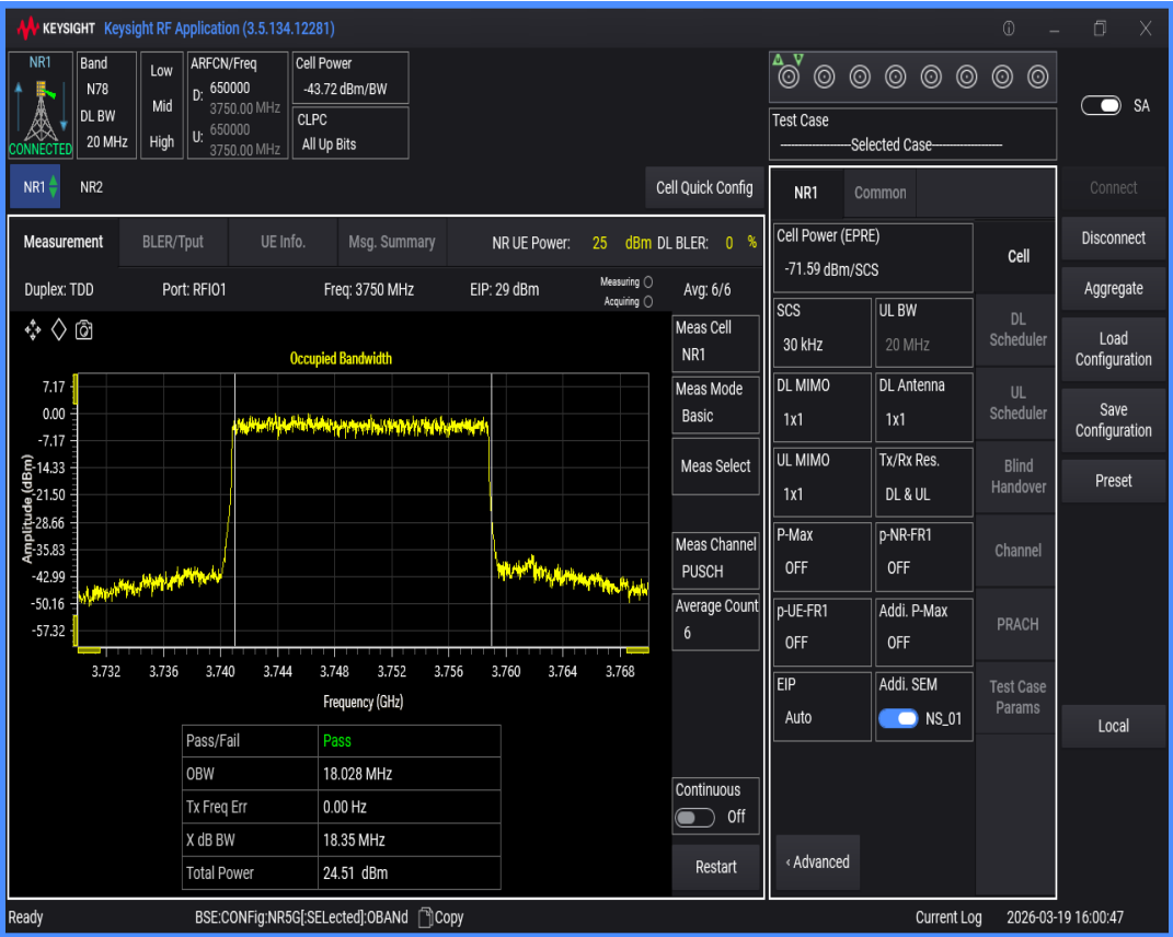
n78(3700-3800) SCS=30kHz DFT_QPSK BW=30MHz Channel=650000 RB=75@0
