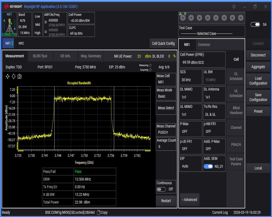
n78(3700-3800) SCS=30kHz DFT_QAM64 BW=30MHz Channel=650000 RB=75@0
