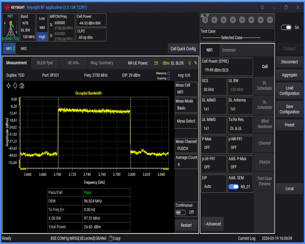
n78(3700-3800) SCS=30kHz DFT_QPSK BW=10MHz Channel=650000 RB=24@0
