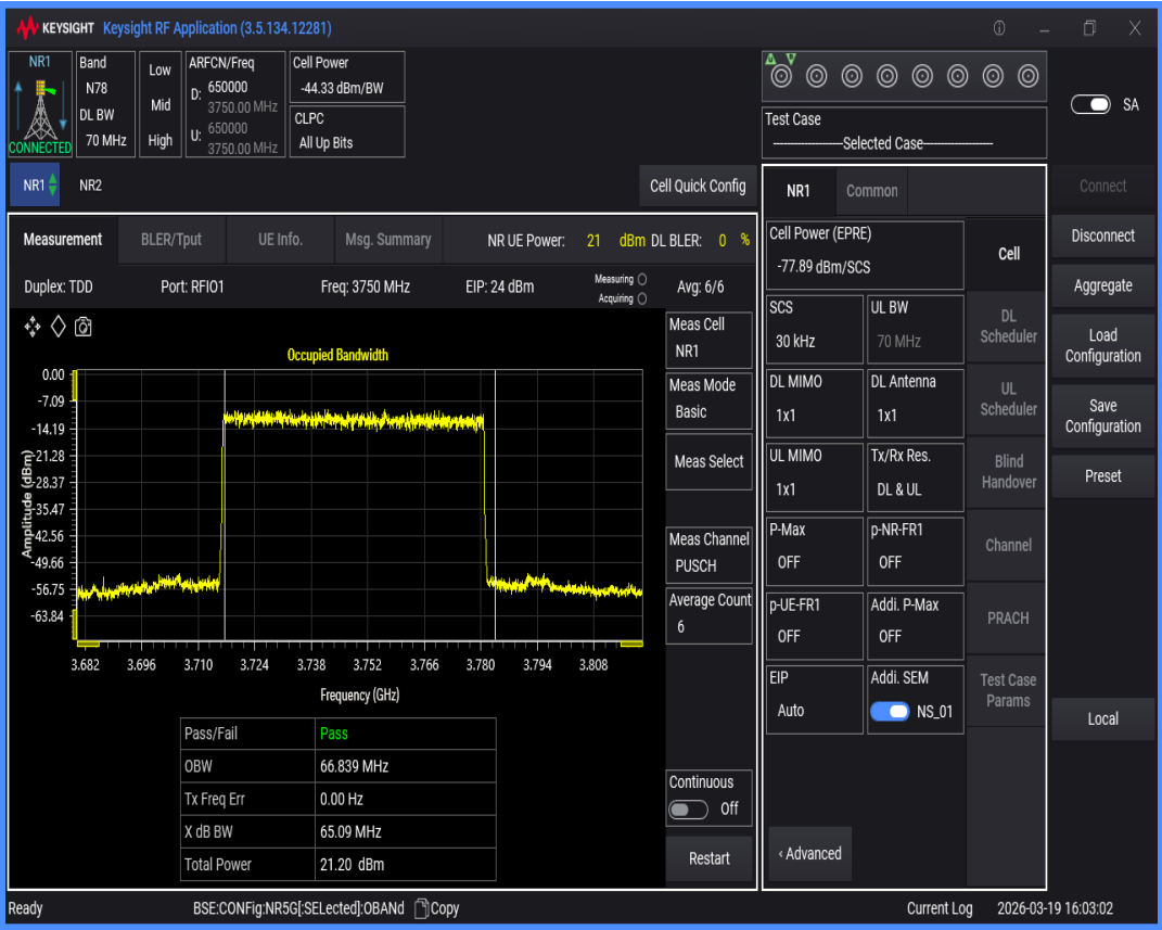
n78(3700-3800) SCS=30kHz DFT_QAM256 BW=80MHz Channel=650000 RB=216@0
