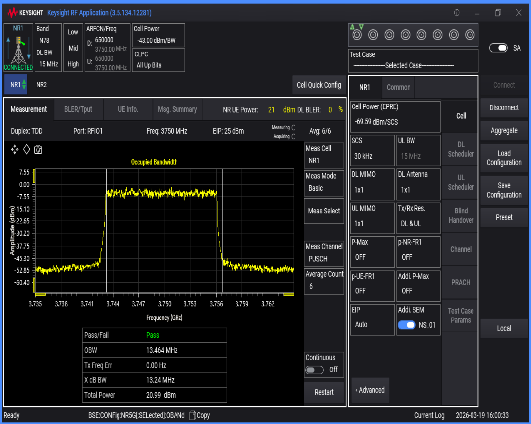
n78(3700-3800) SCS=30kHz DFT_QAM256 BW=30MHz Channel=650000 RB=75@0
