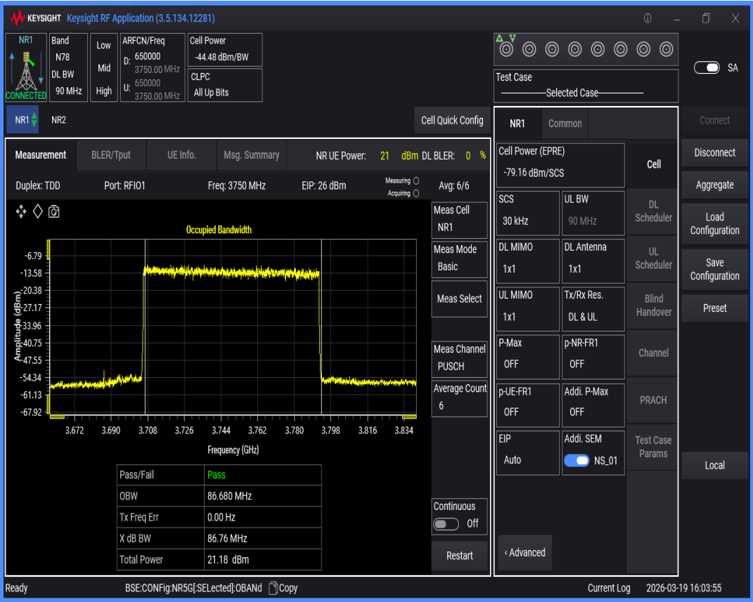
n78(3700-3800) SCS=30kHz DFT_QAM64 BW=10MHz Channel=650000 RB=24@0
