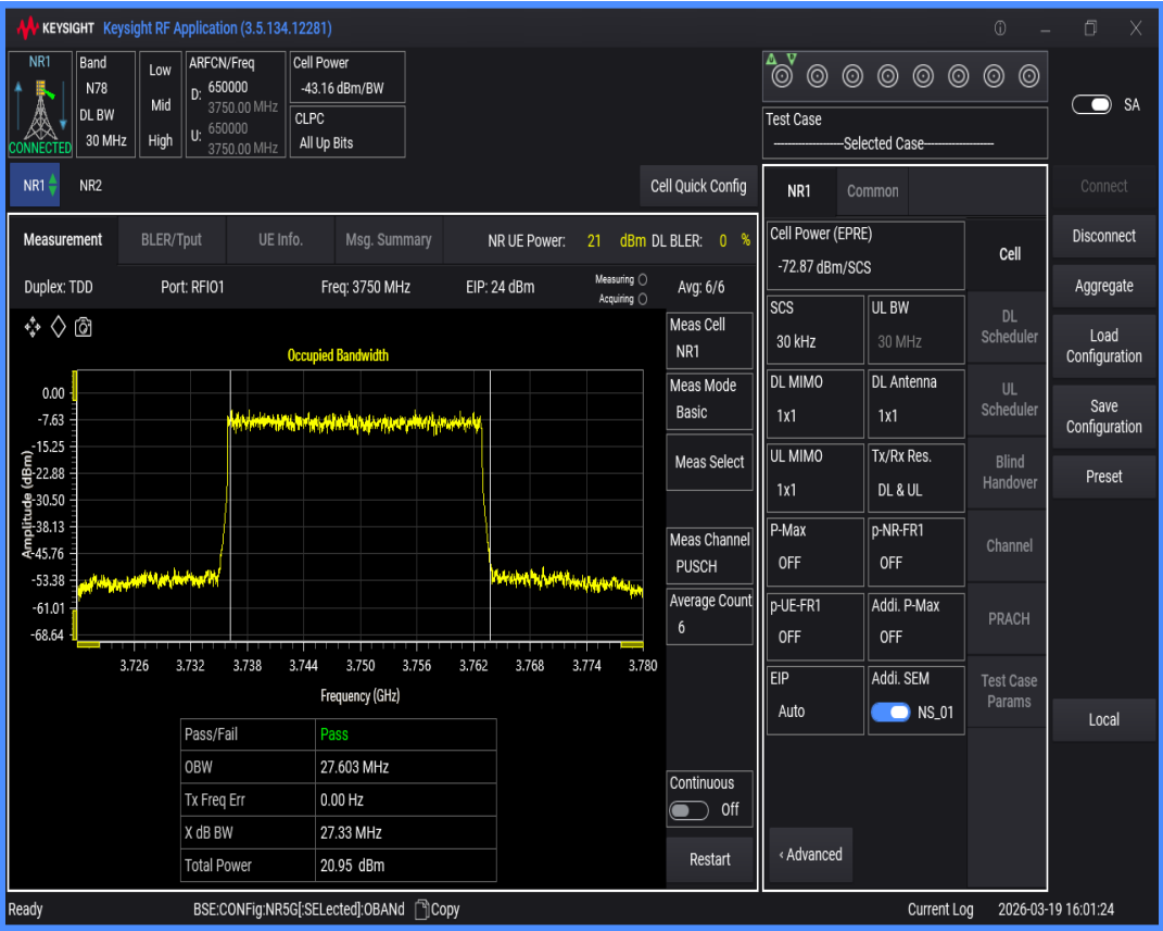
n78(3700-3800) SCS=30kHz DFT_QAM256 BW=40MHz Channel=650000 RB=100@0
