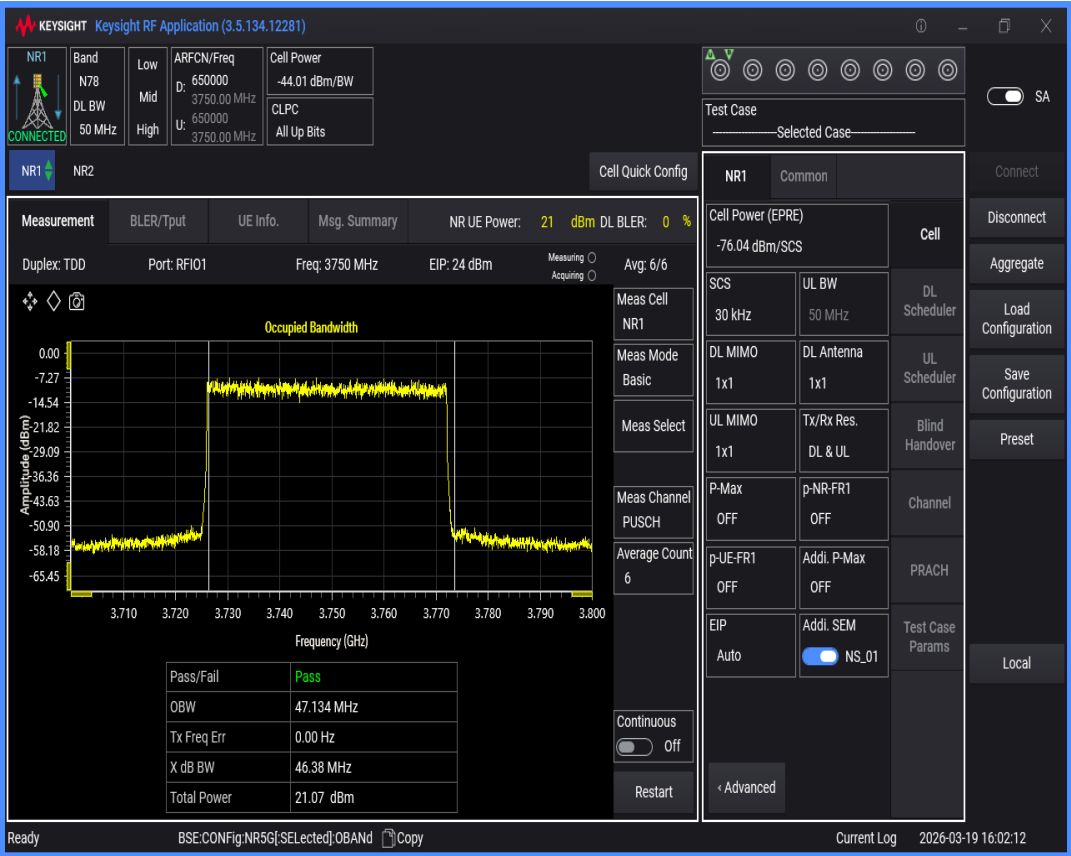
n78(3700-3800) SCS=30kHz DFT_QAM256 BW=70MHz Channel=650000 RB=180@0
