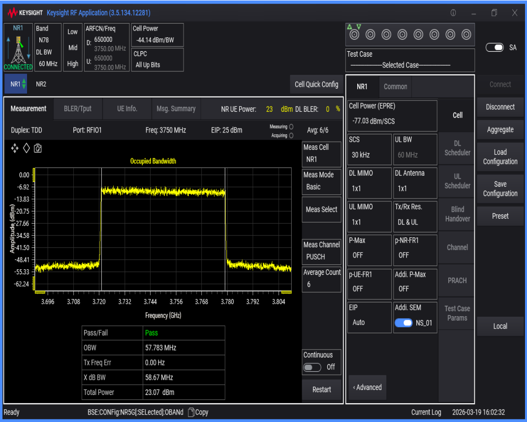
n78(3700-3800) SCS=30kHz DFT_QAM64 BW=70MHz Channel=650000 RB=180@0
