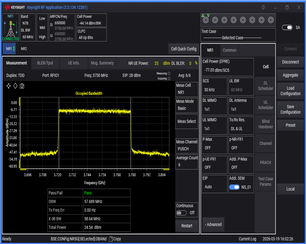
n78(3700-3800) SCS=30kHz DFT_QPSK BW=70MHz Channel=650000 RB=180@0
