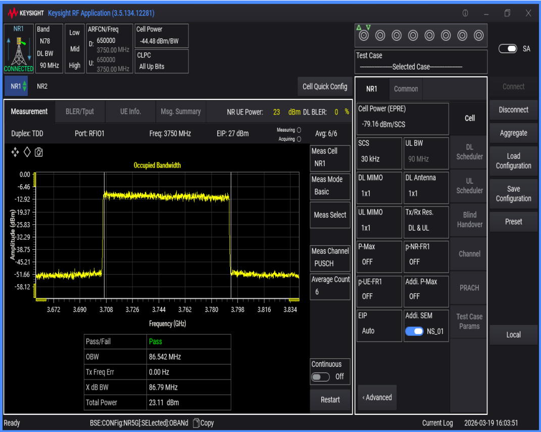
n78(3700-3800) SCS=30kHz DFT_QPSK BW=100MHz Channel=650000 RB=270@0
