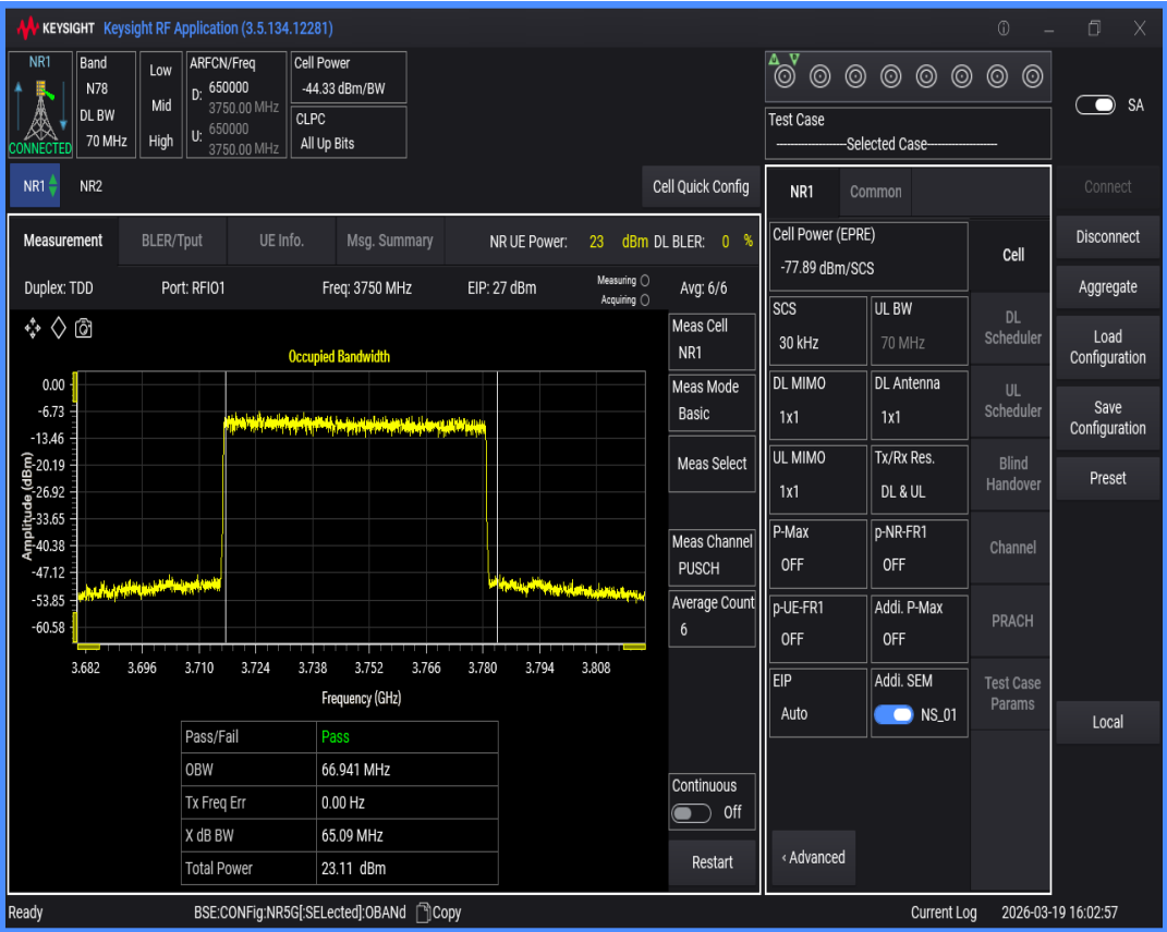
n78(3700-3800) SCS=30kHz DFT_QAM64 BW=80MHz Channel=650000 RB=216@0
