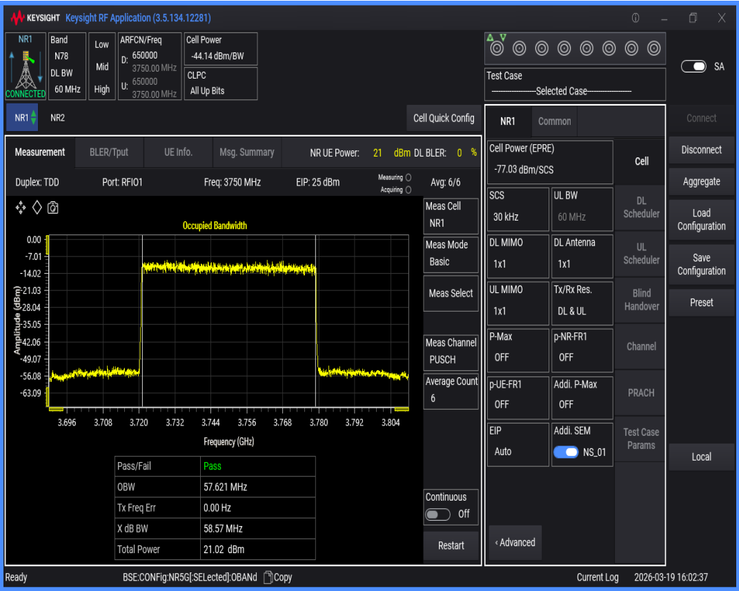
n78(3700-3800) SCS=30kHz DFT_QAM256 BW=50MHz Channel=650000 RB=128@0
