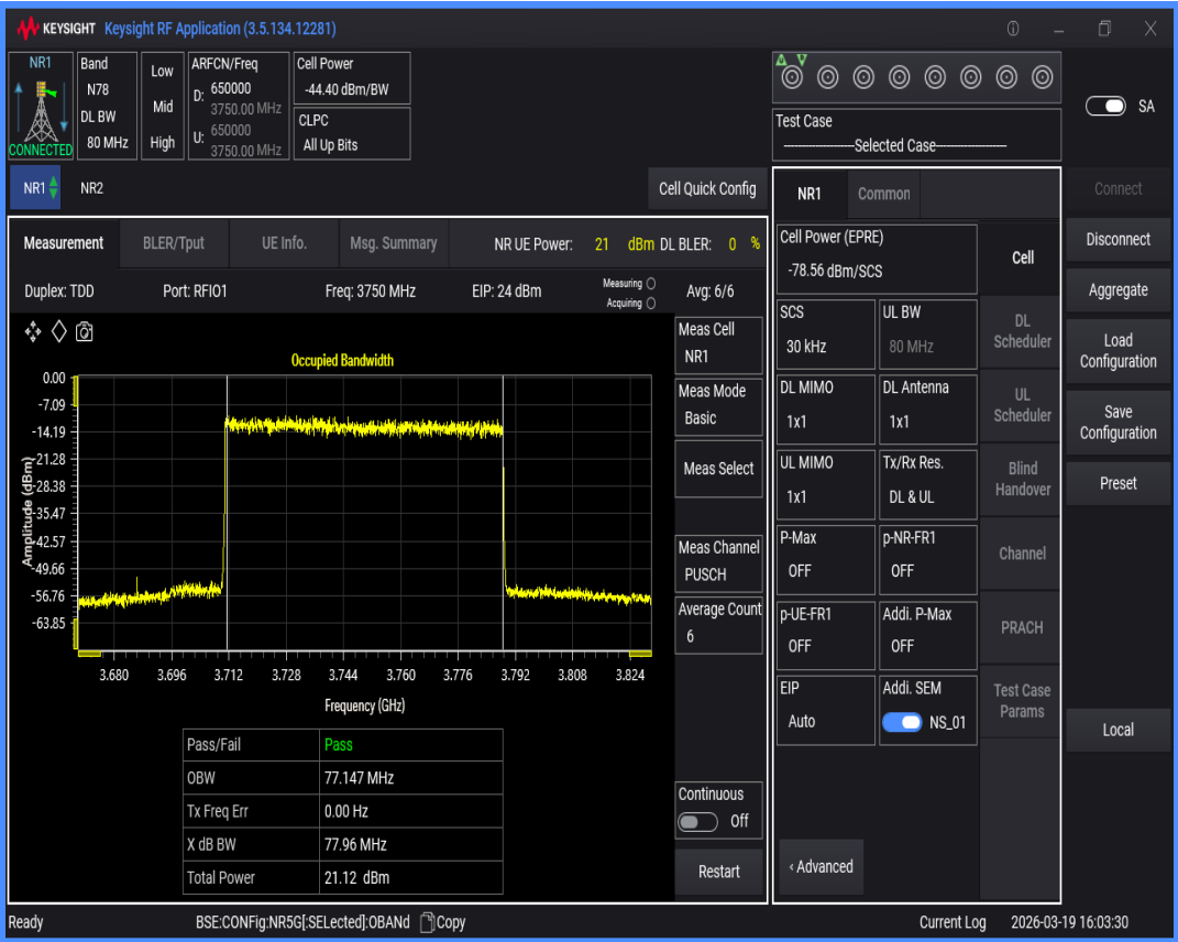
n78(3700-3800) SCS=30kHz DFT_QAM256 BW=90MHz Channel=650000 RB=240@0
