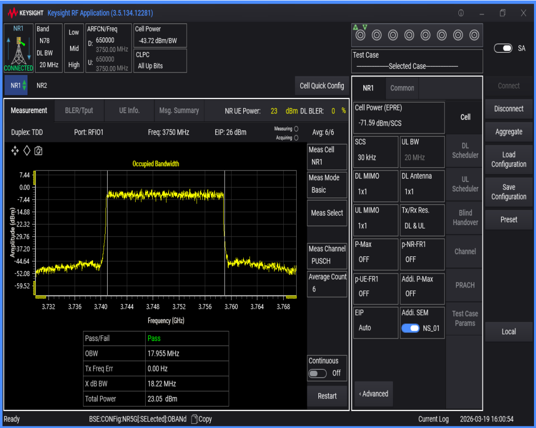
n78(3700-3800) SCS=30kHz DFT_QAM64 BW=40MHz Channel=650000 RB=100@0
