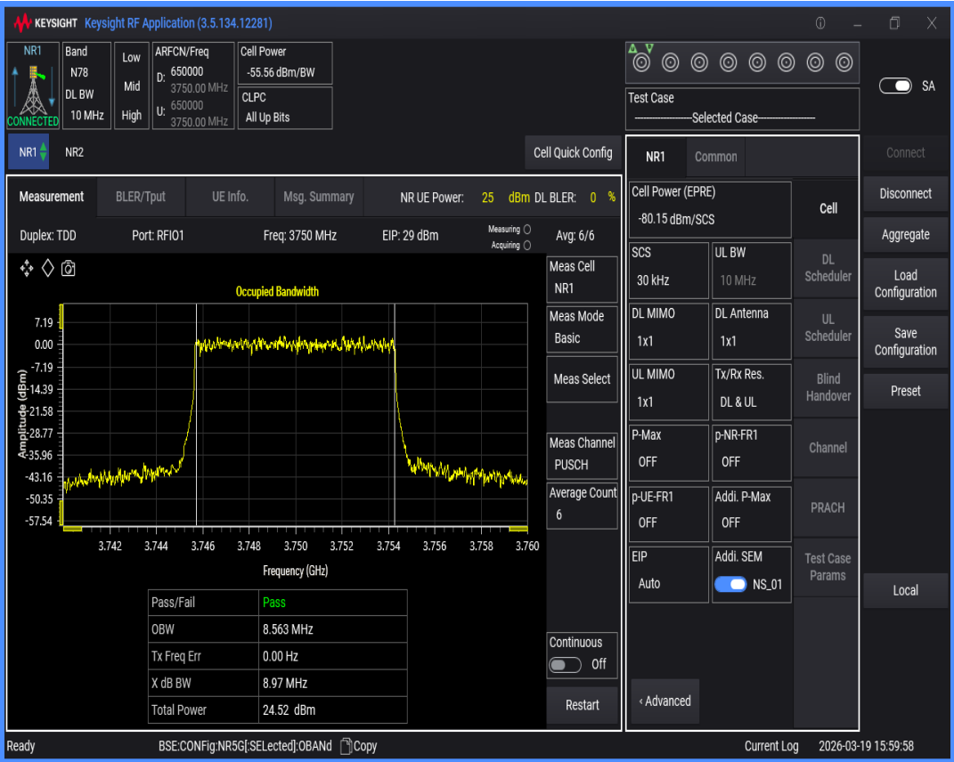
n78(3700-3800) SCS=30kHz DFT_QPSK BW=15MHz Channel=650000 RB=36@0
