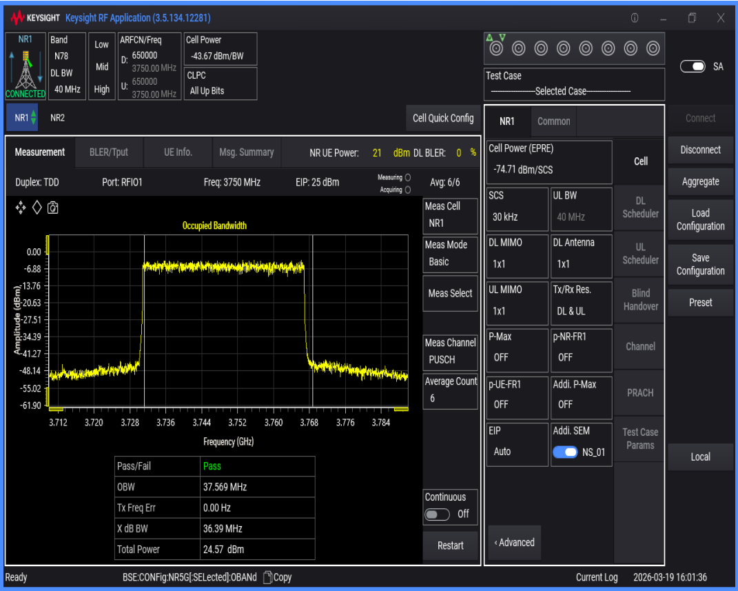
n78(3700-3800) SCS=30kHz DFT_QPSK BW=60MHz Channel=650000 RB=162@0
