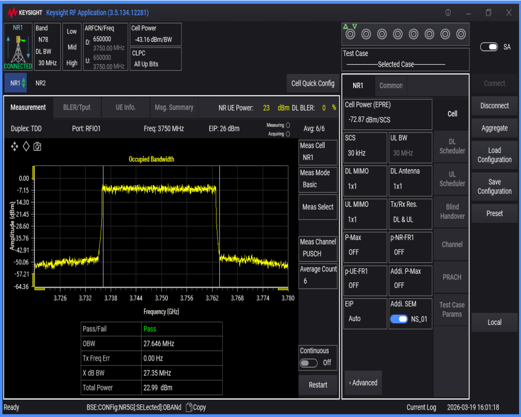
n78(3700-3800) SCS=30kHz DFT_QAM64 BW=20MHz Channel=650000 RB=50@0
