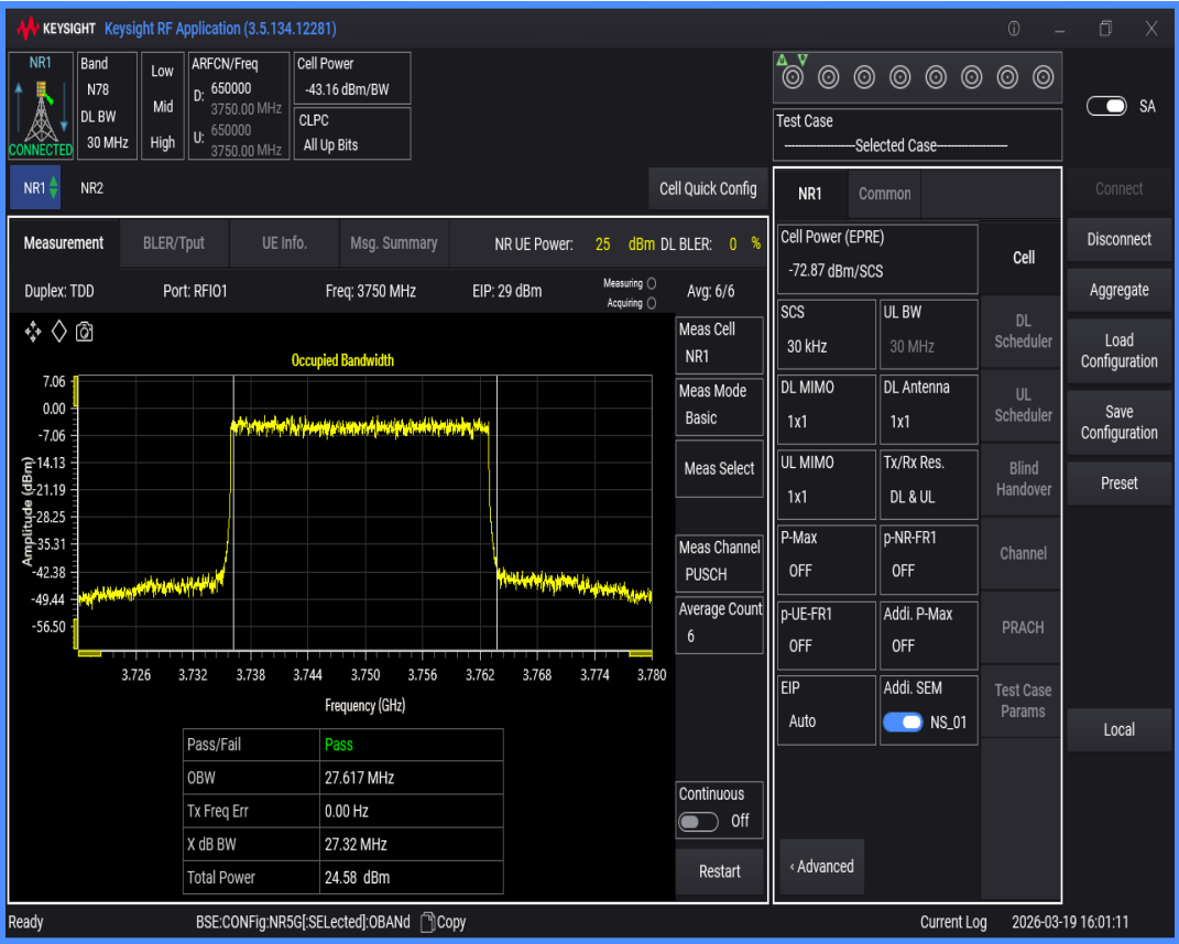
n78(3700-3800) SCS=30kHz DFT_QPSK BW=50MHz Channel=650000 RB=128@0
