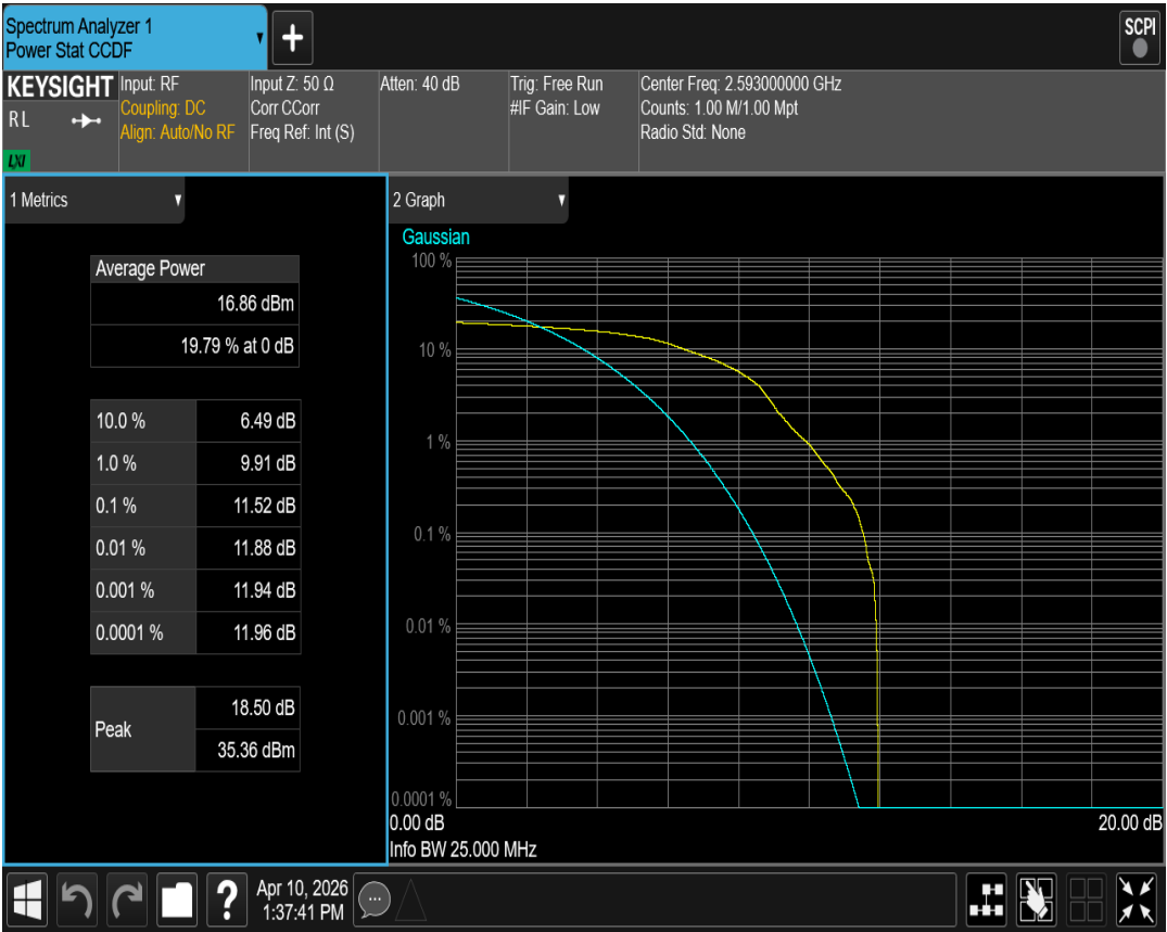
Band41 QAM16 BW=20MHz Channel=40620 RB Size=1 Position=#0
