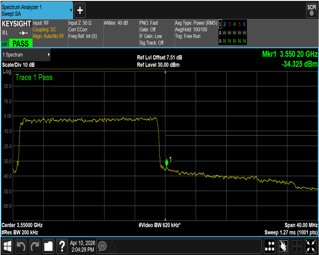
Band42(3450-3550) QPSK BW=5MHz Channel=42115 RB Size=25 Position=#0
