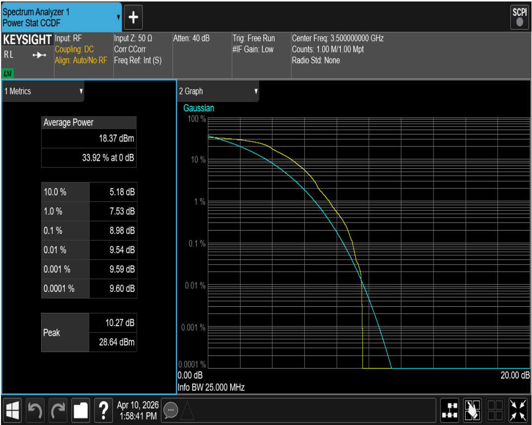
Band42(3450-3550) QPSK BW=15MHz Channel=42590 RB Size=1 Position=#0
