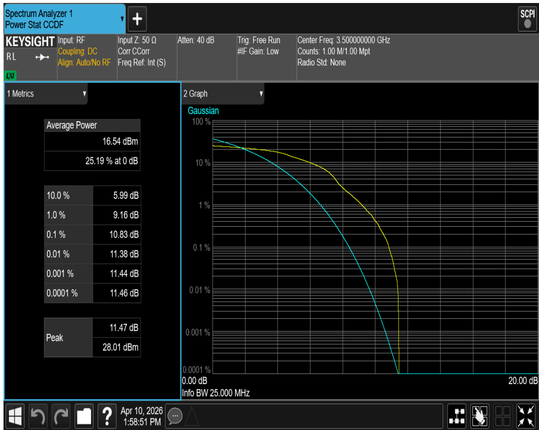
Band42(3450-3550) QPSK BW=20MHz Channel=42590 RB Size=1 Position=#0
