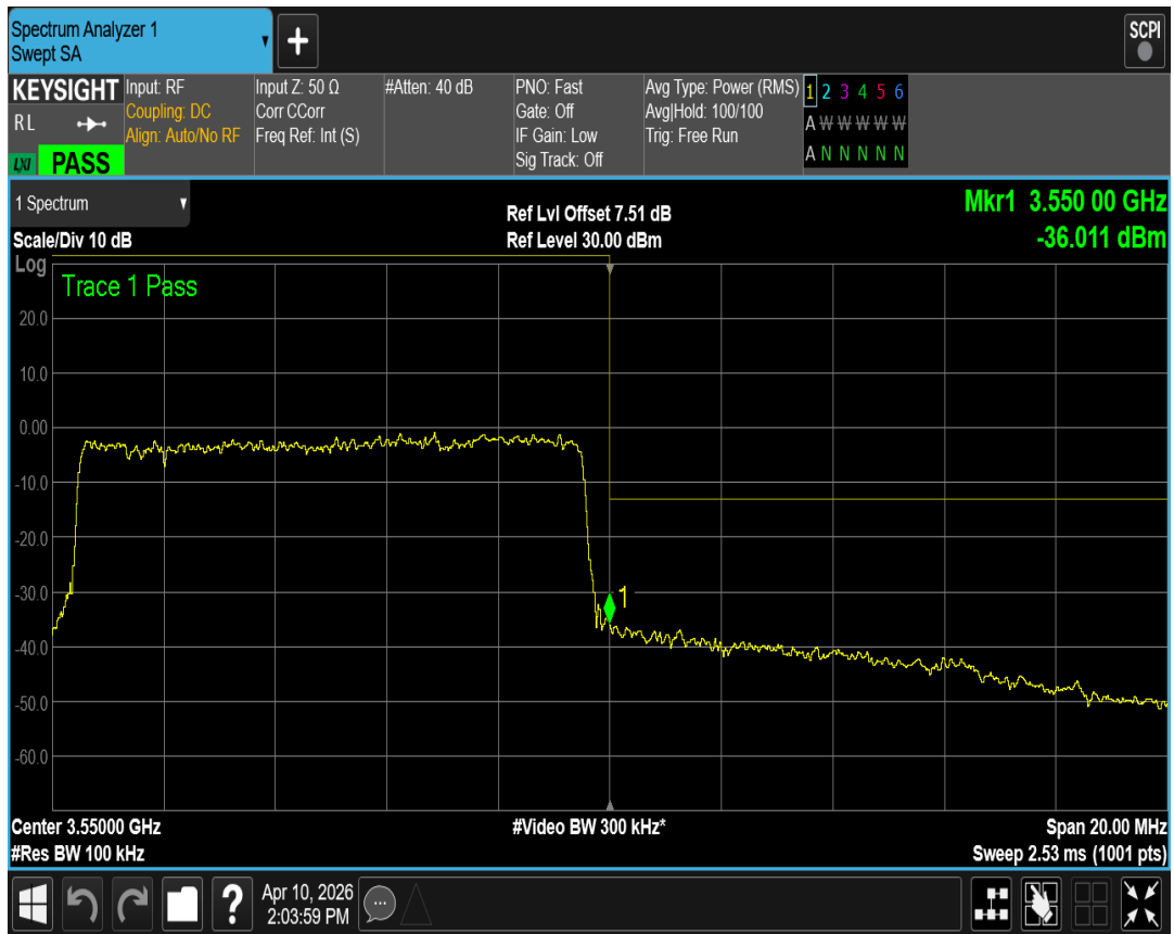
Band42(3450-3550) QAM16 BW=20MHz Channel=42190 RB Size=100 Position=#0
