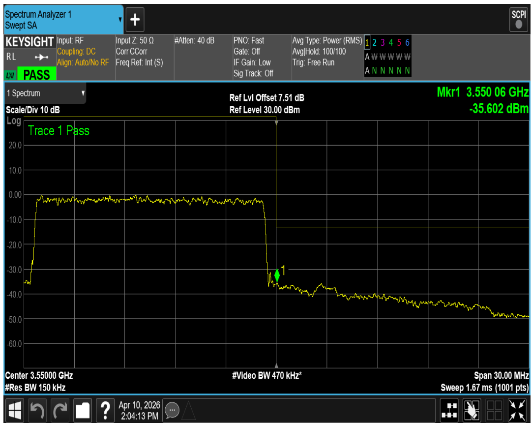
Band42(3450-3550) QPSK BW=20MHz Channel=42190 RB Size=100 Position=#0
