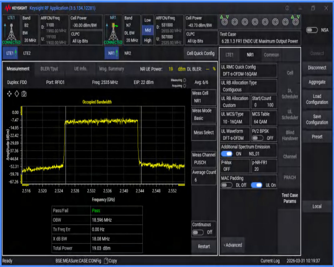
n7 SCS=15kHz DFT_BPSK BW=15MHz Channel=507000 RB=75@0
