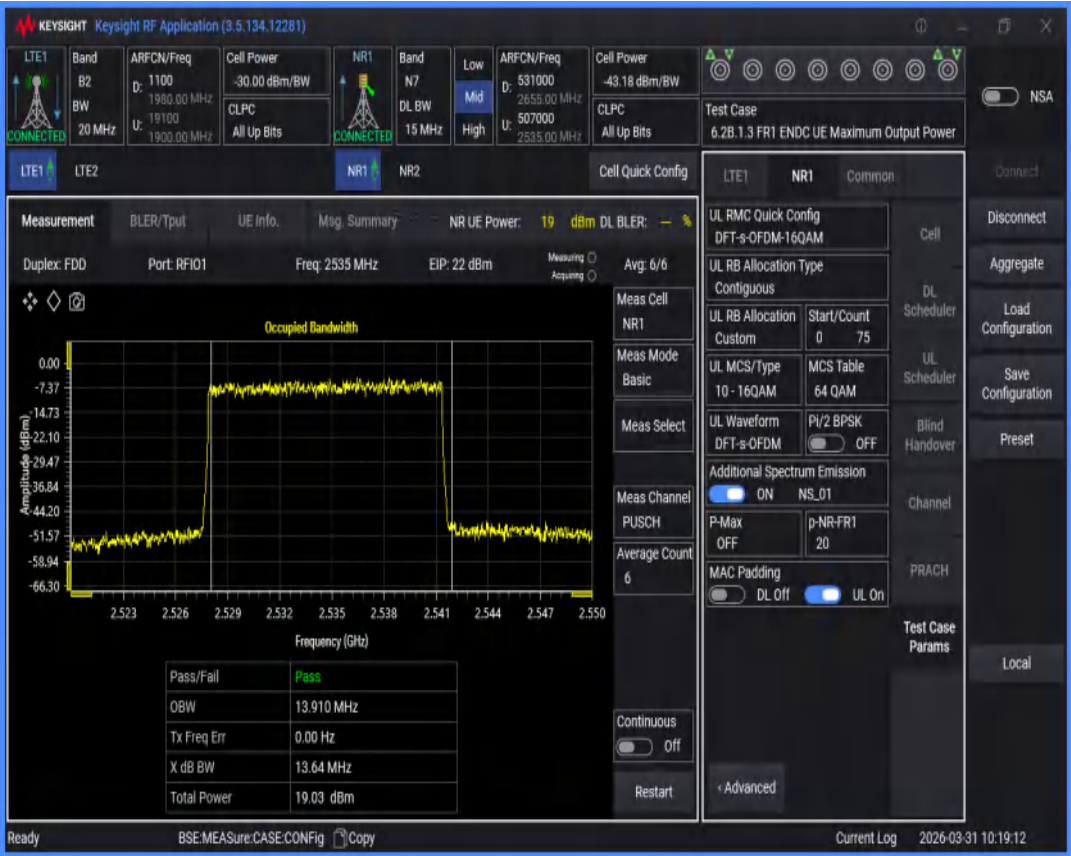
n7 SCS=15kHz DFT_QAM16 BW=20MHz Channel=507000 RB=100@0
