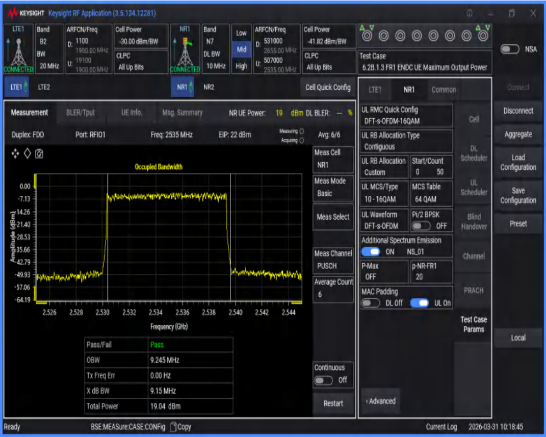
n7 SCS=15kHz DFT_QAM16 BW=15MHz Channel=507000 RB=75@0
