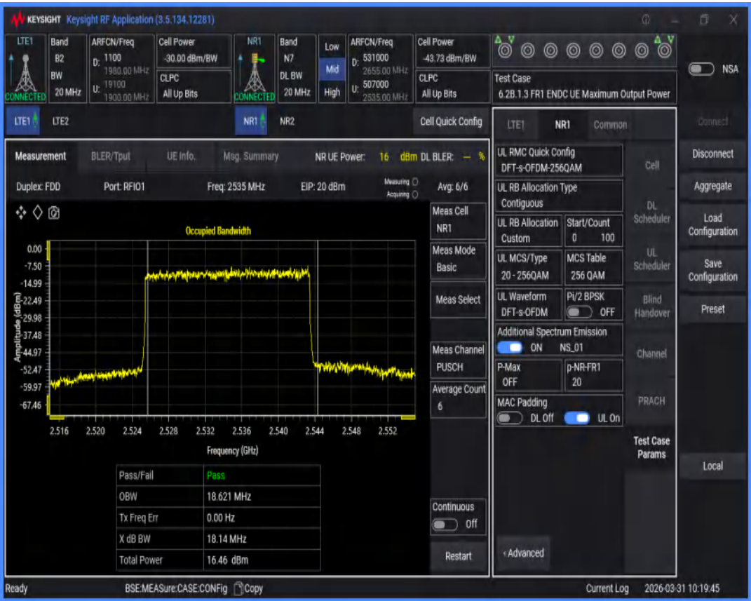
n7 SCS=15kHz DFT_QAM256 BW=5MHz Channel=507000 RB=25@0
