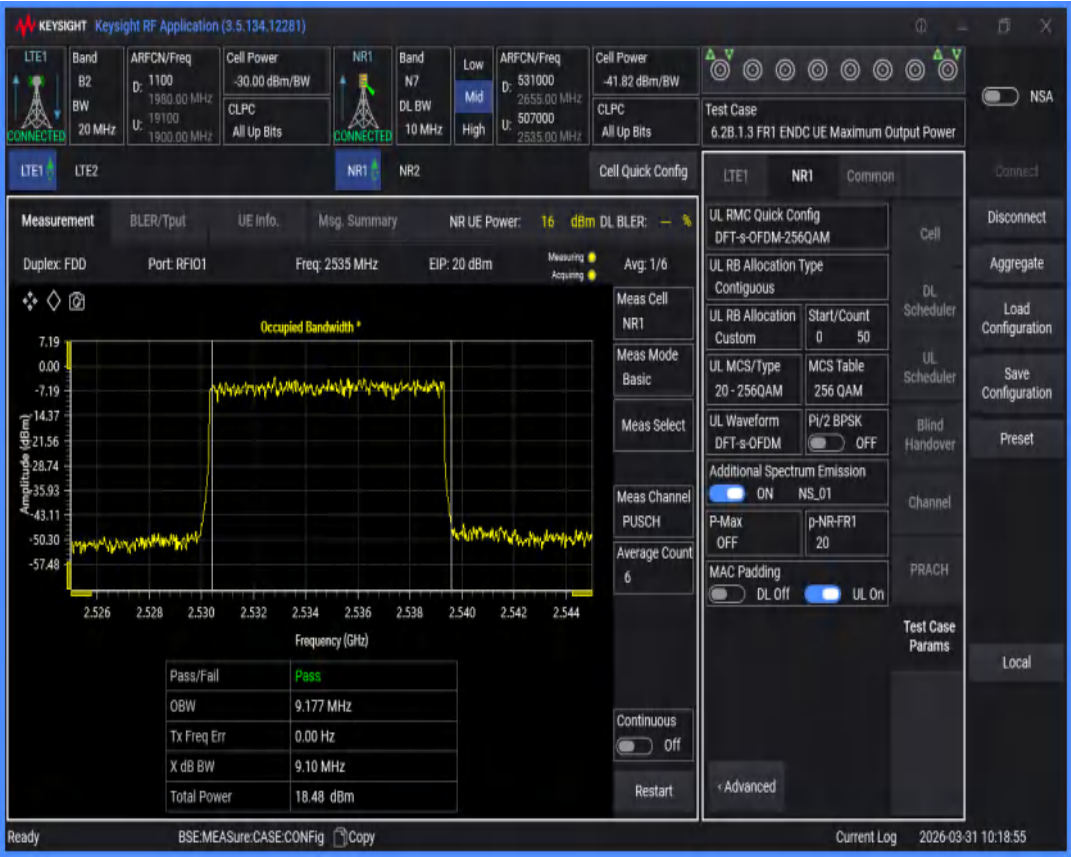
n7 SCS=15kHz DFT_QAM256 BW=15MHz Channel=507000 RB=75@0
