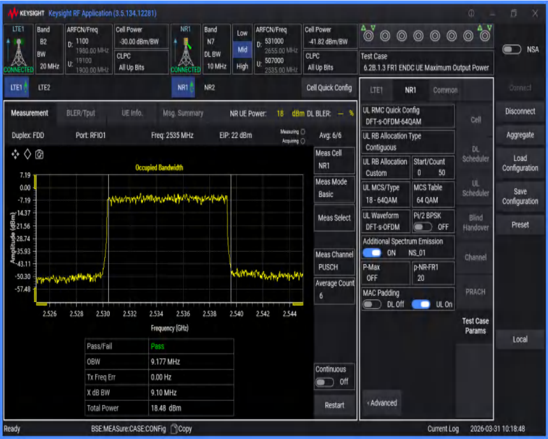
n7 SCS=15kHz DFT_QAM16 BW=5MHz Channel=507000 RB=25@0
