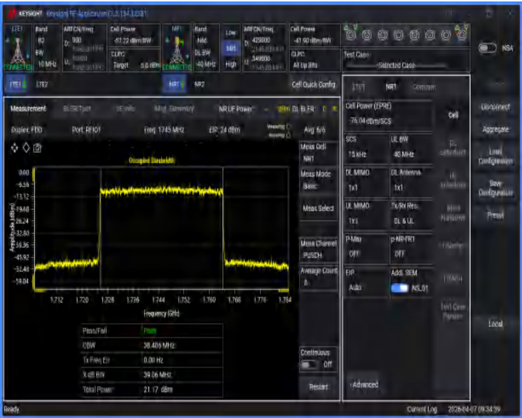
n66 SCS=15kHz DFT_QAM64 BW=20MHz Channel=349000 RB=100@0
