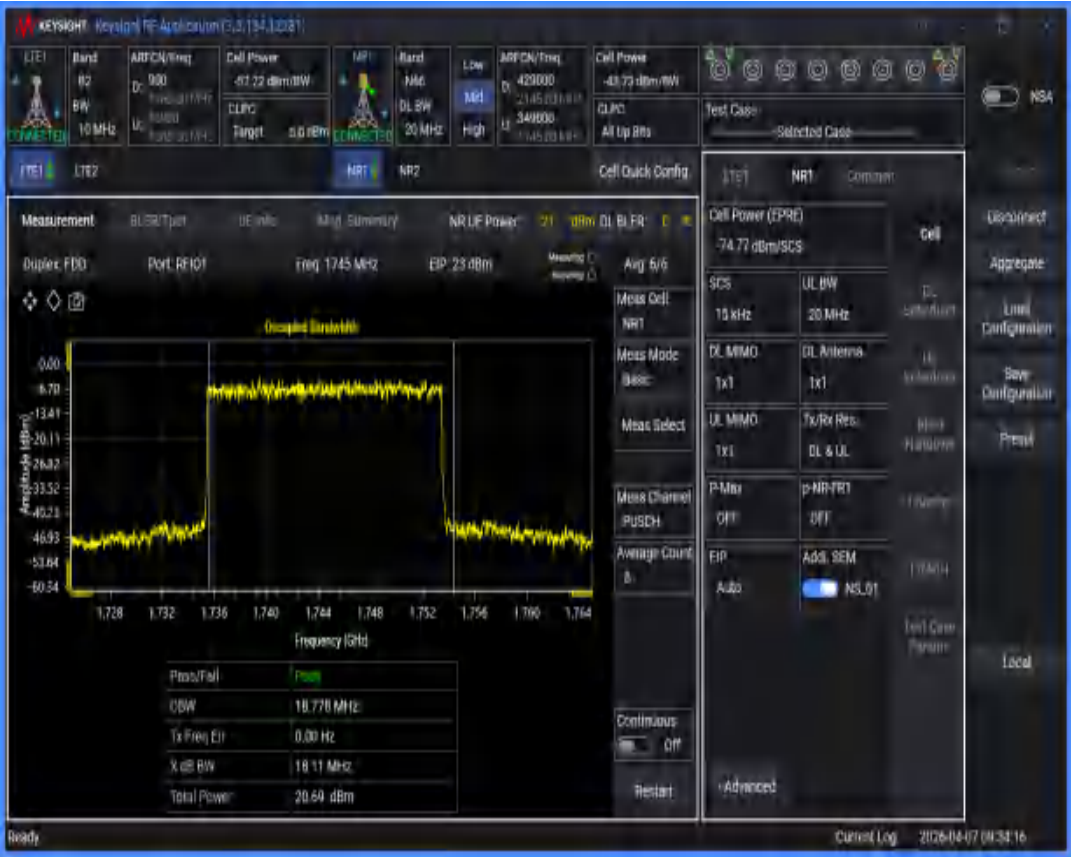
n66 SCS=15kHz DFT_QAM64 BW=40MHz Channel=349000 RB=216@0
