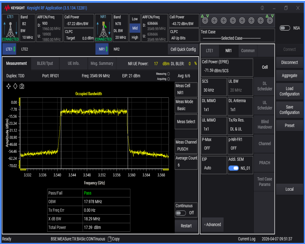
n78 SCS=30kHz DFT_QAM256 BW=60MHz Channel=636666 RB=162@0
