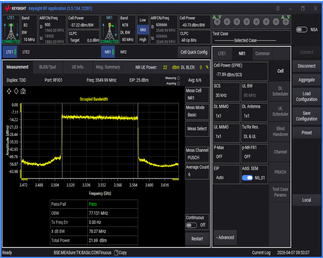
n78 SCS=30kHz DFT_BPSK BW=60MHz Channel=636666 RB=162@0
