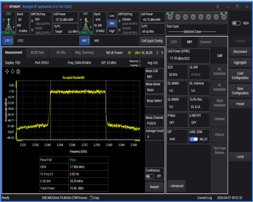
n78 SCS=30kHz DFT_QAM64 BW=40MHz Channel=636666 RB=100@0
