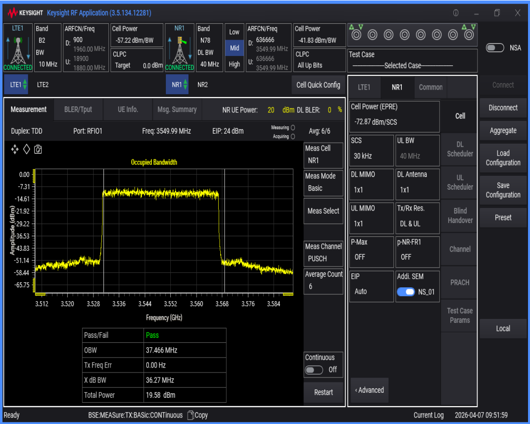
n78 SCS=30kHz DFT_QAM64 BW=10MHz Channel=636666 RB=24@0
