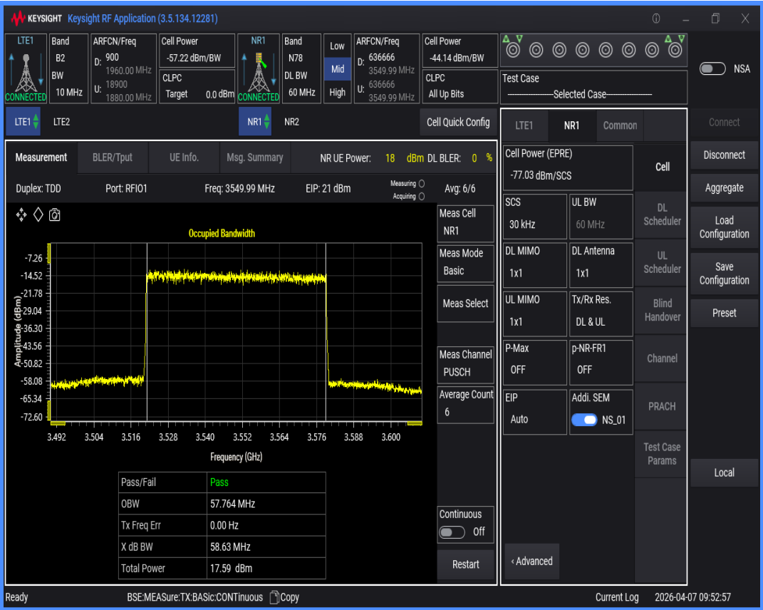
n78 SCS=30kHz DFT_QAM256 BW=50MHz Channel=636666 RB=128@0
