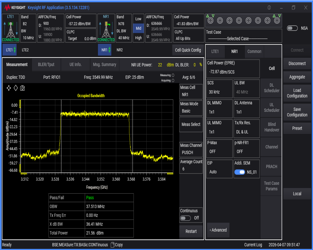
n78 SCS=30kHz DFT_QAM16 BW=50MHz Channel=636666 RB=128@0
