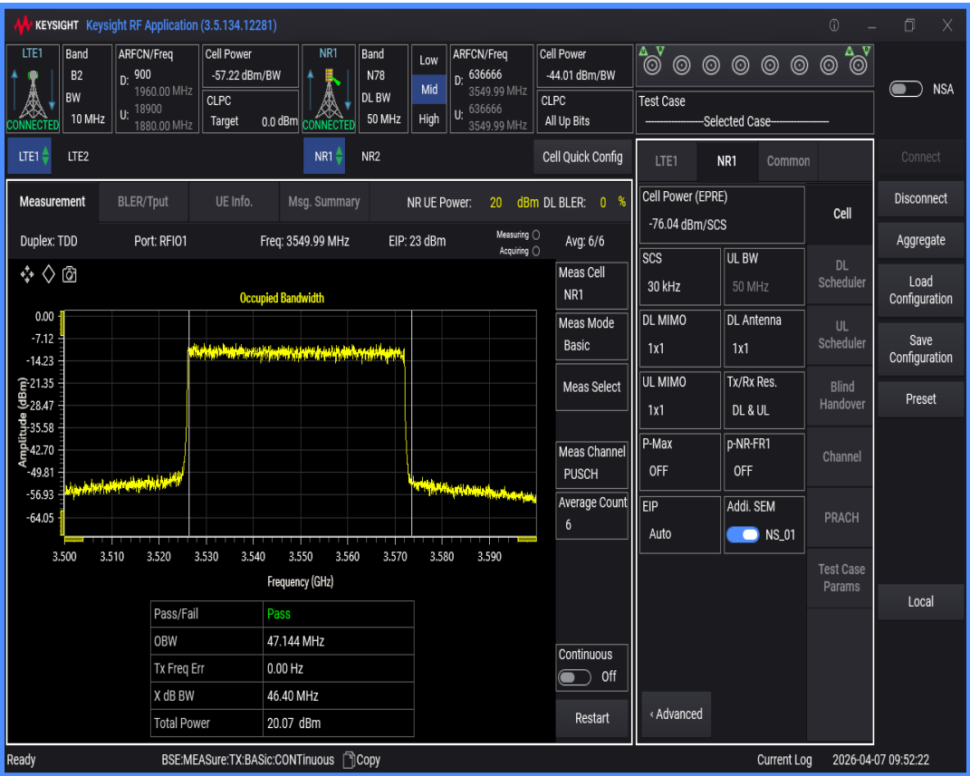
n78 SCS=30kHz DFT_QAM16 BW=60MHz Channel=636666 RB=162@0
