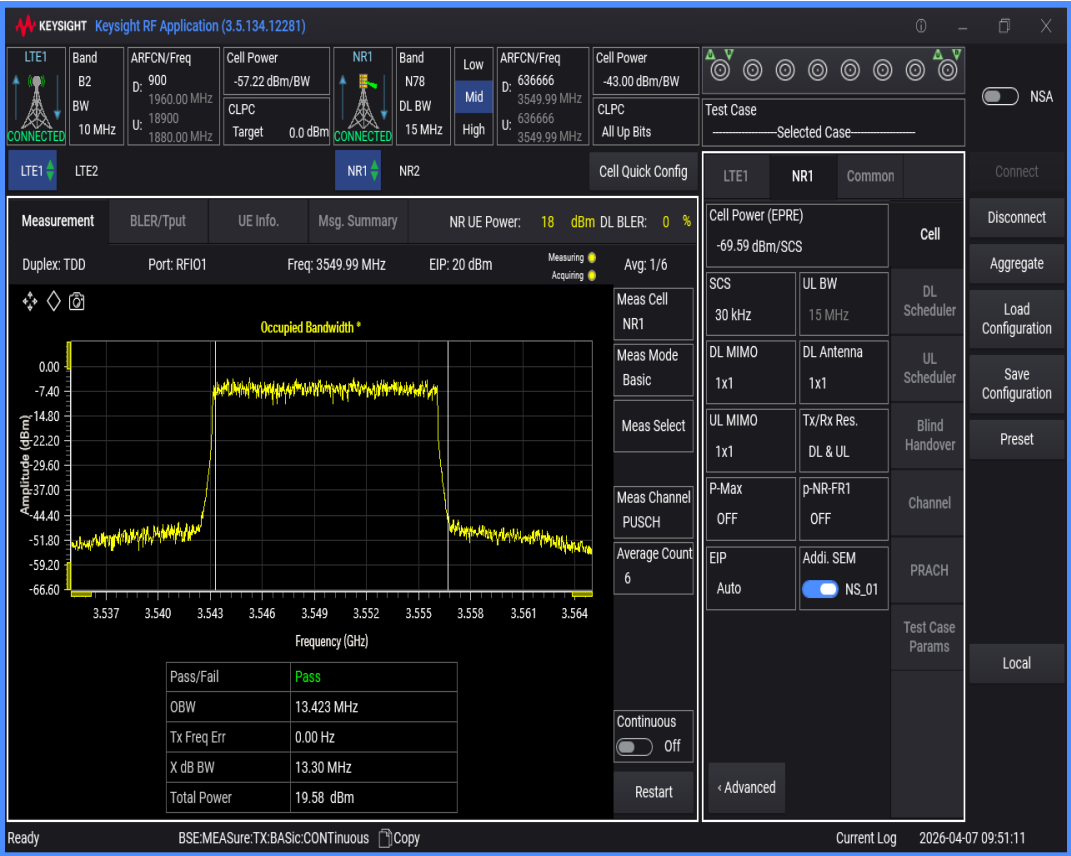
n78 SCS=30kHz DFT_QAM256 BW=10MHz Channel=636666 RB=24@0
