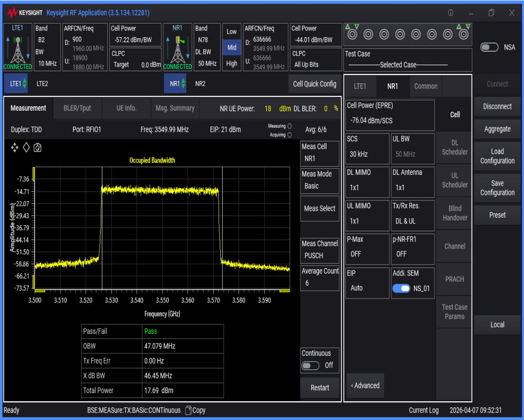
n78 SCS=30kHz DFT_QAM256 BW=100MHz Channel=636666 RB=270@0
