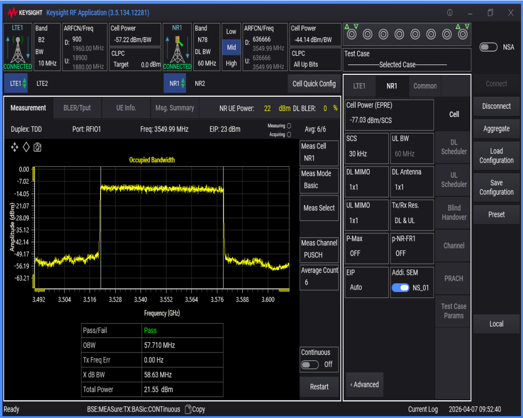
n78 SCS=30kHz DFT_QAM16 BW=100MHz Channel=636666 RB=270@0
