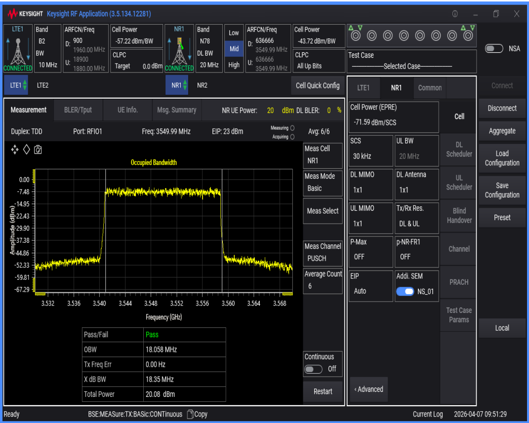
n78 SCS=30kHz DFT_QAM256 BW=40MHz Channel=636666 RB=100@0
