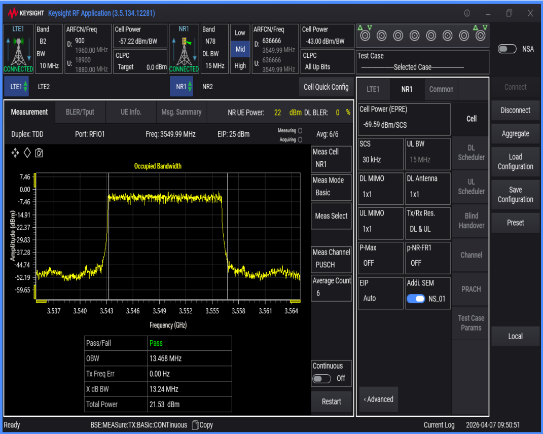
n78 SCS=30kHz DFT_BPSK BW=50MHz Channel=63666 RB=128@0
