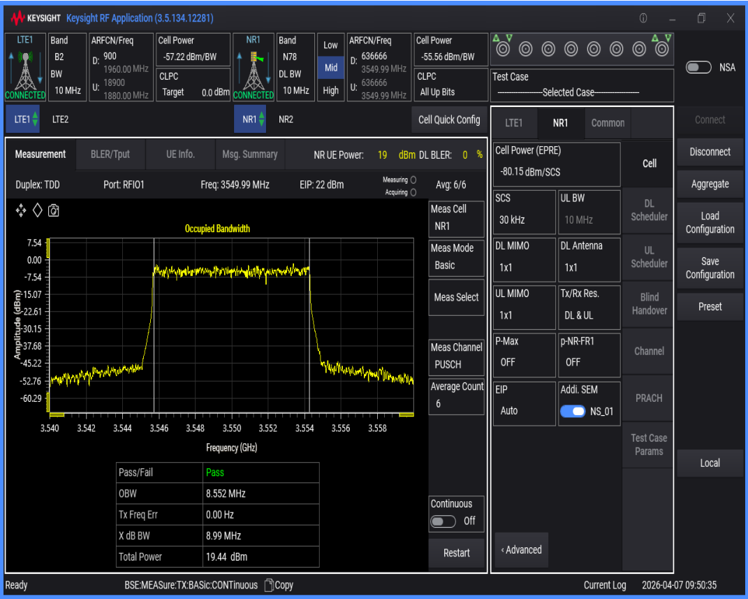
n78 SCS=30kHz DFT_QAM256 BW=80MHz Channel=636666 RB=216@0
