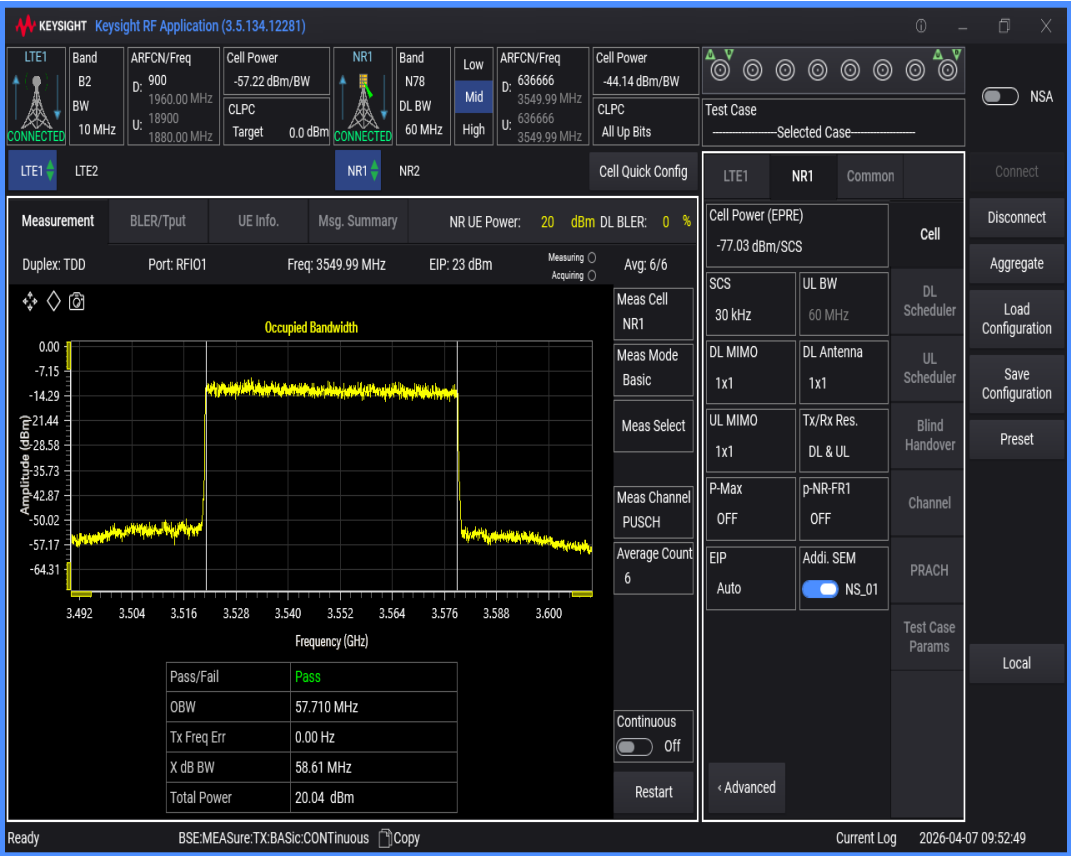
n78 SCS=30kHz DFT_QAM16 BW=80MHz Channel=636666 RB=216@0
