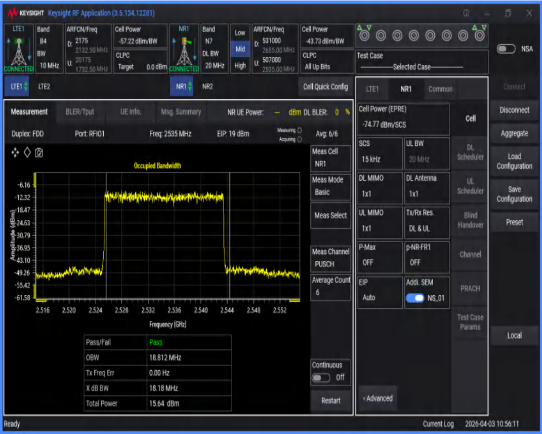
n7 SCS=15kHz DFT_QAM256 BW=15MHz Channel=507000 RB=75@0
