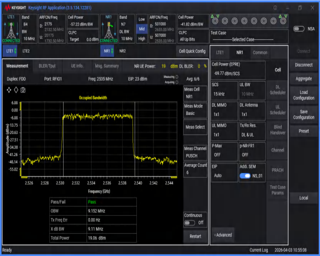
n7 SCS=15kHz DFT_QAM64 BW=5MHz Channel=507000 RB=25@0
