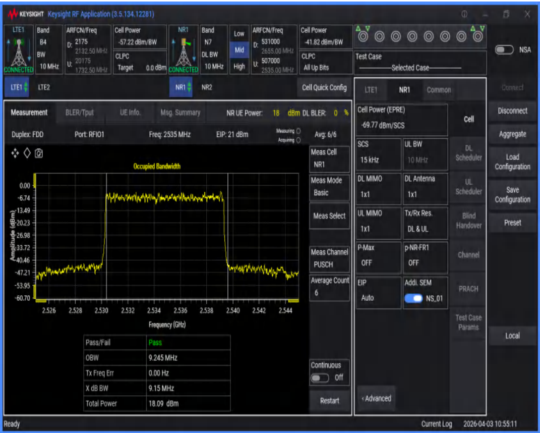
n7 SCS=15kHz DFT_QAM16 BW=5MHz Channel=507000 RB=25@0
