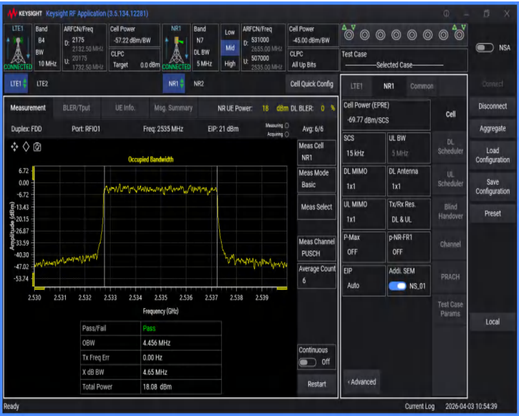
n7 SCS=15kHz DFT_QAM16 BW=20MHz Channel=507000 RB=100@0
