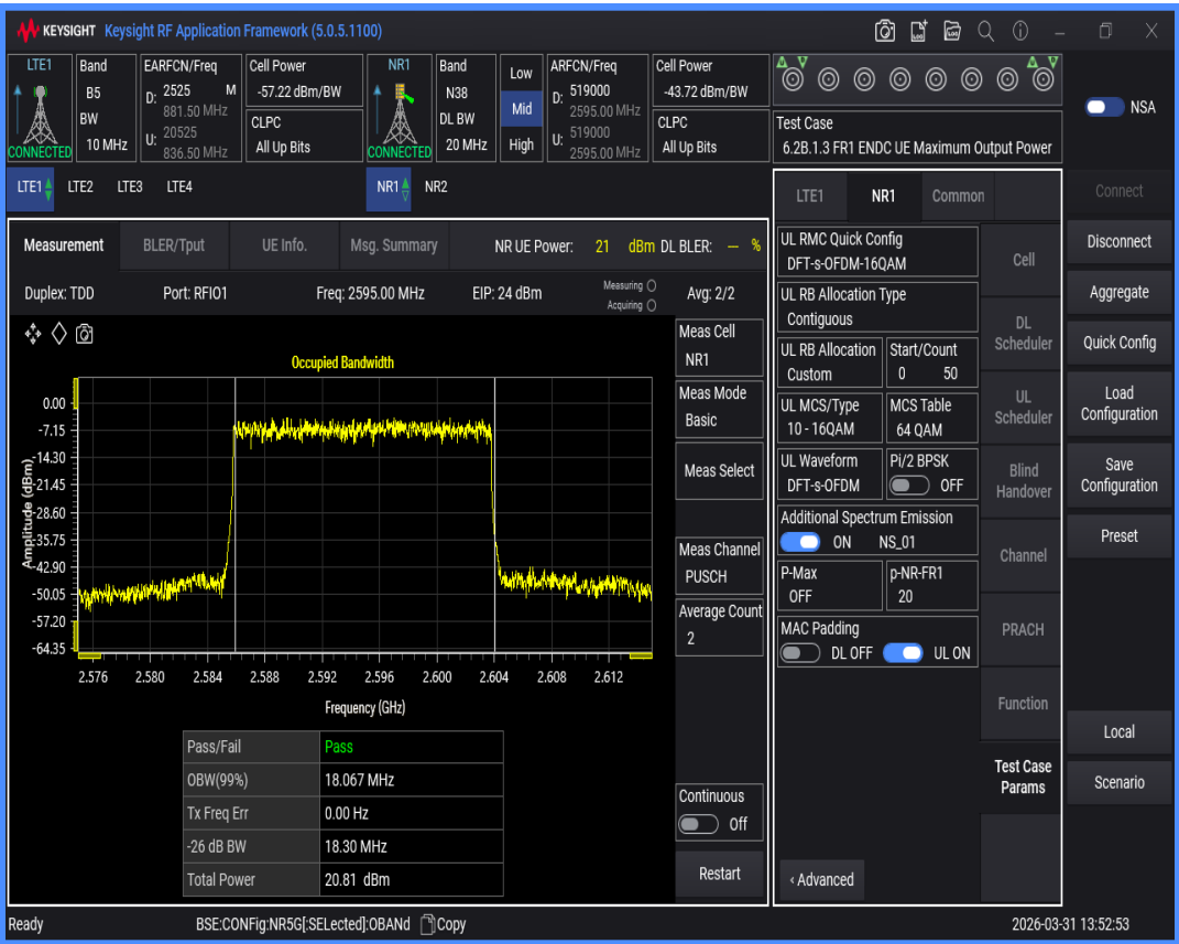
n38 SCS=30kHz DFT_QAM64 BW=10MHz Channel=519000 RB=24@0
